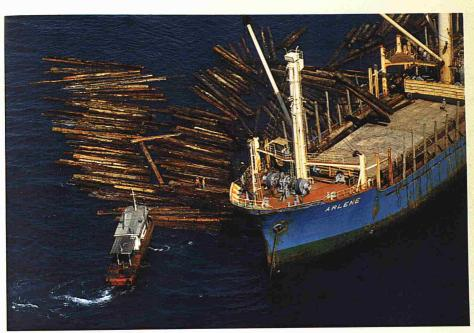
oter makes on efficient transport system for cut logs. They are floated down rivers in log rofts, corrolled and pushed into place by small specially and then loaded from out of the water.
