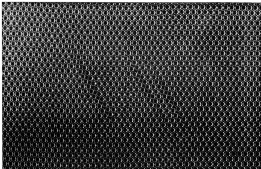
FIGURE 7. Parallel dislocations. Diameter 0.76 mm.
