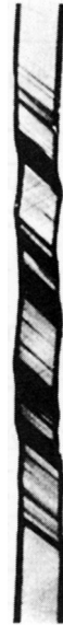
Fig. 30-12. A photograph of a small crystal of copper after stretching. [Courtesy of S. S. Brenner, Senior Scientist, United States Steel Research Center, Monroeville, Pa.]
