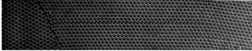
FIGURE 8. Dislocation projecting from a grain boundary. Diameter 0.30 mm.
