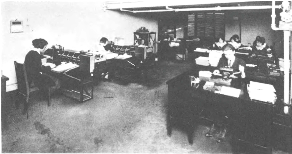
7.2 A punch card “data center,” circa 1920. Notice single card punching on right, volume work on left, and the vertical sorter in upper left-hand corner (courtesy IBM Archives).
