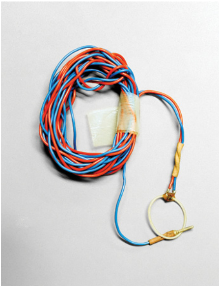
Figure 2.2 A mercury-in-rubber penile strain gauge. The loop at the end of the wires is placed around the base of the penis and measures changes in penile circumference. © Sarah Sudhoff.
