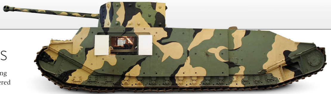
△ TOG II* Date 1941 Country UK Weight 89.6 tons (81.3 tonnes) Engine Paxman Ricardo 12-cylinder diesel, 600 hp Main armament QF 17-pounder gun
