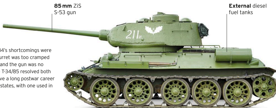
Turret welded for greater protection
