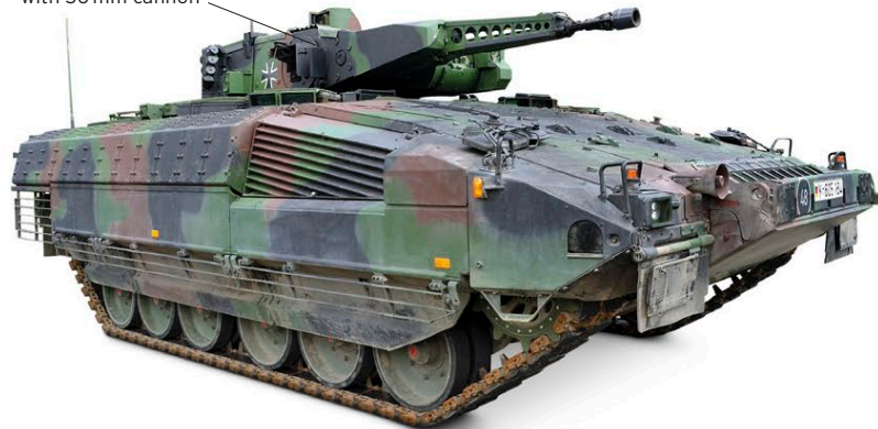
Unmanned turret with 30 mm cannon
