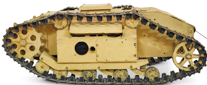
Mine housed in vehicle body
