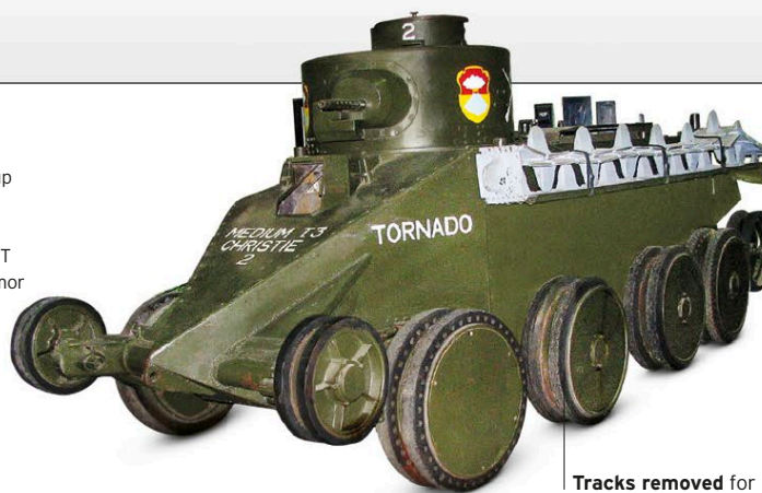
Tracks removed for increased speed
