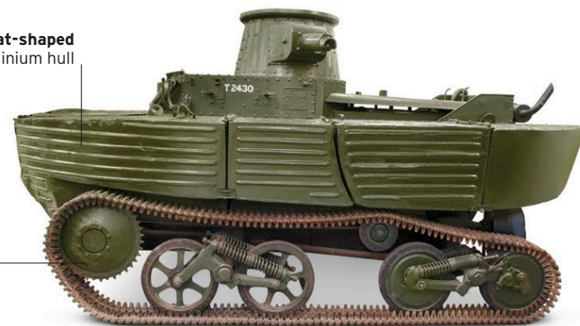
Hollow wheels assist buoyancy
