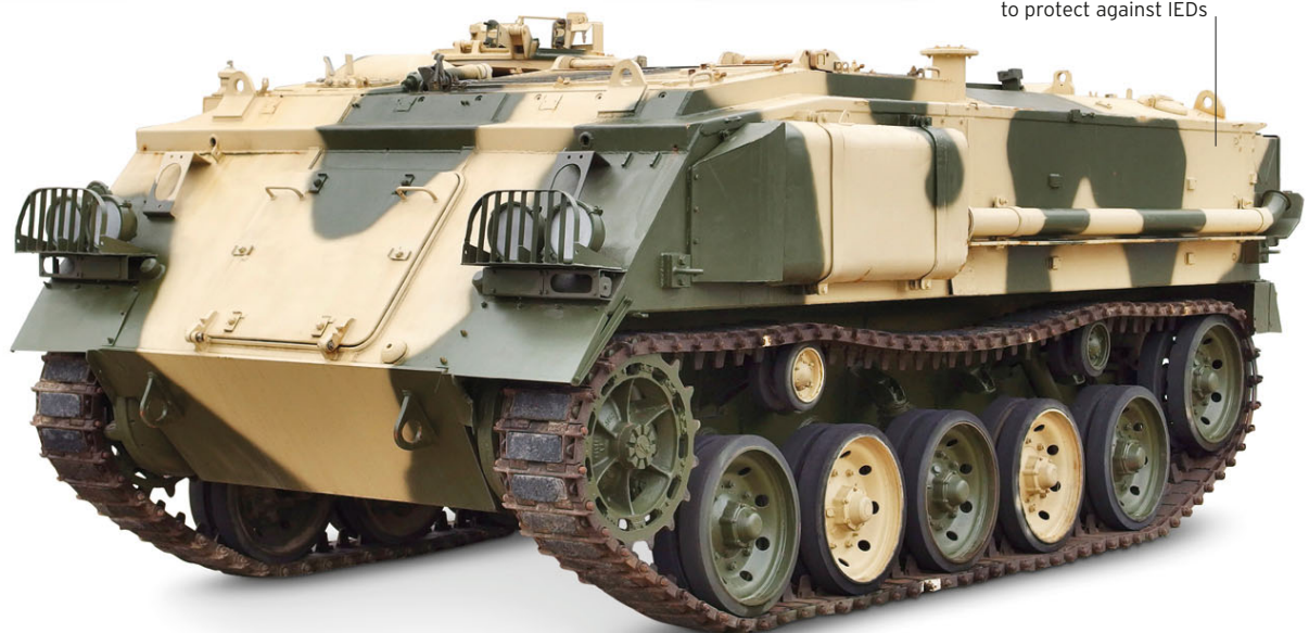
Armor includes kevlar plates to protect against IEDs
