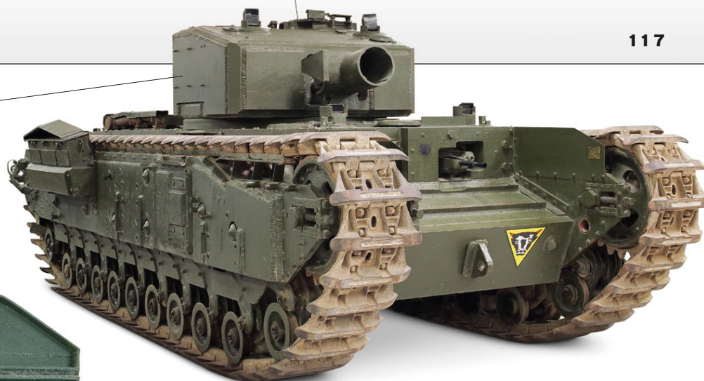
Turret houses 290 mm mortar
