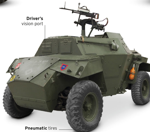
Armored body offered only limited protection
