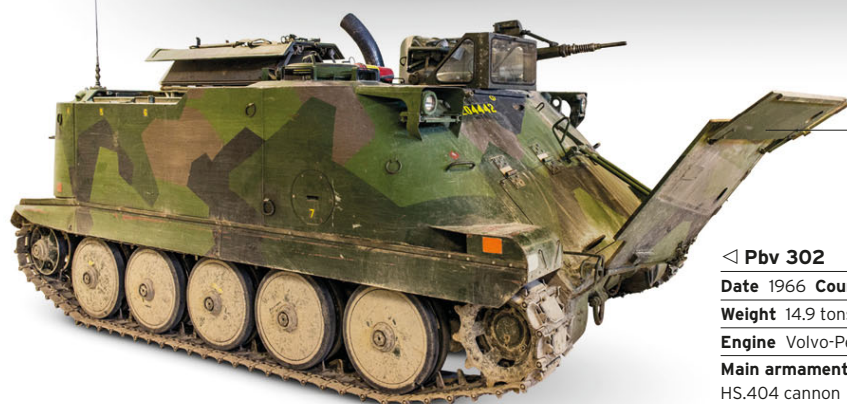
Trim vane used when fording rivers
