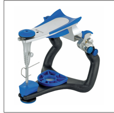
Fig 8-13 The average-value nonarcon articulator in the Artex range (AmannGirrbach) has a curved condylar path. The standard device is oriented to the Bonwill triangle and shows the occlusal plane; the Bennett angle is adjustable between 0 and 20 degrees, and the sagittal condylar path is in the range of 15 to 60 degrees. The exchangeable guide tables have an inclination of 10 to 20 degrees.
