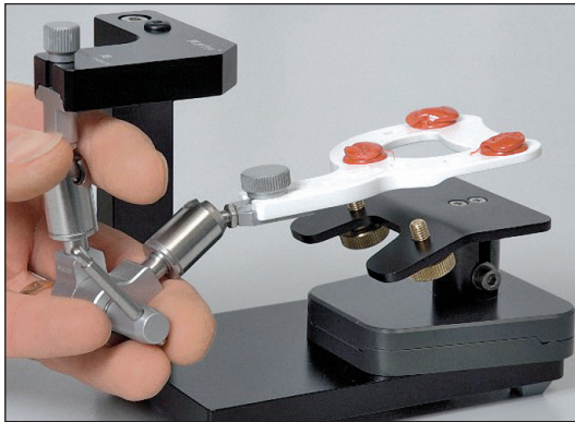
Fig 8-46 The three-dimensional joint support with bite fork is placed in a transfer stand and lies in a defined position over the transfer table, which has been adjusted to the mandibular model holder of the Artex articulator. (Courtesy of AmannGirrbach.)
