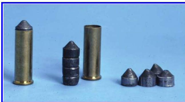
Figure 10.15 .38 Special round loaded with four 50 g bullets.
