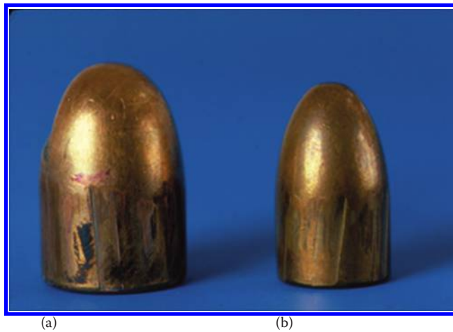
Figure 2.3 Two bullets fired from weapons with (a) left twist and (b) right twist to their rifling.
