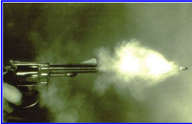
Figure 2.11 A cloud of gas can be seen emerging from the cylinder–barrel gap.
