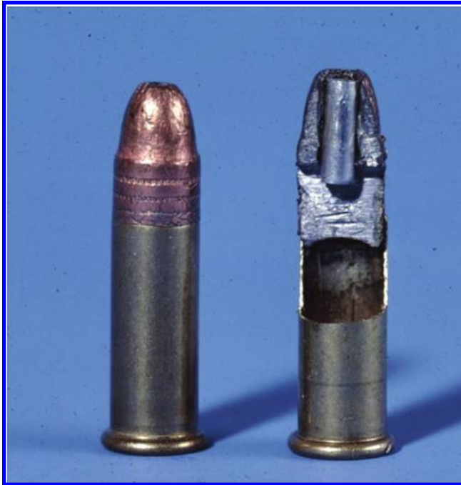
Figure 10.14 Longitudinal section through .22 caliber exploding round.
