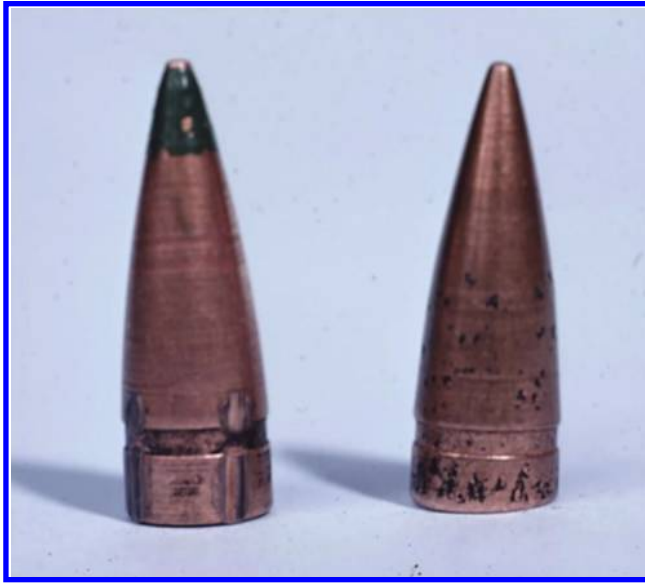
Figure 10.16 Military duplex round. Note the canted base of bullet on right.
