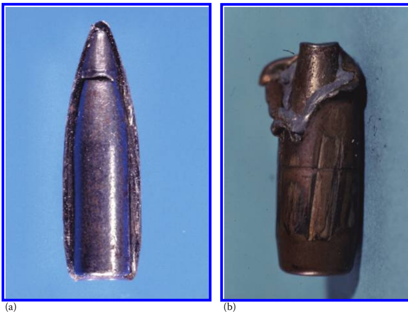
Figure 7.25 A 7.62 × 39 cartridge: (a) cross section of a steel-cored bullet with a lead tip and (b) tip of a bullet sheared off exposing steel core and lead sheath.
