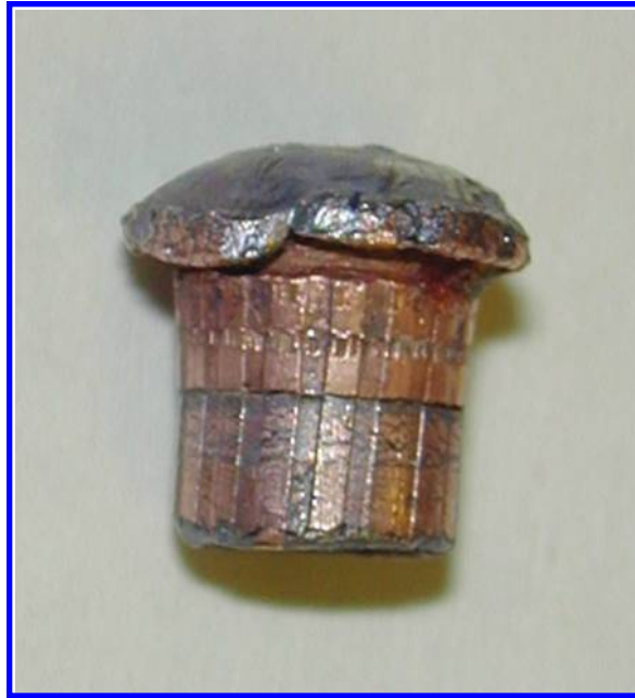
Figure 6.2 .22 Long Rifle bullet with Microgroove rifling.
