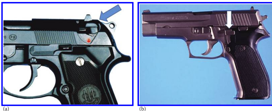
Figure 1.8 (a) Beretta with decocking lever/safety mounted on slide. (b) Sig-Sauer P226 with decocking lever (but no safety) on frame above magazine button.
