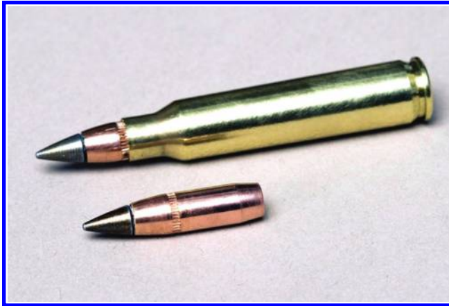
Figure 7.3 M855A1 bullet with exposed steel penetrator tip and copper core. (Photo courtesy of U.S. Army.)
