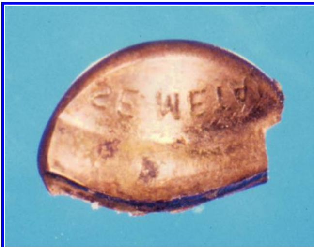
Figure 10.21 Bullet with imprint of lettering from the back of a watch case.
