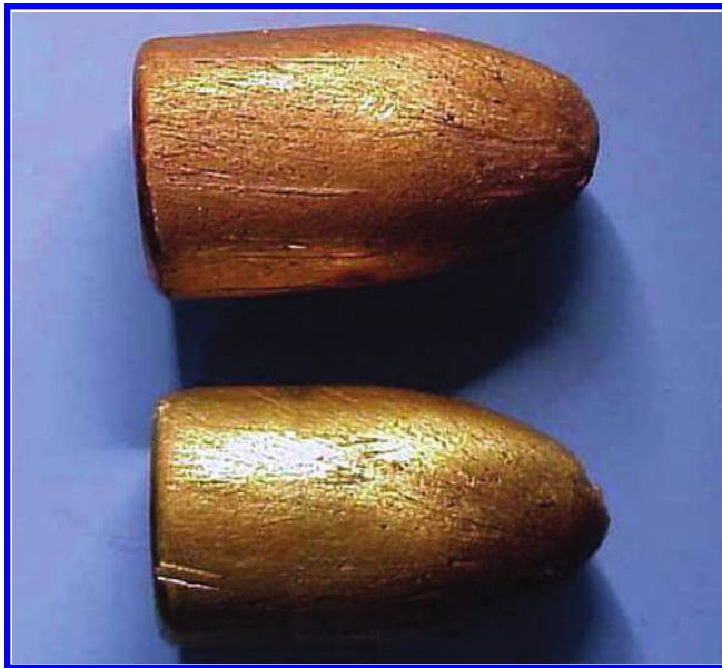
Figure 4.41 Two full-metal-jacketed 9 mm bullets that ricocheted off soft, sandy soil. (Image courtesy of Luke Haag.)
