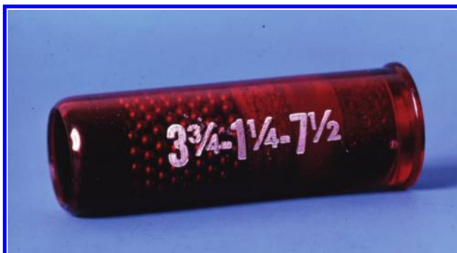
Figure 8.4 Shotgun shell with all-plastic hull.
