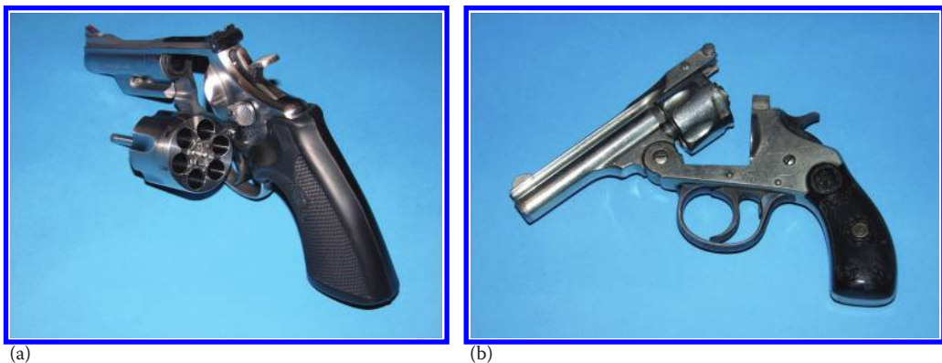
Figure 1.2 (a) A revolver, swing-out type, with cylinder swung open exposing chambers. (b) Break-top revolver with action open. (Photo courtesy of Randall Frost, MD.)
