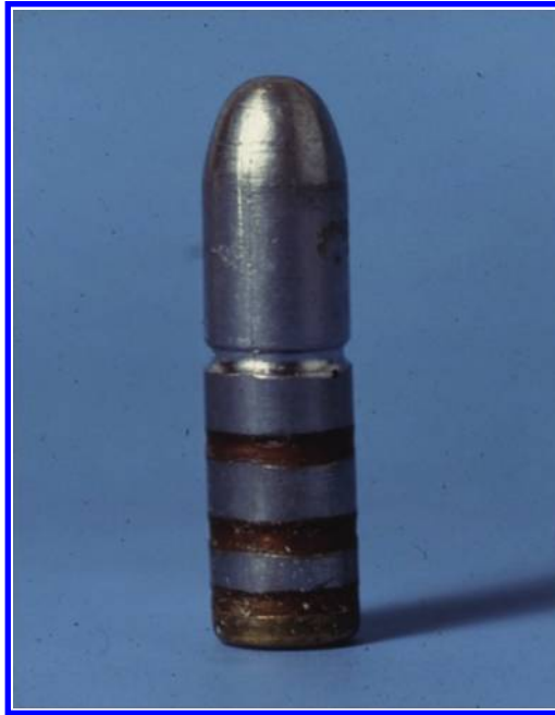
Figure 7.4 Cast rifle bullet with deep cannelures filled with grease.
