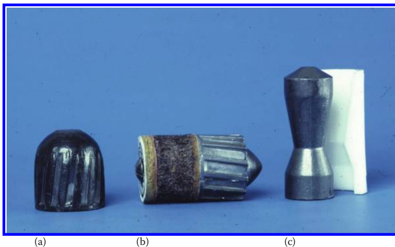
Figure 8.13 Shotgun slugs: (a) Foster, (b) Brenneke, and (c) Smith & Wesson sabot.
