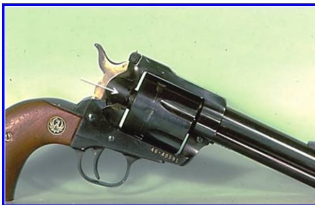
Figure 1.3 Solid-frame revolver with loading gate swung open. Arrow points to loading port where individual cartridges are inserted.
