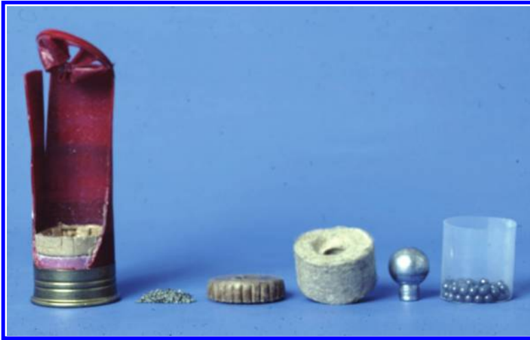
Figure 8.42 Disassembled Winchester tracer round.
