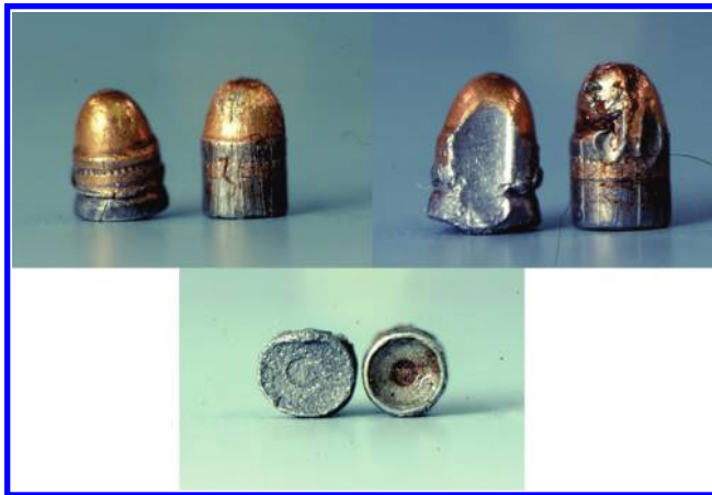
Figure 10.6 The bullet on the left that emerged from the cylinder is shortened, shows the absence of rifling, and has one side sheared off compared to the bullet on the right that emerged from the barrel. The base of the bullet from the cylinder has a granular pockmarked surface resulting from impaction of powder grains.
