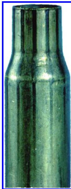
Figure 2.6 Vertical markings on rifle cartridge case due to fluted chamber.
