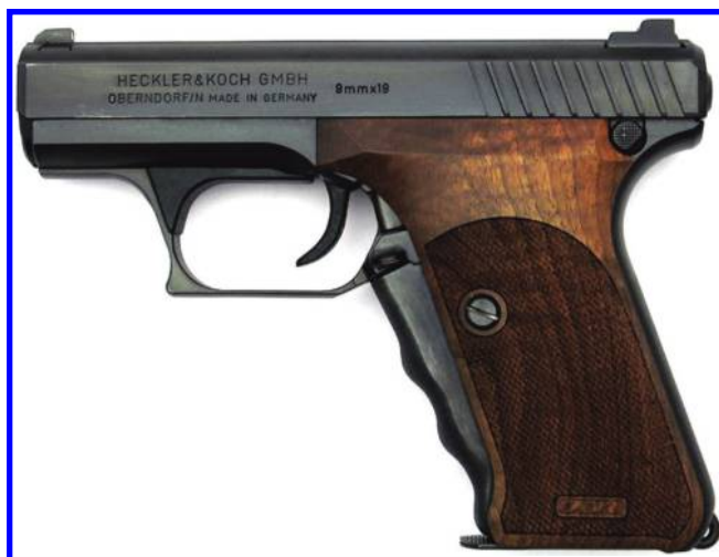
Figure 1.5 Heckler-Koch P7 9 mm pistol with squeeze cocker constituting front portion of grip. (Retrieved from Wikipedia Commons 10/15/2014. Photo released into the public domain by user and author Michael Sullivan, original upload date October 30, 2009.)
