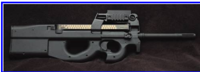
Figure 1.13 Semiautomatic (civilian) version of FN 90 with 16 in. barrel. Note horizontally oriented magazine on top of weapon. (Retrieved from Wikipedia Commons 10/15/2014. Photo made available and published under the Creative Commons Attribution-Share Alike 3.0 Unported license by user and author ROG5728, original upload date November 15, 2011. License can be found here and no changes were made to the image: http://creativecommons.org/licenses/by-sa/3.0/legalcode .)
