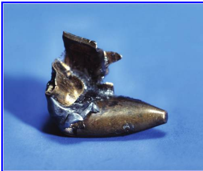
Figure 7.8 M-193 full-metal-jacketed 55 gr. bullet bent at cannelure.
