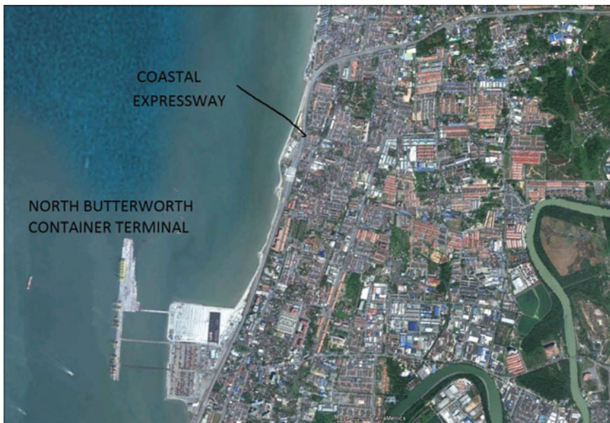
Fig. 5.12 Construction of North Butterworth Container Terminal and Coastal Expressway resulted in impacts on coastal processes along Butterworth coast. Map source Google Earth 2010
