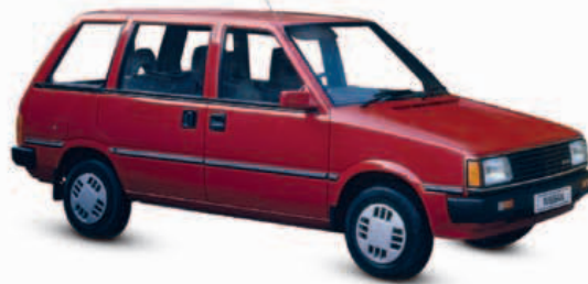
◁ Nissan Prairie 1983 Origin Japan Engine 1,809 cc, straight-four Top speed 99 mph (159 km/h)
