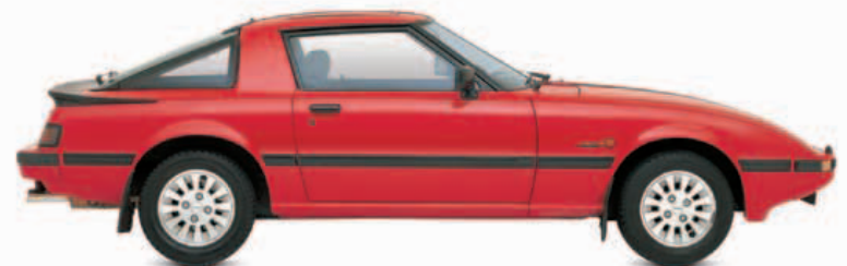
▷ Mazda RX-7 1978 Origin Japan Engine 2,292 cc, two-rotor Wankel Top speed 117 mph (188 km/h)
