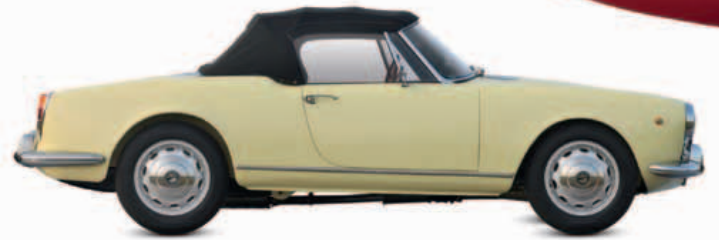
△ Alfa Romeo Giulietta Spider 1955 This beautiful little sports car was built to a very high specification with performance far higher than its 1.3 liters would suggest, thanks to its brilliant twin-cam engine. Origin Italy Engine 1,290 cc, straight-four Top speed 112 mph (180 km/h)
