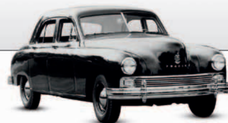
△ Kaiser Frazer F47 1946 Origin USA Engine 3,707 cc, straight-six Top speed 82 mph (132 km/h)
