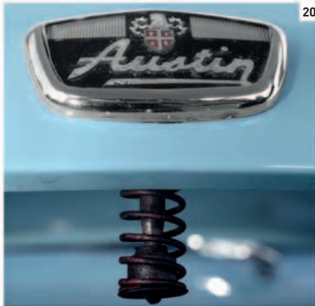
20. Hood-release catch 21. Transverse A-series engine 22. Clutch has hydraulic actuation 23. Battery and spare tire in trunk
