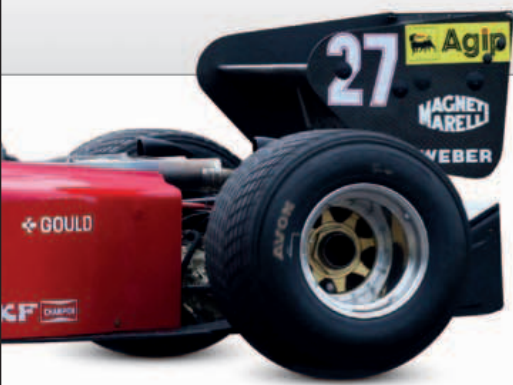
▷ Lotus-Renault 97T 1985 Origin UK Engine 1,492 cc, V6 Top speed 200 mph (322 km/h)
