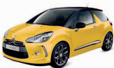
Origin France Engine 1,598 cc, four-cylinder Top speed 133 mph (214 km/h)
