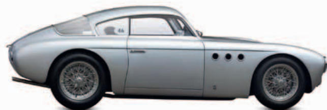
△ Abarth 205 1950 Origin Italy Engine 1,089 cc, straight-four Top speed 108 mph (174 km/h) The first complete car from legendary engine tuner Carlo Abarth, the 205 used a tuned Fiat engine in a body styled by Giovanni Michelotti. It was a successful endurance racer.
