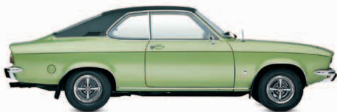
△ Opel Manta GT/E 1970 Origin Germany Engine 1,897 cc, straight-four Top speed 116 mph (187 km/h)
