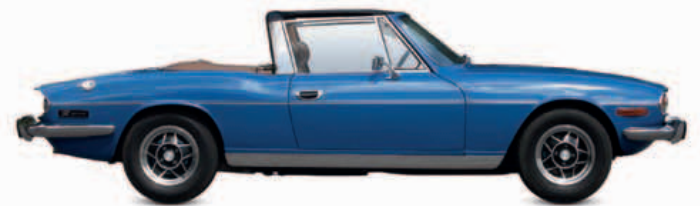
△ Triumph Stag 1970 Origin UK Engine 2,997 cc, V8 Top speed 118 mph (190 km/h)
