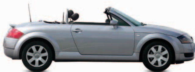
△ Audi TT Roadster 1999 Origin Germany Engine 1,781 cc, straight-four Top speed 138 mph (222 km/h) Built in Hungary with either 4X2 or 4X4, Audi's TT uses Volkswagen Golf technology. It suffered bad press due to high speed instability, prompting recall modifications.
