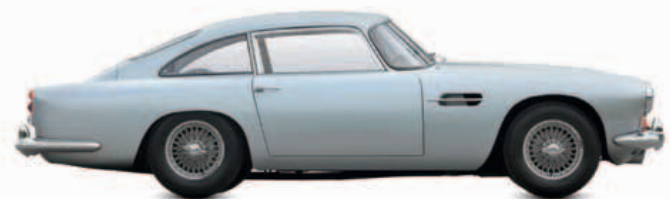
△ Aston Martin DB4 1958 Origin UK Engine 3,670 cc, straight-six Top speed 141 mph (227 km/h) By the end of the decade, the Aston Martin had grown into a true luxury supercar, with exotic Italian styling by Touring and 240 bhp from its new twin-cam engine.
