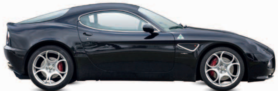
△ Alfa Romeo 8C Competizione 2007 Origin Italy Engine 4,691 cc, V8 Top speed 181 mph (292 km/h) Few believed that the design study exhibited at the 2003 Frankfurt Motor Show would ever make it into production, but Alfa built 500 coupés.
