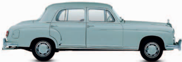
△ Mercedes-Benz 220 1954 Mercedes' first monocoque construction sedan arrived in four-cylinder form in 1953; the more powerful six-cylinder version joined it in 1954. Sturdy and well built, both sold well. Origin Germany Engine 2,195 cc, straight-six Top speed 101 mph (163 km/h)
