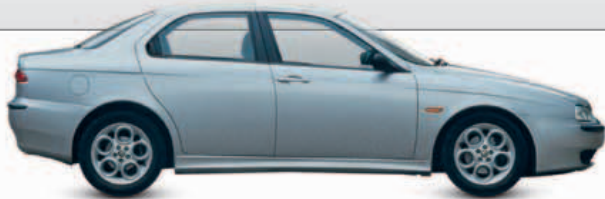
△ Alfa Romeo 156 TS 2.0 1997 Origin Italy Engine 1,970 cc, straight-four Top speed 133 mph (214 km/h) Alfa achieved class-leading styling with this sporting sedan. Features include concealed rear door handles to give it a coupé look.
