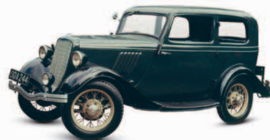
▷ Ford Model Y 1932 Origin UK Engine 933 cc, straight-four Top speed 57 mph (92 km/h)
