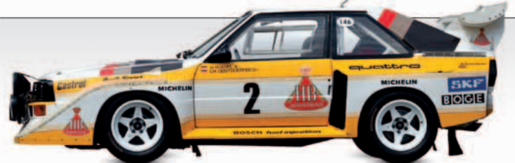
△ Audi Sport quattro S1 E2 1985 Origin Germany Engine 2,133 cc, straight-five Top speed 154 mph (248 km/h)
