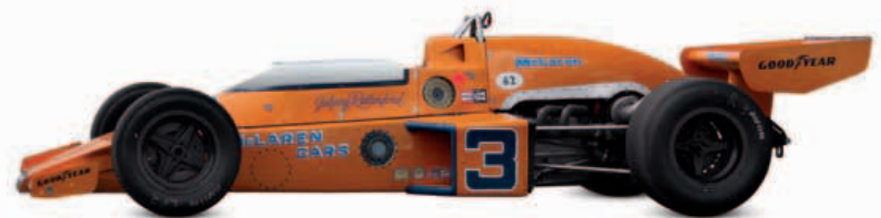
△ McLaren-Offenhauser M16C 1974 Origin UK Engine 2,650 cc, straight-four Top speed 205 mph (330 km/h)
