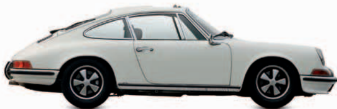
△ Porsche 911S 2.2 1970 Origin Germany Engine 2,195 cc, flat-six Top speed 144 mph (232 km/h) The 911 gained improved handling for the 1970s by moving the rear wheels back by 2.2 in (5.5 cm) and the fuel-injected S took full advantage, becoming a junior supercar.
