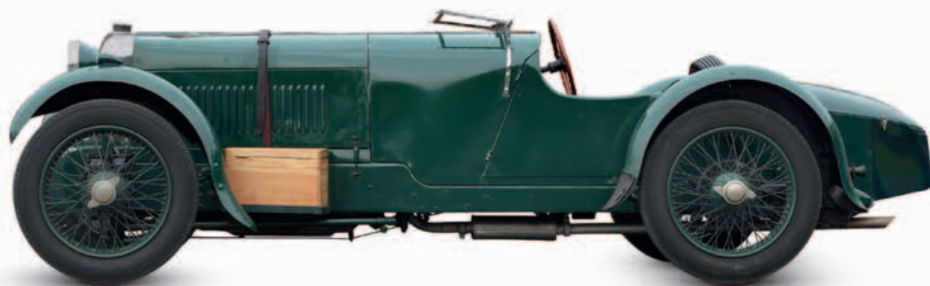
△ Alvis FWD 1928 The first front-wheel-drive, all-independently sprung sports car was too unconventional for its time to sell well. Still, it had great success on the race track. Origin UK Engine 1,482 cc, straight-four Top speed 85 mph (137 km/h)
