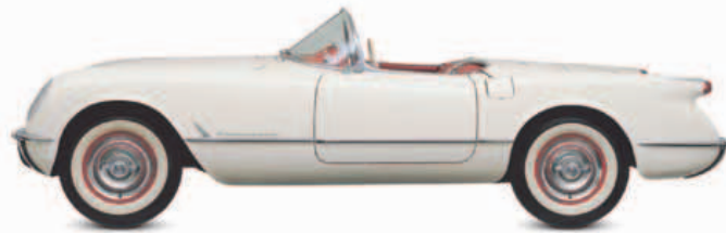
△ Chevrolet Corvette 1953 A Motorama dream car that made it to production, this was the first plastic-bodied car and represented a well-judged leap of faith by Chevrolet. Origin USA Engine 3,859 cc, straight-six Top speed 107 mph (172 km/h)
