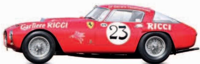
△ Ferrari 375 MM 1953 Origin Italy Engine 4,522 cc, V12 Top speed 150 mph (241 km/h) Built primarily as a competition car, the 375 Mille Miglia won the Spa 24-hour race, Pescara 12-hour race, and Buenos Aires 1,000 km at the start of its glittering racing career.
