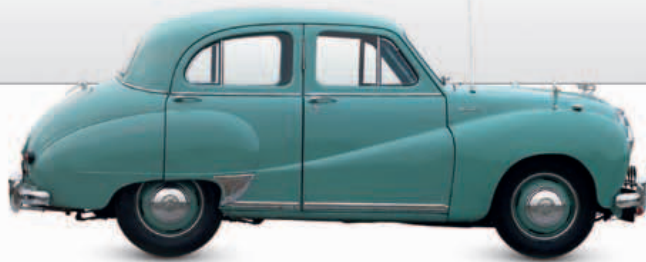
△ Austin A40 Somerset 1952 Comfortable, surprisingly spacious, and agile considering the small engine dimensions, the sturdily built Somerset was a strong seller for Austin: 173,306 in two years. Origin UK Engine 1,200 cc, straight-four Top speed 70 mph (113 km/h)
