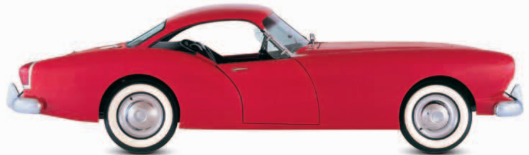
△ Kaiser Darrin 1954 Origin USA Engine 2,641 cc, straight-six Top speed 96 mph (154 km/h) Shipbuilder Henry Kaiser turned to cars after World War II. The fiberglass-bodied Darrin, with doors that slid into the front wings, was the brainchild of designer Howard "Dutch" Darrin.
