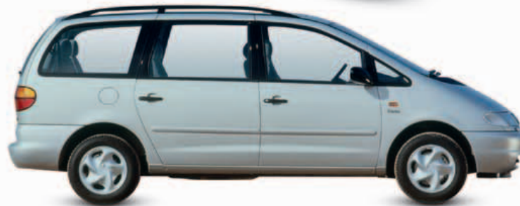
▷ Volkswagen Sharan 1995 Origin Germany/Portugal Engine 1,984 cc, straight-four Top speed 110 mph (177 km/h) Also sold as the SEAT Alhambra and produced alongside the similar Ford Galaxy, Volkswagen's people-carrier didn't have the best reliability record. Engines ranged from 1.8 to 2.8 liters.
