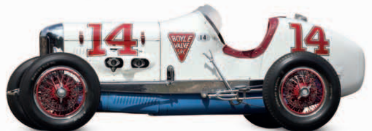
▷ Miller Boyle Valve Special 1930 Origin USA Engine 4,425 cc, straight-four Top speed 140 mph (225 km/h)
