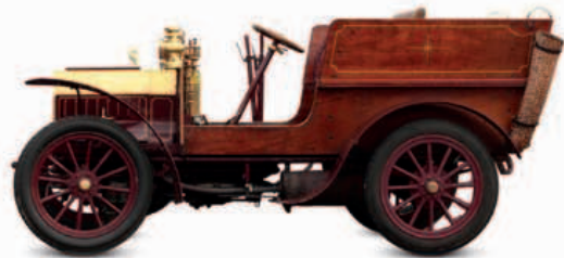
◁ Speedwell 6HP Dogcart 1904 Origin UK Engine 700 cc, single-cylinder Top speed 25 mph (40 km/h)
