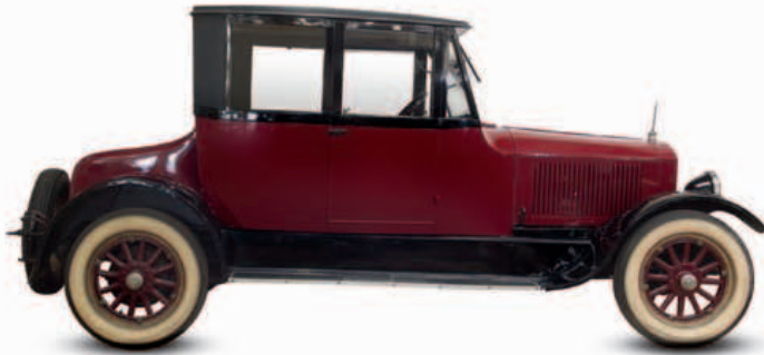
△ Stanley Model 735 1920 Origin USA Engine 2,059 cc, straight-two steam Top speed 60 mph (97 km/h)
