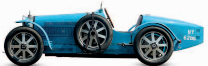
△ Bugatti Type 35B 1927 Origin France Engine 2,262 cc, straight-eight Top speed 127 mph (204 km/h)
