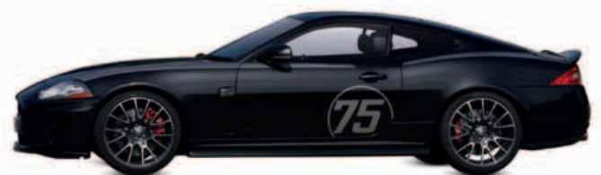
△ Jaguar XKR 75 2010 Origin UK Engine 5,000 cc, V8 Top speed 174 mph (280 km/h) To celebrate the company's 75th anniversary, Jaguar built 75 of these special edition XKRs with improved handling and engines updated to 530 bhp.
