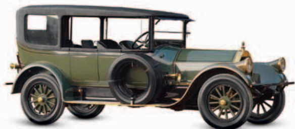
△ Pierce-Arrow 38HP Model 51 1919 Origin USA Engine 8,587 cc, straight-six Top speed 75 mph (121km/h)
