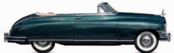
▽ Packard Super Eight convertible 1948 Origin USA Engine 5,359 cc, straight-eight Top speed 98 mph (158 km/h)
