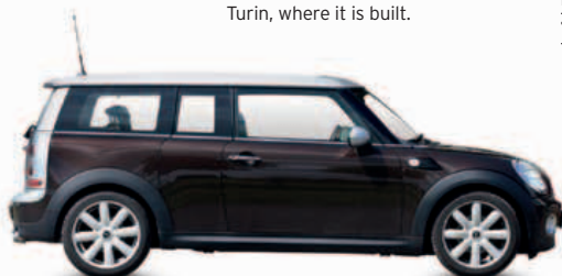
Origin UK Engine 1,598 cc, four-cylinder Top speed 125 mph (201 km/h)
