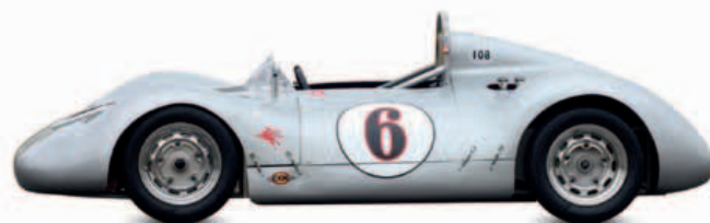
△ Pupulidy-Porsche Special 1954 Origin USA Engine 1,582 cc, flat-four Top speed 130 mph (209 km/h) American racer Emil Pupulidy built a body inspired by Mercedes' Silver Arrows, fitted it to a VW floorpan, and went racing. He won the car's first race at the Nassau Speed Week in the Bahamas.
