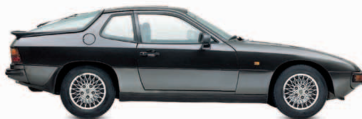
◁ Porsche 924 1976 Origin Germany Engine 1,984 cc, straight-four Top speed 125 mph (201 km/h)
