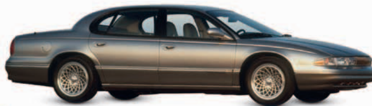
◁ Chrysler New Yorker 1993 Origin USA Engine 3,494 cc, V6 Top speed 134 mph (216 km/h)
