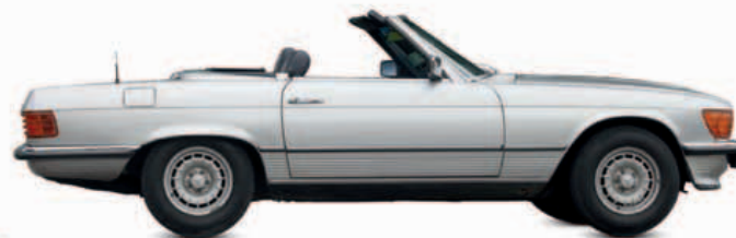
△ Mercedes-Benz 350SL 1971 Origin Germany Engine 3,499 cc, straight-six Top speed 126 mph (203 km/h)
