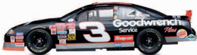
◁ Chevrolet Monte Carlo 2001 Origin USA Engine 5,860 cc, V8 Top speed 190 mph (306 km/h)
