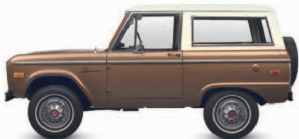
△ Ford Bronco 1966 Origin USA Engine 2,781 cc, straight-six Top speed 76 mph (122 km/h)
