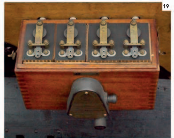
19. Trembler coils for ignition housed in box on dashboard 20. Transmission housing under the floor 21. Hood clip 22. Hood handle 23. Four-cylinder engine has a capacity of nearly 3 liters
