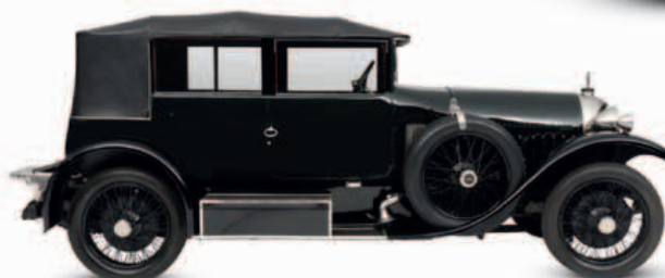
▷ Lincoln L Sedan 1922 Origin USA Engine 6,306 cc, V8 Top speed 82 mph (132 km/h)
