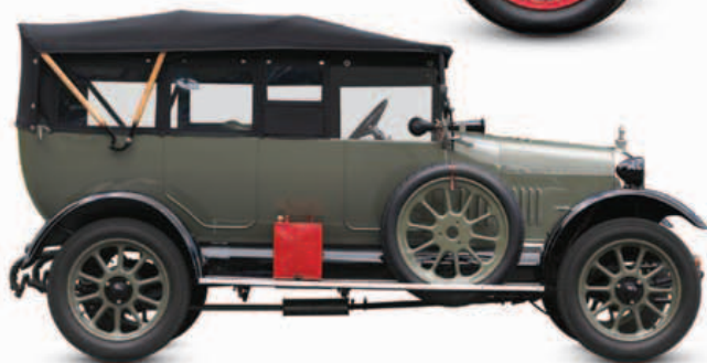
△ Morris Oxford 1919 Origin UK Engine 1,548 cc, straight-four Top speed 60 mph (97 km/h)
