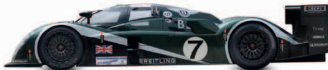
△ Bentley Speed 8 2001 Returning to Le Mans 73 years after its glory days in the 1920s, it took Bentley three attempts before winning once again in 2003. Origin UK Engine 4,000 cc, V8 Top speed 205 mph (330 km/h)
