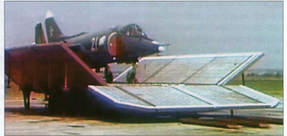
Top and top right: Yak-38 '21 Yellow' (c/n 797786...502409, f/n 0803) was used for experiments with a mobile launch pad based on a trailer. Here the trailer with the aircraft on top is towed by a KRAZ-255B 6x6 heavy-duty lorry.
