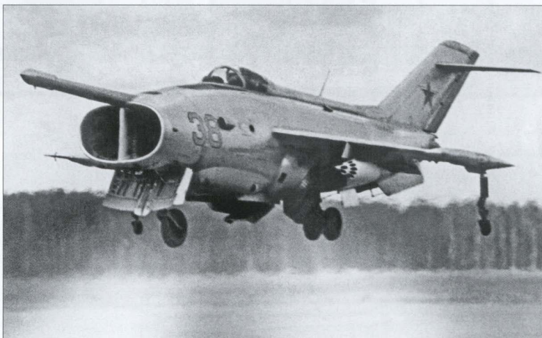
Above and below: Yak-36 '38 Yellow' takes off vertically at the Domodedovo airshow, belching smoke. Note the absence of the blow-in doors which were eliminated when the main intake was enlarged.
