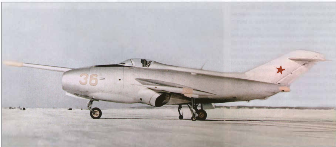
A rare colour photo of Yak-36 '36 Yellow'; note that the areas where the reaction control nozzles are located were painted yellow, making the nose boom look like a monstrous sulphur-tipped matchstick. The quality of the Soviet colour film, which was poor to begin with, has deteriorated after all these years.
