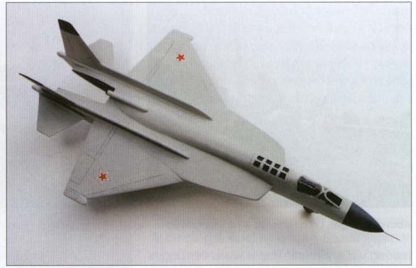
Three views of a desktop model depicting the early version of the Yak-41M with the larger LERXes, redesigned air intakes, strongly tapered wings and stabilizers, and splayed vertical tails.
