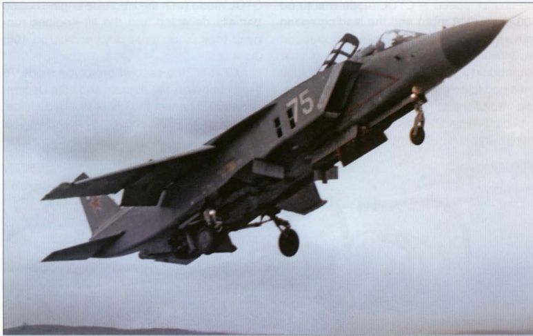
Top and above: Yak-41 '75 White' takes off vertically from SNS Baku during carrier compatibility trials.
