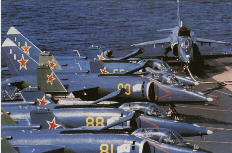
The Yak-38s based aboard SNS Novorossiysk had high tactical codes. It was standard operational procedure to keep the lift engine air intakes open when parked – in case of a scramble.
