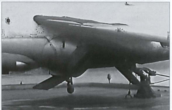
Here, '36 Yellow' becomes airborne and tugs at the tethers during early ground tests. Note the twin auxiliary intake doors on the sides of the nose. The aircraft is parked over a special exhaust gas evacuation device – a specially shaped pit closed by a steel grille.
