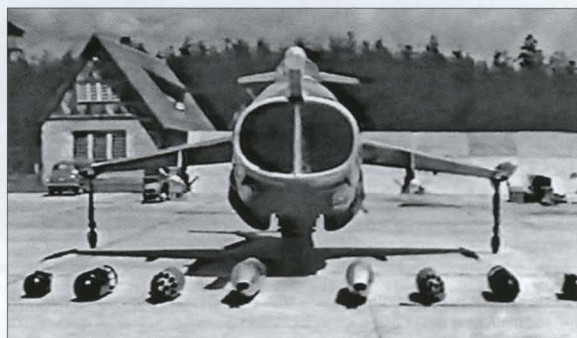
Above, left and below: The second prototype is seen here parked at the Yakovlev OKB's flight test facility in Zhukovskiy with R-3S missiles on the wing pylons and a weapons array in front (UPK-23-250 cannon pods, UB-16-57UM FFAR pods, FAB-100 and FAB-250 bombs) for the benefit of an MoD delegation. Note the quaint-looking cottage in the background with a jet blast deflector wall beside it. The engine nozzles are in vertical thrust position.
