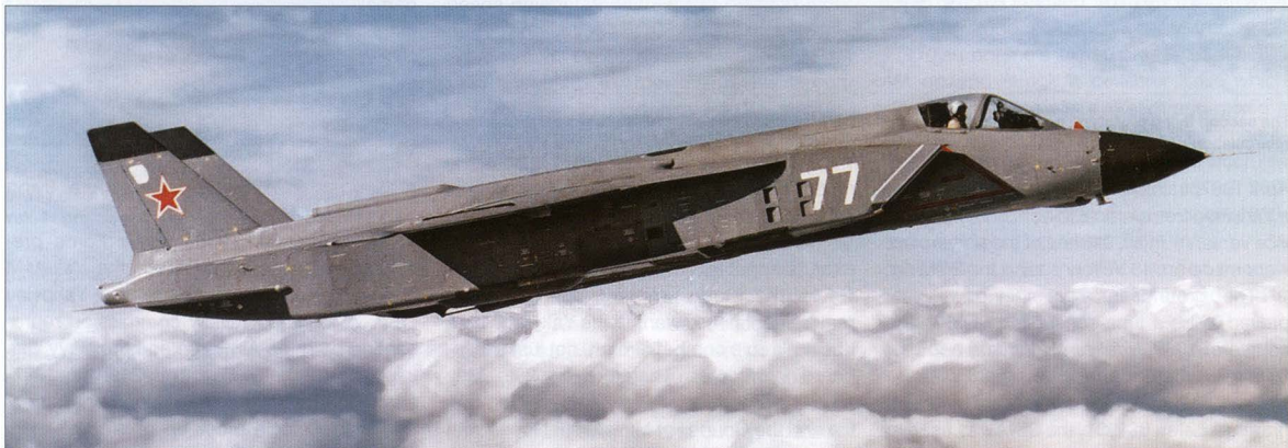
These air-to-air shots of the second prototype show the undernose fairing of the forward reaction control puffer which replaced the rear puffers (one of the latter is replaced by an FDR in a crashworthy housing). Note also the main engine nozzle door actuator and the black heat-insulating compound on the belly.
