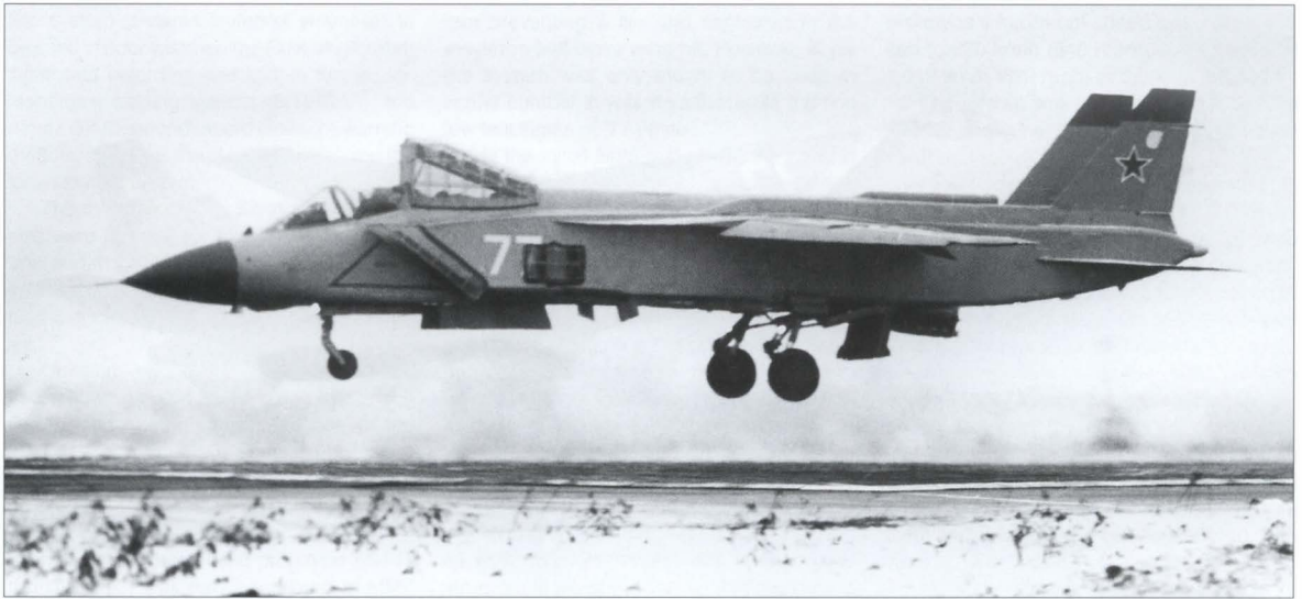
The second flying prototype performs a hover; again, FOD protection screens are fitted. Note the open main engine nozzle door and the deployed transverse recirculation dams.
