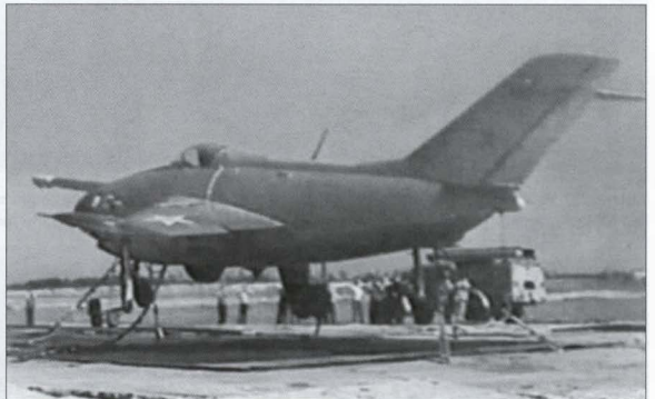
Top and above: Yak-36 '36 Yellow' suspended from the 'cable crane'. The latter was quite a large installation, as this view shows!
