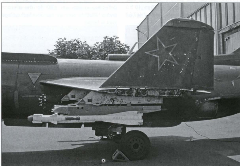
The port wing of a Yak-38M, showing the wing folding hinge, the twin weapons pylons and the wingtip bulges housing reaction control puffers.
