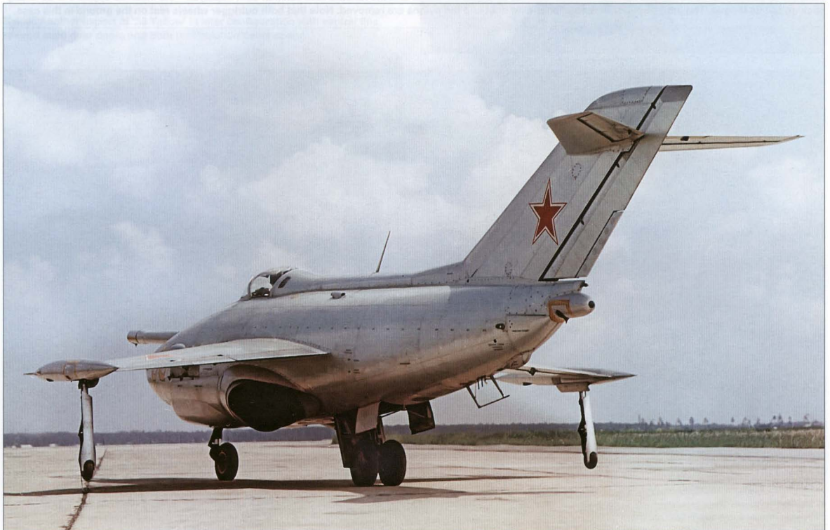
Excellent colour views of the second flying prototype prior to modification. The reaction control puffers are marked by yellow boxes and the data link aerial under the tail is well visible. Note how the machine sits 'on an even keel', neither of the outrigger wheels touching the ground.
