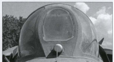
Top: The dielectric nosecone and pitot probe. Above, right and top right: The cockpit canopy of the single-seat Yak-38.
