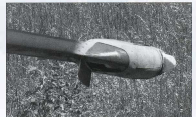
Above: Close-up of the port wingtip fairing incorporating the reaction control nozzle and ECM antennas.
