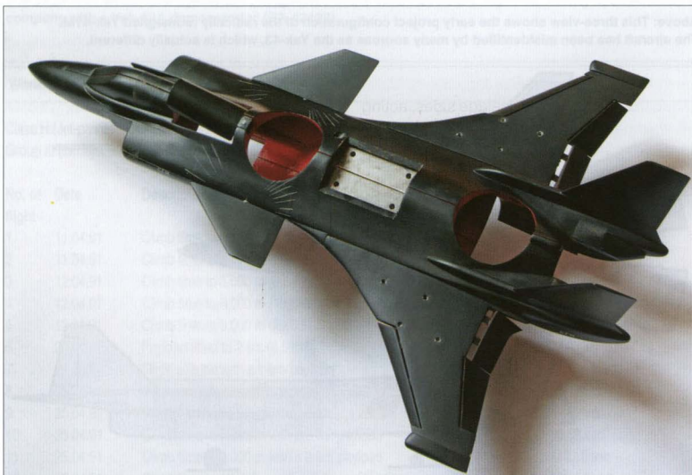
A wind tunnel model of a projected advanced VTOL aircraft utilising the canard layout. Once again, the aircraft has a mixed powerplant with two lift engines and a single lift/cruise engine
