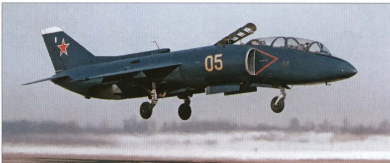
The Yak-36MU prototype makes its first vertical take-off. The trainer had an oddly banana-shaped fuselage.
