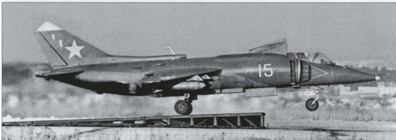
Here, '15 Yellow' makes a short rolling take-off from a mobile ski jump developed for ad hoc tactical airstrips.
