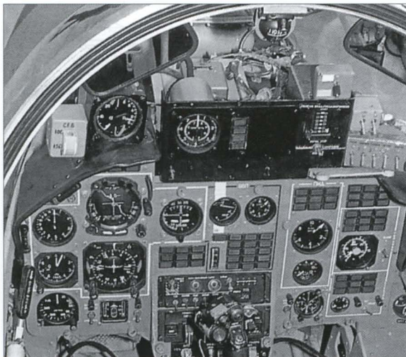
Above: The cockpit of this Yak-41 shows a very different instrument panel and lacks the HUD. Note the rearview mirrors.
