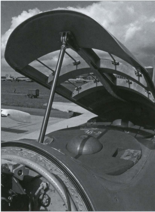
Above: The lift engine air intake door of the first prototype. The spring-loaded suction relief doors have been removed and the engine inlets are closed by blanks. Right and top right: The nozzle of the R79V-300 lift/cruise engine. The fairings above it accommodate the brake parachute (on the centerline) and the FDR. Far right: The 'snap-action' nozzle door of the main engine in the open position.
