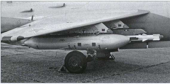
Above: A UPK-23-250 cannon pod and an R-60M air-to-air missile under the wing of Yak-38M '88 Yellow' at Khodynka. Right: A UB-16-57UMP-73 FFAR pod and a dummy R-60 AAM on an APU-60-1 launch rail under the wing of Yak-36M f/n 0201.
