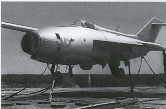
Here, '36 Yellow' becomes airborne and tugs at the tethers during early ground tests. Note the twin auxiliary intake doors on the sides of the nose. The aircraft is parked over a special exhaust gas evacuation device – a specially shaped pit closed by a steel grille.
