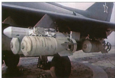
Above: Three FAB-100M54 bombs on an MBD3-U4 multiple ejector rack. Above right: A napalm tank is ready for hooking up. Far right, above and below: The VM-4 is seen with a large weapons array at a new hardware display for high-ranking military officials.
