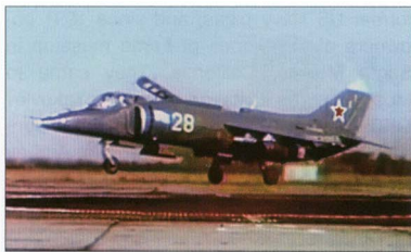
Yak-38 '28 Yellow' was used for tests involving VTOL operations on a small metal landing pad at Saki.
