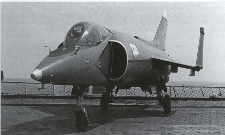
Yak-36M1/n 0201 on the deck of SNS Kiev with the wings folded (note the AK-90F tiles on the deck). The wingtip fairings house puffers. The aircraft still has the narrow-track main gear and old air intake design.
