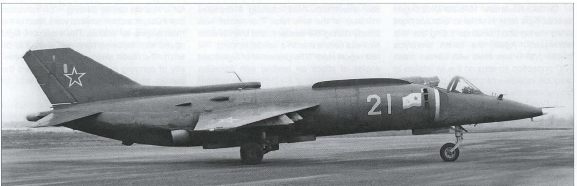
These pictures probably depict the same aircraft in modified form, with dorsal recirculation dams and an Opushka-VM crash data recorder on the tailcone.
