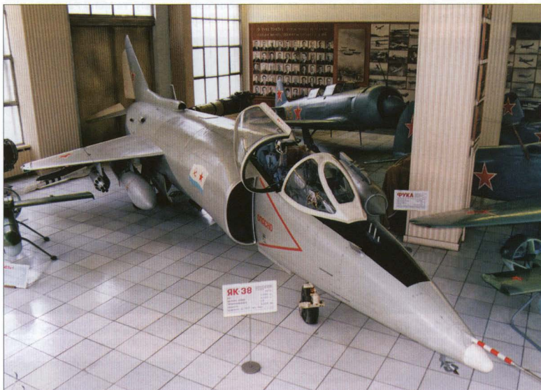
Above: Yak-36M f/n 0201 was preserved in grey colours at the Yakovlev OKB museum in Moscow. This machine retained the old air intake design and narrow-track landing gear.
