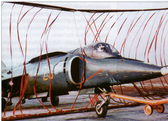
This production Yak-38 coded '23 Yellow' (possibly f/n 0703) was used for testing the crash barrier developed for Kiev class aircraft carriers. Note the dark green undersurfaces characteristic of production examples.
