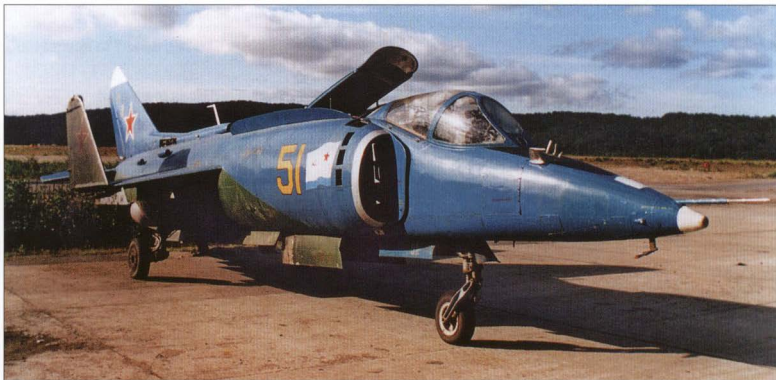
Yak-38 '51 Yellow' looks rather forlorn, with missing panels and the undernose antenna askew.
