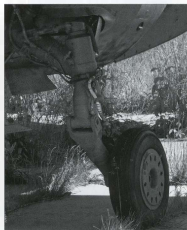
Left: The early-model narrow-track main landing gear with straight struts.
