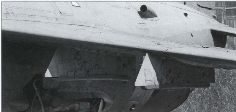
Above: Close-up of the port wingtip fairing incorporating the reaction control nozzle and ECM antennas.
