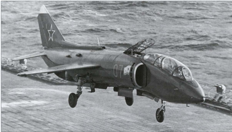
'07 Yellow', another in-service Yak-38U, shows the wide-track landing gear and the raked fin tip of the production version.
