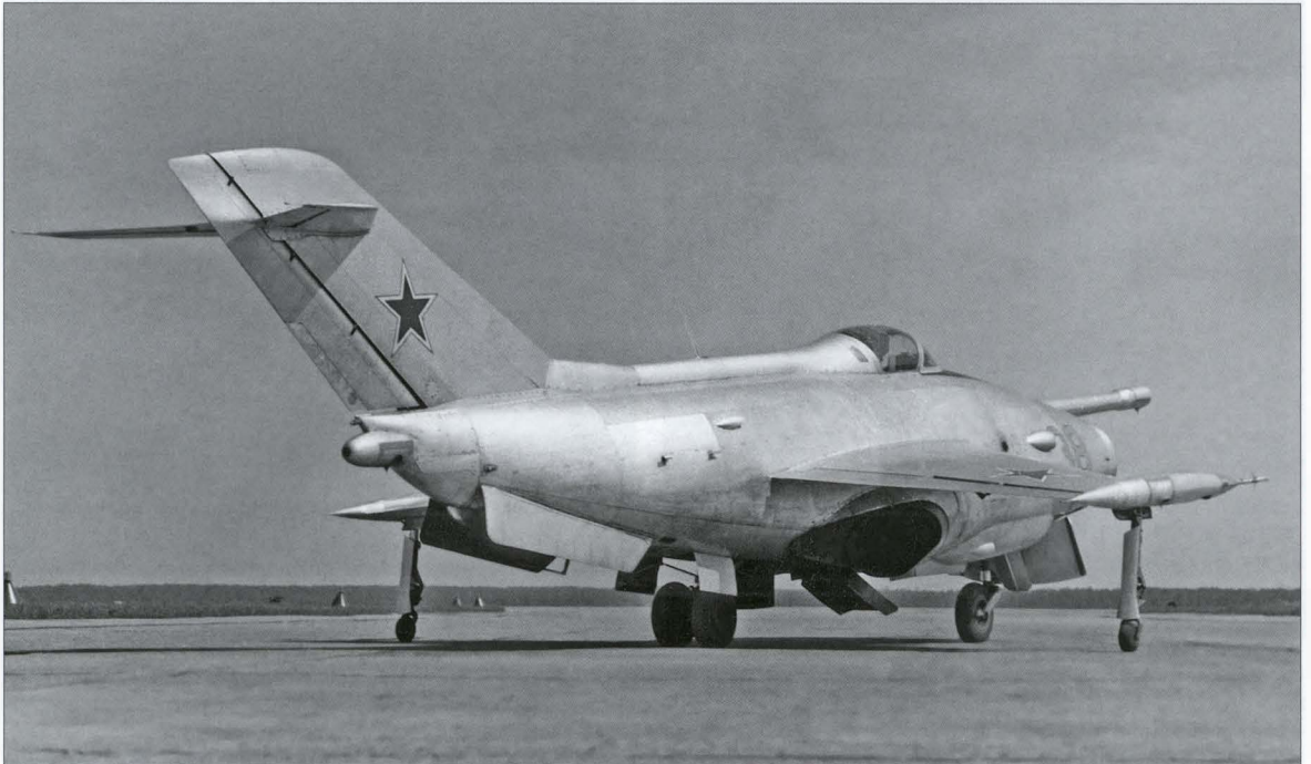
Below: Another aspect of '38 Yellow' in later configuration with ventral fins, revised main gear doors and both recirculation dams open.
