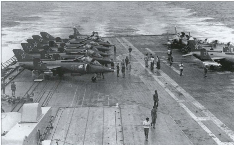
Above: The rear deck of SNS Minsk , with eight Yak-38s visible; two of them are armed with Kh-23 missiles. The stern deck lift is in the foreground.
