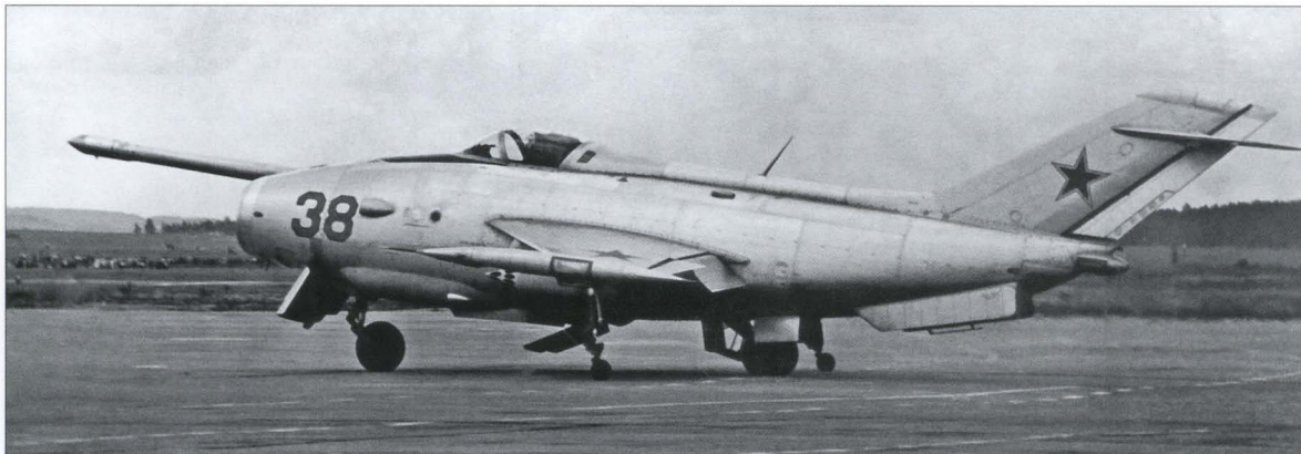
Above: Here, the second flying prototype is armed with two UB-16-57UM rocket pods. The Yak-36 had a strong nose-up ground angle.
