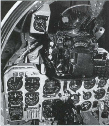
Above: The instrument panel of a typical Yak-38 dominated by an ASP-PFD-21 sight.
