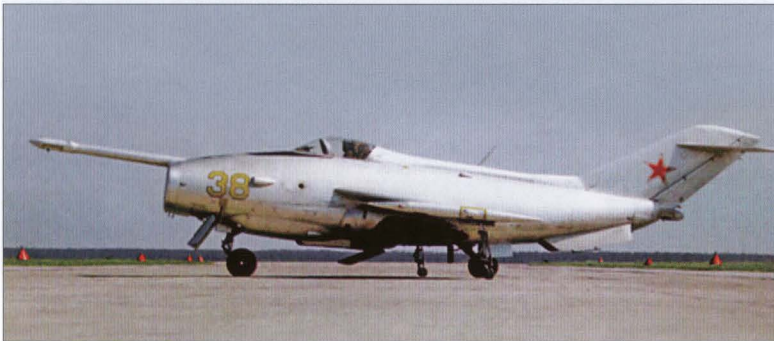
Above and left: Further aspects of the second prototype. Note the longitudinal strakes under the centre fuselage flanking the rear recirculation dam.
