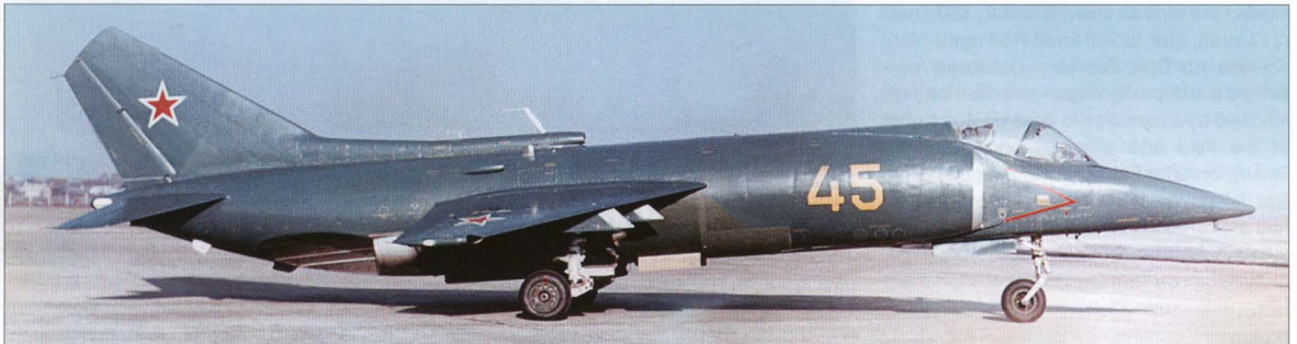
Top and above: Two more shots of the fourth prototype, showing the definitive nose and tail shape, the revised air intakes (with boundary layer splitter plates and auxiliary blow-in doors), the new wide-track main gear units and the characteristic nose-up ground angle. The forward door of the nose gear unit is missing.
