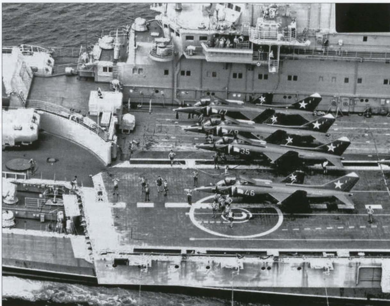
Four Yak-38s sit side by side at the front end of the Minsk's flight deck. The launch pad marked 'C' (a Cyrillic 'S') is for a search-and-rescue helicopter.
