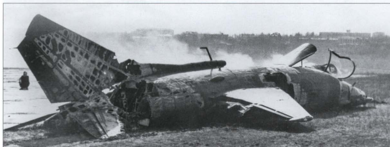
On 4th April 1975 Mikhail S. Deksbakh suffered a landing accident in Yak-36M f/n 0302 at Saratov-Yoosnyy. The extent of the fire damage to the aircraft is clearly visible; the machine was a total loss.
