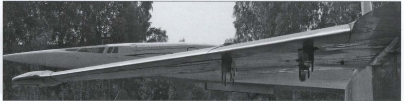
Above: The starboard wing, showing the leading-edge flap, the LERX and the two weapons pylons.
