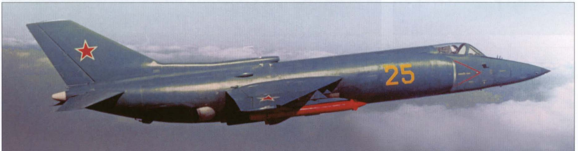
The VM-2 is shown here with the later pointed nosecone (instead of a rounded dielectric cap) and two dummy Kh-23s. Note the overall blue finish.
