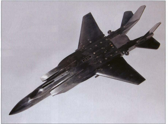
Top and top left: '47 Yellow' represents the configuration of the Yak-41 that was eventually finalised, using a conventional (non-BWB) design with raked two-dimensional air intakes and an axisymmetrical vectoring nozzle between two tailbooms. Note the brake parachute container above the engine nozzle.
