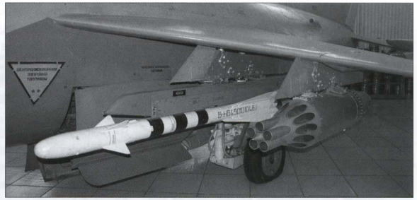
Above: A UPK-23-250 cannon pod and an R-60M air-to-air missile under the wing of Yak-38M '88 Yellow' at Khodynka. Right: A UB-16-57UMP-73 FFAR pod and a dummy R-60 AAM on an APU-60-1 launch rail under the wing of Yak-36M f/n 0201.
