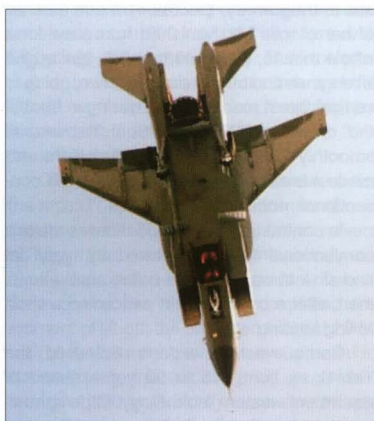
These shots of the Yak-41 from below taken at Farnborough show the glowing combustion chambers of the lift engines as the machine hovers and then transitions to forward flight.
