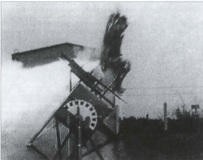
The crew rescue system test rig built under the programme is shown just as a Yakovlev KYa-1 ejection seat with a dummy is catapulted from it. The rig could be tilted to emulate various attitudes of the aircraft.
