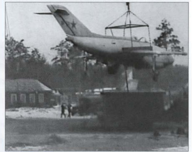
Top and above: Yak-36 '36 Yellow' suspended from the 'cable crane'. The latter was quite a large installation, as this view shows!
