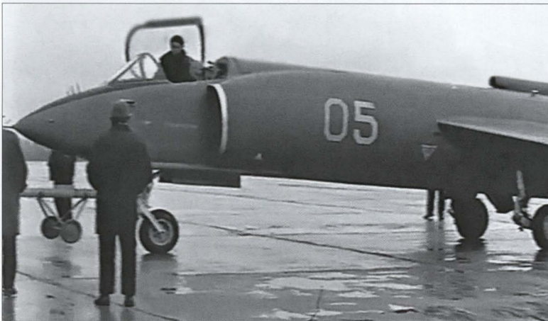
Top, right, and top right: '05 Yellow', the first prototype Yak-36M (the VM-1), on the 'cable crane' at Zhukovskiy. It, too, represented the short-nosed/square-tailed EVM configuration. Note the 'Danger, air intake' warning triangles, the tethering cables and the sensor cable leading to remote data recorders. Above: The VM-1 is towed at Zhukovskiy. Note the plain air intakes without splitter plates or blow-in doors. Above right: The first prototype undergoing tests on the SSM dynamometric rig.
