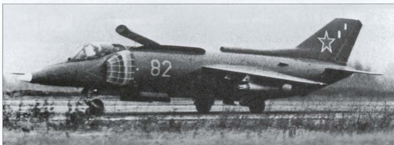
Top: '82 Yellow', the first prototype Yak-38M (izdeliye 82-1). Centre and above: '82 Yellow' undergoes trials with FOD protection screens.
