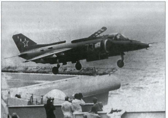
These pictures show Yak-38s '73 Yellow' and '74 Yellow' (c/ns 797786...286815 and 797786...286840) making short take-offs from SNS Novorossiysk during special tests (note the cameramen in the photo on the right). The aircraft have the late-model dorsal and ventral recirculation dams.
