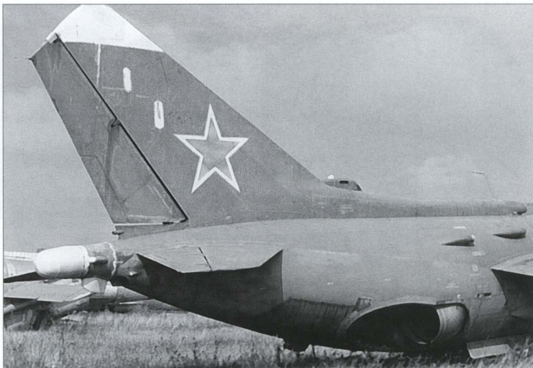
The rear fuselage and tail unit of a late Yak-38 sans suffixe with an Opushka-VM FDR on the tailcone.
