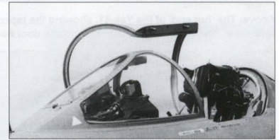
Above: The cockpit of a partially completed Yak-41 prototype, showing the ejection seat, instrument panel and HUD.
