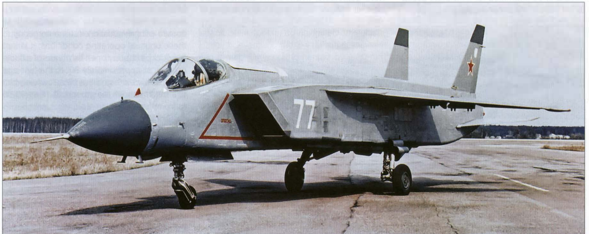
Centre: The second flying prototype, '77 White' (izdeliye 48-3), poses with dummy R-73 and R-27R AAMs; this is the only available photo of it with weapons. Above: The same machine minus missile launch rails. '77 White' also had a small nosewheel.
