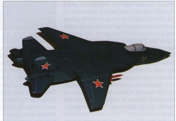
Above: A later version of 'Shekhter's Monster' with an air intake centrebody and main gear units retracting aft into wing fairings. Right: An early three-engined model with a 2-D vectoring nozzle and lift engines placed ahead of the cockpit. The tactical code may hint at the year of development.
