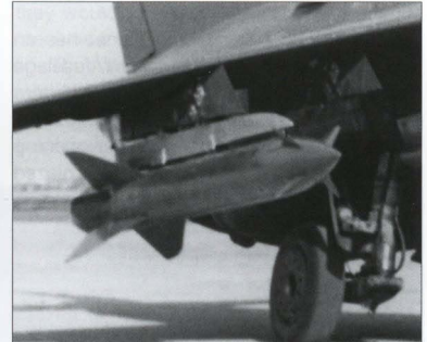
Above: A UPK-23-250 cannon pod and an R-60M air-to-air missile under the wing of Yak-38M '88 Yellow' at Khodynka. Right: A UB-16-57UMP-73 FFAR pod and a dummy R-60 AAM on an APU-60-1 launch rail under the wing of Yak-36M f/n 0201.
