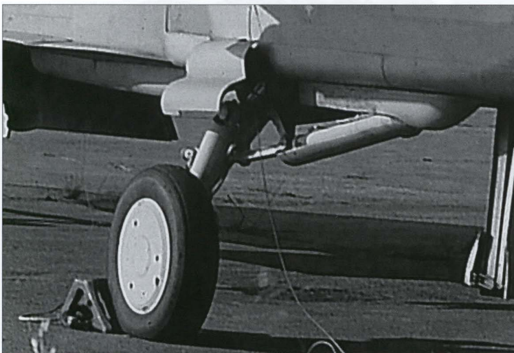
Above: The port main gear unit with its externally located retraction ram. Right: The nose gear unit features a remarkably small wheel.
