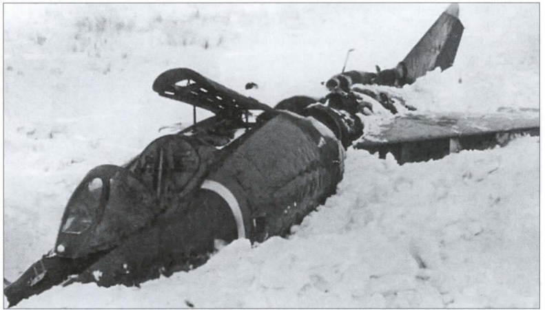
Above: Another accident in Saratov on 4th March 1976 when Yak-36M c/n 7977861609443 (f/n 0903) kicked the pilot out of its own accord.
