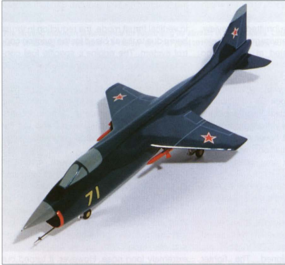
These models show how the two concepts of the Yak-41 evolved. Above: This tadpole-like single-engined aircraft was proposed by Leon M. Shekhter's team. Right: This three-engined model is very close to the real Yak-41, except for the lateral doors covering the main engine's vectoring nozzle.
