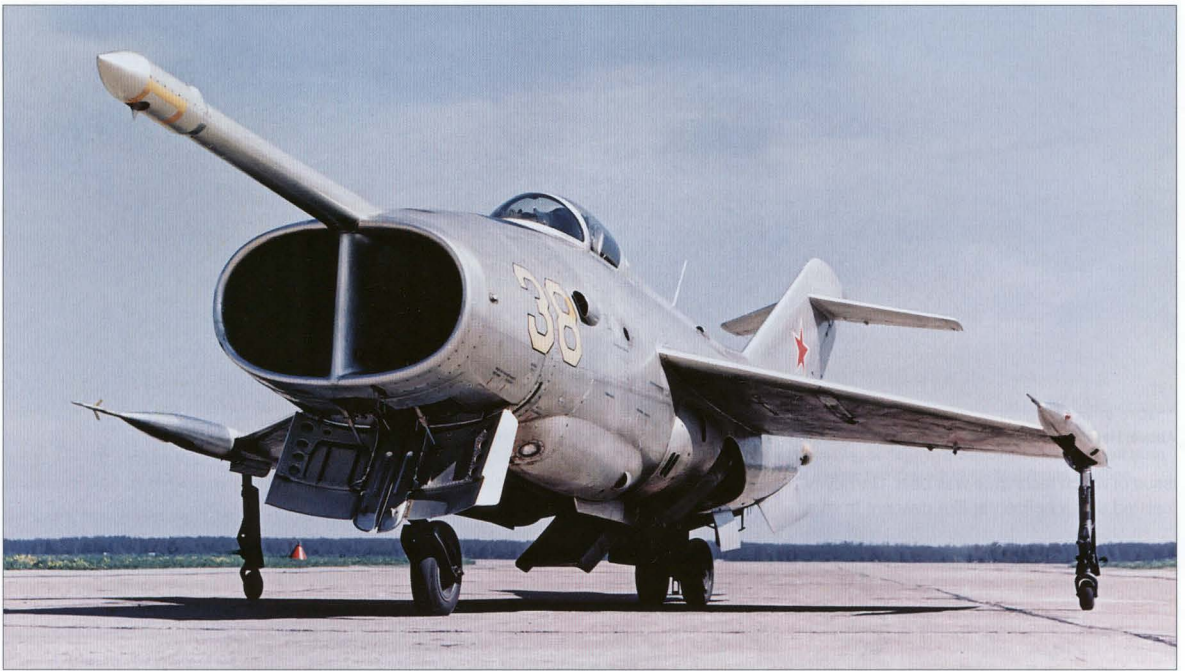
Above and left: Further aspects of the second prototype. Note the longitudinal strakes under the centre fuselage flanking the rear recirculation dam.
