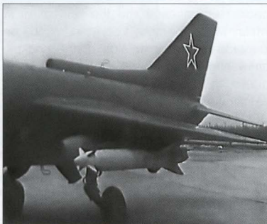
Close-up of the Kh-23 missile and the UPK-23-250 cannon pod under the mock-up's port wing.
