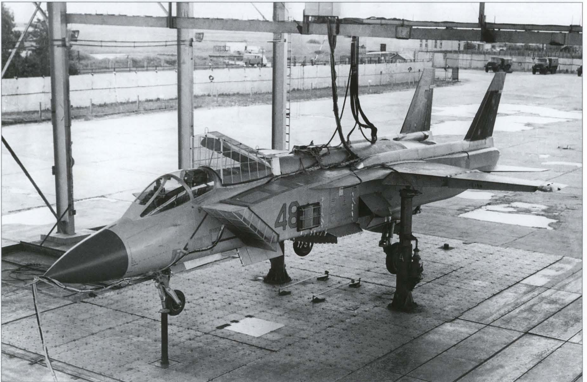
Two more views of the izdeliye 48-1 on the dynamometric rig. The underlying surface is protected by AK-90F ceramic tiles. Interestingly, the nosewheel and the lift engine air intake scoop were removed in the course of the tests. Note that the SSM rig is located in a shed protecting it from US surveillance satellites.
