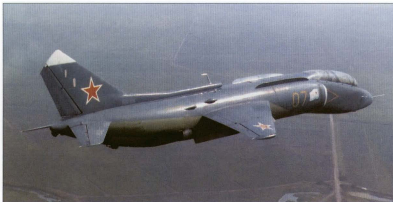
Above: This Yak-38U coded '07 Yellow' was operated by LII and used for test and development work. Note the non-standard nose pitot.
