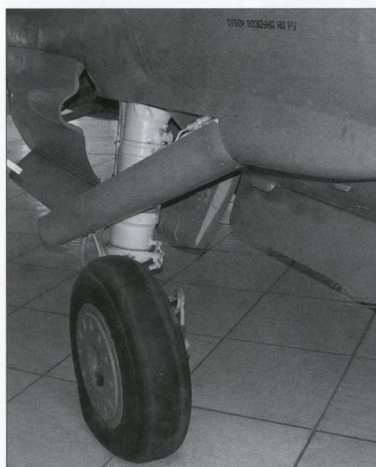
Left: The early-model narrow-track main landing gear with straight struts.
