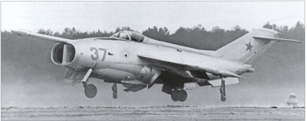
Above: '37 Yellow' lifts off vertically at Domodedovo with the recirculation dams deployed.
