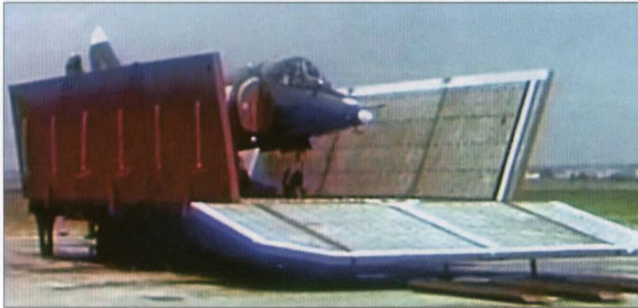
Top and top right: Yak-38 '21 Yellow' (c/n 797786...502409, f/n 0803) was used for experiments with a mobile launch pad based on a trailer. Here the trailer with the aircraft on top is towed by a KRAZ-255B 6x6 heavy-duty lorry.
