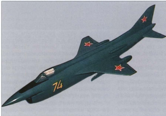
Above: A later version of 'Shekhter's Monster' with an air intake centrebody and main gear units retracting aft into wing fairings. Right: An early three-engined model with a 2-D vectoring nozzle and lift engines placed ahead of the cockpit. The tactical code may hint at the year of development.
