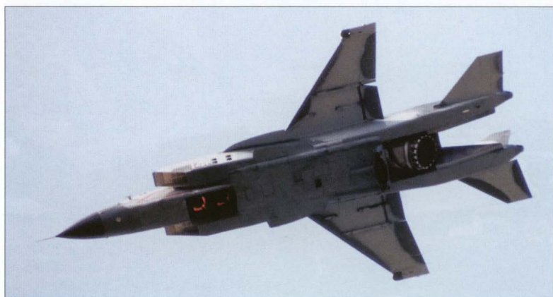
These shots of the Yak-41 from below taken at Farnborough show the glowing combustion chambers of the lift engines as the machine hovers and then transitions to forward flight.
