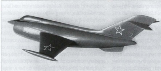
The Yakovlev OKB attempted to turn the Yak-36 into a true combat aircraft. In so doing the forward fuselage was considerably lengthened and the cockpit was moved forward to improve the field of view. The resulting project version illustrated by a model and a three-view drawing was designated Yak-36-70.
