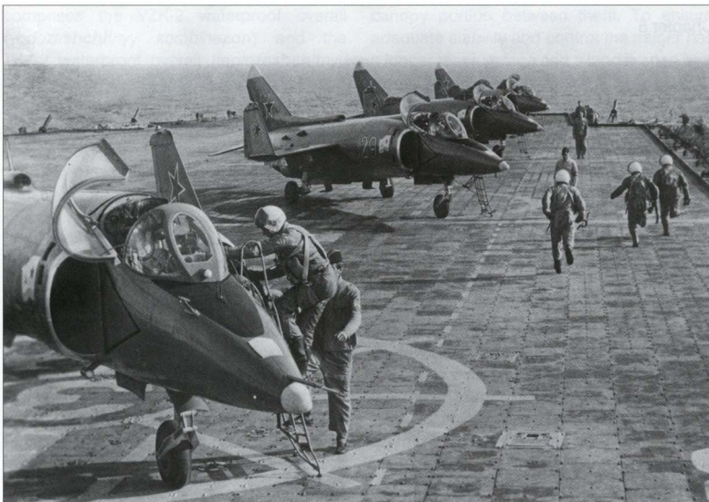
Above: The 'flight line' on the deck of the Kíev , with four Yak-38s on the launch pads marked by circles. A practice scramble is depicted here.
