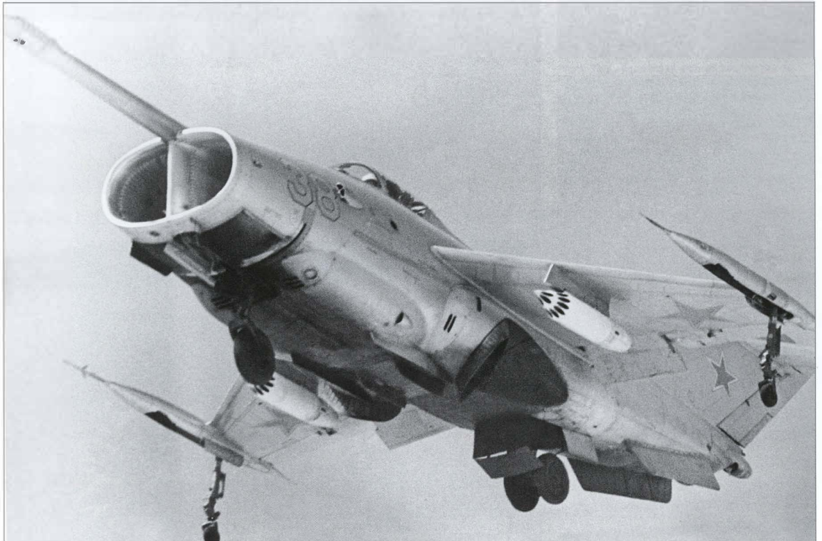
This view shows details of the second flying prototype's underside; note the fixed strakes flanking the rear recirculation dam, which has its own strakes.
