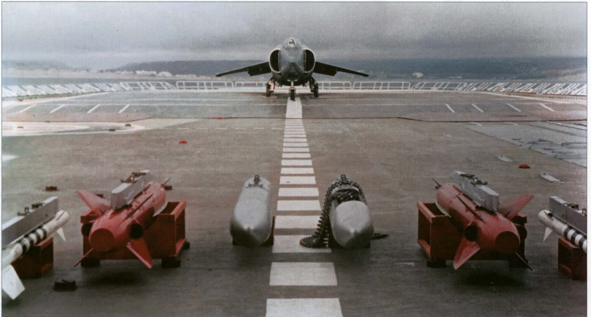
The VM-2 is parked on the deck of SNS Moskva , with weapons arrayed in front for the Navy top brass (R-3S AAMs, Kh-23 ASMs – dummies in both cases – and UPK-23-250 cannon pods. The aircraft sits on a special steel platform protecting the deck from the jet exhaust (note the solid lines instead of hatched ones).
