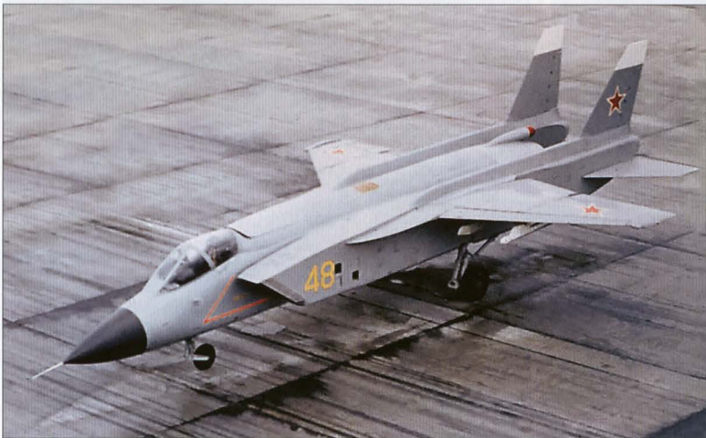
Top, centre and above: '48 Yellow', the izdeliye 48-1, after rollout. Despite being non-flyable, it wore full insignia. Note the lack of the rear reaction control puffers and the large nosewheel.
