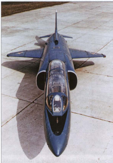
Top: '05 Yellow', the Yak-36MU trainer prototype (VMU-1). Note the horizontally cropped fin. Left and above: Sharks' R'Us. The VMU-1 looks rather strange from these angles. Note the forward reaction control puffer and the narrow wheel track.
