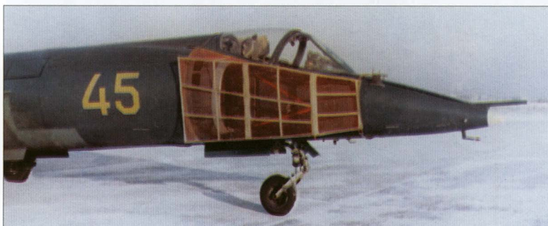
Among other things, the VM-4 served for rough-field tests. The air intakes were fitted with large FOD screens; the open auxiliary blow-in doors are visible. Note the new white dielectric nosecone.
