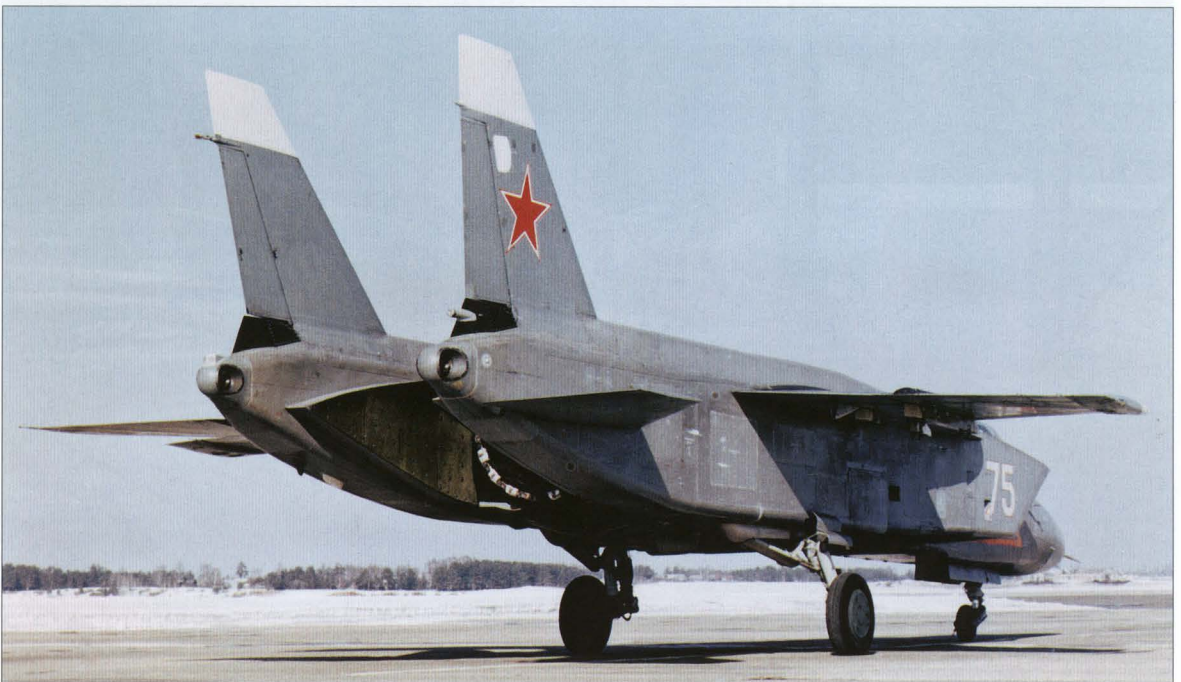
Three aspects of '75 White', the first flying prototype ( izdeliye 48-2). Note the reaction control puffers at the tips of the tailbooms and the small nosewheel.
