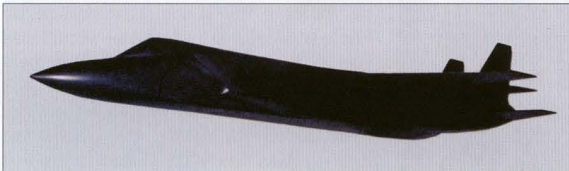
Centre and above: A wind tunnel model of the Yak-41 in the final configuration. The fixtures allow it to be placed in the tunnel with different angles of attack.
