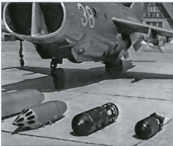
Above, left and below: The second prototype is seen here parked at the Yakovlev OKB's flight test facility in Zhukovskiy with R-3S missiles on the wing pylons and a weapons array in front (UPK-23-250 cannon pods, UB-16-57UM FFAR pods, FAB-100 and FAB-250 bombs) for the benefit of an MoD delegation. Note the quaint-looking cottage in the background with a jet blast deflector wall beside it. The engine nozzles are in vertical thrust position.
