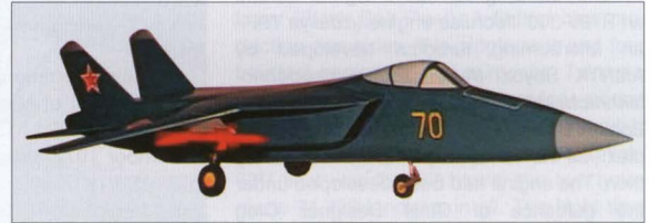
These models show how the two concepts of the Yak-41 evolved. Above: This tadpole-like single-engined aircraft was proposed by Leon M. Shekhter's team. Right: This three-engined model is very close to the real Yak-41, except for the lateral doors covering the main engine's vectoring nozzle.
