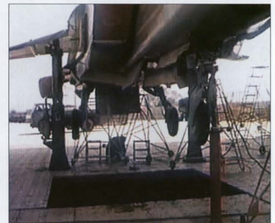
'48 Yellow' erected on the SSM dynamometric rig, with FOD protection screens on the air intakes. Note the open jet blast gate below the aircraft.
