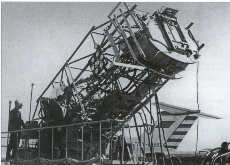
This test rig served for verifying the Yak-36's fuel system. A Yak-40 feederliner, СССР-87687, is parked beyond.
