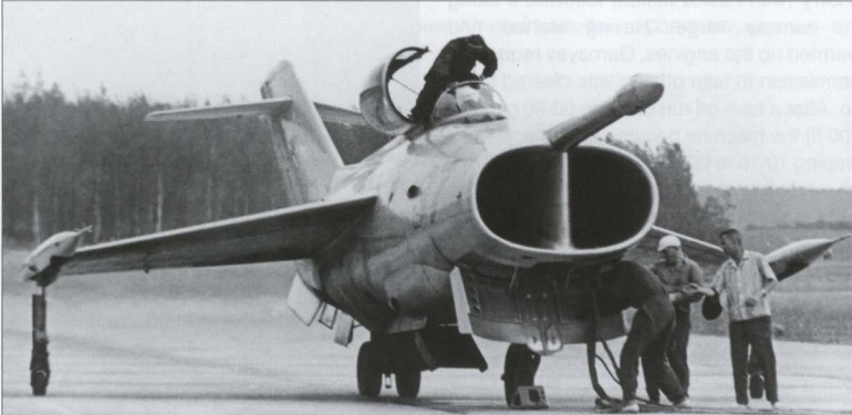
Above: '37 Yellow', the first flying prototype, shows off some of the modifications made in the course of the tests – the enlarged oval air intake, the hinged recirculation dams and the longitudinal strakes.
