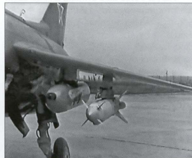
Close-up of the Kh-23 missile and the UPK-23-250 cannon pod under the mock-up's port wing.
