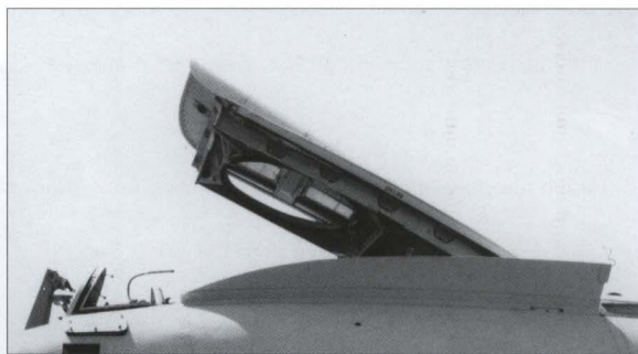
Above: The semi-recessed starboard nozzle of the main engine, with a heat shield aft of it. Right: The open lift engine air intake of a derelict Yak-38M.
