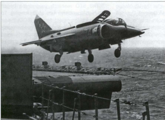
These pictures show Yak-38s '73 Yellow' and '74 Yellow' (c/ns 797786...286815 and 797786...286840) making short take-offs from SNS Novorossiysk during special tests (note the cameramen in the photo on the right). The aircraft have the late-model dorsal and ventral recirculation dams.
