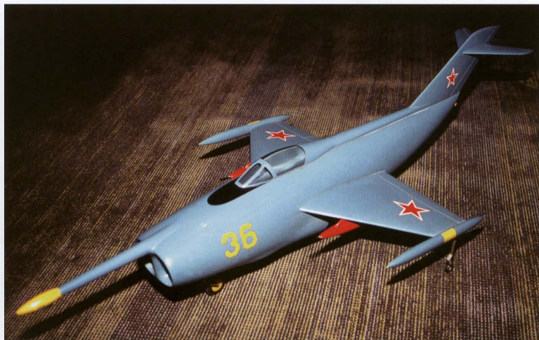
A desktop model of the Yak-36 (izdelye V) VTOL attack aircraft, showing the long outrigger boom of the forward reaction control nozzle. Note the cannon pods under the wings.
