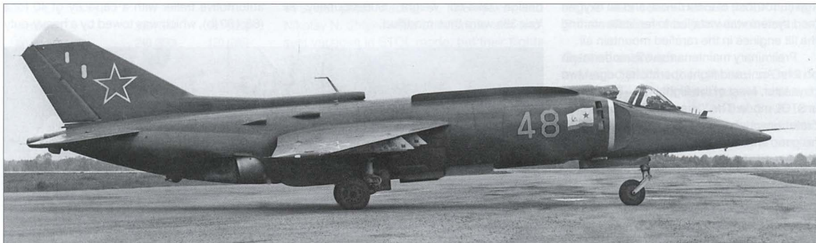
Three views of an early-production Yak-38M (f/n 0102). Note the longer dorsal recirculation dams, the larger main engine air intakes, the Opushka-VM FDR and the steerable nose gear unit with lateral doors only (no forward door segment).
