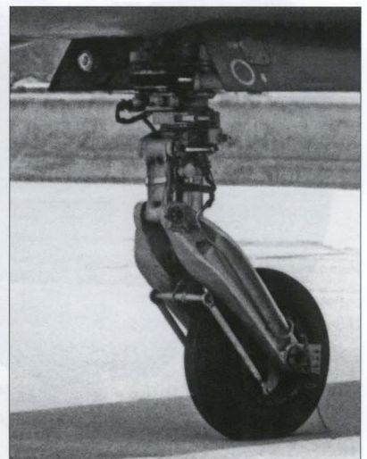
Above: The port main gear unit with its externally located retraction ram. Right: The nose gear unit features a remarkably small wheel.
