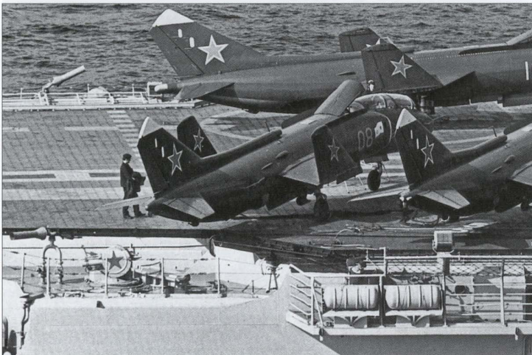
Above: Yak-38U '08 Yellow' shares the deck of SNS Kíev with two single-seat Yak-38s. One of them ('10 Yellow') has an Opushka-VM FDR on the tailcone.
