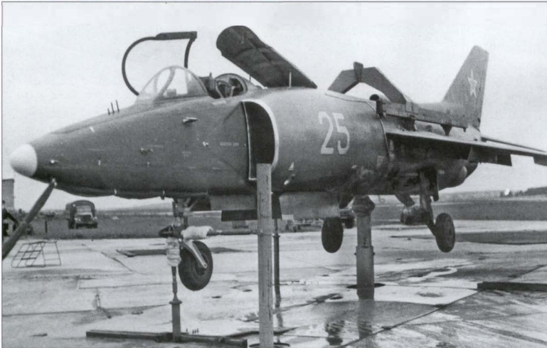
Centre left and above: The VM-2 ('25 Yellow') undergoes tests on the SSM rig, showing the original nose shape (long but still upturned) and the old squared-off tail. Note the fixture for the 'cable crane'. Centre: The second prototype in cruise flight. Centre right: The VM-2 was fitted with FOD protection grilles at some stage of the tests. Right and above: The second prototype was also used for testing the canopy jettison system. Here the canopy is jerked away by a special cable.
