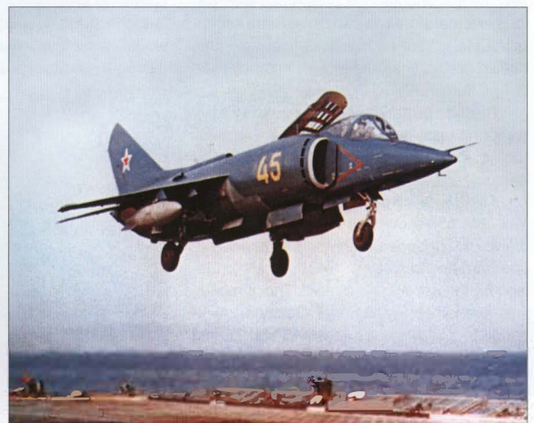
Above right: The same machine takes off vertically, toting two ZB-360 napalm tanks. Note the temporary airdata probe on top of the nose.
