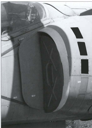
These photos provide a comparison of the main engine air intakes of the Yak-38 sans suffixe (left) and the Yak-38M. The latter's auxiliary blow-in doors are closed by ground covers.
