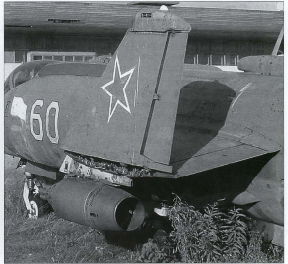
The folded wings of a Yak-38 sans suffixe , showing the ailerons; the starboard aileron has a trim tab. Note the ECM antennas at the wingtips.
