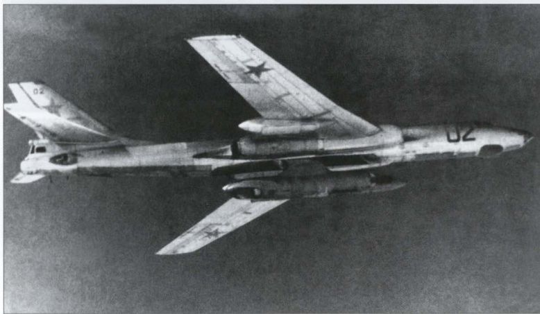
Above and left: Later, the propulsion rig was modified – the stub wings were removed and a massive double pylon was added on top. With the help of this pylon it was attached to a Tu-16LL engine testbed coded '02 Blue' (c/n 4201002). Called DLL, the rig was semi-recessed in the Tu-16LL's bomb bay on the ground and lowered clear before the R27V-300 engine was started.
