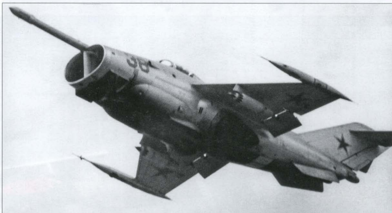
Above and below: Yak-36 '38 Yellow' takes off vertically at the Domodedovo airshow, belching smoke. Note the absence of the blow-in doors which were eliminated when the main intake was enlarged.
