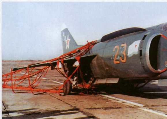
This production Yak-38 coded '23 Yellow' (possibly f/n 0703) was used for testing the crash barrier developed for Kiev class aircraft carriers. Note the dark green undersurfaces characteristic of production examples.
