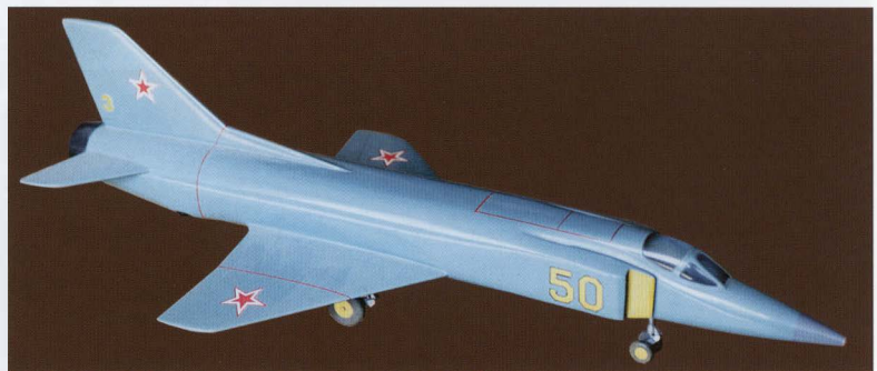
This desktop model represents the radically redesigned Yak-36P interceptor with low-set wings, an R79V-300 main engine, three lift engines and a radar. This project is described in Chapter 2.
