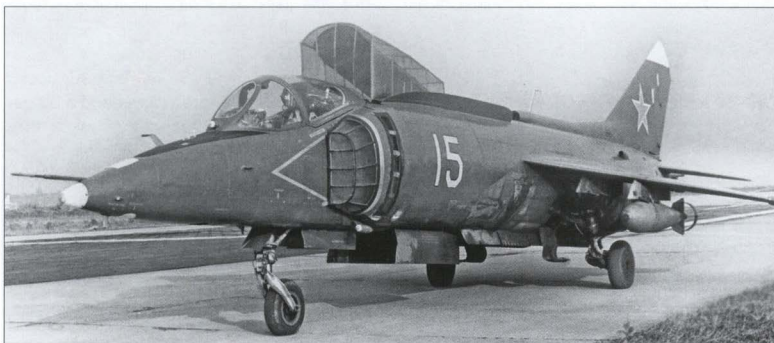
Yak-38 '15 Yellow' was used by LII for exploring the short take-off technique. FOD screens were fitted to all air intakes; the FAB-250M62 bombs were merely ballast to prevent a premature take-off.
