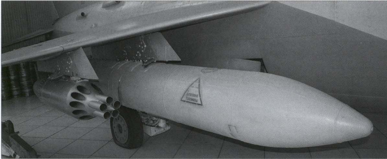
Above: The other wing of Yak-36M f/n 0201 with a 500-litre drop tank on the inboard pylon. Right: A dummy Kh-23M air-to-surface missile under the wing of a Yak-36M.
