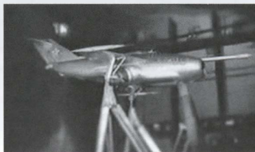
Above: Three views of the first Yak-36, '36 Yellow' (the ground test example), in the T-101 wind tunnel at TsAGI. Before that, the machine had already made tethered hovers. Note the sharply tapered wings.
