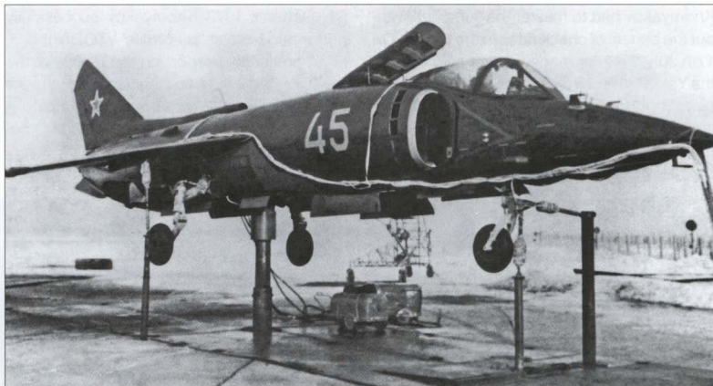
Above: The fourth prototype (VM-4) on the SSM dynamometric rig; note the sensor cable.
