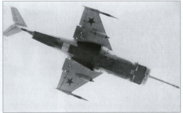
Left: The Yak-36 'cleans up' as it passes overhead; the outriggers retract first. Above: This view illustrates the shape of the Yak-36's fuselage which is bulged amidships and tapers off sharply towards the tail.
