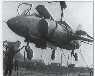
Top, right, and top right: '05 Yellow', the first prototype Yak-36M (the VM-1), on the 'cable crane' at Zhukovskiy. It, too, represented the short-nosed/square-tailed EVM configuration. Note the 'Danger, air intake' warning triangles, the tethering cables and the sensor cable leading to remote data recorders. Above: The VM-1 is towed at Zhukovskiy. Note the plain air intakes without splitter plates or blow-in doors. Above right: The first prototype undergoing tests on the SSM dynamometric rig.
