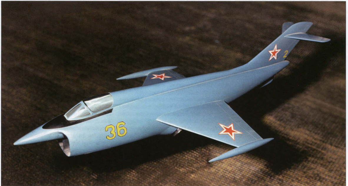
Another view of the Yak-36-70 desktop model, showing to advantage the redesigned nose, the fat spine aft of the cockpit and the neat nosecone incorporating the forward puffer instead of the Yak-36's distinctive 'matchstick'.
