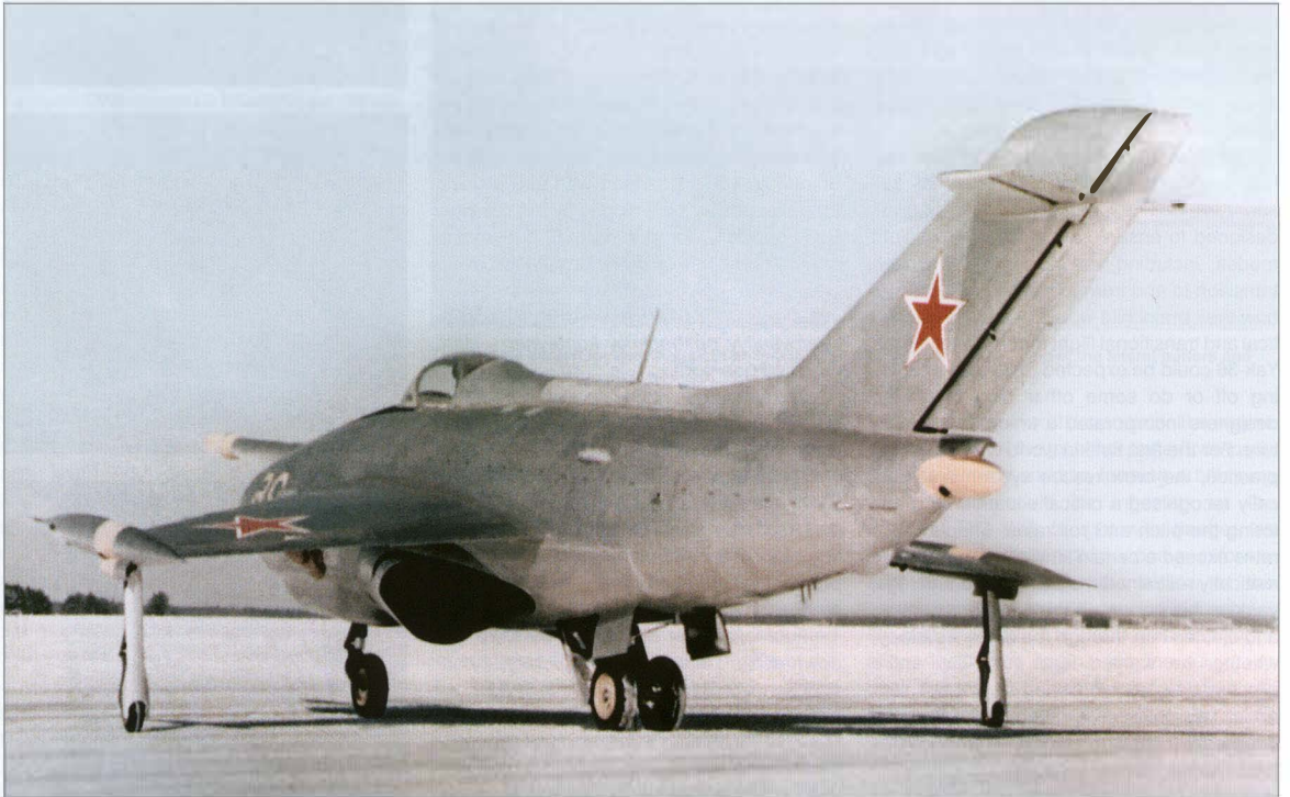
A three-quarters rear view of the same machine, showing the large vectoring nozzles in the forward thrust position and the lack of ventral fins. The nosewheel and the mainwheels were of identical size.
