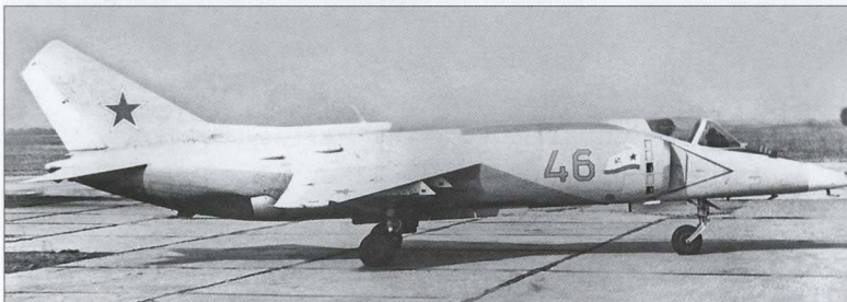
This grey-painted Yak-38, likewise coded '46 Yellow' and fitted with a VSPU-36, is a different machine (c/n 797786...174635, f/n 0312). Note the RR8311-100 air sampling pod for radiation reconnaissance.
