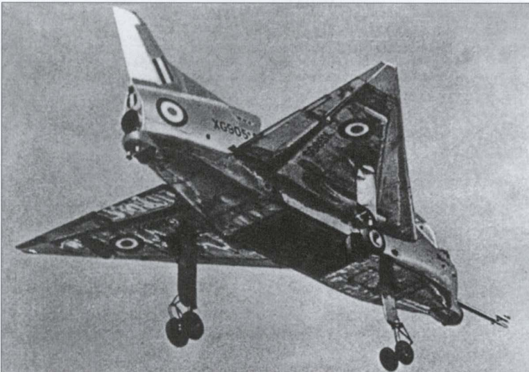
The second SC.1 (XG905) in flight, showing off its tailless-delta layout, the rectangular exhaust port of the four lift engines and the reaction control puffers under the nose, tail and wingtips.
