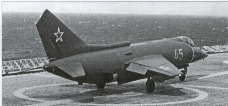
This view of the VM-4 on the Kiev's deck shows well the raked fin tip introduced on this aircraft and adopted for production.
