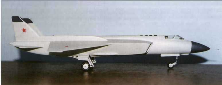
Three views of a desktop model depicting the early version of the Yak-41M with the larger LERXes, redesigned air intakes, strongly tapered wings and stabilizers, and splayed vertical tails.
