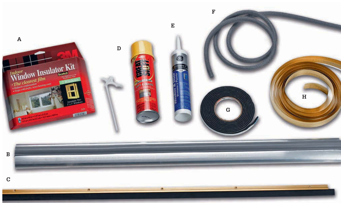
Weatherizing products commonly found in home centers include: A clear film, heat-shrink window insulator kit (A); an aluminum door threshold with vinyl weatherstripping insert (B); a nail-on, rubber door sweep (C); minimal expanding spray foam (D); silicone window and door caulk (E); open-cell foam caulk-backer rod (F); self-adhesive, closed-cell foam weatherstripping coil (G); flexible brass weatherstripping coil, also called V-channel, (H).
