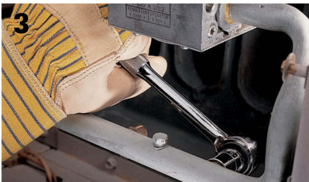
3 To avoid bending or damaging the spud threads, hold the manifold steady with one hand as you remove each spud.
