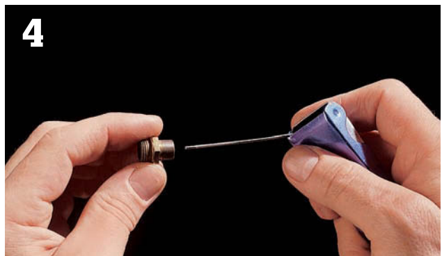
4 Clean each spud orifice carefully with a pilot jet tool, taking care not to scratch or enlarge the orifice.
