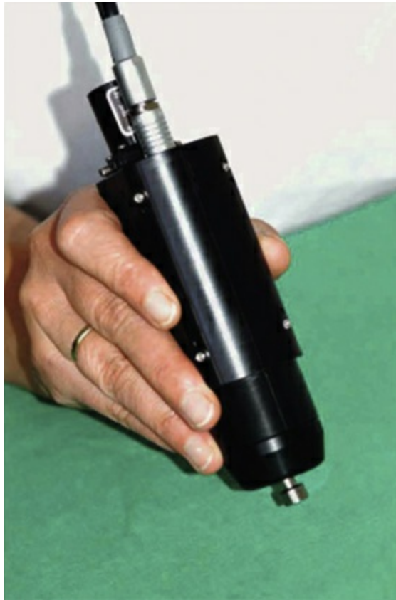
FIG. 11.7 Prototype of a handpiece for three-dimensional high-frequency scanning using the VuMax UBM 35/50 (Sonomed).
