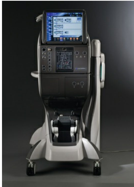
FIG. 115.13 Front view of a new Constellation© vitrectomy unit, providing phacoemulsification, vitrectomy, photocoagulation, diathermy, and air/gas/silicone tamponades in one machine.
