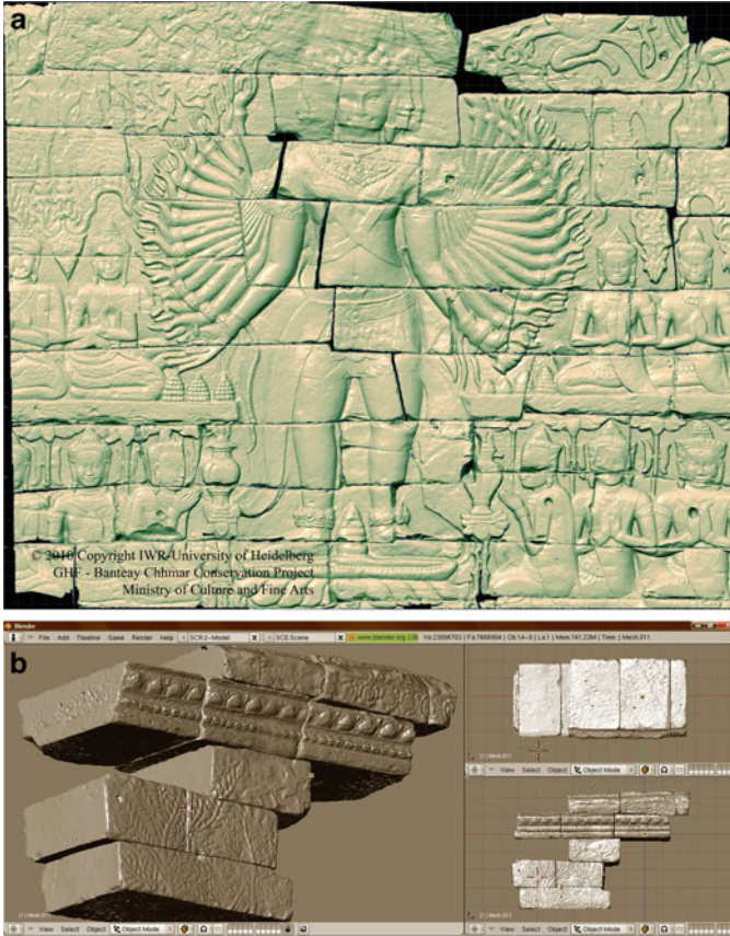
Fig. 8 (a, b) 3D digital scanning of Avalokiteshvara bas-relief and other wall portions (GHF, IWR University of Heidelberg, Ministry of Culture and Fine Arts Cambodia, 2010, 2012)
