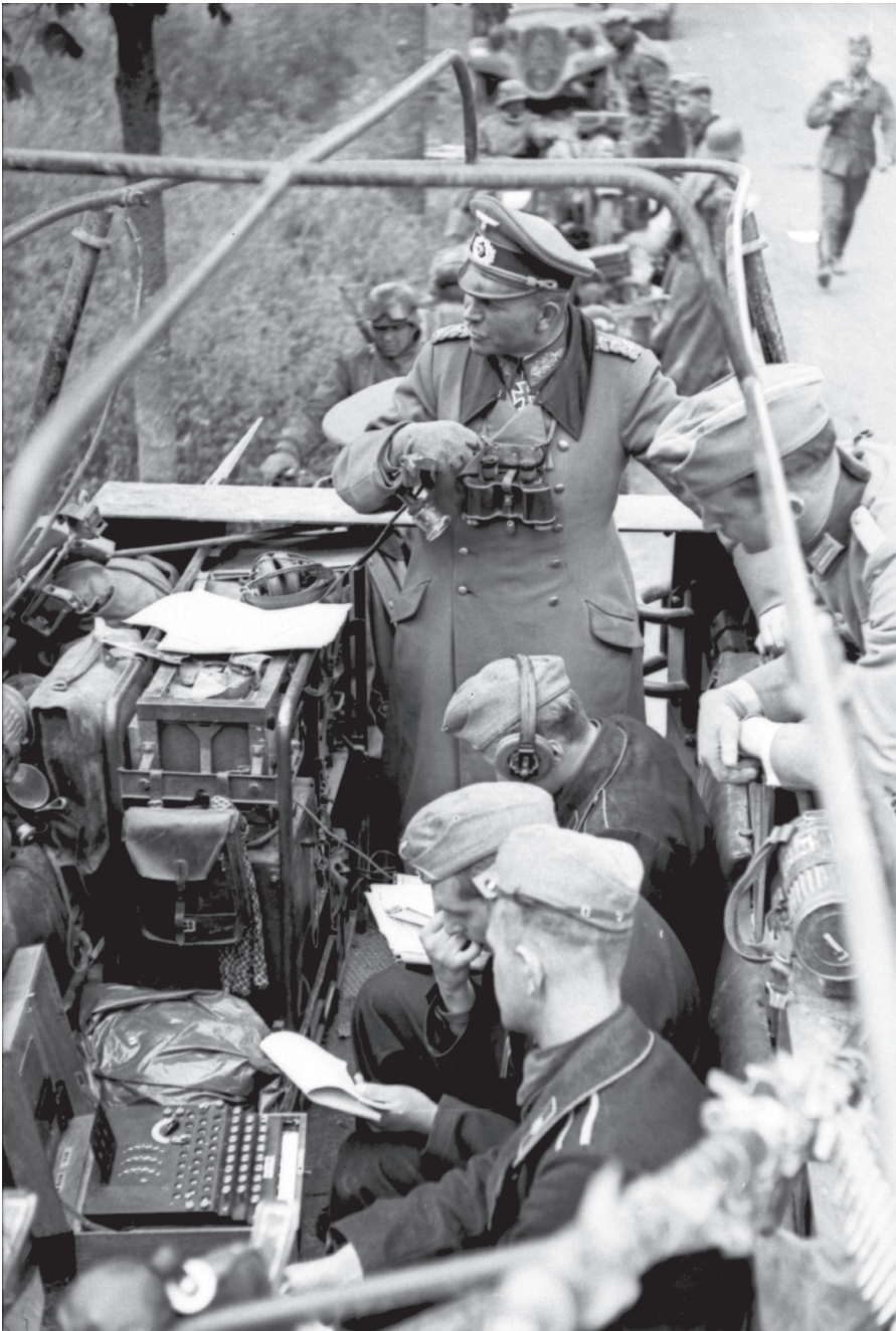
General Heinz Guderian in his armored command carrier during the Battle of France in May 1940; front left an Enigma cryptographic machine. Photographer: E. Borchert. BArch/101I-769-0229-12A.
