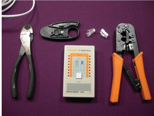
FIGURE 3.4 Patch cable tools
