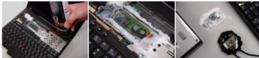
Figure 30: demonstration of the Cold Boot RAM Extraction method
