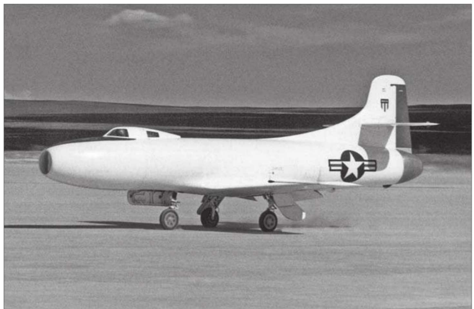
Three turbojet-powered Douglas D-558-I Skystreaks were built as research aircraft for the US Navy and NACA in the late 1940s, although the rate of technical advancement soon made them obsolete. NASA
