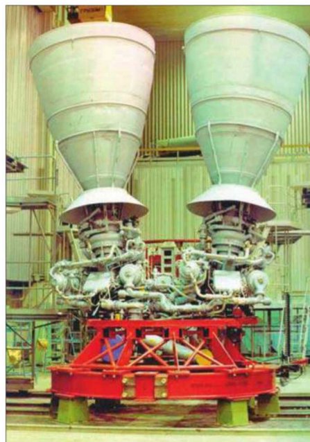
This page, left: The RD-701 tri-propellant engine was specifically developed by Glushko for the MAKS spaceplane. This very efficient engine would initially use kerosene and LOX and then switch to liquid hydrogen and LOX to provide a higher specific impulse. RKK Energia
