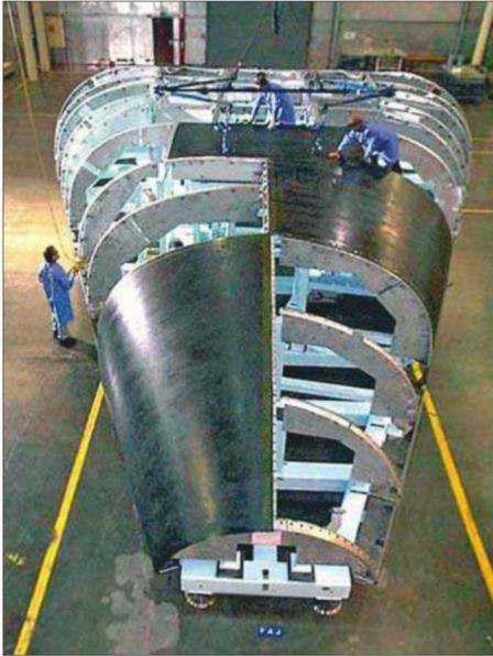
Top left: Forward section of the X-33 airframe under construction. Lockheed Martin
