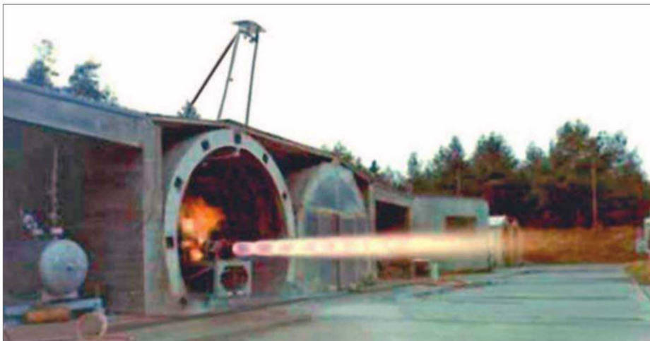
A scale sized liquid fuel engine proposed for the Silbervogel spaceplane is tested at the Trauen rocket facility in Germany during 1942. Bill Rose
