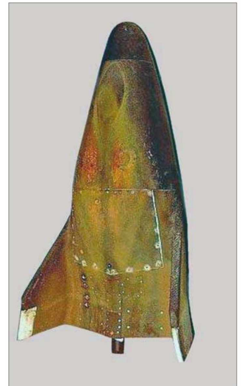
Below: Built by Martin Marietta, the X-23A Prime was a small rocket-launched lifting body hypersonic test vehicle. USAF
