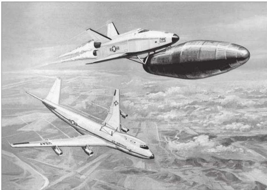
Left: Another image showing an ALSV launch from the back of a modified Boeing 747-200. In this case the carrier aircraft has a V-tail. USAF
