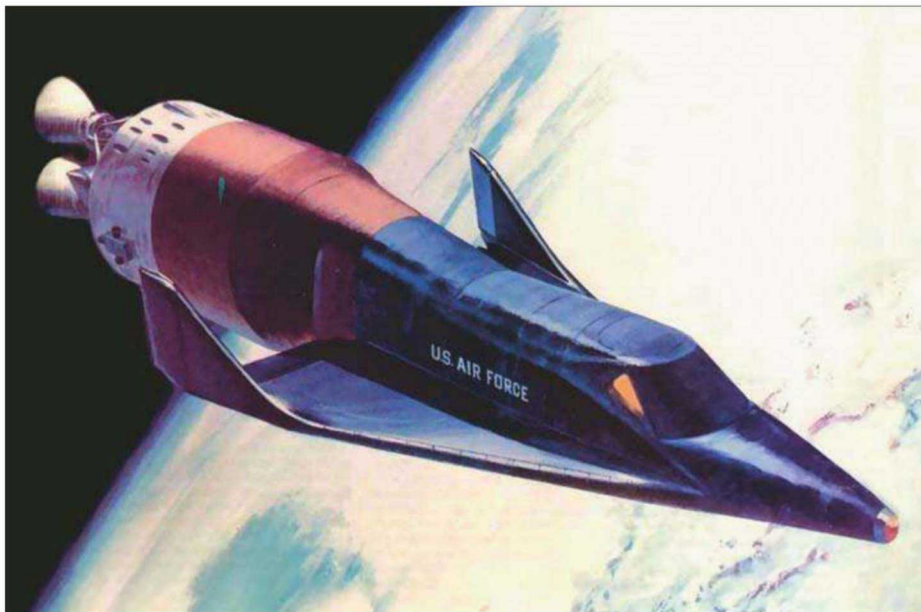
Artwork depicting the Boeing X-20 in orbit, with transition stage attached and windshield protector in place. USAF
