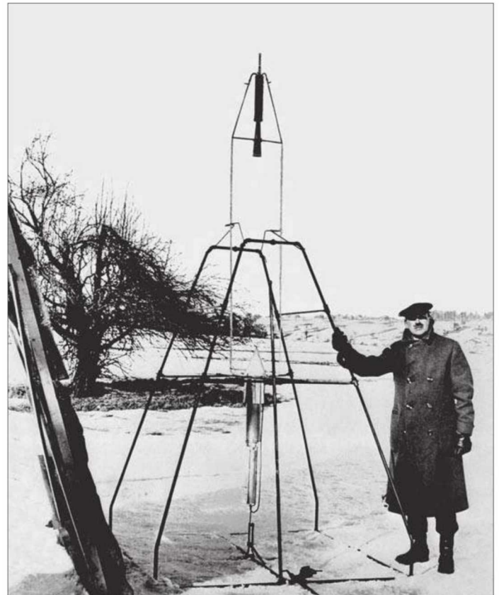
Above: American rocket pioneer Dr Robert Goddard stands beside a small liquid fuel rocket on 16th March 1926. NASA
