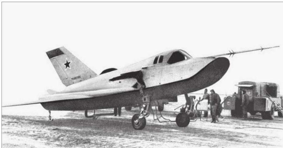
Atmospheric test version of the MiG spaceplane designated 105-11. This prototype was equipped with many components intended for use with the more advanced versions. NPO Mash
