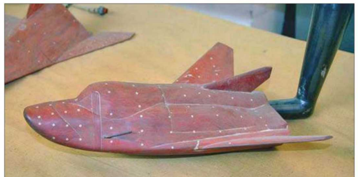
Below right: A small wooden model of the BOR-4 vehicle produced at TsAGI during the 1970s. In the background is what appears to be a wooden model of the earlier M.48 spaceplane. RKK Energia
