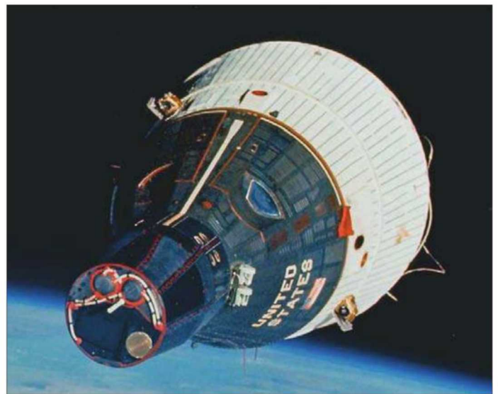
Bottom right: This Gemini B spacecraft in USAF markings was used for heat testing purposes. Gemini B was not intended to function as a stand-alone spacecraft and would have been used as a crew return vehicle for the MOL. It is currently on display at the National Museum of the USAF. USAF
