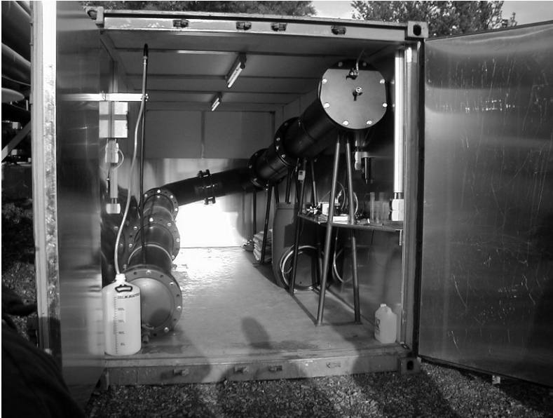
Fig.3. Investigation container with reactor on site at the Königstein mine site.
