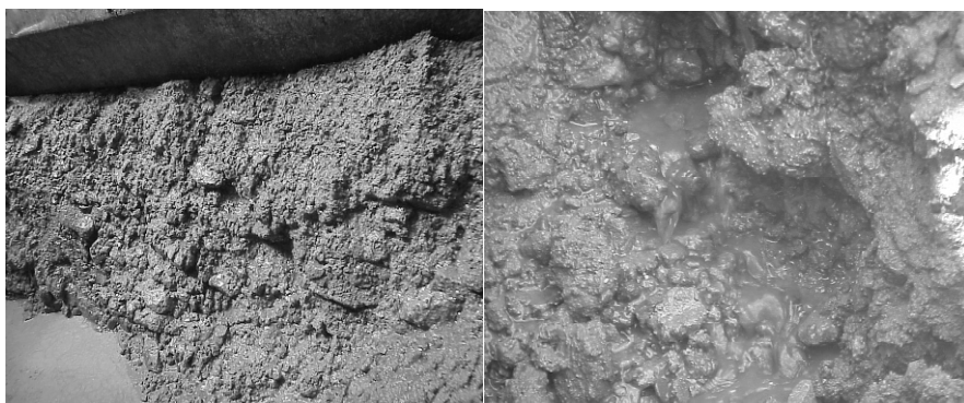
Fig.1. The sediments fragment from the PRB wall on the test site.
