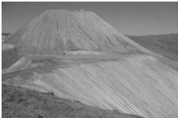
Fig. 2. “The Taboshar Hill”, a pile of ground low grade uranium ore.
