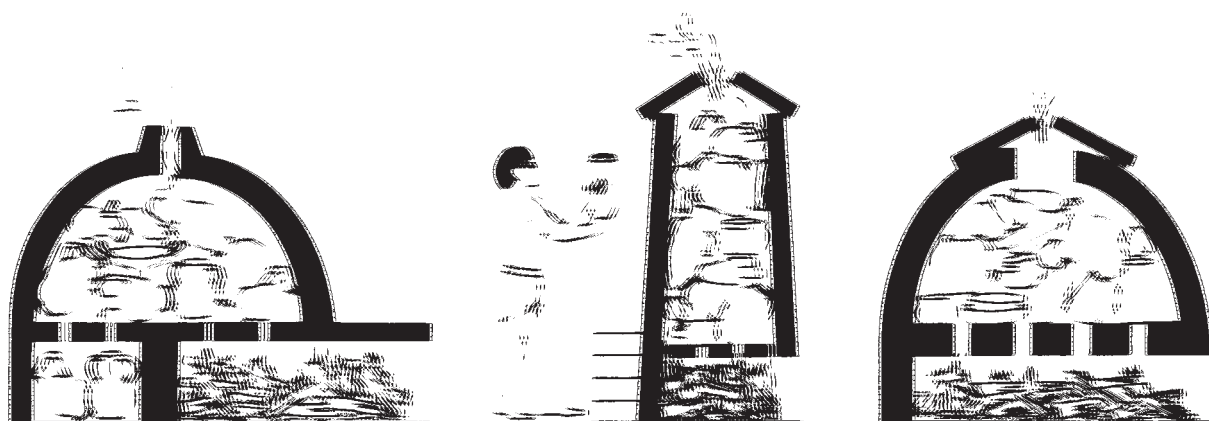
8.38 Pyrotechnology: the control of fire. Initially pottery was made in an open fire. The introduction of the potter's kiln meant higher temperatures could be achieved, also spurring on the development of metallurgy. (Left) Mesopotamian dome-shaped kiln of the early 4th millennium BC, built largely of clay, with an outer wall of stone or mud brick. (Center) Egyptian kiln of c. 3000 BC reconstructed from tomb paintings. The potter may have stood on the small platform to load the kiln. (Right) Greek kiln of c. 500 BC, reconstructed from scenes on Corinthian plaques: the extended fire opening probably improved combustion.
