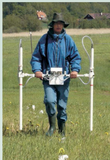
3.55 The Bartington Grad601-2 single axis, vertical component high-stability fluxgate gradiometer system.
