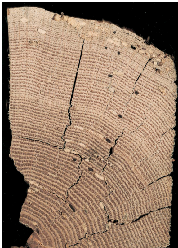
4.14 Section of an oak beam from the wall of a log cabin in Hanover, Pennsylvania, USA: the annual growth rings are clearly visible, and since this sample contains complete sapwood (top of image), a precise felling date of 1850/1 can be established.
