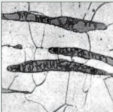
8.45 Wrought iron at x200. The light grain is iron, the darker material slag.
