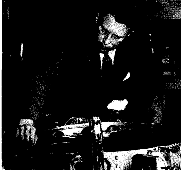
24. Lawrence's Nobel Prize-winning cyclotron battered secrets from the nucleus and proved a potent source of neutrons. Here Lawrence examines the vacuum chamber of the 37-inch machine, completed in 1937.
