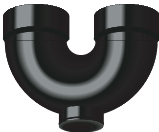
trap U-shaped pipe beneath a fixture containing a quantity of water to prevent sewage gases from escaping.
