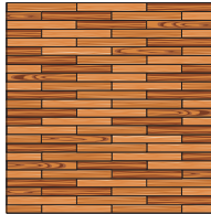
strip flooring with alternate joints
