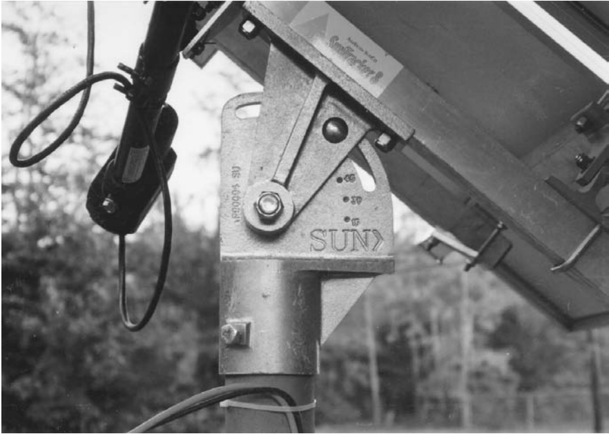
FIGURE 8-19 Actuator motor of the suntracker. (Source: American Sun Company, Blue Hill, Maine. With permission.)
