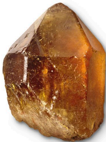
Natural citrine | Much of the "citrine" quartz variety in the marketplace today is heat-treated amethyst. This Brazilian crystal is totally natural, and shows some water wear.
