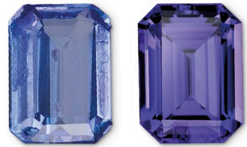
Tanzanite surface coated to deepen and improve color—before (left) and after (right)
