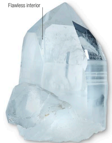
Rock crystal rough | This well-formed crystal is internally flawless, and is suitable for cutting into gems, carving, or being sliced into oscillator plates for electronics.
