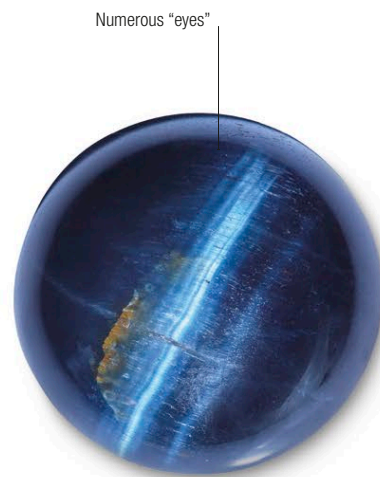
Hawk's-eye quartz | The rich blue color in hawk's-eye quartz comes from numerous parallel fibers of the mineral crocidolite enclosed within it.
