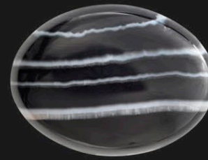
Onyx RI 1.54–1.55 Onyx can be black or brown with white color banding, giving a fairly restrained dispersion.
