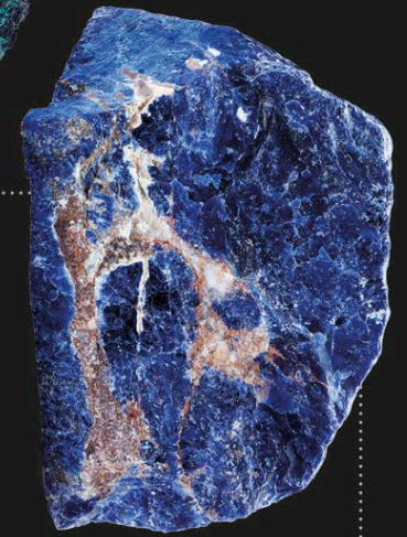
Sodalite RI 1.48 Transparent sodalite is rare, and its RI is low; however, good quality gemstones can be cut.
