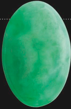
Jadeite RI 1.65–1.68 Jadeite varies in color, and is white in its pure form. It has a moderate amount of dispersion.
