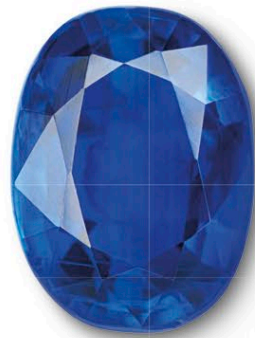
Kyanite | See p.280 | Kyanite has a vitreous, pearly luster and is blue, green, brown, yellow, red, or colorless. It ranges from transparent to translucent.
