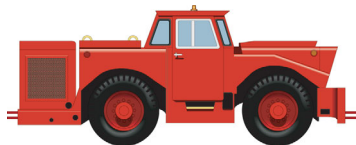
tow tractor Very heavy vehicle that pulls or pushes an aircraft onto the maneuvering area or the parking area.
