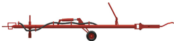
tow bar Device that connects the tow tractor to the aircraft's front landing gear.
