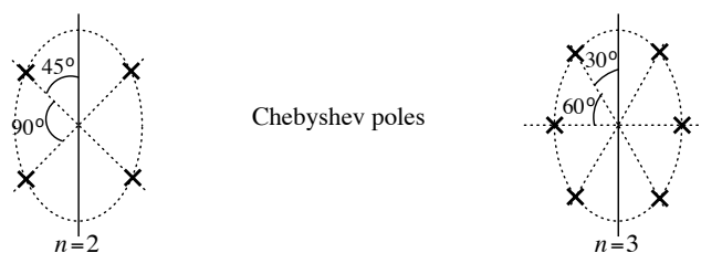
Figure 13.11 Pole locations of Chebyshev lowpass prototypes
