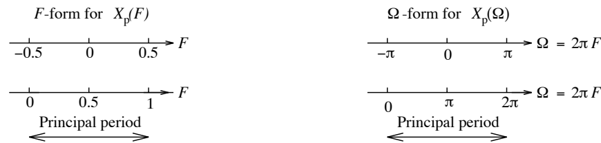
Figure 15.2 Various ways of plotting the DTFT spectrum
