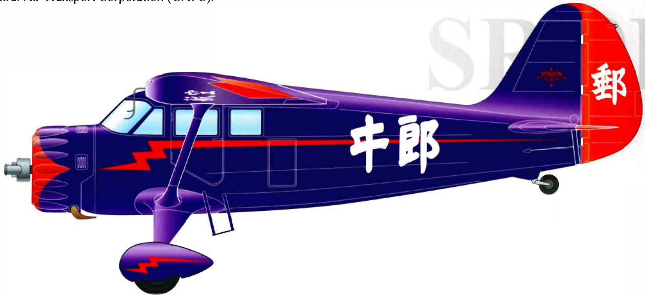
Stinson SR-9D Reliant Stinson SR-9D Reliant "Niulang" of the South-Western Aviation Corporation (SWAC), probably c/n 5250 or 5251. This was one of nine Stinson Reliants of different models that were used by this Canton-based company.
