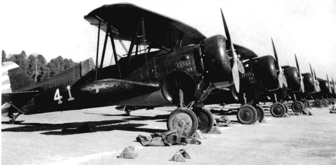
The first Curtiss Hawk III fighters with retractable undercarriage were delivered in 1936.
