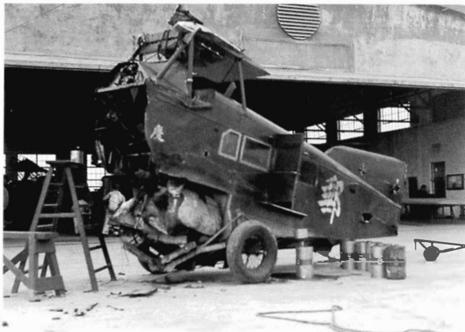
Centre: The hull of a damaged Loening Air Yacht, No 2 "Anking" or No 6 "Chungking".
