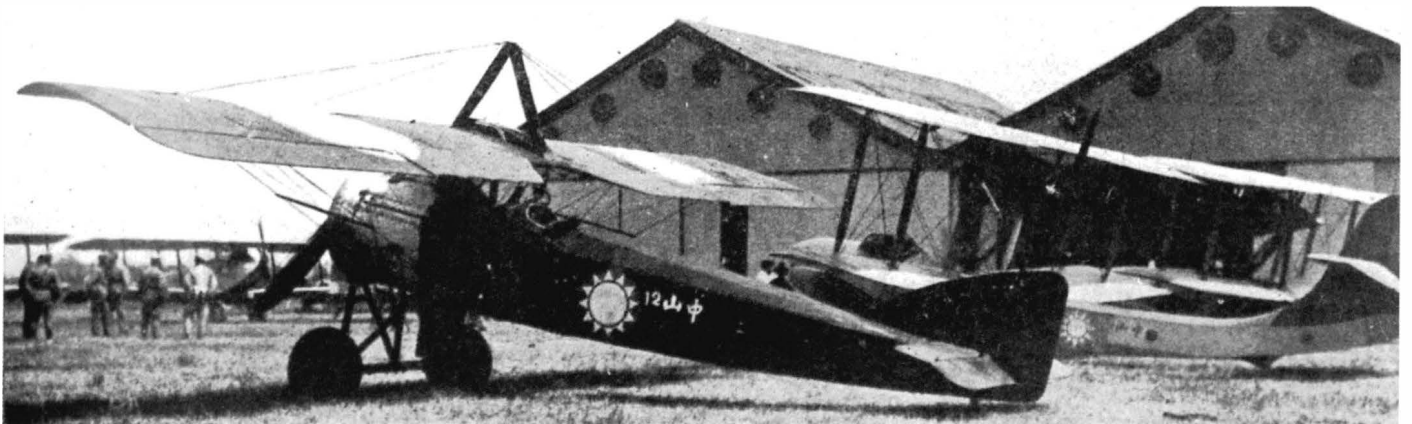
Morane Saulnier MS 35 "Shan Chung 12". The aircraft behind is a Schreck FBA 17 amphibian.
