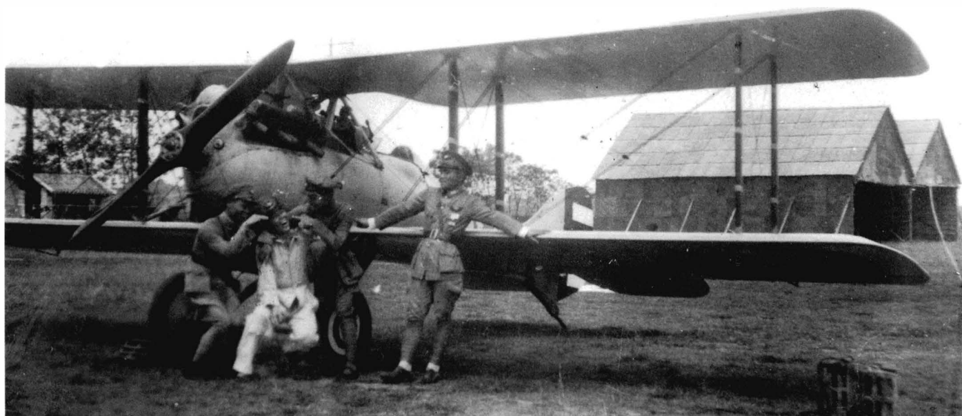
A number of Japanese aircraft were acquired by Kwangsi in 1934-35, including old Nakajima Army Type Ko 4 Fighters (Nieuport ND 29C1). (Wings of China)
