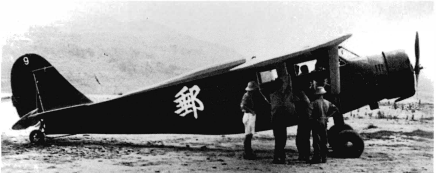
In 1930 six Stinson SM-1F Detroiters were transferred to CNAC from the Nanking Government. No 9 "Tientsin" has been modified and fitted with an engine cowling.
