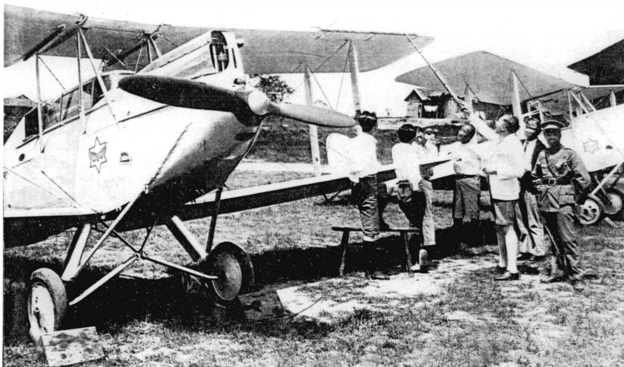
The leading edge slats of Chang Hsueh-liang's personal de Havilland DH 60M Moth de Luxe being demonstrated at Mukden.
