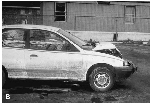
Figure 12 (A) and (B) A 1995 GEO Metro with minor front-end damage consistent with an impact speed of less than 15 k.p.h. (9 m.p.h.).
