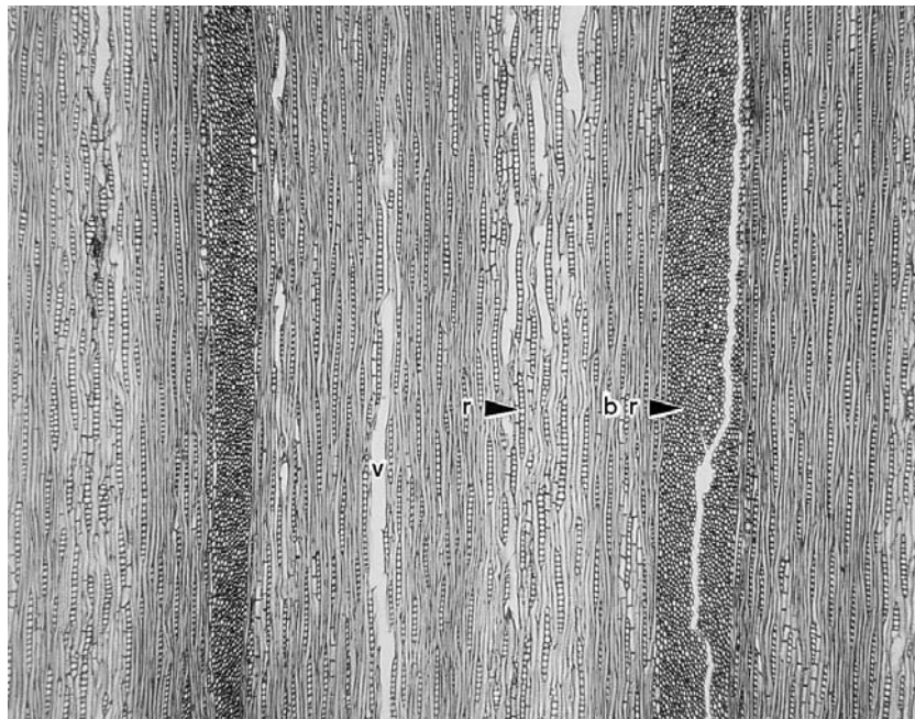
Figure 6 Tangential section of oak. br, multiseriate ray; r, uniseriate ray; v, the hole left by a vessel which was torn away in sectioning. Vessels are tubes, composed of cells connected end to end (vessel elements), which are aligned roughly parallel to the other fibrous elements in the wood. Compare with Fig. 5. Original magnification \times 40 .
