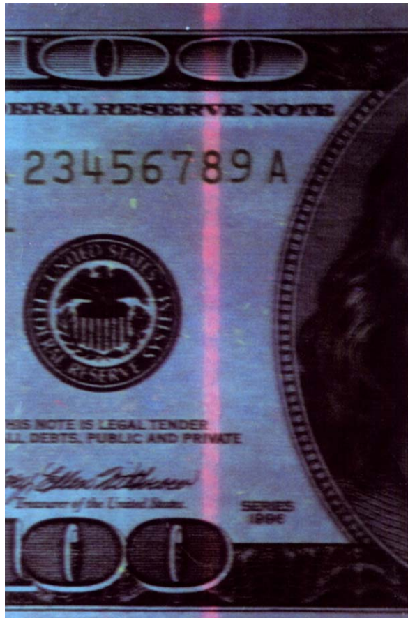
Plate 28 FORGERY AND FRAUD/Counterfeit Currency Fluorescence of genuine US $100 FRN security thread.
