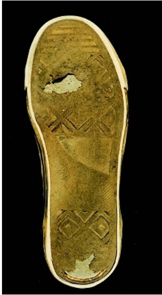
Plate 40 PATTERN EVIDENCE/Bare Footprint Marks Outsole of a running shoe, showing wear areas on the ball of the foot and the heel.
