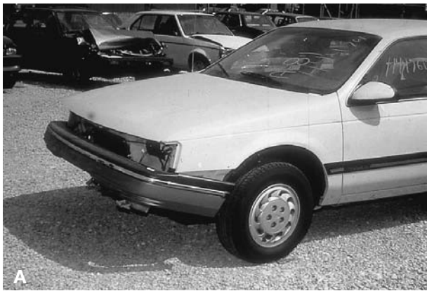
Figure 10(A) and (B) A 1991 Ford Taurus was involved in a very minor glancing collision between the front bumper and a guardrail. There was no underlying frame, fender or structural damage.
