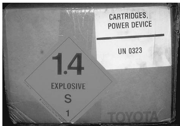
Figure 1 The air bag is transported as an explosive material. Sodium azide is the explosive propellant used in the majority of air bag modules.
