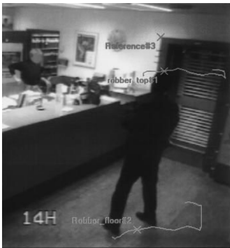
Figure 8 Measuring the height of a robber by reverse projection from a digitized surveillance video recording. The height was calculated from an image sequence and the path of the robbers movement in the bank have been tracked.
