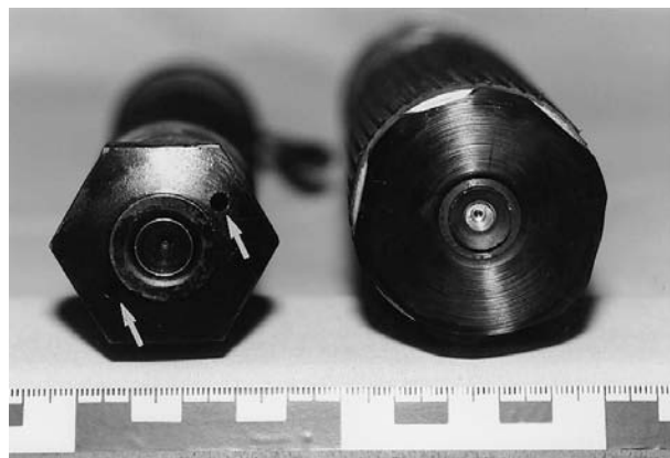
Figure 2 Muzzle end of two captive-bolt stunners. Left: Kerner type with two opposite openings (outlets for the explosion gases; arrows); right: Schermer type without additional smoke conduits.
