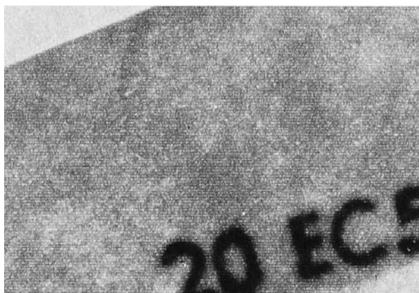
Figure 2 A notation '20EC5' on the inside flap of an envelope represents the stock number (20), the initials of the company that placed the order (EC) and the last digit in the year of manufacture (5).
