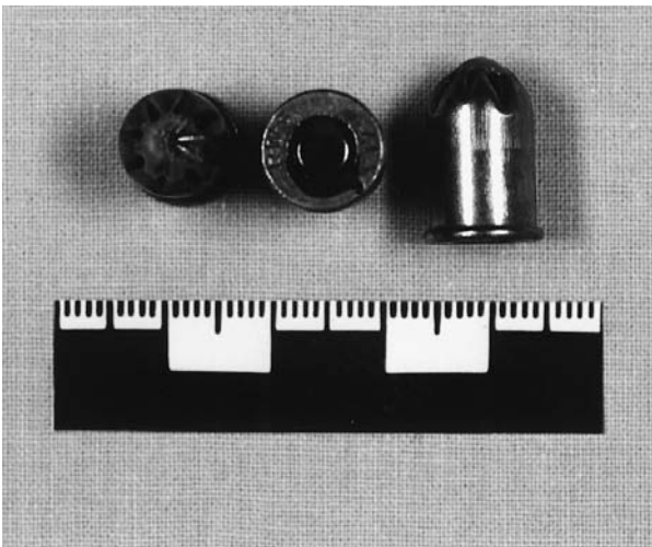
Figure 3 Blank ammunition for captive-bolt stunners. Cattle-killing cartridges RWS 9 × 17 mm; the case mouth is sealed by crimping the metal and inserting a wax plug. The strength of the cartridge is designated by a green color marking on the base of the case ('green' meant for small cattle and pigs).
