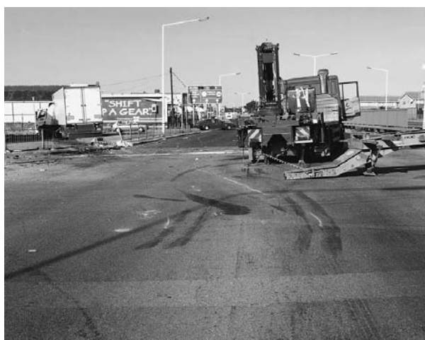
Figure 1 Tire marks scrapes and gouges can be seen in the roadway following this incident involving two goods vehicles. © Metropolitan Police Service.
