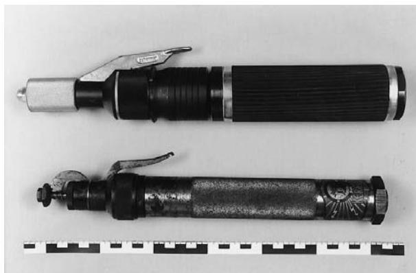
Figure 1 Two makes of captive-bolt stunners. Top: Schermer type (mod. ME, cal. 10 × 11 mm, diameter of the bolt 12 mm); bottom: Kerner type (mod. 289, cal. 9 × 17 mm, diameter of the bolt 11 mm).
