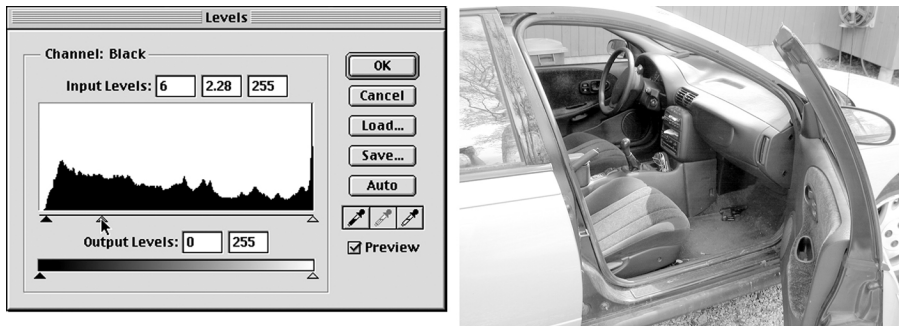
Figure 17 Adjusting the gamma value by shifting the mid-grey point on the histogram of Figure 14 , and the resulting altered contrast.
