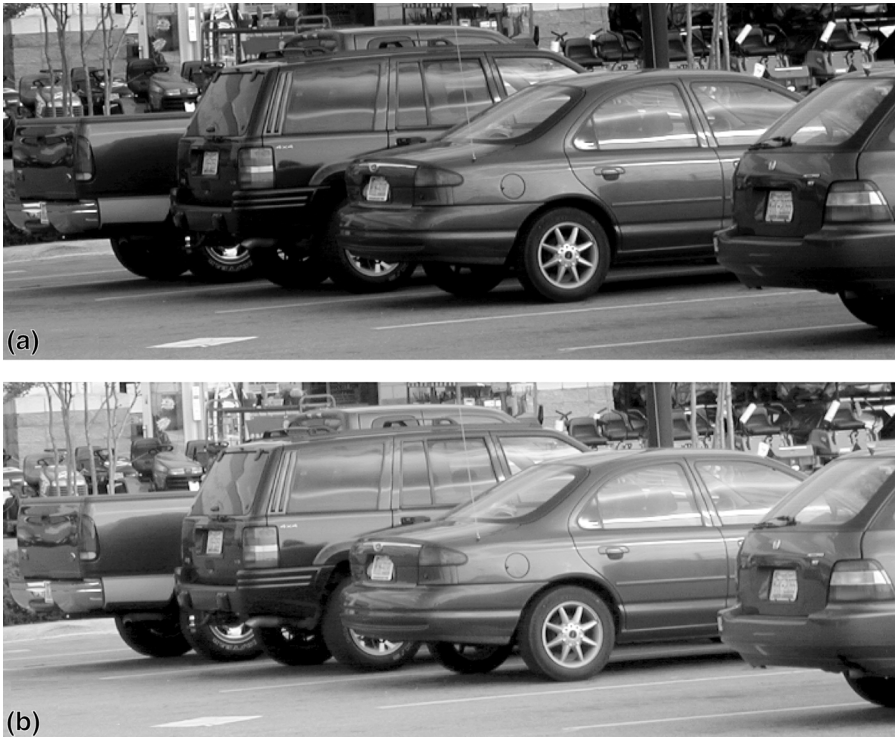
Figure 20 Image of cars in a parking lot: (a) as photographed; (b) after adjustment of R, G, and B intensities to make the paving neutral grey (Plates 10 and 11).
