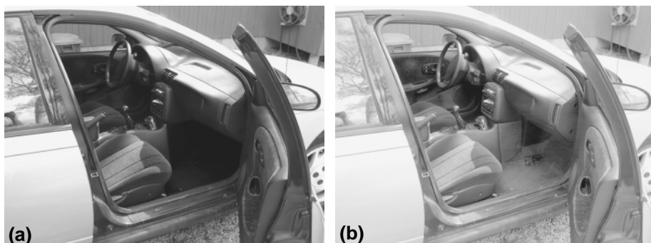
Figure 9 Example of contrast expansion to show details in a dark region: (a) original; (b) expanded contrast, as described in Chapter 2.
