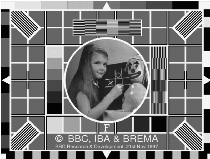
Figure 27 Typical video test pattern, which includes sets of horizontal and vertical lines to test spatial resolution and areas with uniform grey steps used to test tonal resolution. The pattern is also used to test for image distortion, and has areas of known colors to test for color rendition.
