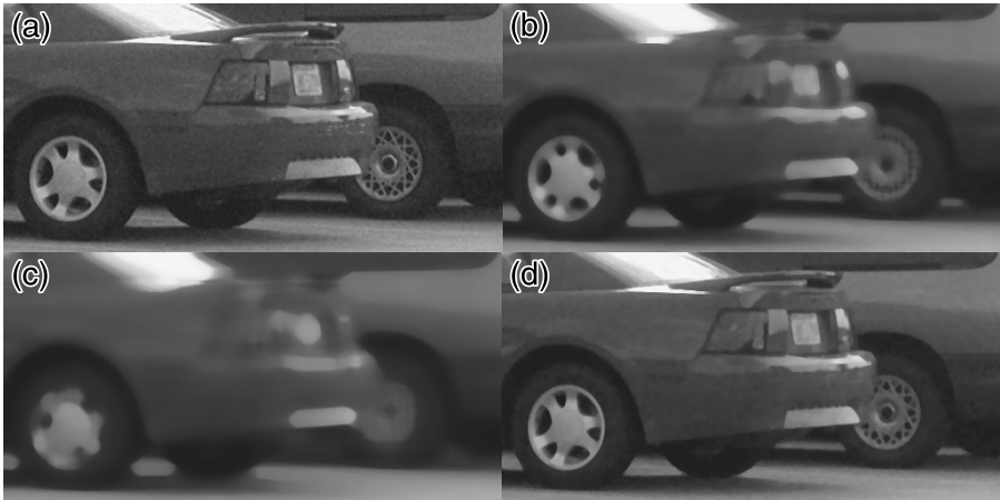
Figure 5 Application of a median filter to the image from Figure 3 : (a) 3 pixel wide neighborhood; (b) 11 pixel wide neighborhood; (c) 21 pixel wide neighborhood; (d) 3 pixel wide neighborhood, repeated 10 times.
