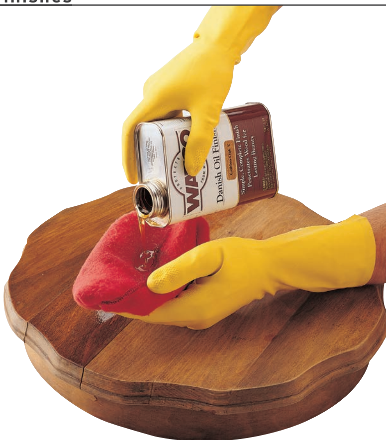
Penetrating oil application.
