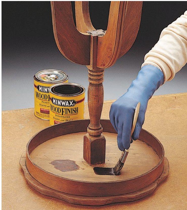
Testing stain colors on a hidden area.
