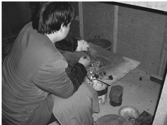
Figure 4.3. A worker is de-soldering circuit boards over a grill. The E-waste recycling practice causes severe environmental pollution of PBDEs and other contaminants in Guiyu.
