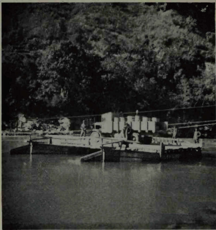
A pontoon ferry on Mekong River made of gasoline drums.
