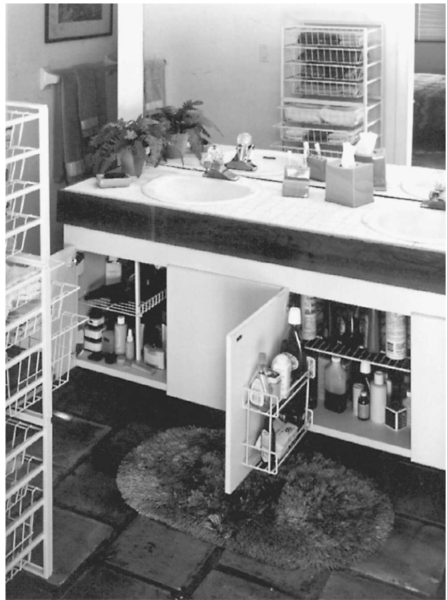
Fig. 19-41 Bathroom storage and convenience can be increased by using racks and shelves that swing or roll out to save shelf space. (Closet Maid by Clairson.)
