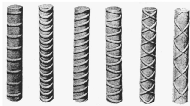
Fig. 3-19 A. Identification for ASTM standard reinforcing bars. B. Various types of deformed bars.
