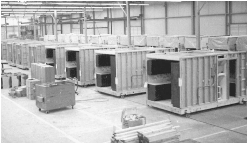
Fig. 18-18 Units are wrapped before being shipped to the job site. (Western Wood Products.)
