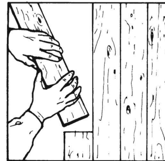
Fig. 17-82 Placing a piece of cut-to-fit red cedar lining vertically in a closet. (Grossman Lumber.)
