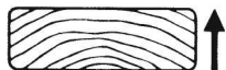
Fig. 3-57 The bark side of the lumber is exposed when using treated wood for a deck or other exposed surface. (Southern Forest Products Association.)
