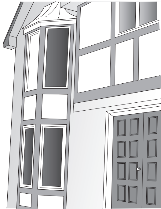
Fig. 5-55 A. A bay window rests on overhanging floor joists. B. A different type of bay. Both types rest on overhanging floor joist systems.
