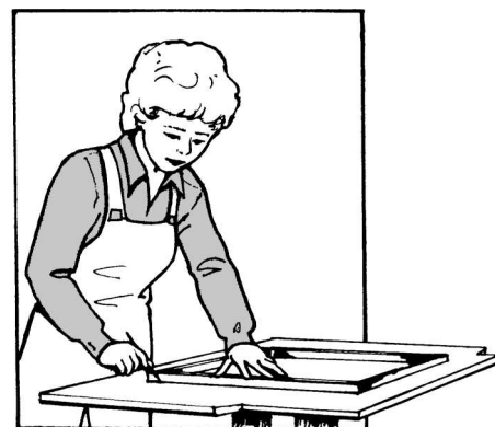
Fig. 17-36 A. Edges may be trimmed with edge trimmers or routers. (Rockwell International, Power Tool Division.) B. Edges may also be files. Note direction of force. C. Marking around the sink rim for the cutout in the countertop. (Grossman Lumber.)
