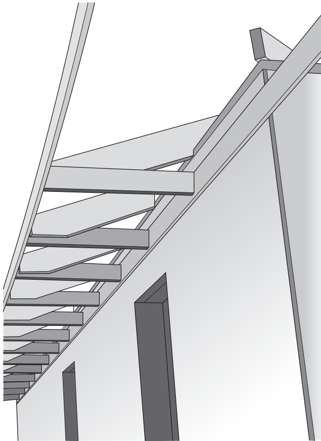
Fig. 10-28 Lookouts are nailed first to the rafter tail. Then they are toenailed to a solid part of the wall.
