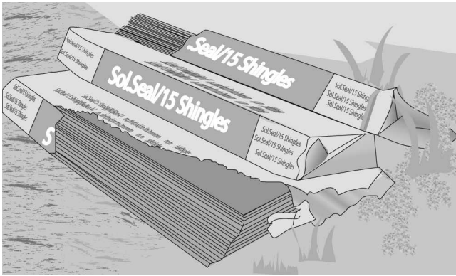
Fig. 2-35 Broken bundle of shingles.
