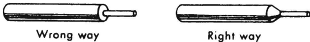
Fig. 11-26 The right and wrong ways to cut insulation from a piece of wire.
