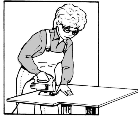
Fig. 17-32 Cutting plastic laminate with a saber saw. (Grossman Lumber.)
