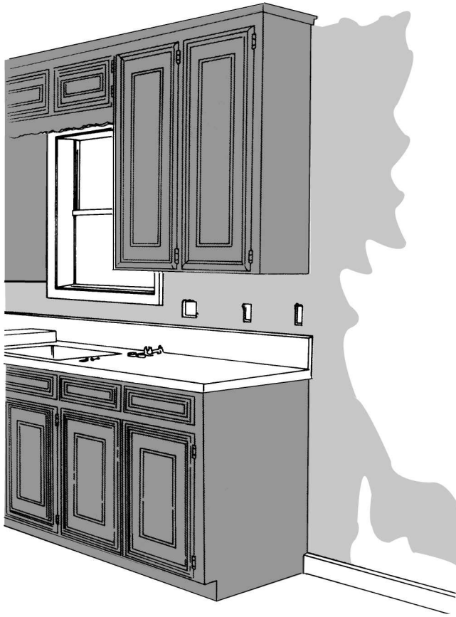
Fig. 15-59 Cabinets are stained before walls are painted or papered. Note the overspray around the edges.
