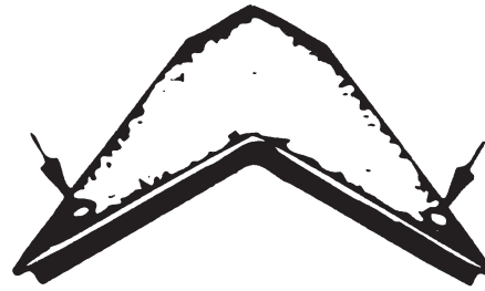
Fig. 8-75 Seal down each installed ridge unit with elastomeric adhesive, and face nail each shingle with two nails. (Ridglass.)
