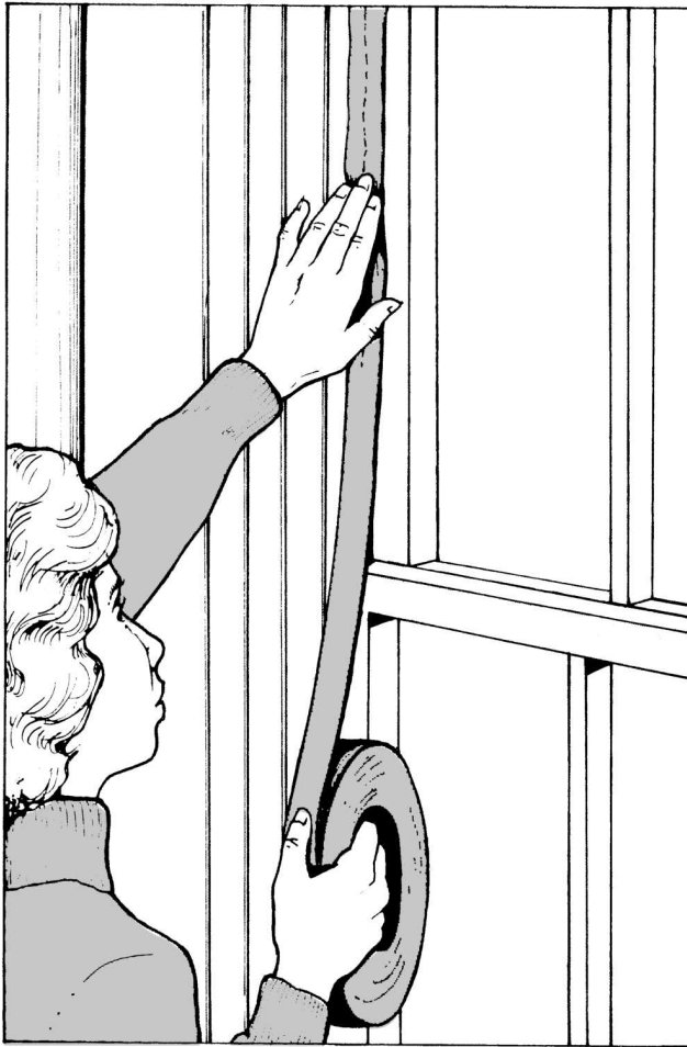
Fig. 13-57 Applying clear tape around windows. (Manco Tape.)
