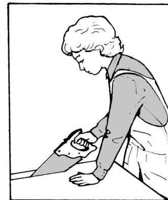
Fig. 17-33 Cutting laminate with a hand saw. (Grossman Lumber.)
