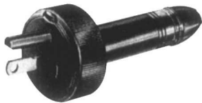
A ground continuity tester for use on energized circuits only. It is equipped with a ground and a neutral blade. If the light comes on when it is plugged into a grounding-type receptacle, the ground continuity is complete. If the light does not come on, there is a fault in the circuit. It uses a penlite cell for power.
