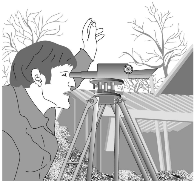
Fig. 2-12 Using the optical (or builder's) level on the job. (David White Instruments.)
