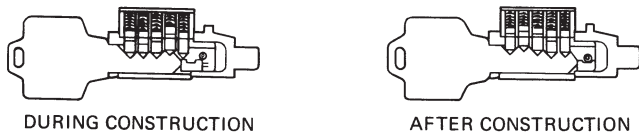
Fig. 9-121 Construction keying of locksets. (National Lock.)
