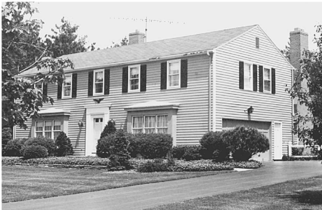
Fig. 7-5 Two-story house with a gable roof. Note the bay windows with a hip roof.
