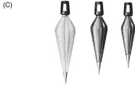
Fig. 1-27 A. Using a level to make sure that a window is placed properly before nailing. (Andersen.) B. A commonly used type of level. (Stanley Tools.) C. Plumb bobs. (Stanley Tools.)
