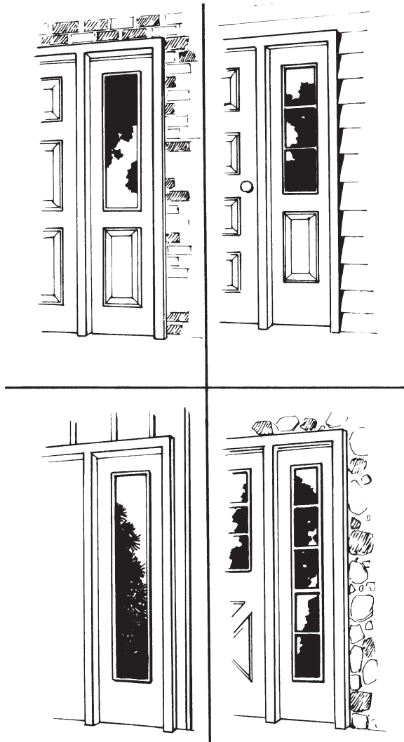
Fig. 9-81 Sidelights are designed for fast installation as integrated units in wood or plastic models. This insulated safety glass comes in 12- or 14-inch widths. (General Products.)
