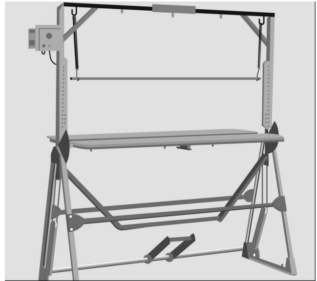
Fig. 21-41 A thermal cutter. Note the white line that is part of the cutting device. It is attached to the transformer on the left of the framework. (PCC.)
