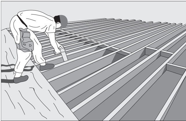
Fig. 5-27 Installing engineered wood joists.
