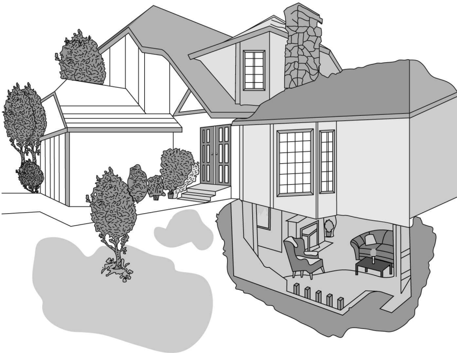
Fig. 22-3 A cutaway showing the comfortable room addition possible by using a PWF for a house.
