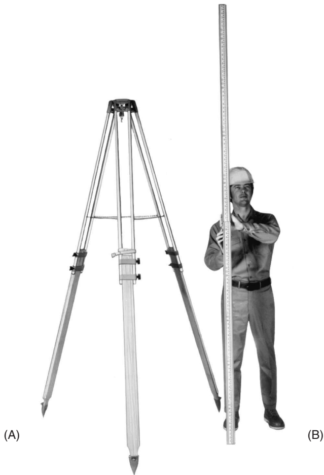
Fig. 2-13 A. The tripod for an optical level. B. The rod holder for use with an optical level. (David White Instruments.)
