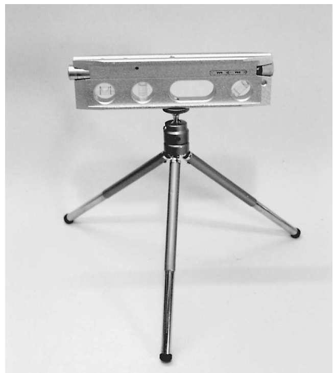
Fig. 2-8 B. A laser level on a short tripod can be used on batter boards and leveling stakes.
