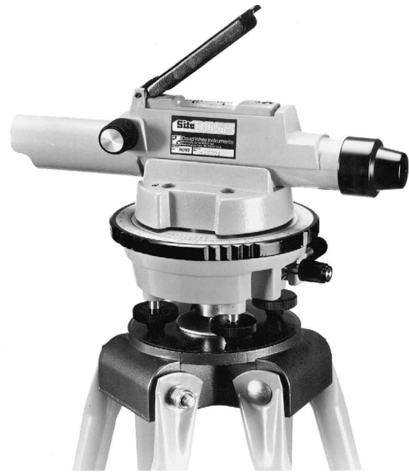
Fig. 2-19 Builder's level. (David White Instruments.)
