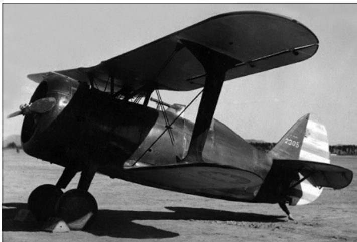
An I-15bis of the 23rd PS in 1940, little changed from the version first delivered to China three years earlier – except for the substitution of a 0.50-calibre machine gun for one of the fighter's four ShKAS weapons. On 13 September 1940, Chinese pilots like Kao, You-hsin and Hsu, Chi-hsiang flew I-15bis very similar to this one against the Japanese
