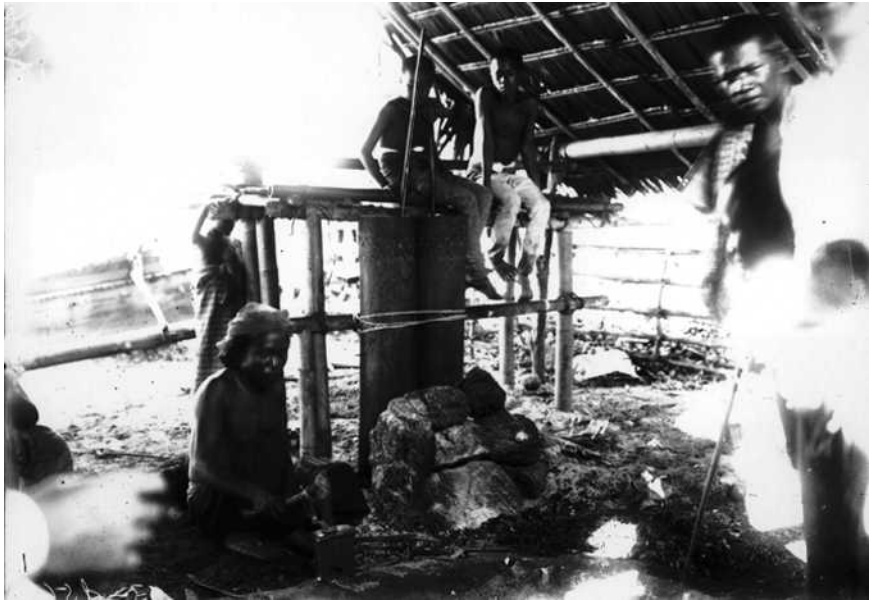
Figure 9.1. Traditional ironworking among the Tausug (Sulu) of Jolo, showing stone-lined smelting furnace and bamboo pistons, 1898. (Courtesy of Dean Worcester Photographic Collection, University of Michigan Museum of Anthropology)
