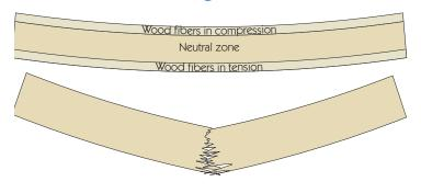
In a bending beam, the bottom-most fibers are in tension, while the top fibers are in compression.
