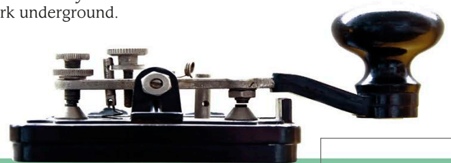
Machine for key-tapping Morse code
