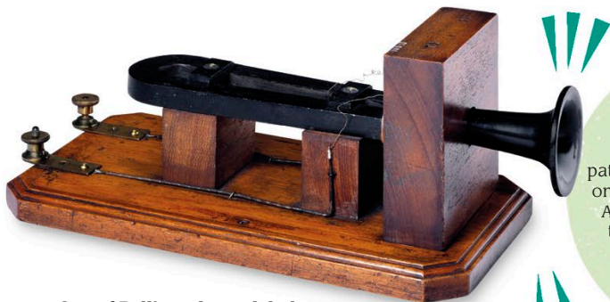
One of Bell’s early model phones, known as a box telephone, had a trumpetlike mouthpiece.
