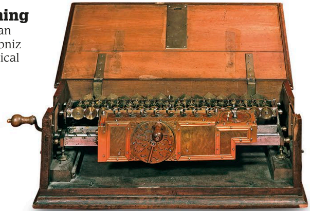
Modern replica of the Stepped Reckoner
