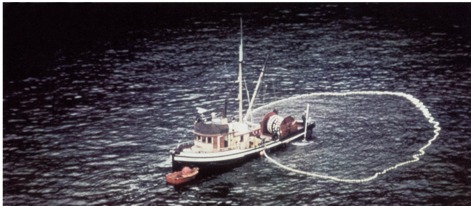
Seiner, with its tender alongside, completing a set.
