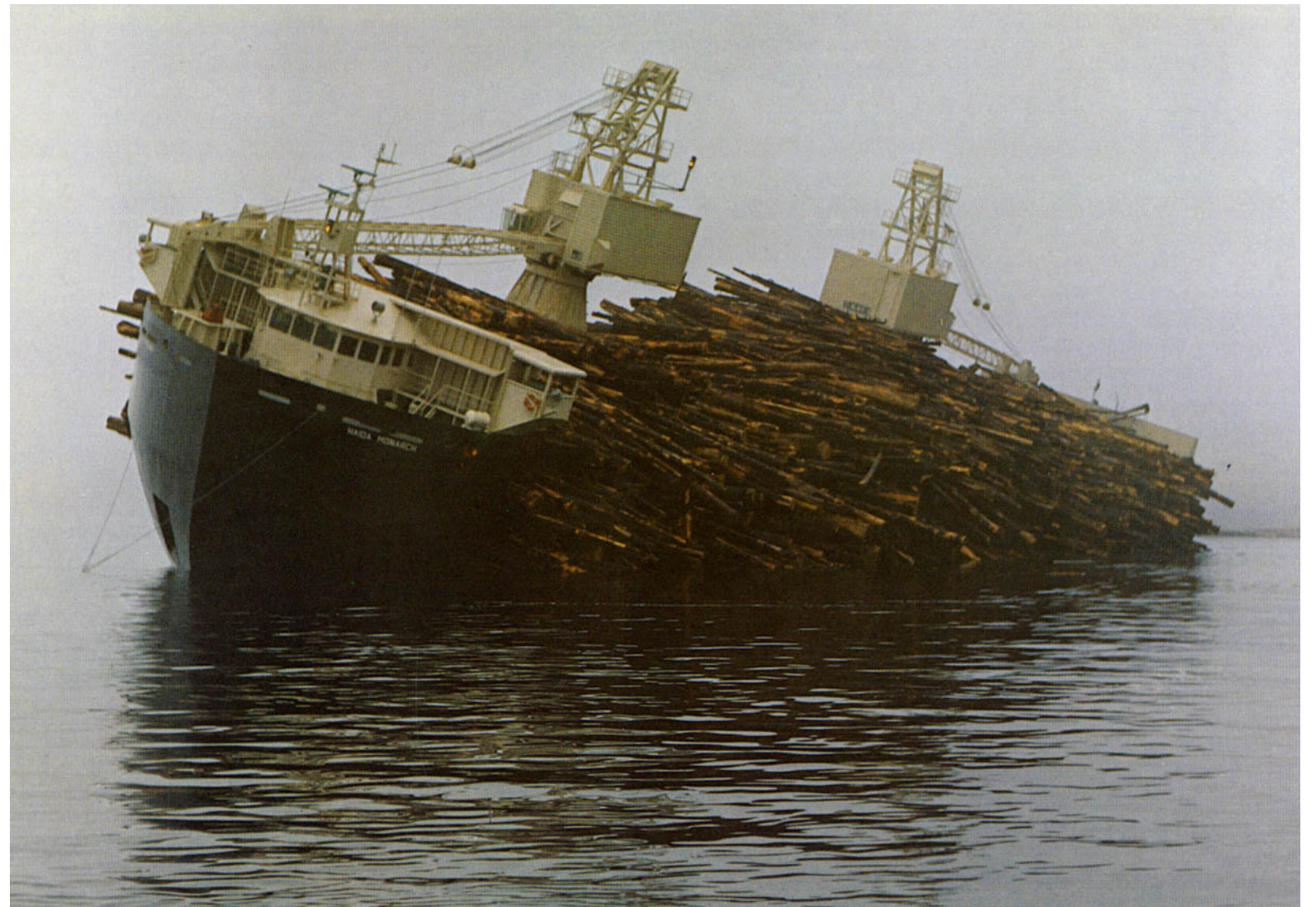
The Haida Monarch, a self-propelled, self-dumping log carrier built in North Vancouver, shown in the process of unloading.
