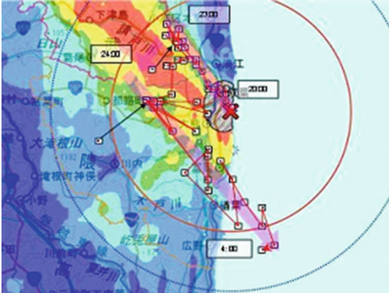
Fig. 5.9 Path of the plume released at 20:00 on March 15 (TEPCO, Fukushima Nuclear Accident Analysis Report)
