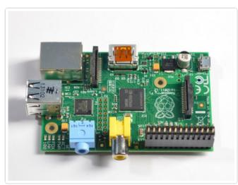
Plug the extra tall female header into the GPIO port on the Pi as shown. Make sure its seated nice and flat
