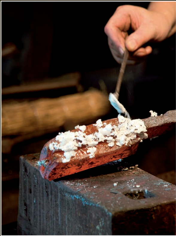
Yoshindo spreads borax over the composite bar.
