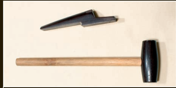
The tsuka-nuki tool and the wooden hammer or mallet used to loosen a tight hilt or tight habaki.
