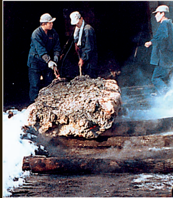
Workers remove the new kera from the tataru by rolling it out over a series of logs.
