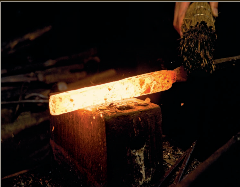
The steel bar is partially drawn out here. The end where the handle is attached will become the tang.
