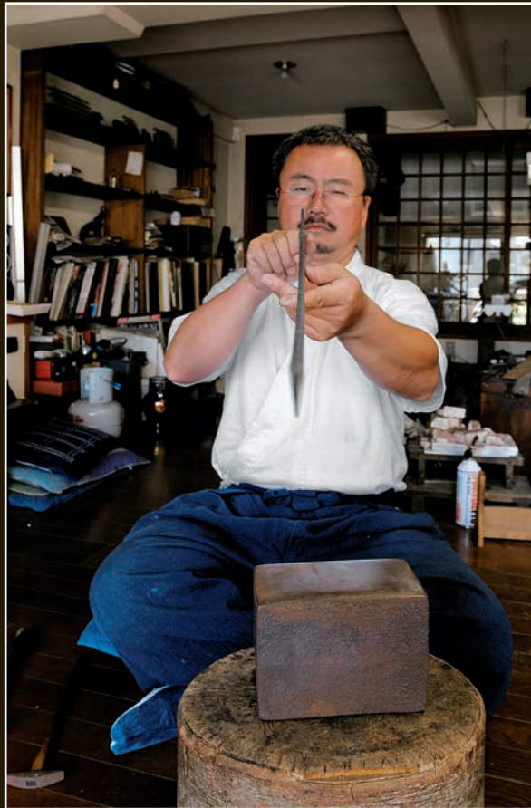
Yoshikazu checks the blade for warping and twisting.
