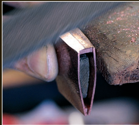
Filing the top surface. The front of the insert, which is visible in the narrow end of the habaki, will rest against the hamachi.
