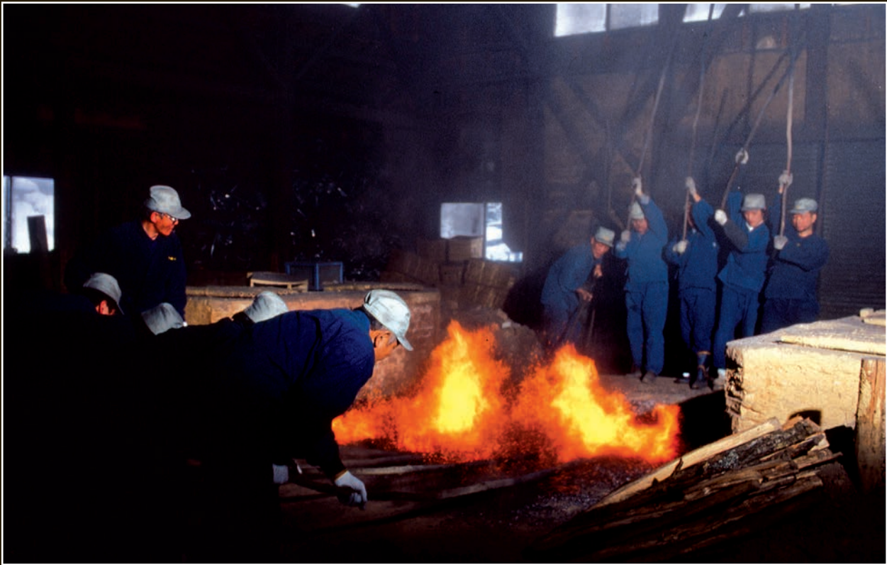
Constructing the furnace is a very important process. The success of the tataru's operation depends on the structure and design of the furnace and the clay used to make it, as well as on the murage (supervisor). Building the tataru and choosing the appropriate clay depend on the murage's knowledge and experience.
