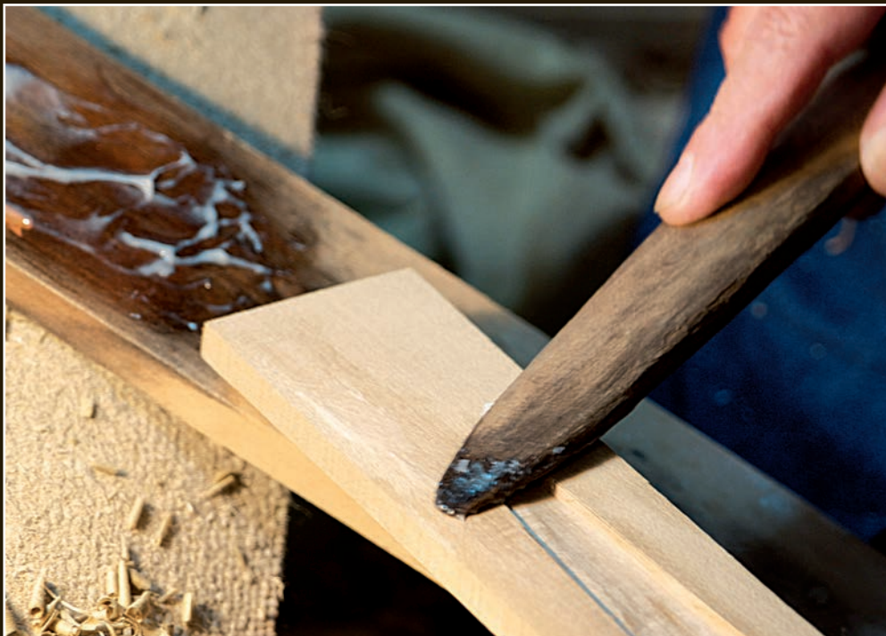
Okumura spreads sokui glue over the hilt surfaces.
