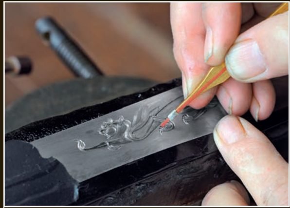
All of the inner surfaces of the horimono are polished with a fine abrasive stone.
