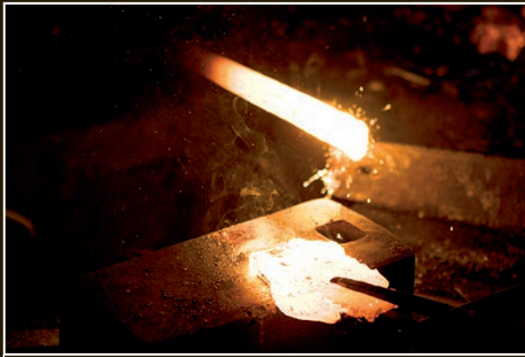
The teko and the steel plate on which the tamahagane will be stacked are heated separately.
