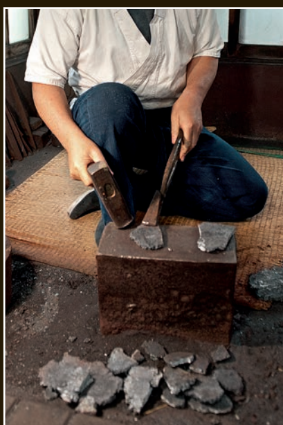
Breaking a plate of tamahagane into small pieces with a hammer.
