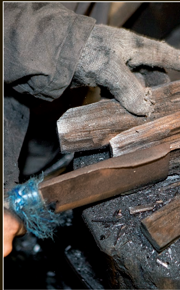
The charcoal is cut with a tool resembling a bamboo knife. Here, Yoshindo's student is preparing to cut new lengths of charcoal into smaller pieces of uniform size.
