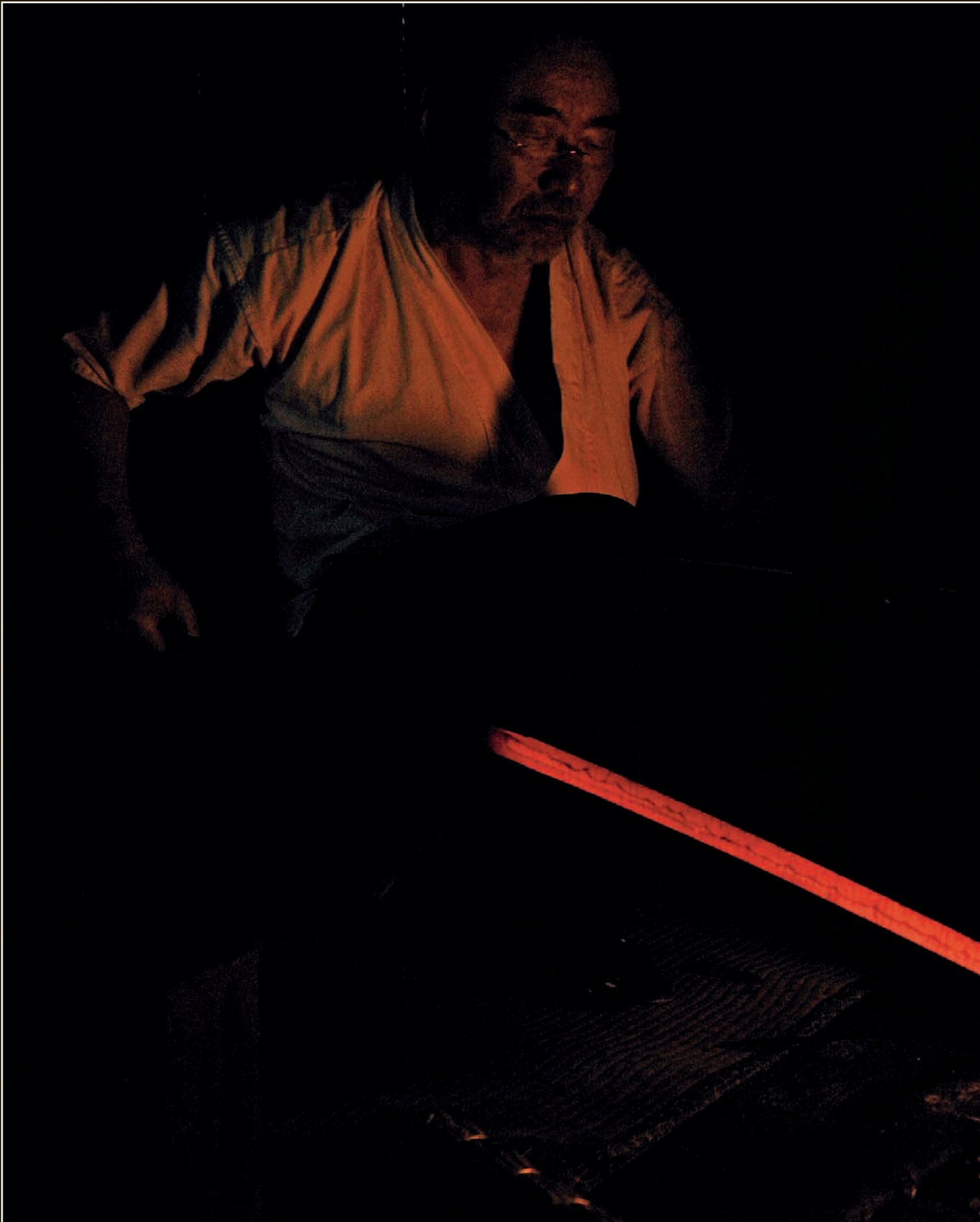
As the sword is slowly drawn through the forge, the temperature of the steel increases and the color progresses from black to red to orange to yellow.
