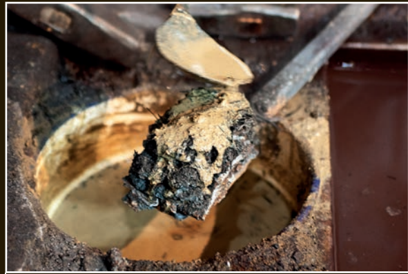
The tamahagane is covered with ashes and clay.
