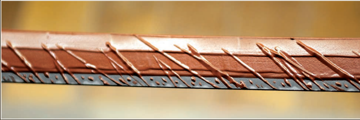
This clay pattern will produce a slanted and variable gunome wave hamon.
