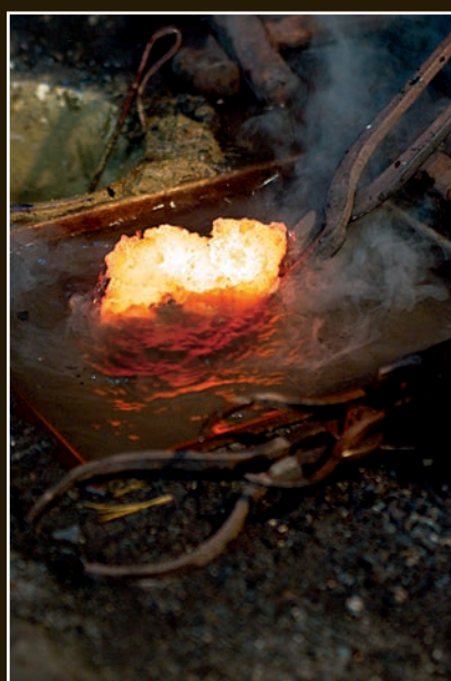
Quenching the tamahagane. A piece of tamahagane is heated and forged into a thin plate. When the plate is still a red or yellow color it is quenched in water to cool it rapidly. It is then broken up into small pieces.
