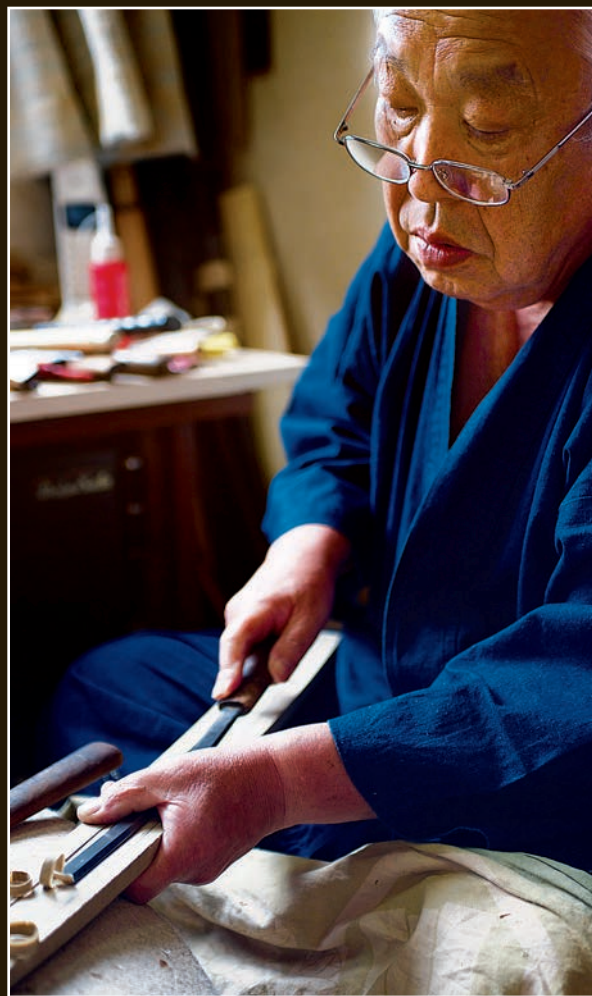
Okamura uses a saya chisel to begin carving out the space where the sword will fit.
