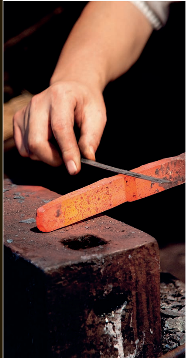
Checking the dimensions of the steel where the tang is being formed.
