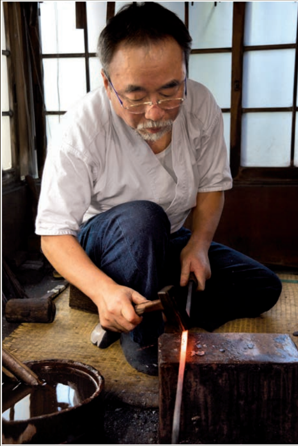
The hammer and anvil are constantly wetted during the forging process.
