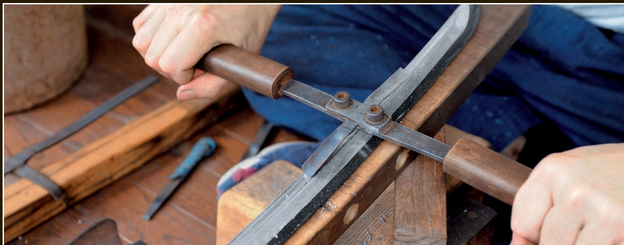
Mizuki begins to cut the groove with a sen (drawknife). He starts in the center of the marked area and slowly widens and deepens the groove. Several different types of sen are used during this process. The edge of the blade and the point are covered with electrical tape to protect them.
