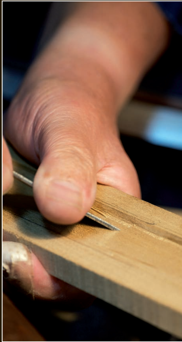
Okumura shaves the inside of the saya to obtain a very smooth surface.
