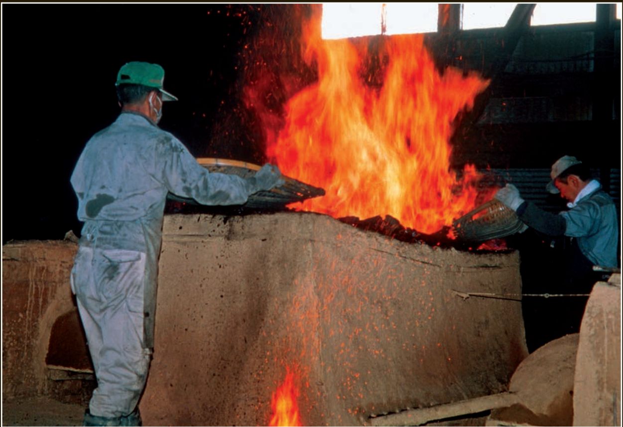
When the tatar is in operation, it is periodically filled to the top with fresh charcoal, and new iron sand is spread over the top. The workers here are adding iron sand.
