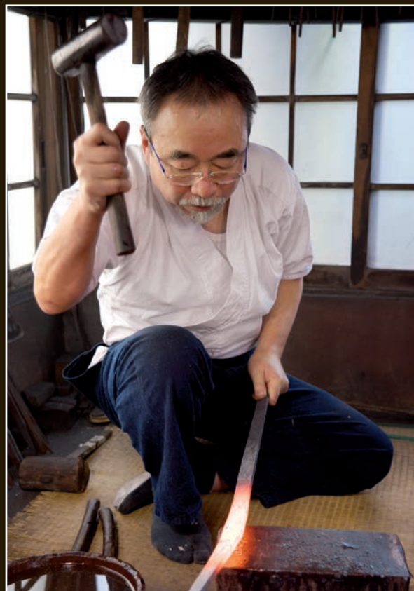
The sunobe expands where Yoshindo is forming the cutting edge. The bulge in the sunobe just above the tang is the beginning of the new edge.
