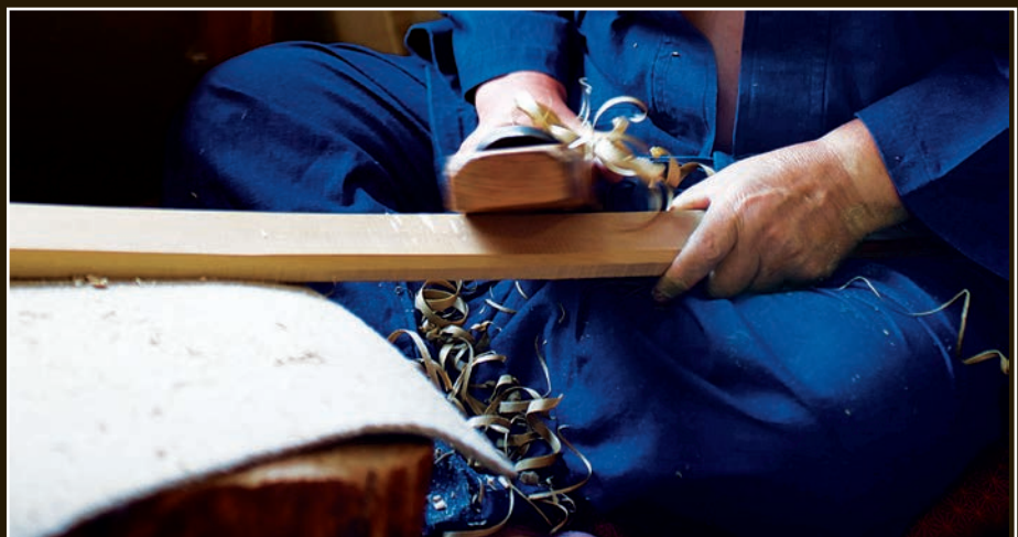
All of the inside and outside surfaces of the wood are smoothed with a plane.
