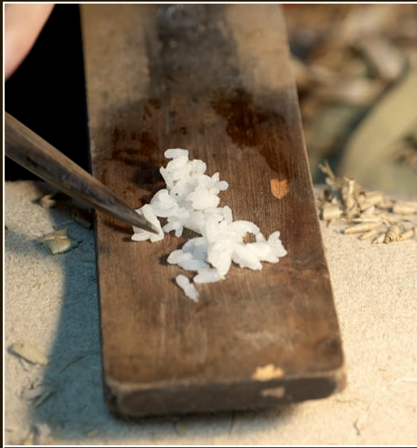
Cooked rice is used to make the sokui glue that holds the two halves of the saya together.
