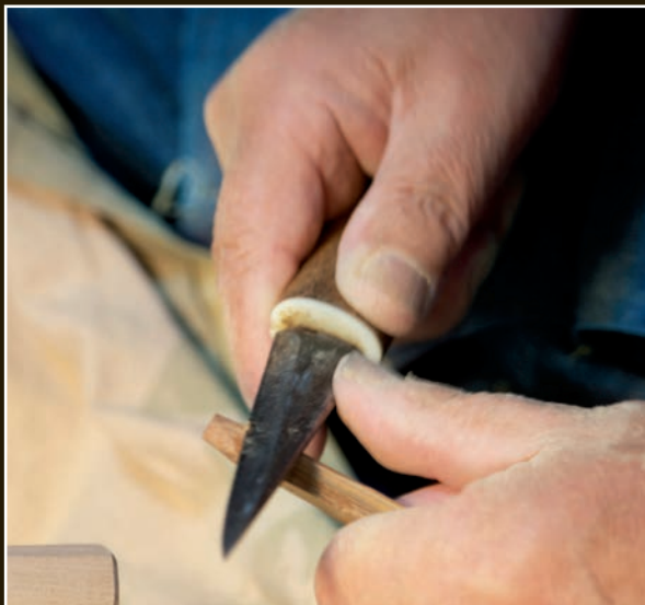
Using a kiridashi knife, Okumura begins to shape a mekugi (bamboo rivet).
