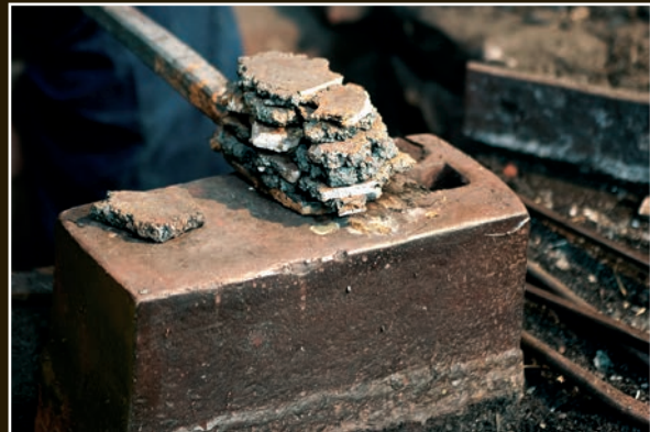
The tamahagane is stacked and ready for forging.
