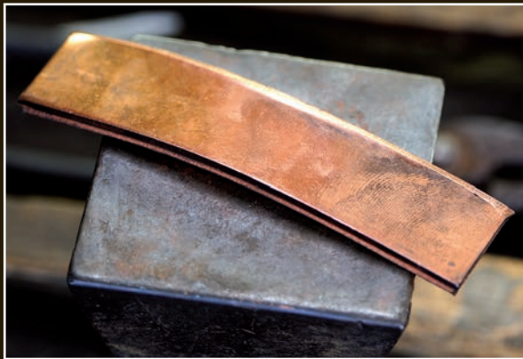
Metal for making the habaki is cut from a stock sheet.
