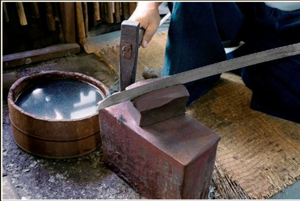
A large copper block with a deep groove is prepared. The groove must be large enough to accommodate the back surface of the sword.
