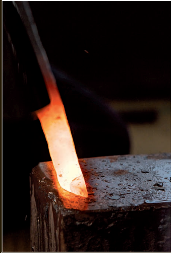
Forging has progressed to the point area, which is now being delineated.
