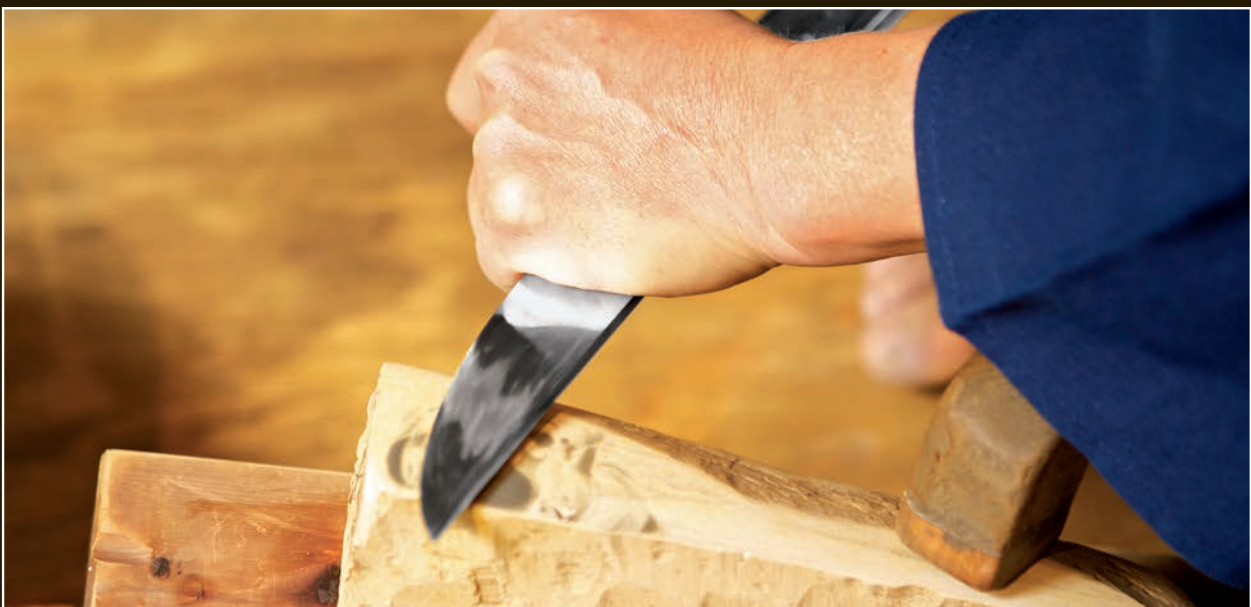
Takaiwa grips the bare blade with his left hand. Although his hand is wrapped around the sharp edge, there is no contact between the edge and his skin.
