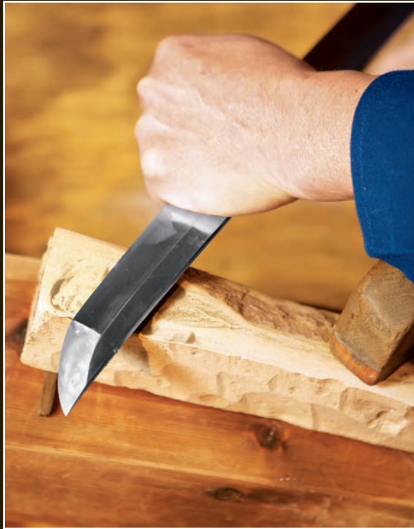
Polishing the body of the sword below the point. The contrast between the point and body of the sword is now much more evident.
