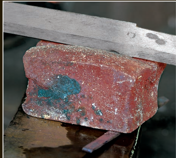
The back of the sword is placed on the hot copper block. The small area where the steel heats up is turning black.
