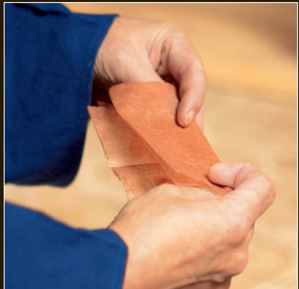
Takaiwa folds a washi sheet into eight layers. He will use this to filter the nugui before applying it to the sword.
