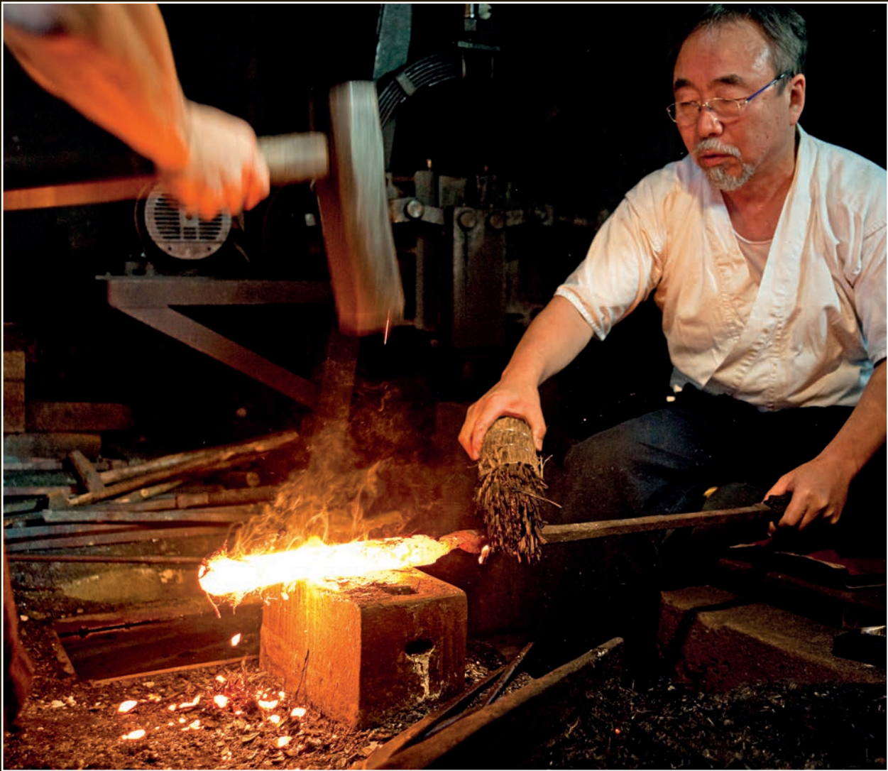
The bar is forged to draw out the steel and to unify the inner and outer components. Here it is becoming noticeably longer.
