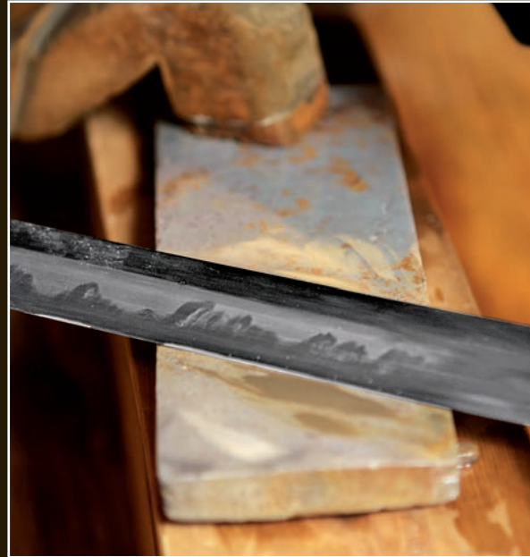
Here the suita stone, the first of the uchigumori stones, is being used. The outline of the hamon is clear, and the hamon is beginning to stand out distinctly from the body of the sword.
