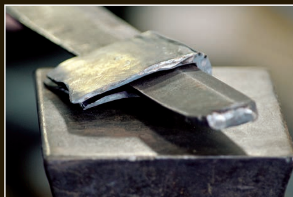
After the habaki has been folded into a U shape, it is forged around the mune surface of the tang. The inside of the habaki must conform very closely to the shape of the tang.
