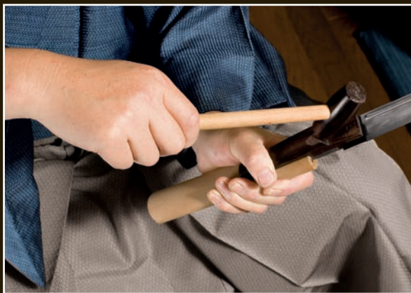
Yoshindo has tapped the tsuka-nuki with the hammer, moving the tang partly out of the hilt. It can now be grasped and removed from the hilt completely.
