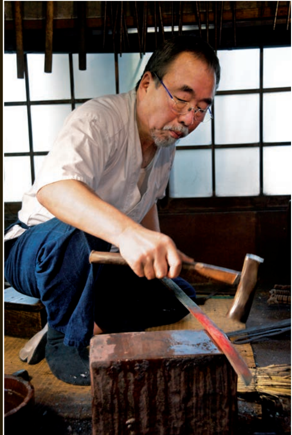
Yoshindo continues to refine the shape of the sword by additional forging. Here he is working his way back from the point to the tang.
