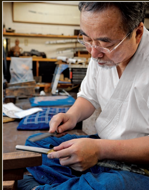
Using a finer file to make the yasurime (decorative file marks) on the tang. Yoshindo uses a copper guide, visible under his left thumb and forefinger, to produce very regular, uniform, parallel file marks.
