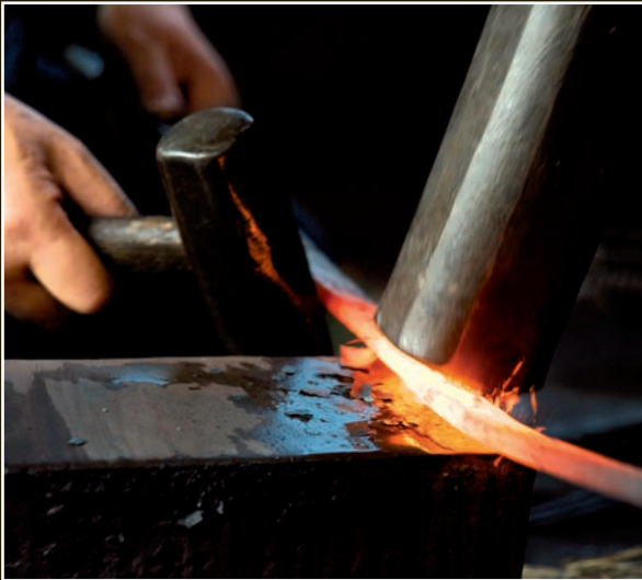
Forging close to the point area. Yoshindo positions the sword while his assistant hits it with a sledgehammer.
