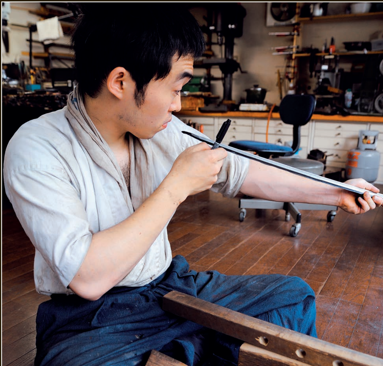
The grooves must be inspected frequently while they are being worked on to ensure that the insides are smooth, straight, and uniform in depth along their entire length.
