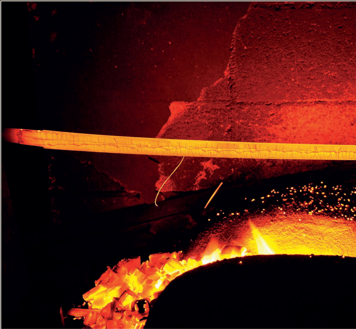
Yoshindo has let the fire in the forge die down so he can see the color of the sword as clearly as possible. The blade should be an even color before quenching, with the edge noticeably brighter than the rest of the sword.
