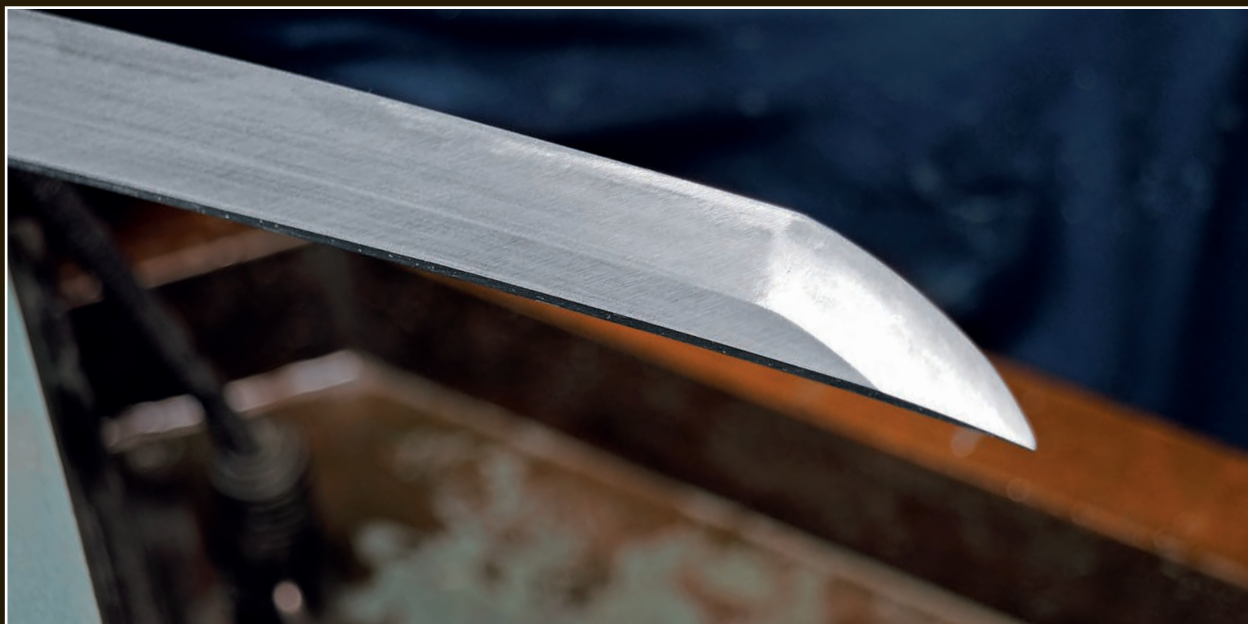
The sword has been polished with a 240-grit polishing stone.
