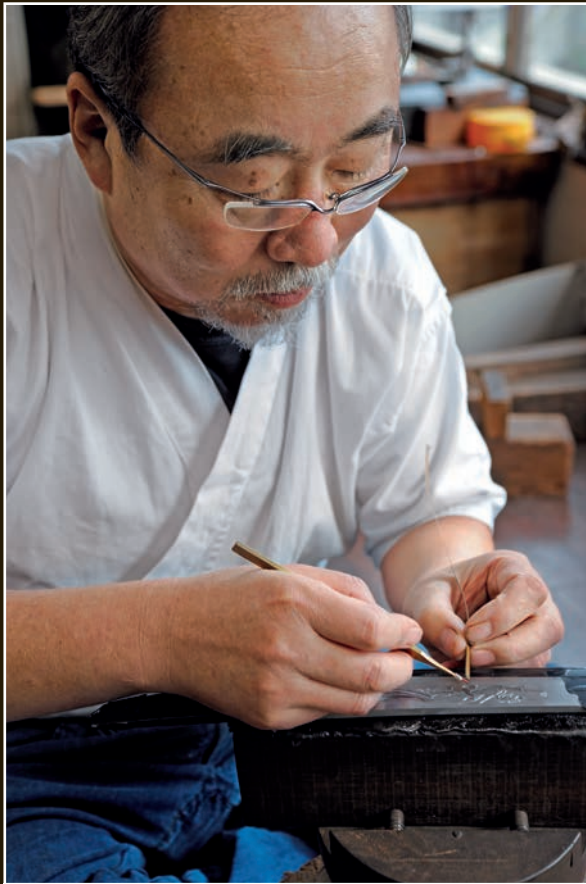
The inner surface is sanded to a fine finish. The horimono will have high relief and a very smooth three-dimensional surface.
