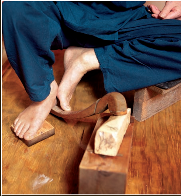
Takaiwa is seated in his working position. His right foot rests on a wooden block, with his right heel holding the fumaegi in position. His left leg is supported by the stool, with the left toes resting on the fumaegi.
