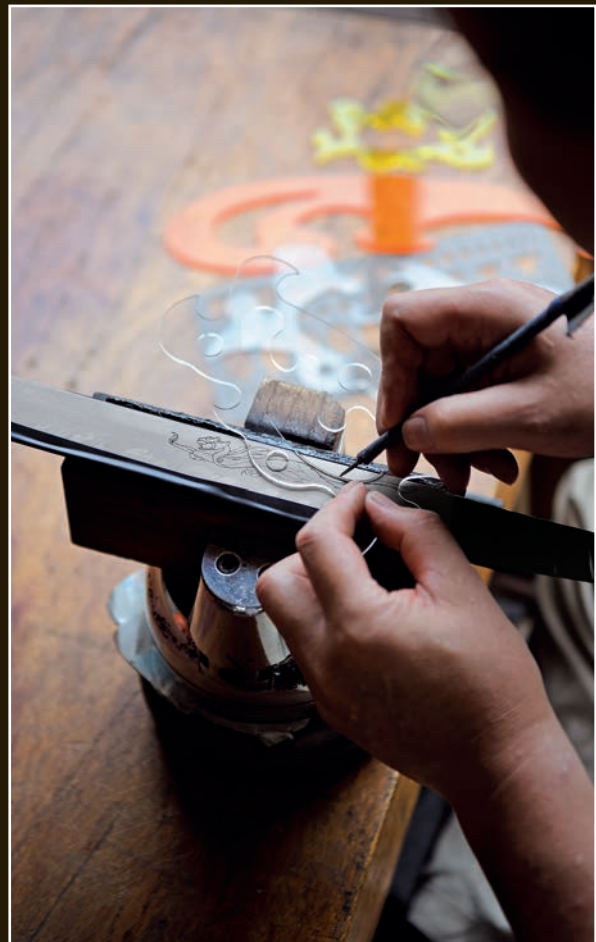
A French curve template is used to give the tiger its shape.
