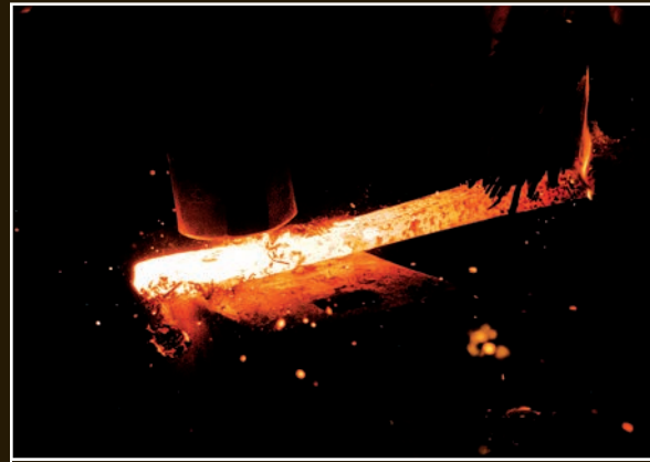
The steel is being forged to draw it out. The assistant's hammer and the straw bundle held by Yoshindo are visible.
