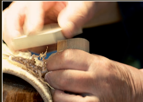
Shaping the hilt with a tokusa sanding block. The top of the hilt now has a rounded surface.
