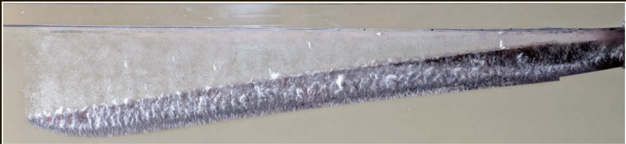
The blade 0.7 seconds after entering the water. It has now curved downward, giving the edge a concave contour. There are bubbles all over the sides of the blade, including many large ones.
