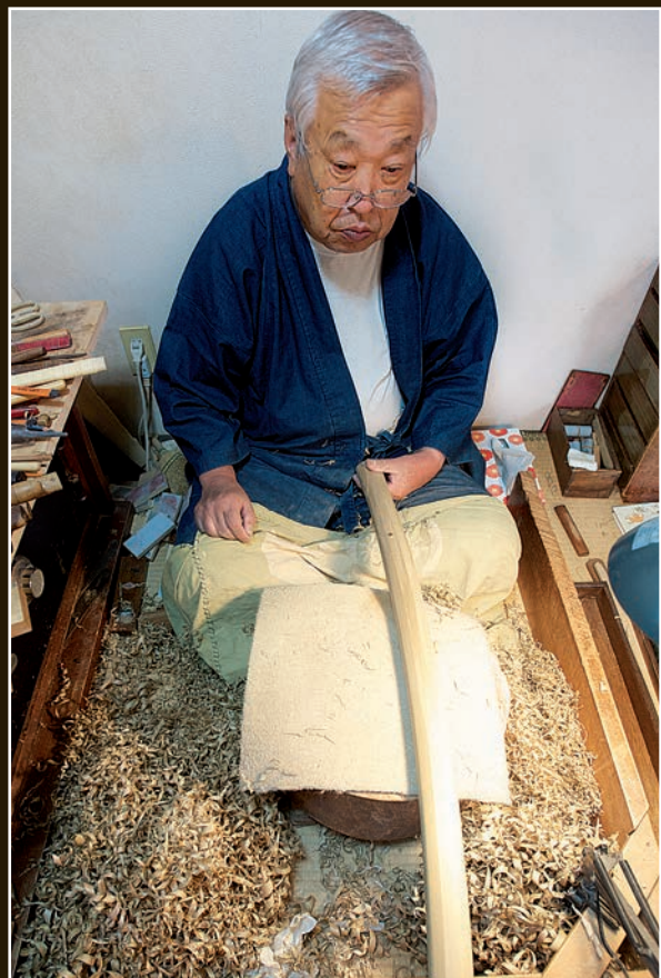
Okumura examines the finished shirasaya. Since ho wood is rather soft, he keeps his working surfaces covered with heavy cloth to protect the saya.
