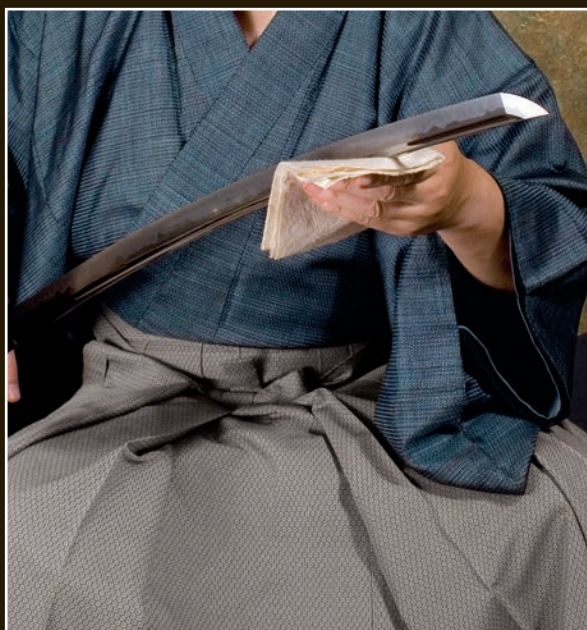
The polished blade of the sword should always be protected from direct contact with bare skin. Here, Yoshindo rests the blade on a clean sheet of paper. The tang of the sword may be held in the bare hand.
