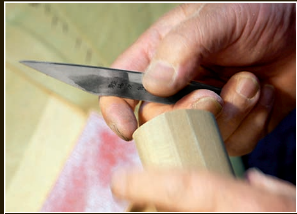
Fine bevels are made around the top and bottom surfaces.
