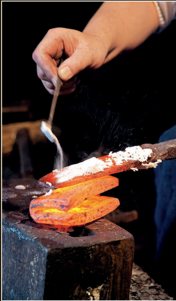
Borax, which serves as a flux, is spread over the surfaces to be welded together.
