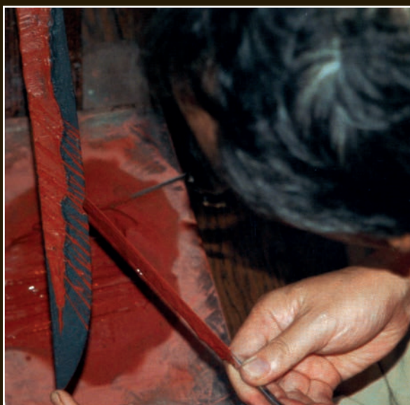
Yoshindo applies a two-component clay coating to a new sword to form the hamon. The pattern of the clay can be very detailed; it is the experience and skill of the swordsmith that will determine what the resulting hamon will look like.
