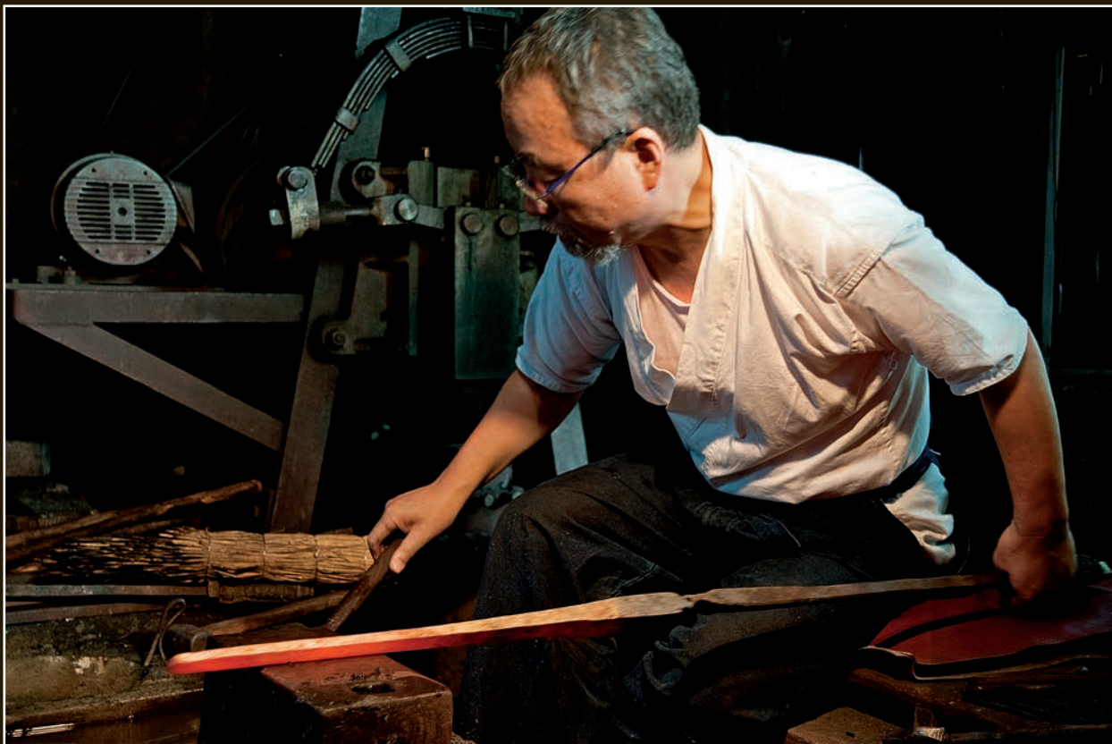
Yoshindo checks the dimensions of the steel bar, which has become much longer.
