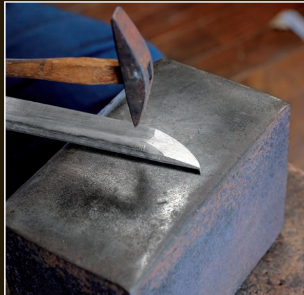
A hammer with a narrow face is used to expand the shinogi-ji and straighten the blade around the point area. This allows corrections to be made in very small areas. The black areas show where curvature was added to the blade.
