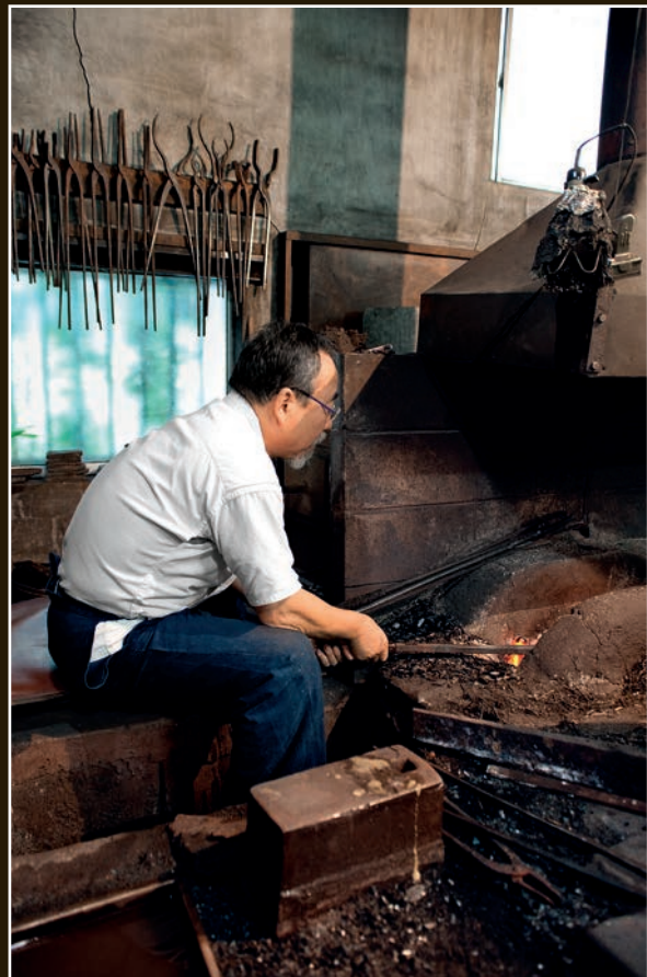
Yoshindo places the tamahagane in the forge. He will carefully pile up charcoal around the steel and heat the forge.
