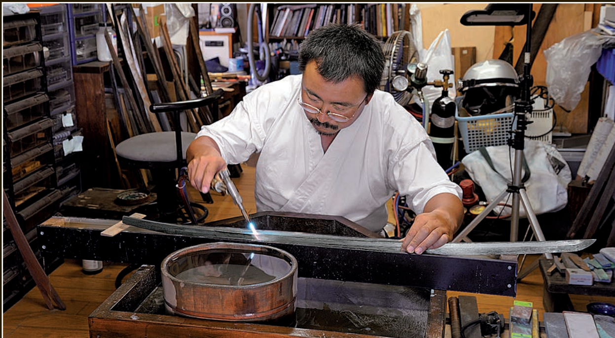
The mune is heated with a gas torch in areas where curvature is required. Water is kept close at hand to cool the blade.
