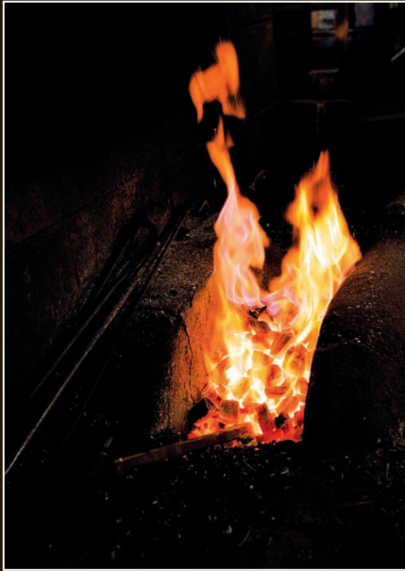
The tamahagane is covered with charcoal and the forge is heated.
