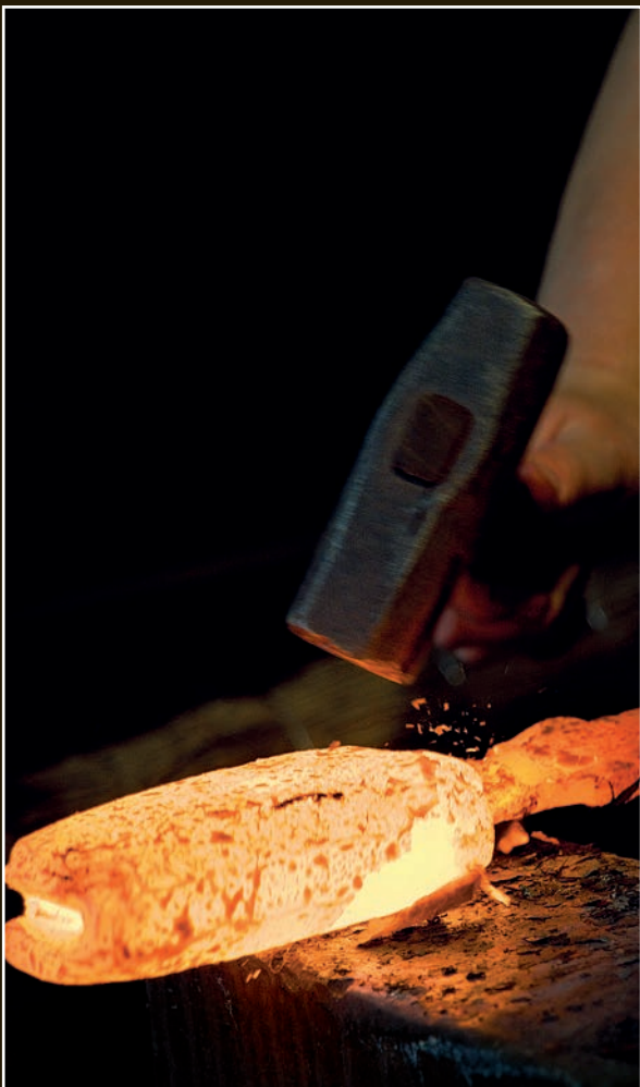
The bar is welded into a single composite structure.
