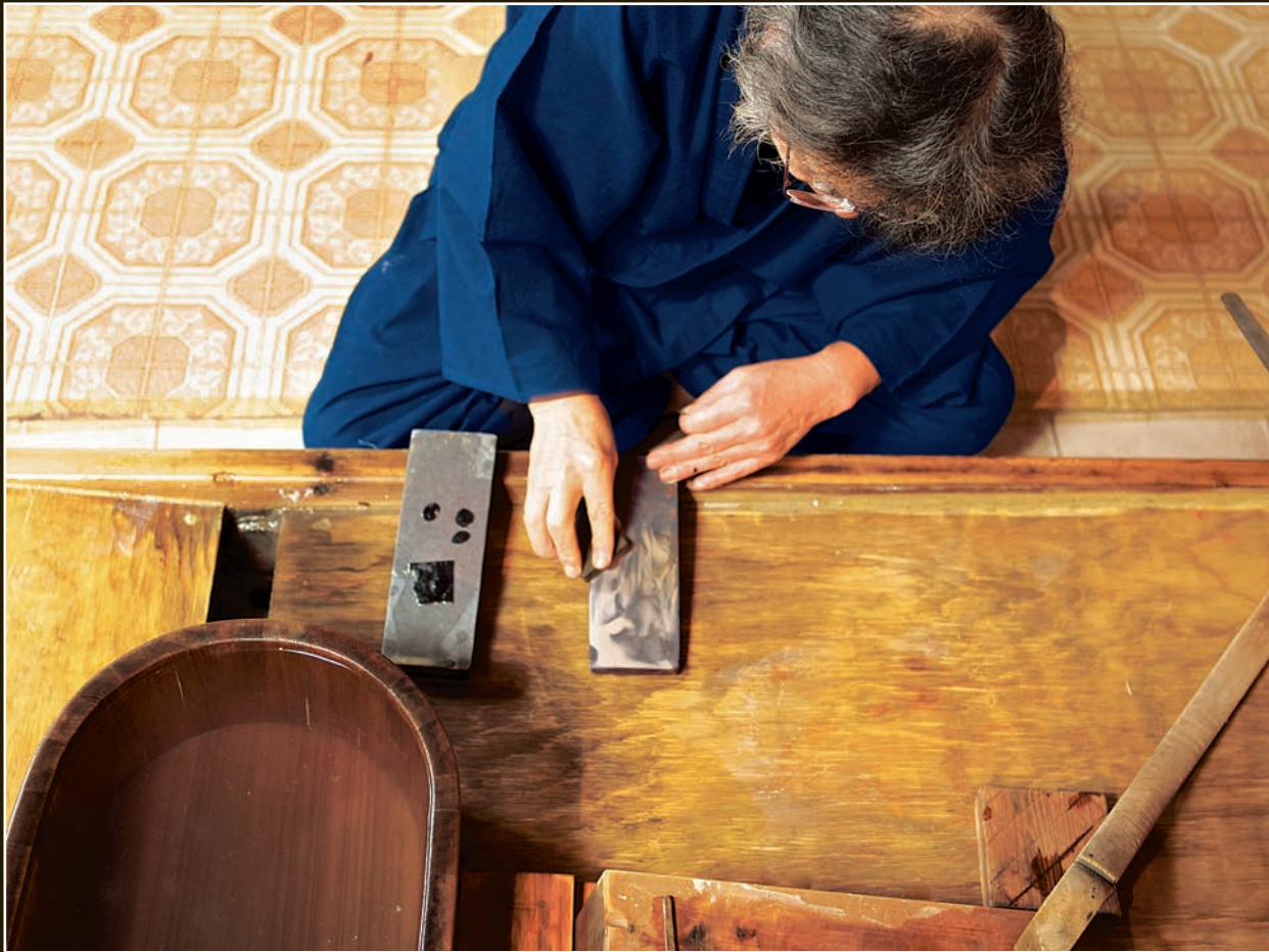
Takaiwa rubs a piece of uchigumori over a wet uchigumori stone to make a paste called "tojiru." This will be used as a lubricant between the hadori and the sword's surface while Takaiwa is polishing the hamon.
