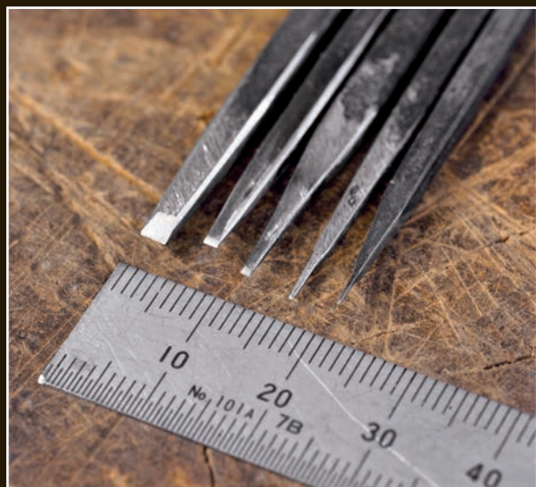
More chisels used for horimono. These have relatively large tips.
