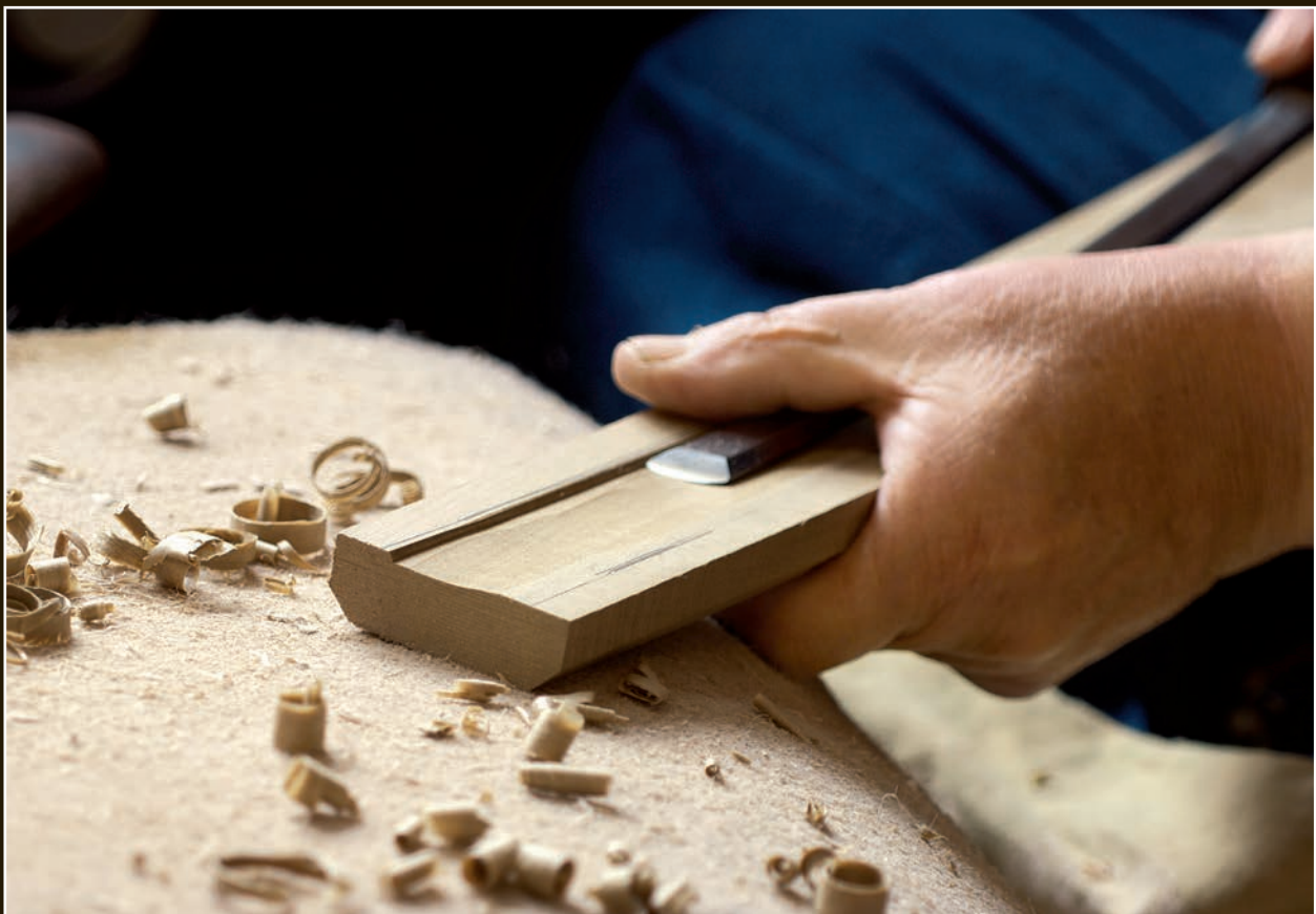
The space inside of the saya is deepest on the mune side, where the sword is thickest, and thinnest at the edge side. Okumura carves out the interior slowly, moving from the mune side. Here, he has not yet begun carving the area of the saya where the edge will rest.
