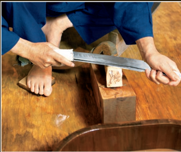
The back surface (mune) is being polished here. Takaiwa will polish one side of the mune along its full length before moving on to the other side.
