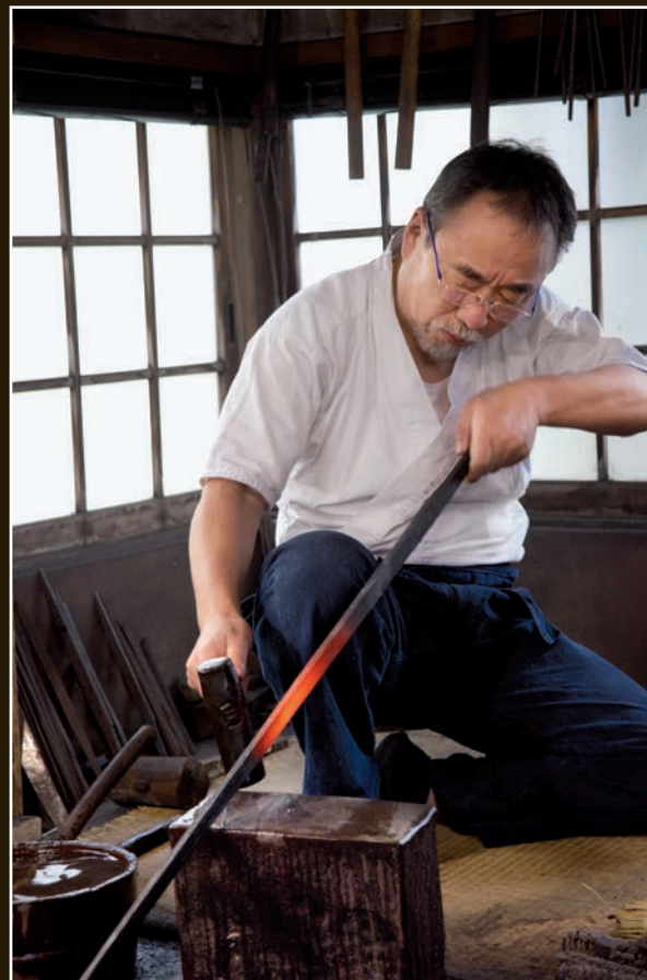
Yoshindo checks the lines of the sunobe.
