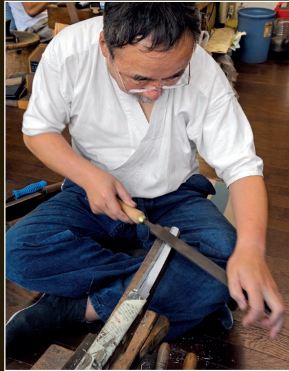
Using a rough file to finish the tang.
