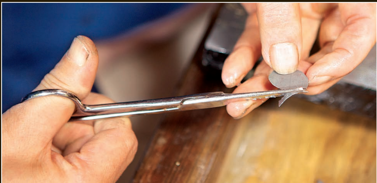
The pieces of hazuya are cut into ovals to make the hadori. The exact size and shape are determined by the size and shape of the hamon to be polished.
