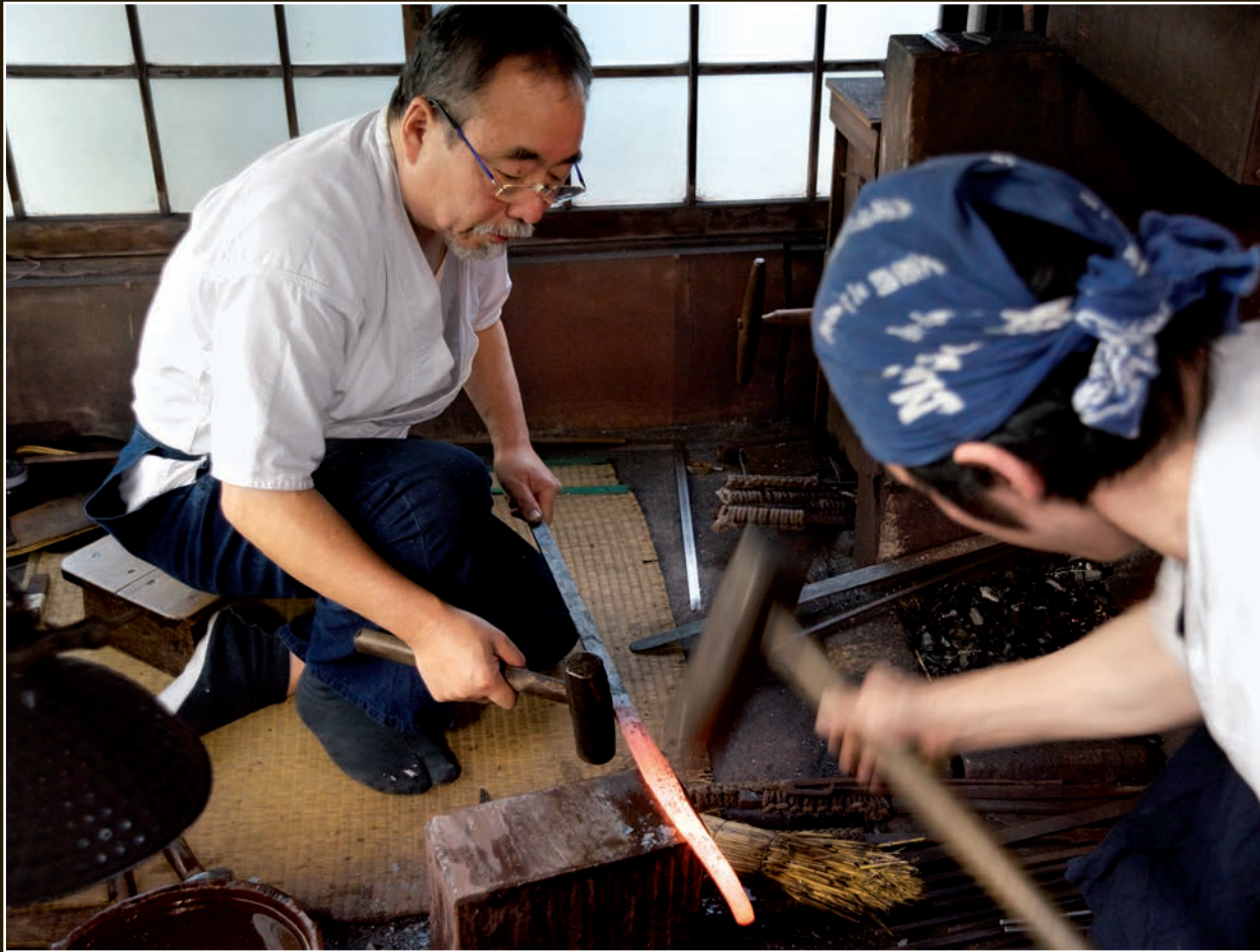
Sometimes Yoshindo's assistant uses a sledgehammer to help with the shaping.
