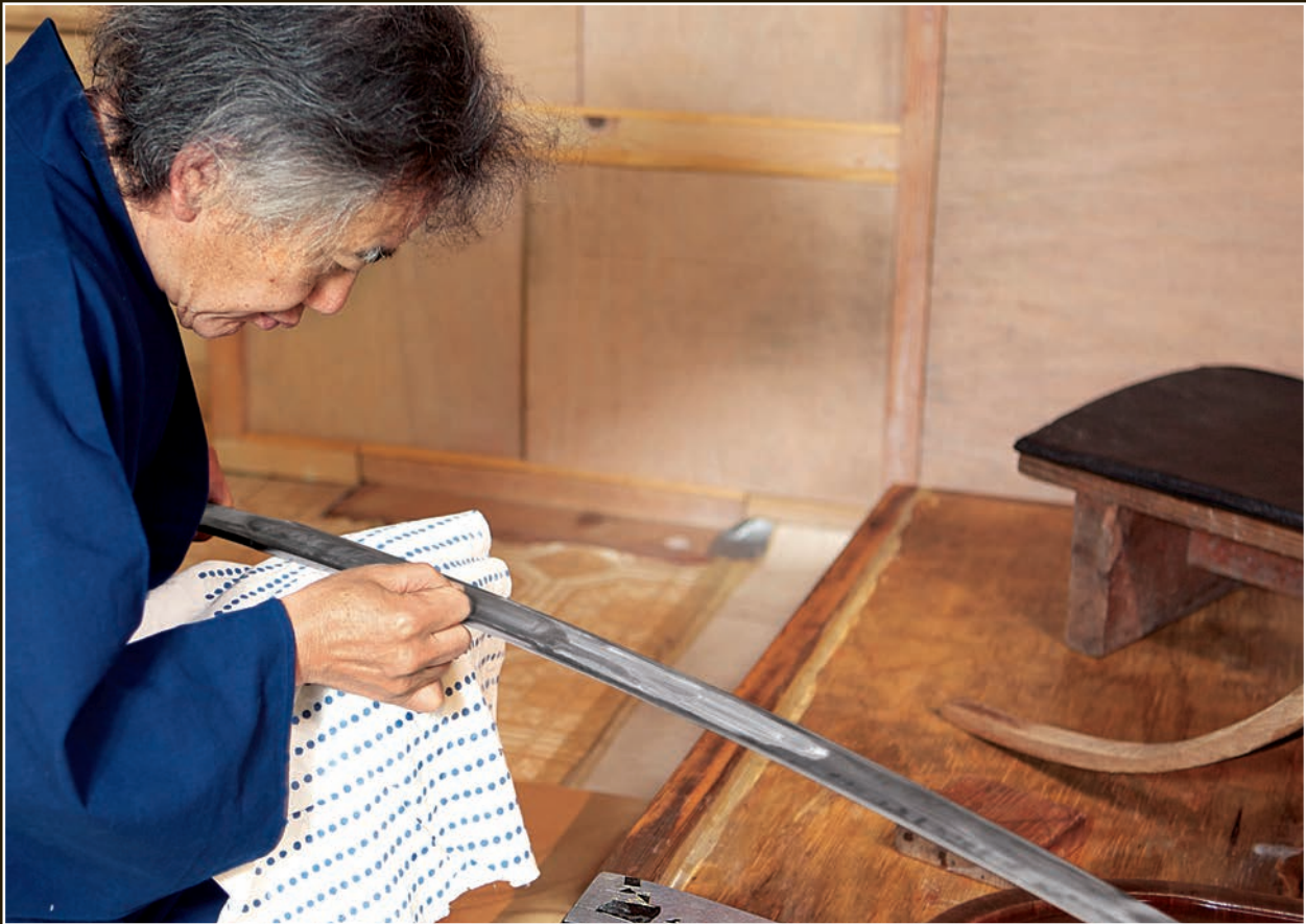
Takaiwa will go over the hamon and edge of the entire blade with the hazuya. The stone wears out and dissolves during this process; the white paste on the sword is residue left from the stone.
