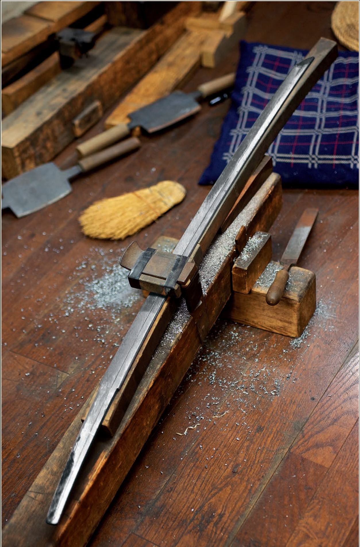
The sword is clamped between two pieces of wood to hold it in position while it is shaped with the sen and file.
