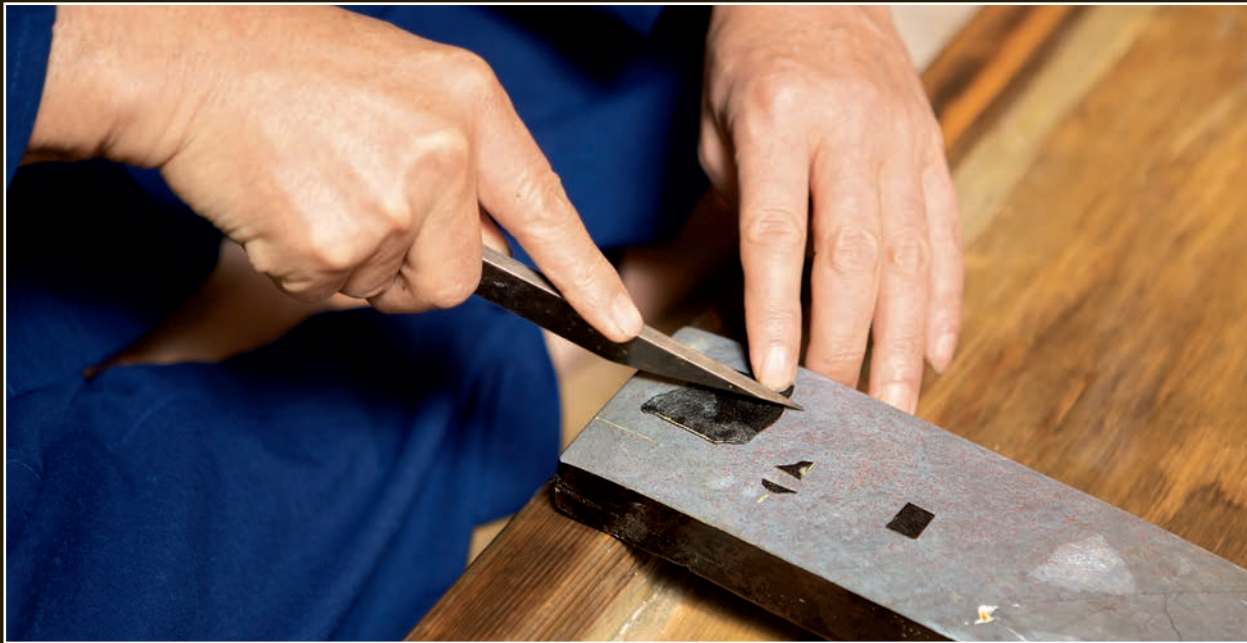
Takaiwa is cutting the hazuya stones into small squares for convenient use. The back side, covered with the lacquer and washi paper, is facing up.
