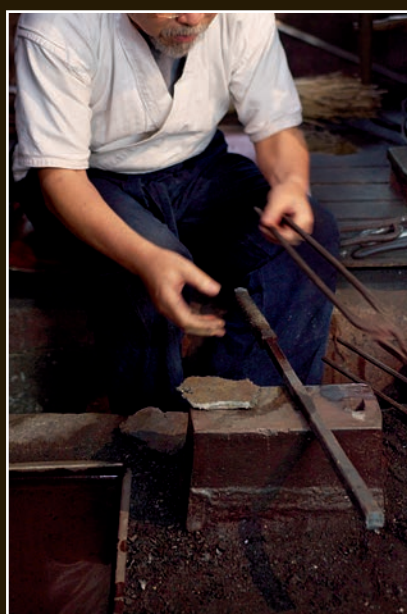
Preparing the teko (steel handle) and the tamahagane plate that it will be welded to.
