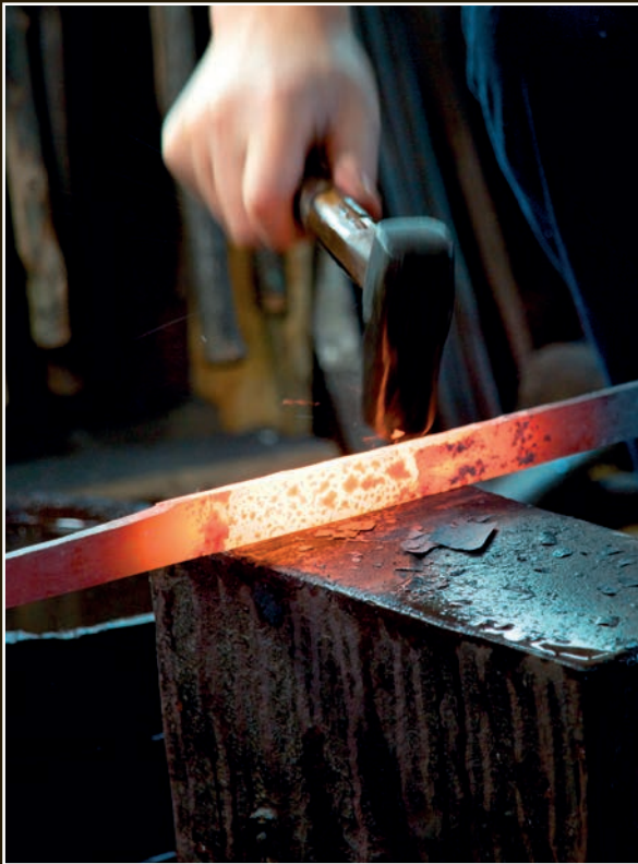
Yoshindo works on the end nearest to the tang. He is forming the iori mune, the roof-like shape along the back surface of the sword.
