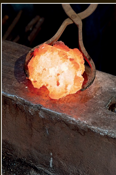
Quenching the tamahagane. A piece of tamahagane is heated and forged into a thin plate. When the plate is still a red or yellow color it is quenched in water to cool it rapidly. It is then broken up into small pieces.
