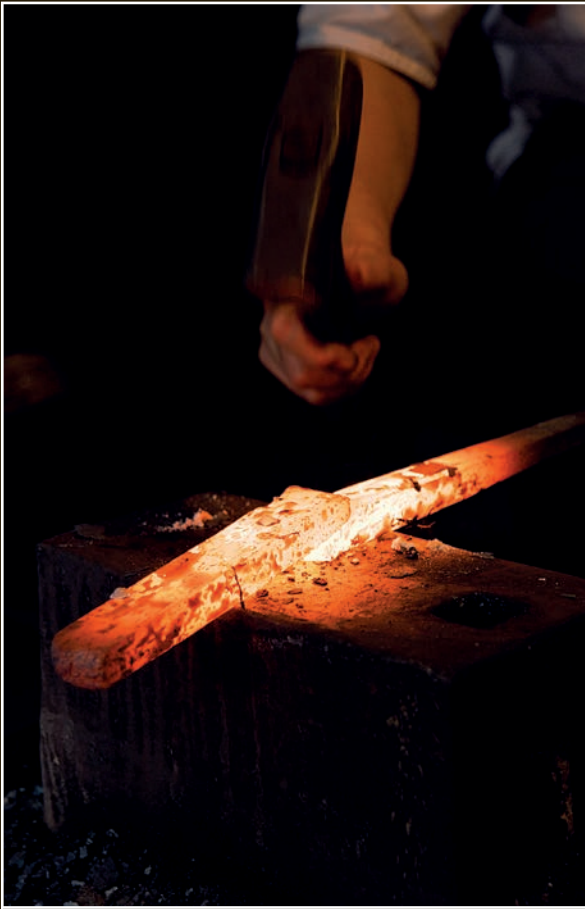
The shingane steel bar is welded onto a handle.
