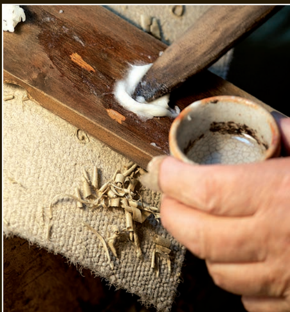
Water is added a drop at a time until the sokui has the proper consistency.
