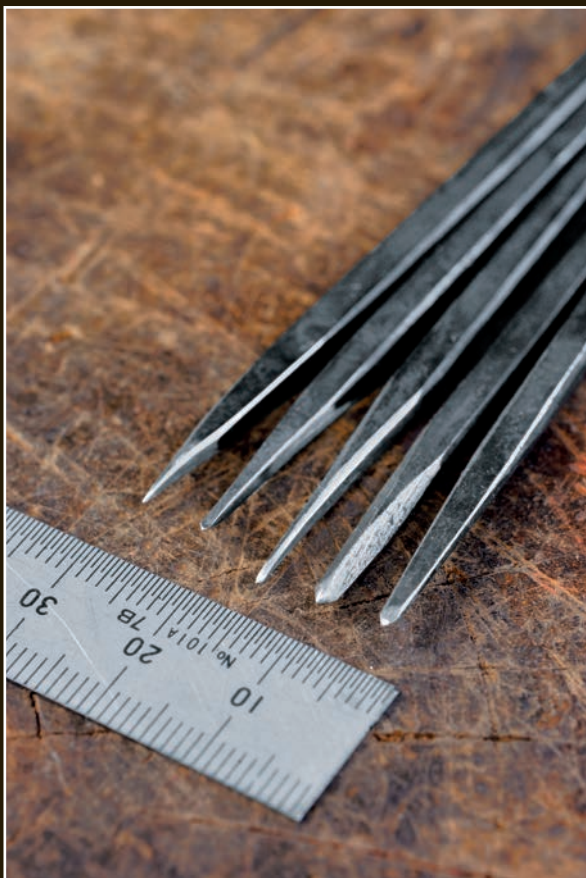
Some of the chisels used for engraving work. There are a number of different sizes, with differently shaped points; these have very fine points.
