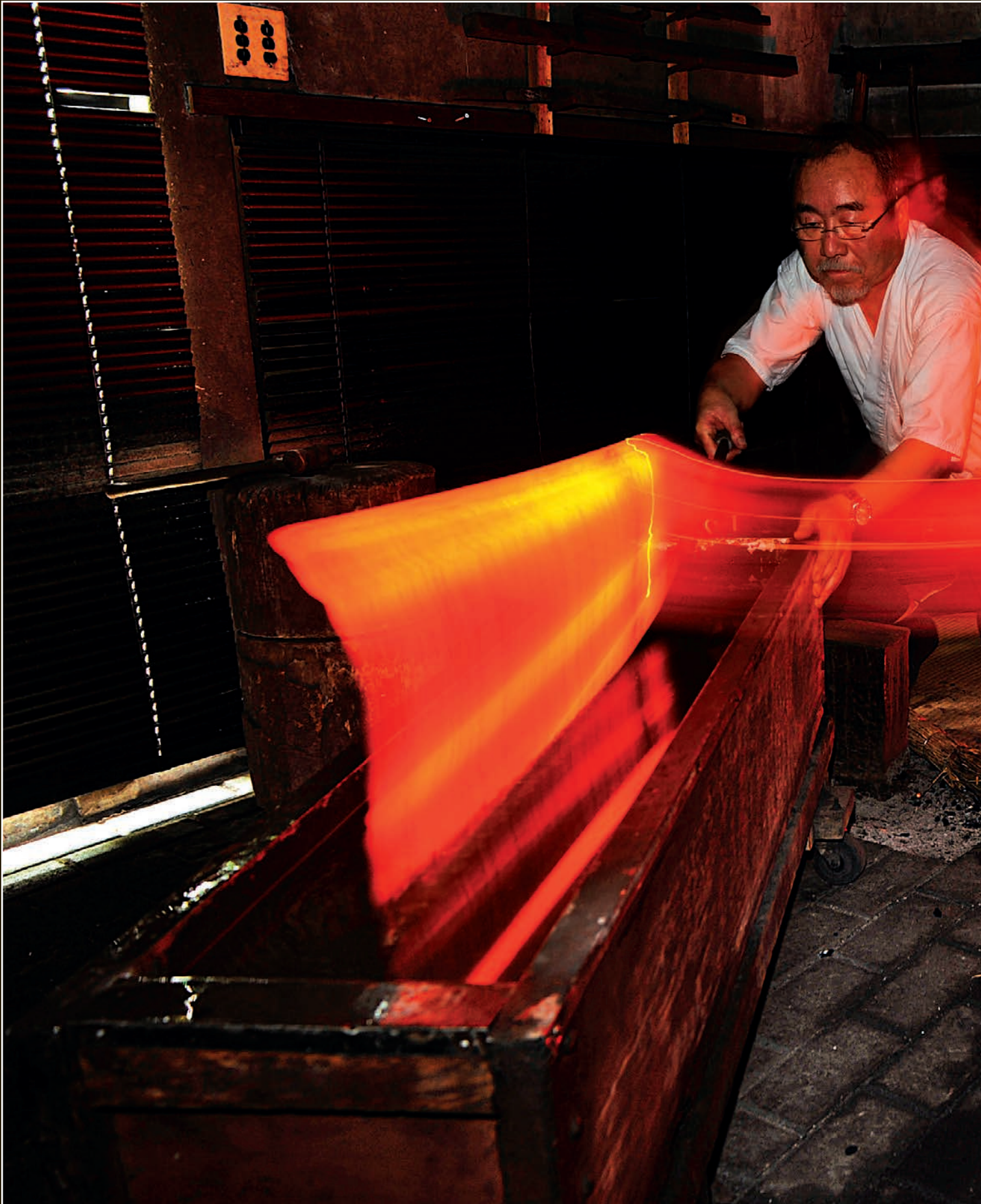
When the sword reaches the crucial temperature, Yoshindo has only a few seconds to be sure that it is evenly heated along its entire length and that it is the proper color. When it is ready, it is rapidly moved parallel to the ground and plunged into a tank of water to cool it. If everything has gone well, the sword will now have a hamon.
