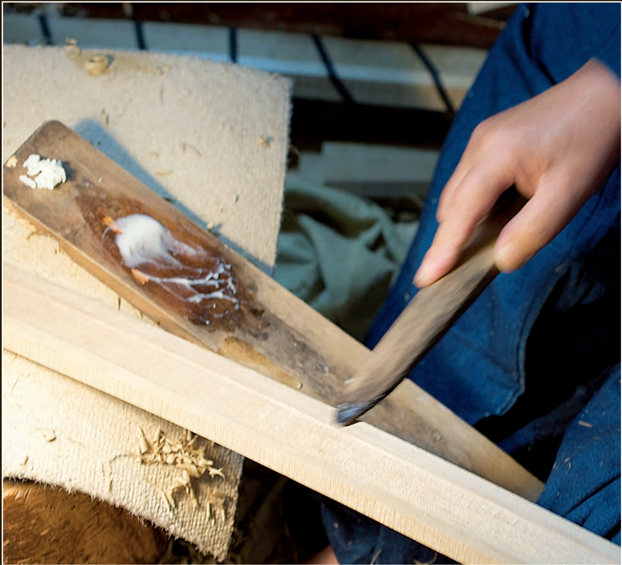
A bamboo spatula is used to spread the sokui glue over the surfaces that are to be glued together.
