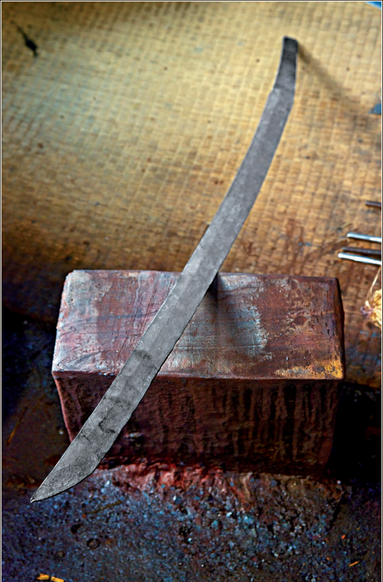
The shaping of the composite steel bar into a blade is now complete.
