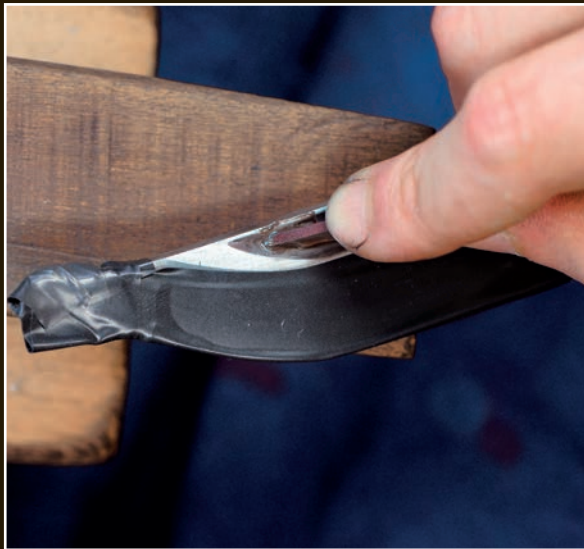
The insides of the groove ends are cleaned again with a fine stone. Kerosene is used to lubricate the grooves while working with the stone.
