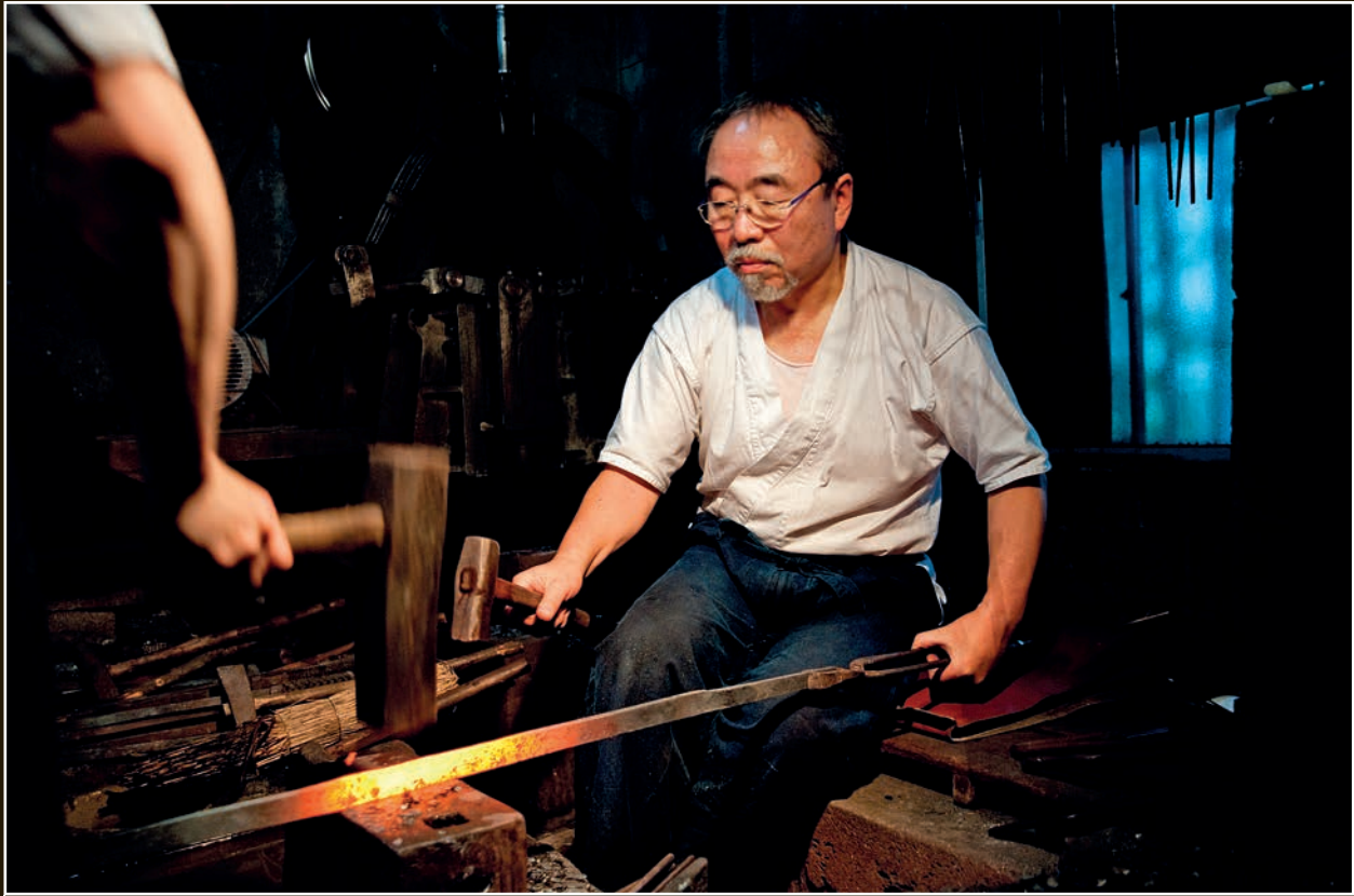
Yoshindo uses a pair of tongs to grip the tang while his assistant hammers the steel. They are working to draw out the steel to the desired length.
