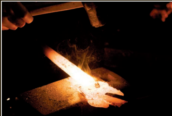
Hammering the teko and steel plate while they are heated.
