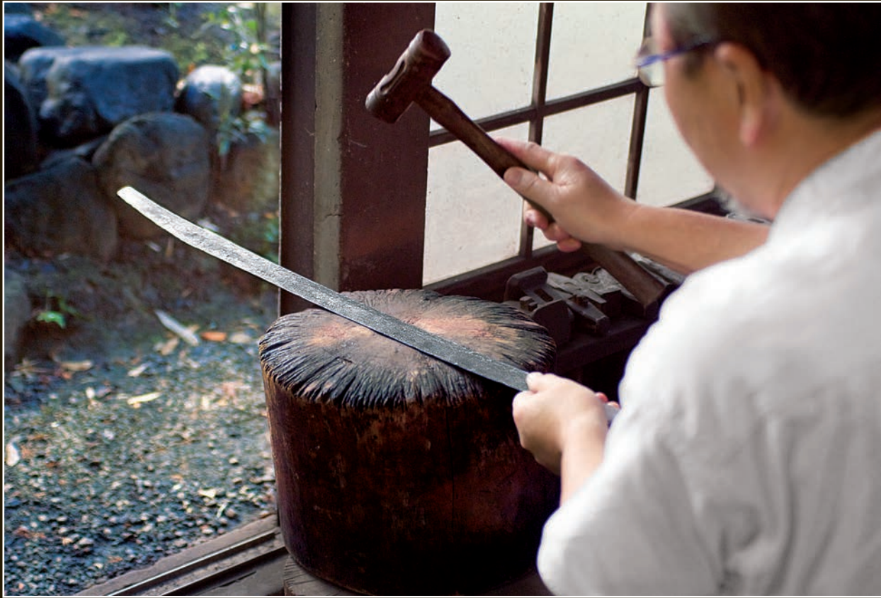
Yoshindo straightens the blade by hammering it on a wooden anvil.
