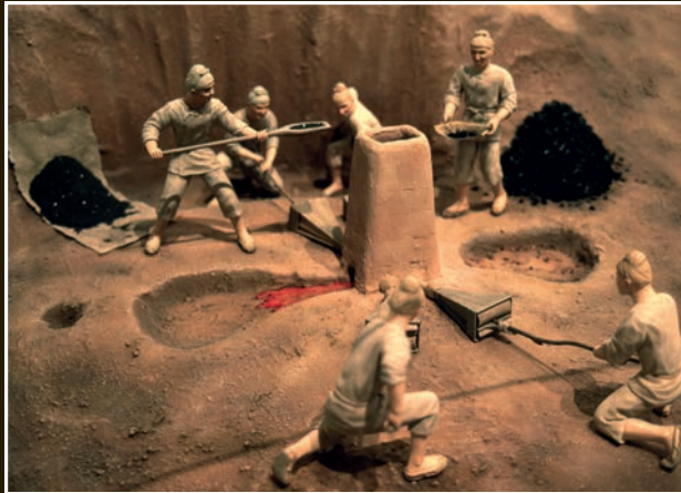
A model of an early tatara operating in the open at the base of a slope. The size is small compared to Edo-period tatara.
