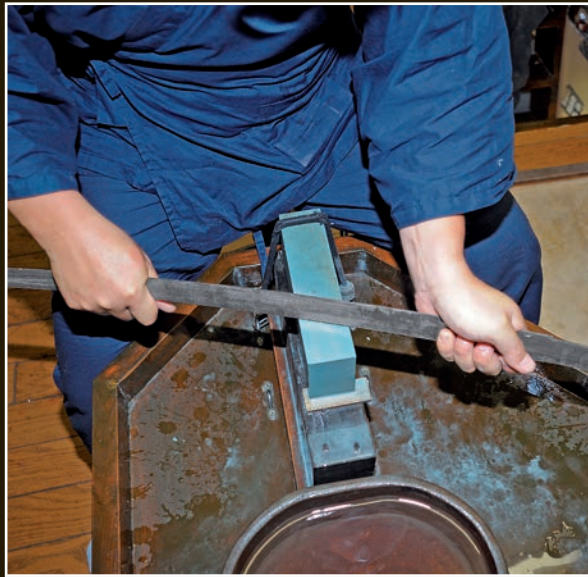
Polishing the mune surface with a stone.
