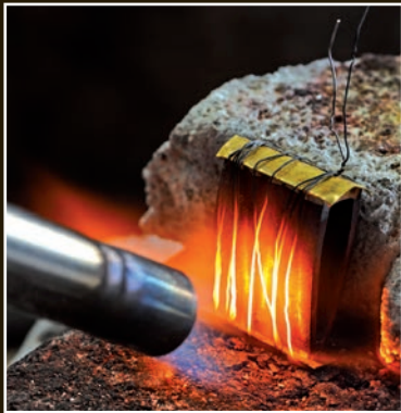
The habaki is heated with the gold foil in place on the mune and ha surfaces.
