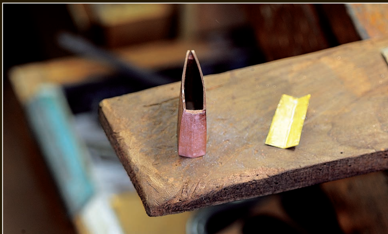
Shaping of the habaki is complete, and all of the surfaces are clean and smooth. Although it looks like copper, this habaki is made out of a gold-copper alloy called shakudo. The gold foil will be soldered onto the mune surface of the habaki.
