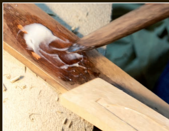
The sokui glue is ready to be applied to each half of the saya.
