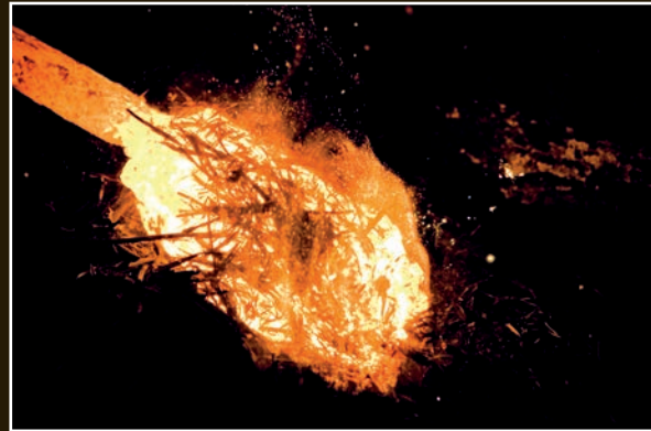
The tamahagane billet is periodically rolled in straw ashes during the heating process. The ashes help protect the steel from oxidation and decarburization.
