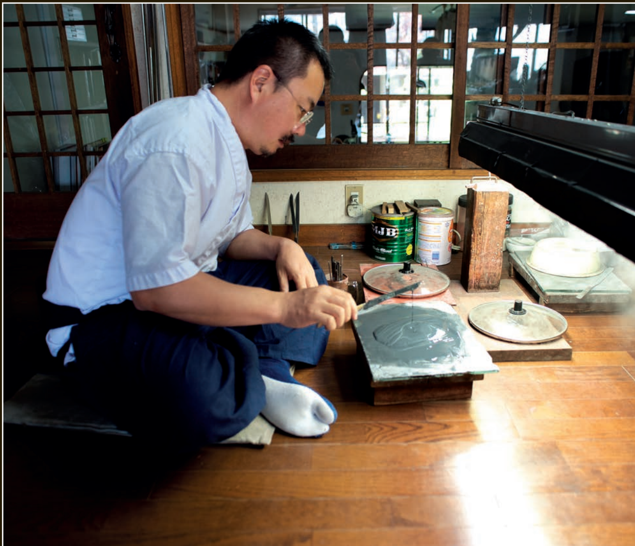
Yoshikazu prepares the black clay mixture that will define the hamon area. When it is at the proper consistency, all of the clay will have dissolved and the mixture will be wet enough to spread over the steel easily. Once it is on the sword, the clay dries rapidly, becoming unworkable.
