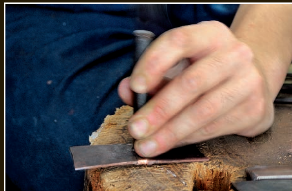
A large, round-faced punch is used to make the inside surface of the center of the habaki slightly concave.
