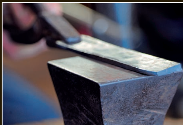
The habaki stock is noticeably thinner on one edge; the cross-section is becoming triangular.
