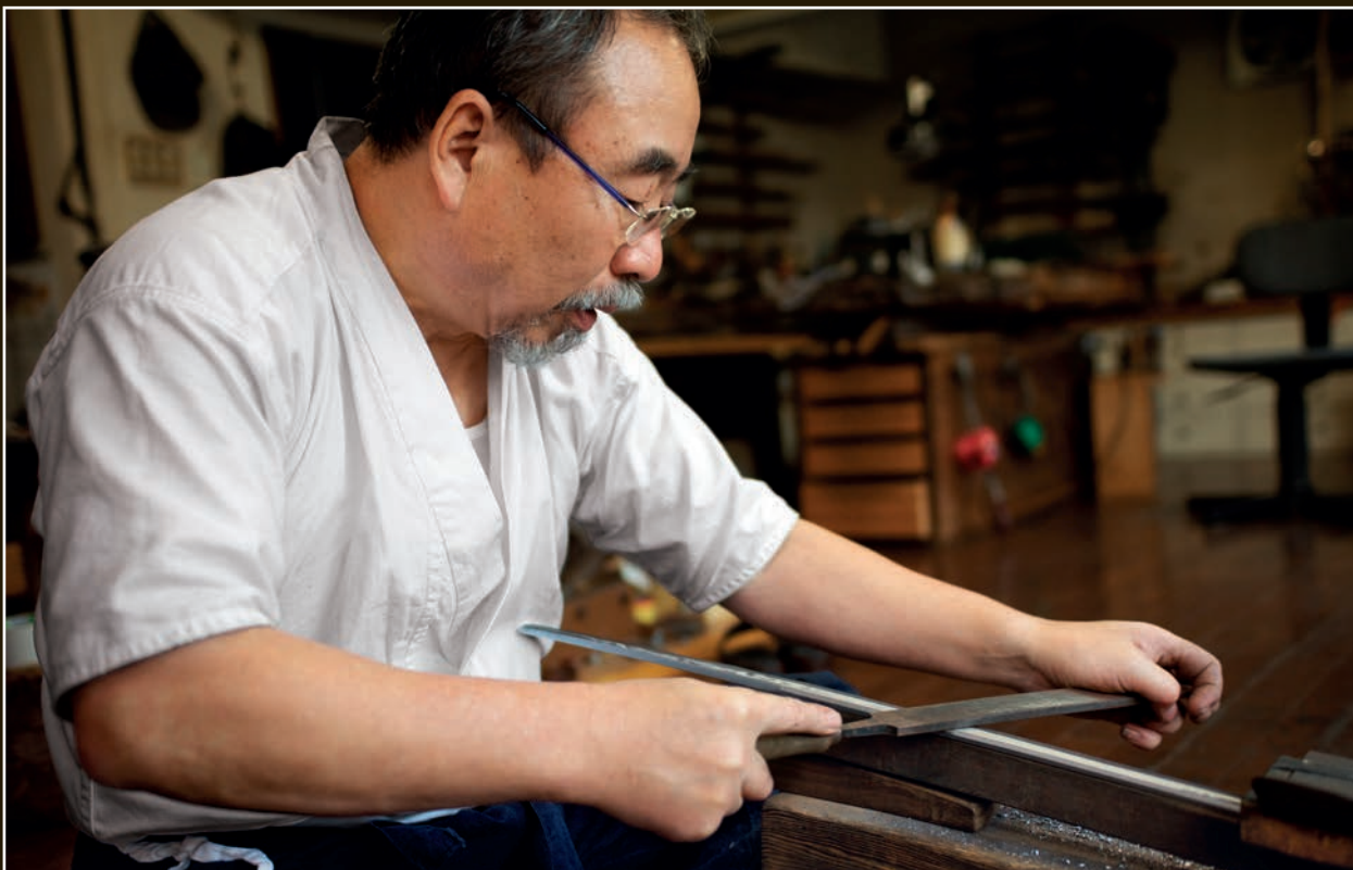
After using the sen, Yoshindo files the surface to make it smoother.
