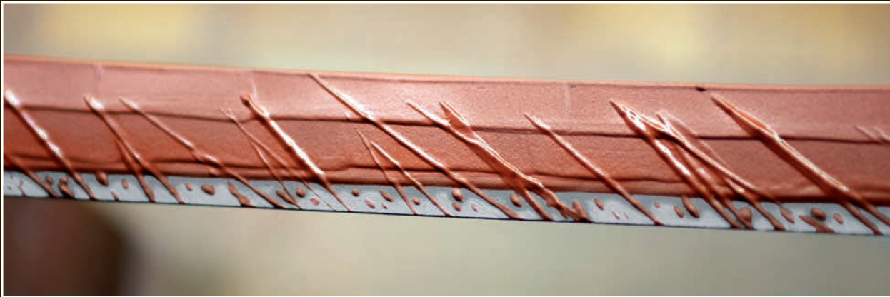
The partly dry gray area gives an idea of the final appearance of the slanted gunome hamon.
