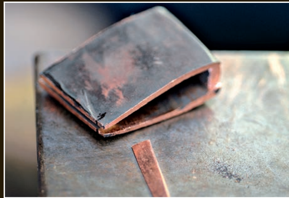
The habaki and the small metal insert that will be soldered in to close the habaki and hold it in place against the hamachi (the notch at the base of the cutting edge).
