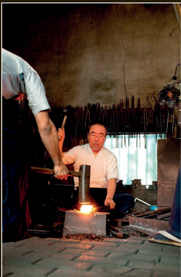
Yoshindo sets the pace as the sakite hammer the steel.
