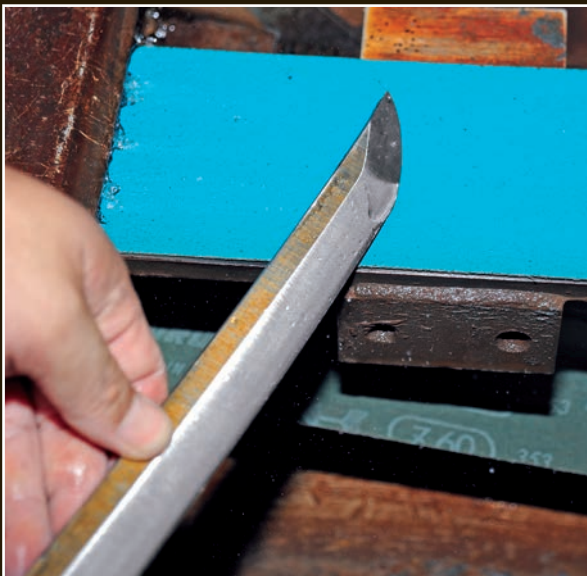
Shaping the point area and edge. When using the belt grinder along the curved point, the cutting edge must be correctly positioned relative to the movement of the belt.
