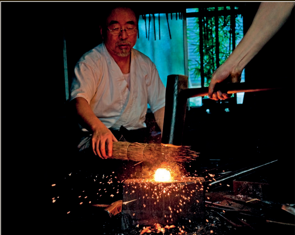
Yoshindo and a student hammer the steel bar.
