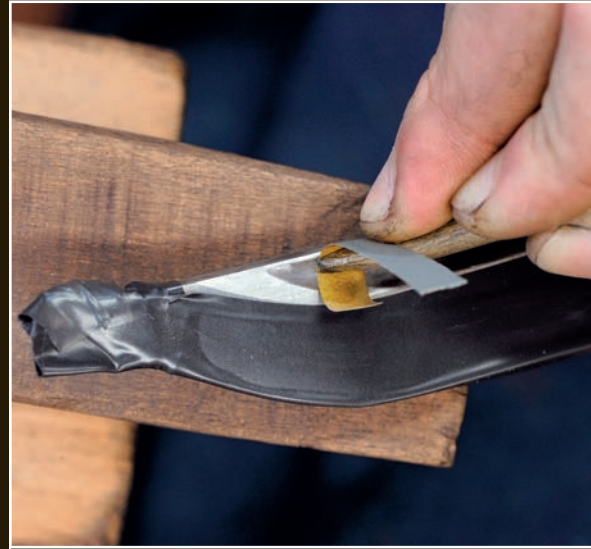
The groove ends are sanded again with finer sandpaper that is held with a piece of bamboo.
