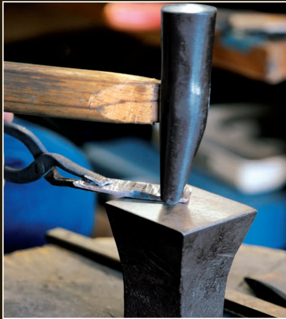
The center of the metal is left thick, while the sides are forged to be much thinner. The thick part in the center will be positioned over the mune surface of the tang.
