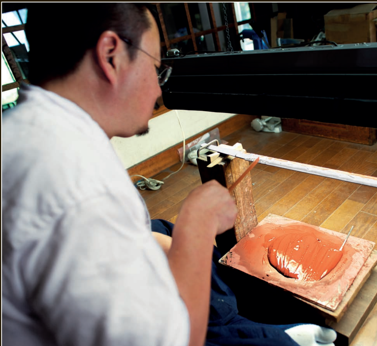
Yoshikazu begins to apply the red clay to the blade.
