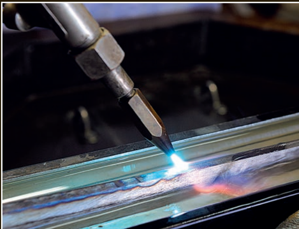
A close-up of the mune being heated with a gas torch. The shinogi-ji and the mune turn black wherever the torch is focused, so it is easy to monitor the process.
