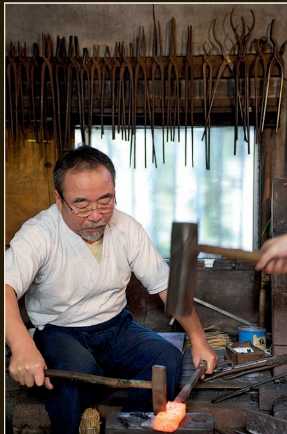
The drawn-out billet will be scored with a chisel while hot, and then folded over onto itself.
