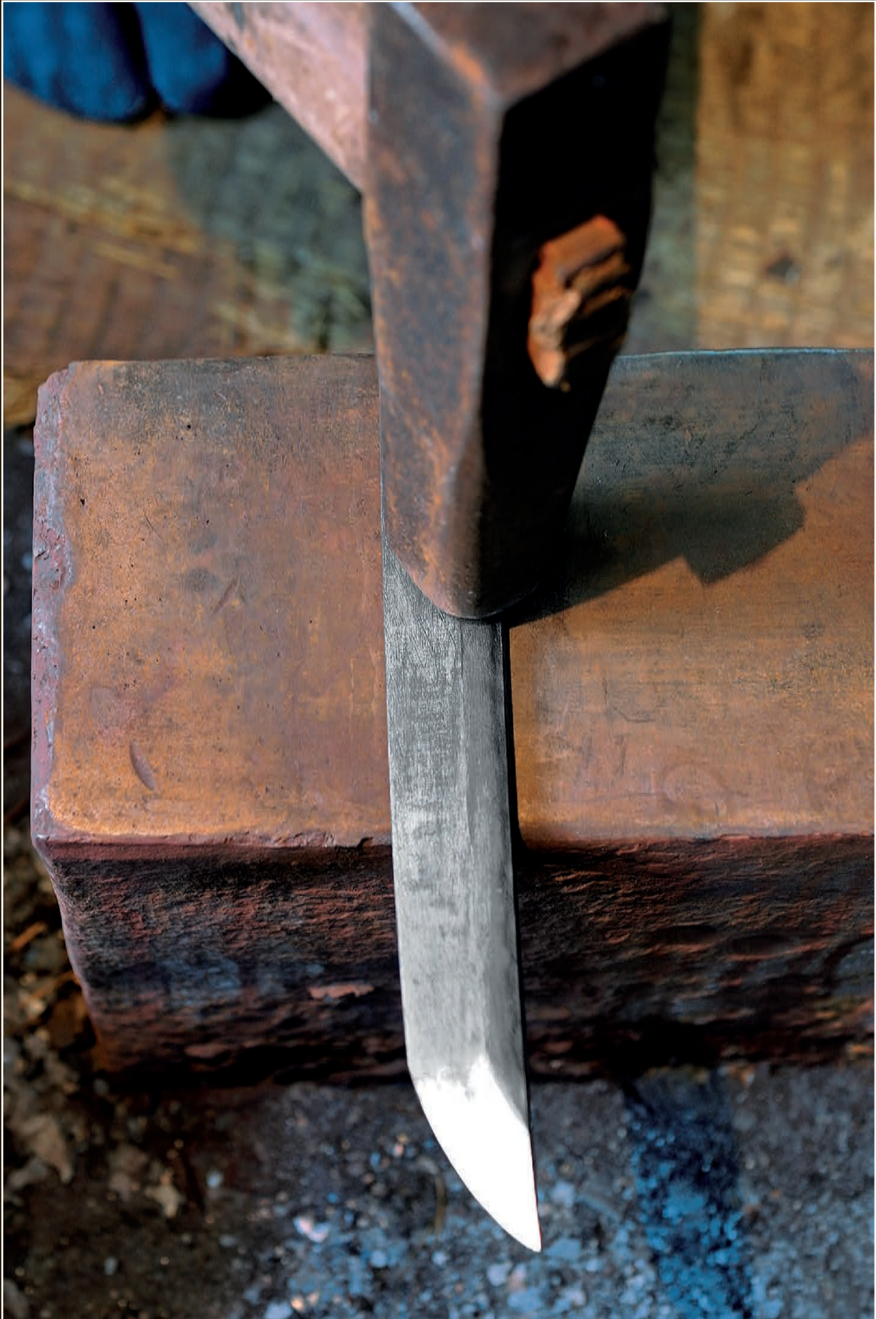
The sori is adjusted by hammering on the shinogi-ji. The black marks on the mune show where the blade was heated to introduce more curvature.
