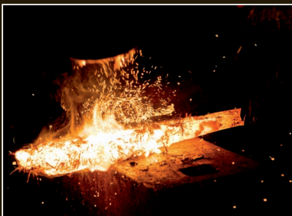
Forging the steel bar. The sparks swirling around the steel are from the straw ashes.
