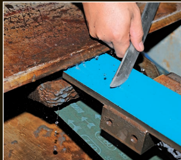
The ha (cutting edge) is formed on the point area.
