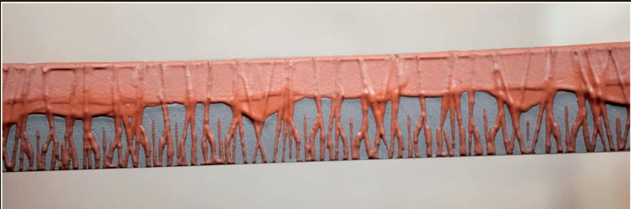
Ashi are placed along the entire hamon. In this photo, the upper red layer is visibly thicker, and the red ashi are visible over the black clay. This pattern will produce a choji-midare hamon.
