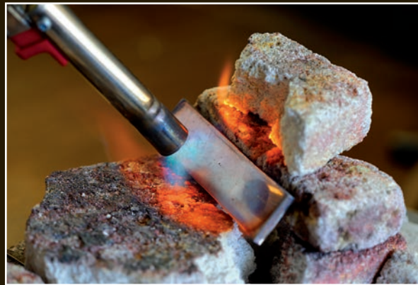
Work-hardened metal is heated to a red color and then cooled. The metal will then be soft enough to continue forging.
