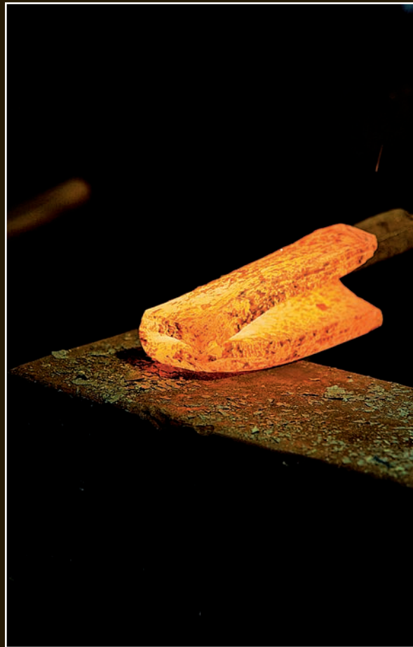
The kawagane is ready for the shingane to be inserted.
