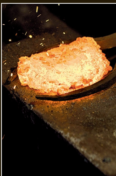
Quenching the tamahagane. A piece of tamahagane is heated and forged into a thin plate. When the plate is still a red or yellow color it is quenched in water to cool it rapidly. It is then broken up into small pieces.
