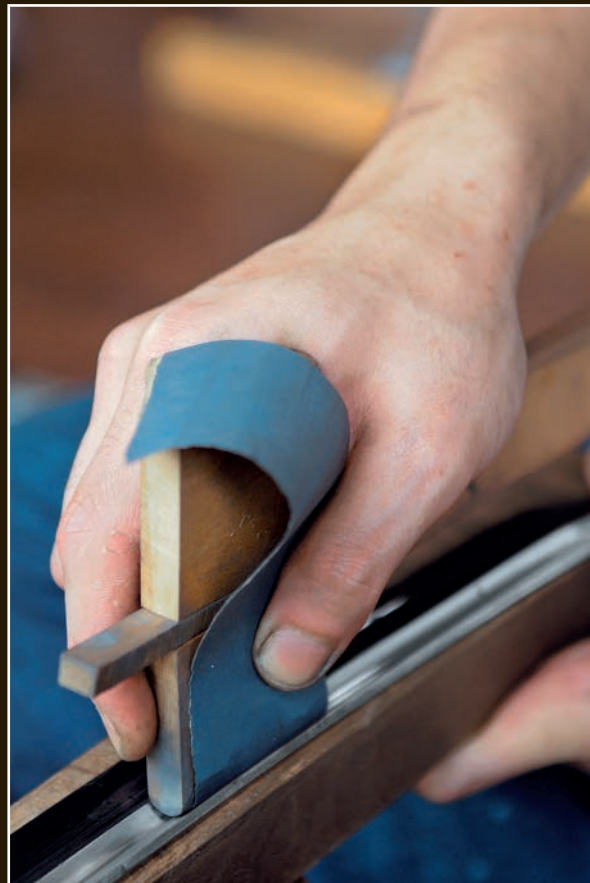
After filing, the insides of the grooves are sanded to a very smooth finish. Mizuki is using a rounded sanding block to control the sandpaper.
