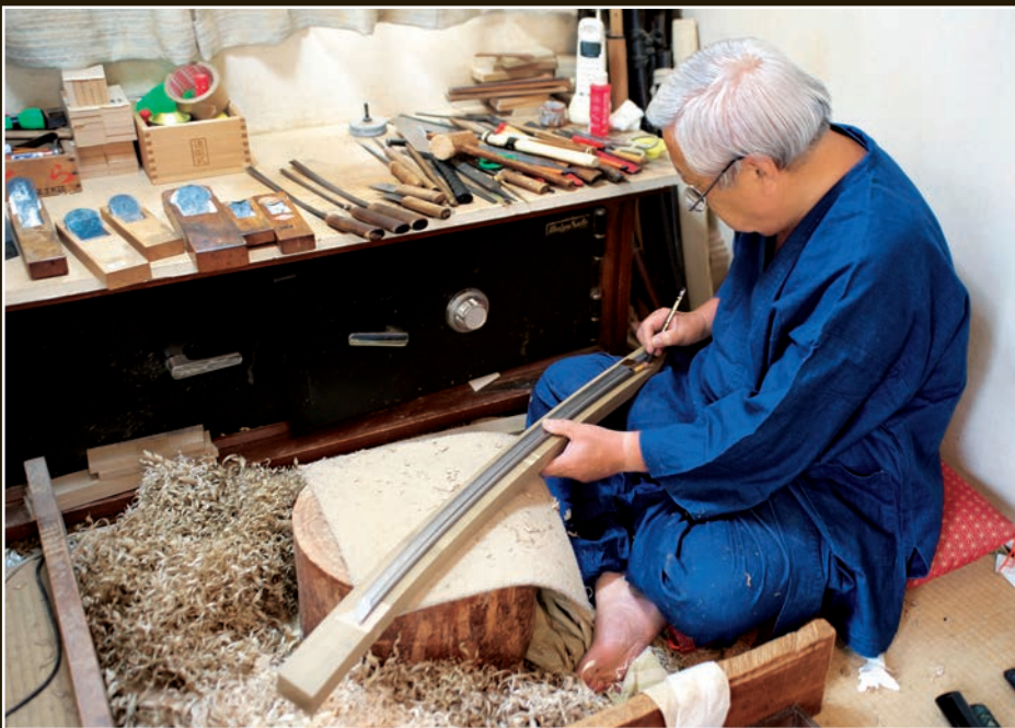
Okumura marks the line at the top of the habaki to determine where the top of the saya will be. He will then make the cut to separate the hilt from the scabbard.
