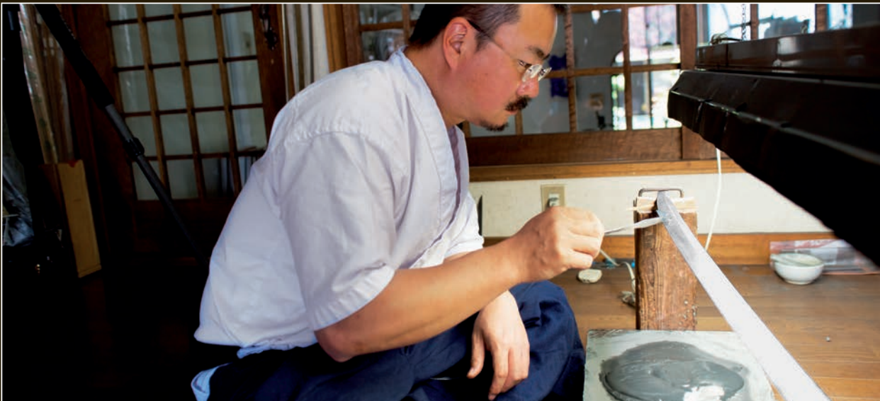
Yoshikazu begins to spread the black clay mixture over the area where he plans to form the hamon. He uses a small spatula to apply the clay exactly where he wants it.
