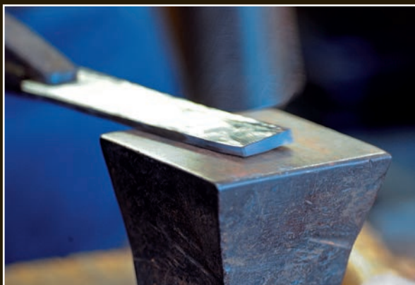
The habaki is forged so that one edge is thinner than the other.
