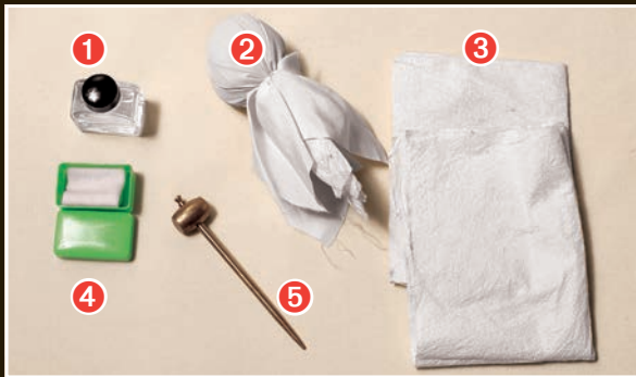
Items used to maintain and clean a sword. 1. Clove or camellia oil. 2. Uchiko wrapped in two layers of fabric. 3. Handmade Japanese washi paper used to wipe swords (plain facial tissue may also be used). 4. A small square of cotton cloth used to hold the oil. 5. The mekugi-nuki hammer used to remove the bamboo pin that secures the sword in the hilt.
