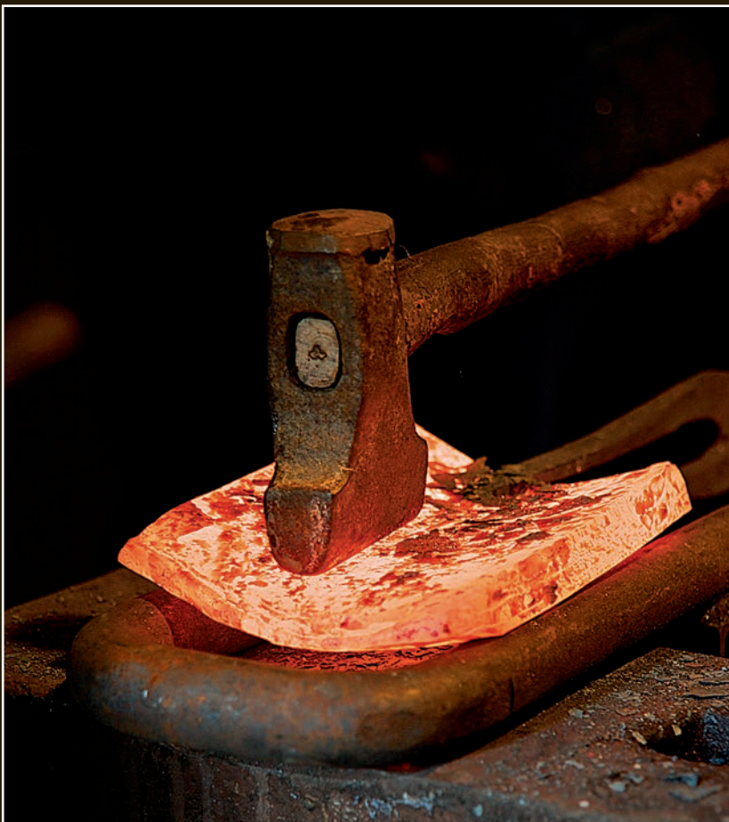
Beginning to bend the kawagane plate into a U shape.
