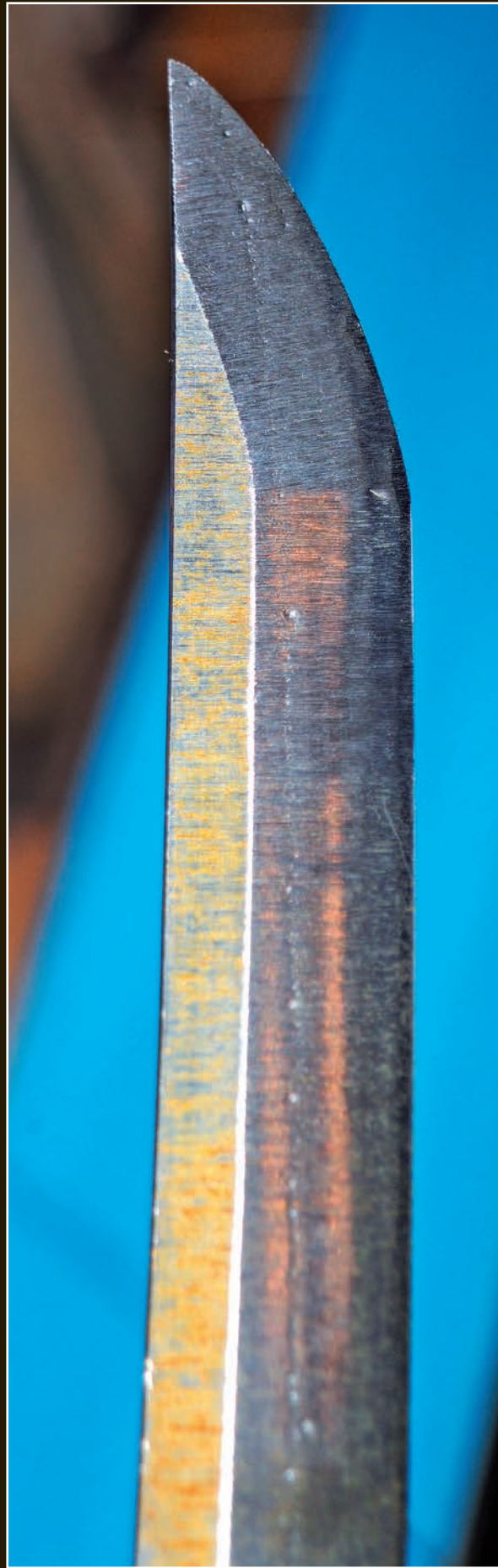
The work with the belt grinder is finished, and the complete detailed shape of the sword is now defined.
