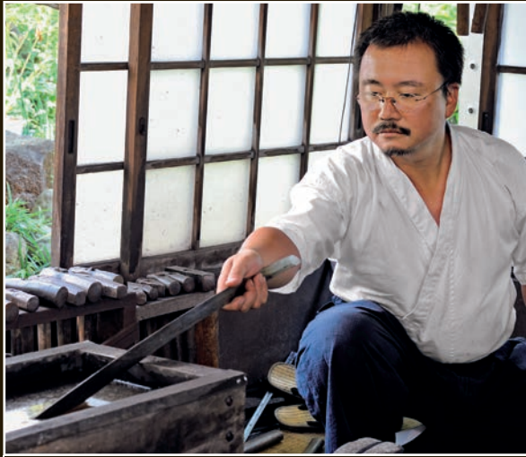
Each time the the sword is heated to adjust the curvature, it is quenched in water. The hamon can be damaged if the steel gets too hot.
