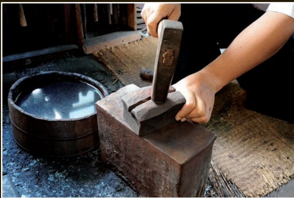
The copper block is adjusted to fit the sword.
