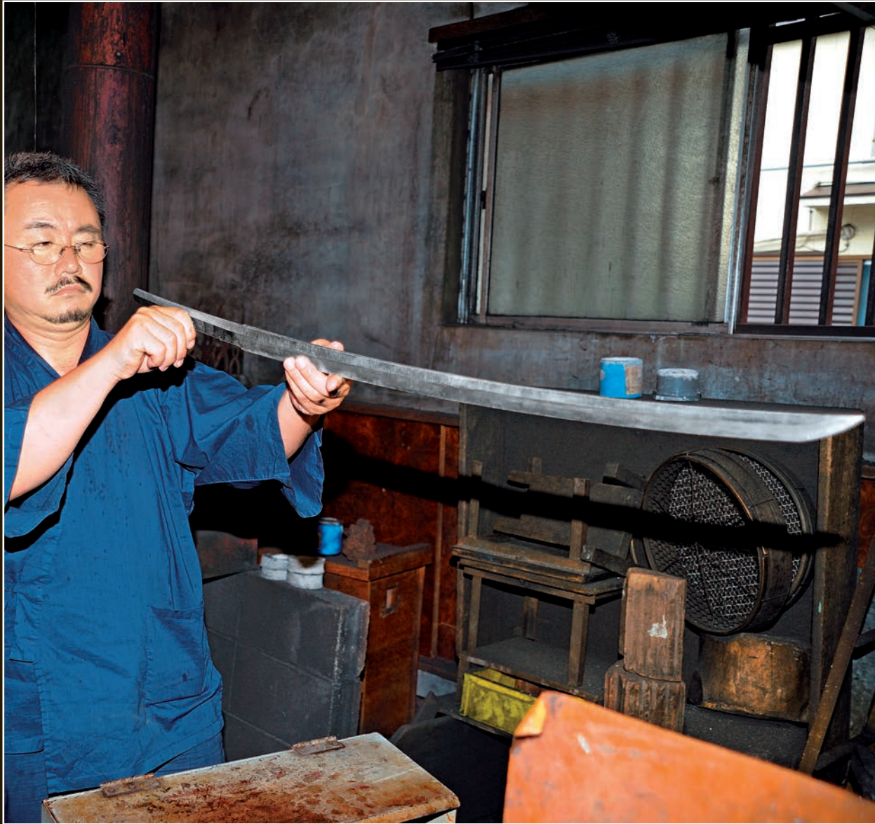
The blade is checked frequently and carefully. There must be no uneven surfaces. Once the shape is formed, taganeha (cutting a beveled sharp edge) begins.
