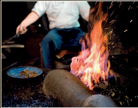
Charcoal is burned to heat the forge.
