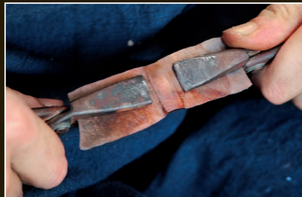
Using smooth-jawed pliers to begin bending the habaki into a U shape.
