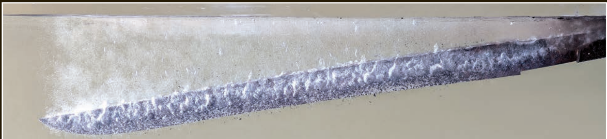
The blade 1.2 seconds after entering the water. It is a bit straighter, and there are fewer bubbles along the edge. The sides are covered with numerous large bubbles.
