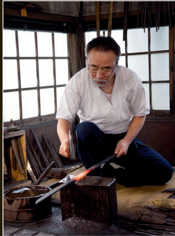
Finishing and adjusting the lines and surfaces of the sunobe.
