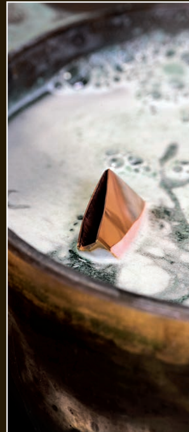
The habaki is immersed in a hot solution of cupric sulfate and cupric oxide to give its surface a glossy black patina.
