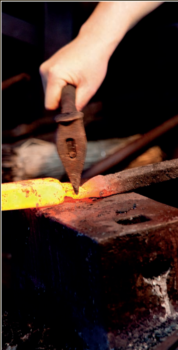
Cutting off the handle that was welded to the shingane core steel. This end of the bar will form the tang.
