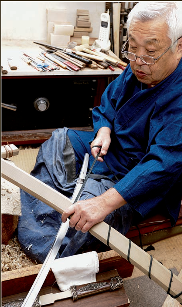
The cord securing the halves of the saya must be tied very tightly, the surfaces fit together seamlessly.
