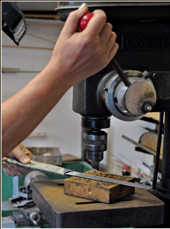
Drilling the hole for the mekugi (bamboo rivet).
