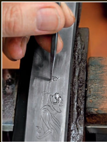
Yoshindo uses a hammer and chisel to deepen the lines and details of the horimono, starting with the paw and claws on the leading edge of the engraving and working his way down.
