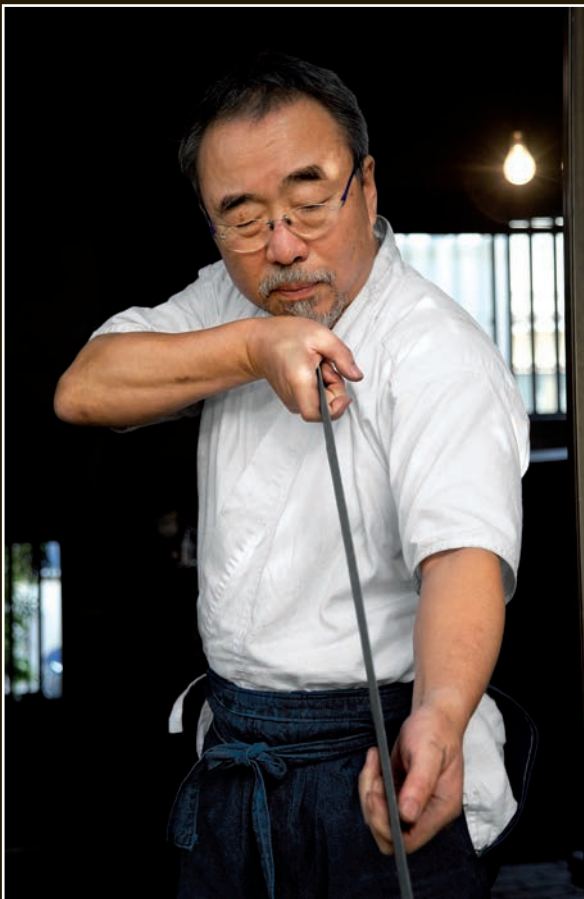
Inspecting the shape of the blade. The blade is constantly inspected to monitor the straightening process.
