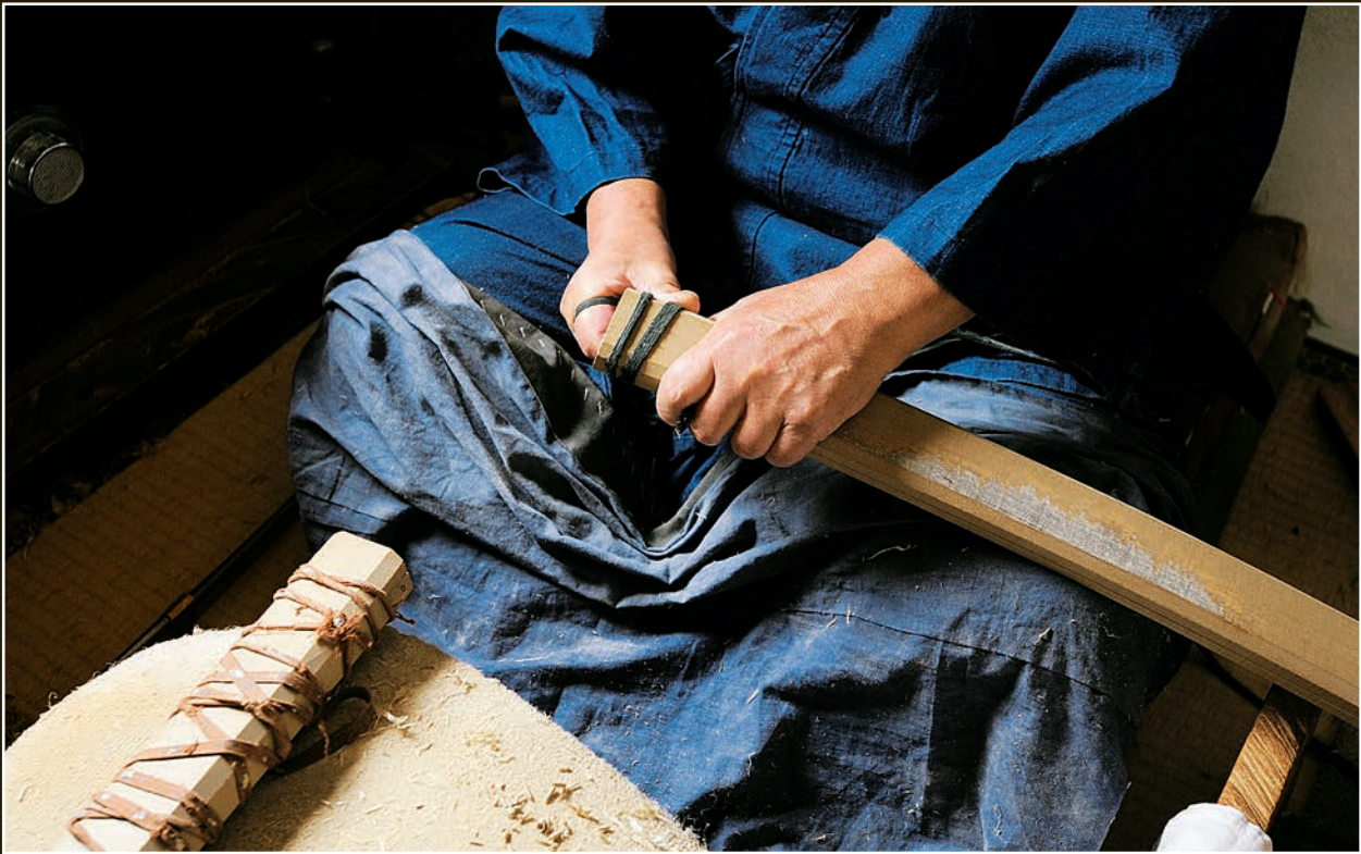
It is essential that the interior surfaces are correctly positioned when the halves are glued together. Okumura is tying the two halves of the saya tightly together with a cord so that they do not slip. The two halves of the hilt, already tied together, are in front of him.
