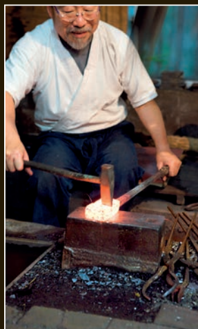
Using a chisel to cut partway through the steel.
