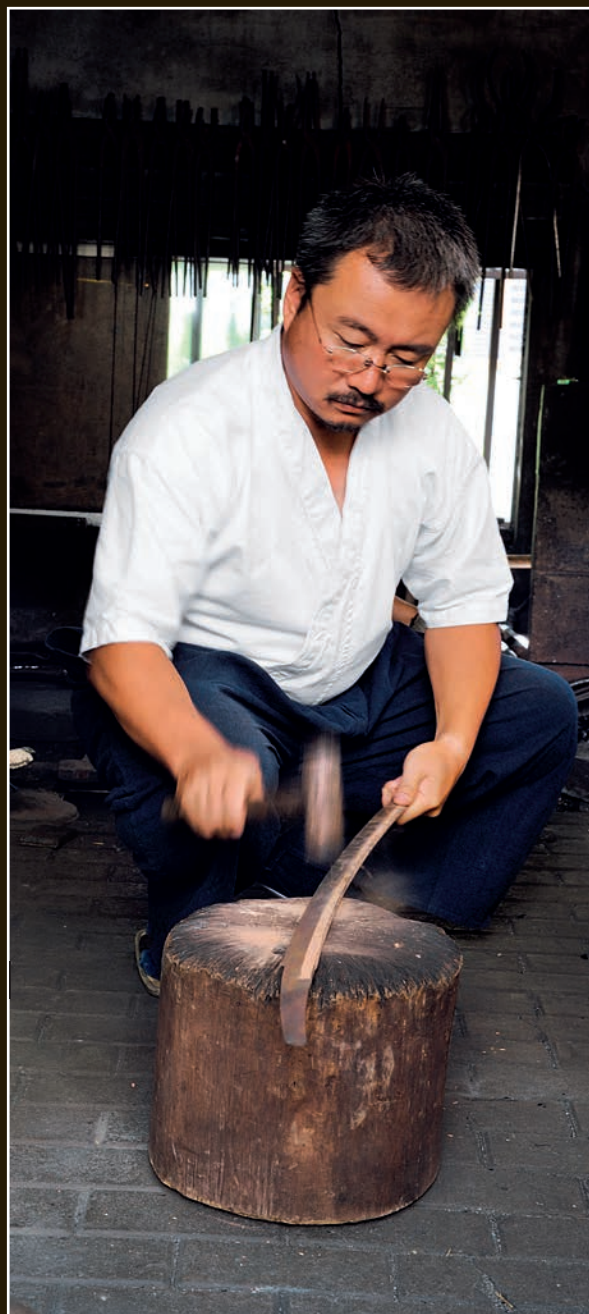
Yoshikazu straightens the sword by hammering along the shinogi-ji .
