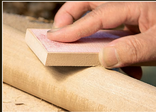
Cleaning the surface with a tokusa sanding block to produce a fine surface finish.
