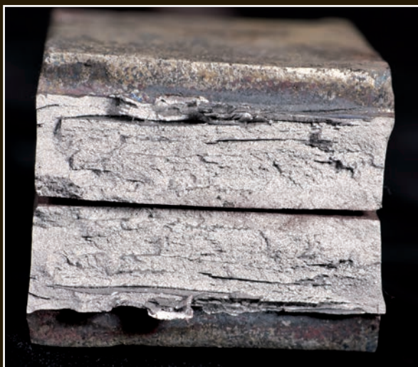
Cross-section of the tamahagane billet after the shita-kitae stage.
