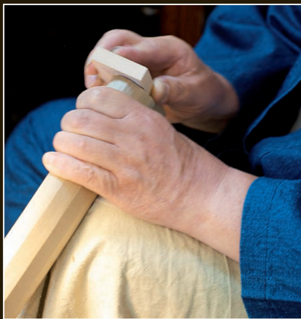
Okumura uses a tokusa sanding block so that the mouth of the saya and the base of the hilt will mate perfectly.
