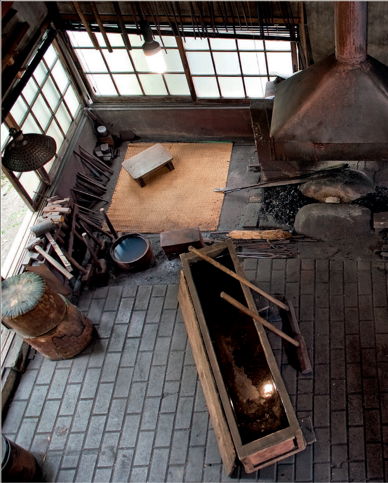
A view of Yoshindo's shop. Every surface is covered with ash and charcoal dust. The shop is kept dark so that the color of the steel can be accurately observed during forging.
