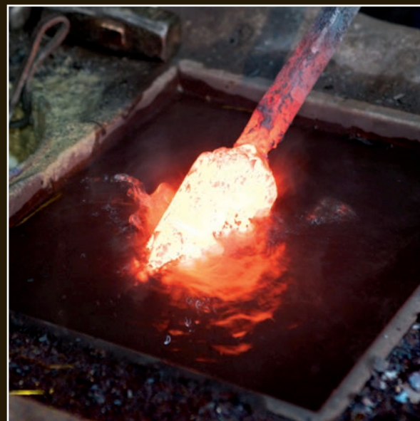
The billet is quenched in water.
