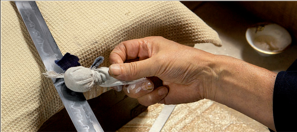
Before burnishing the sword, a fine, waxy powder called "ibota" is applied to the surface and wiped off. This acts as a lubricant during burnishing.
