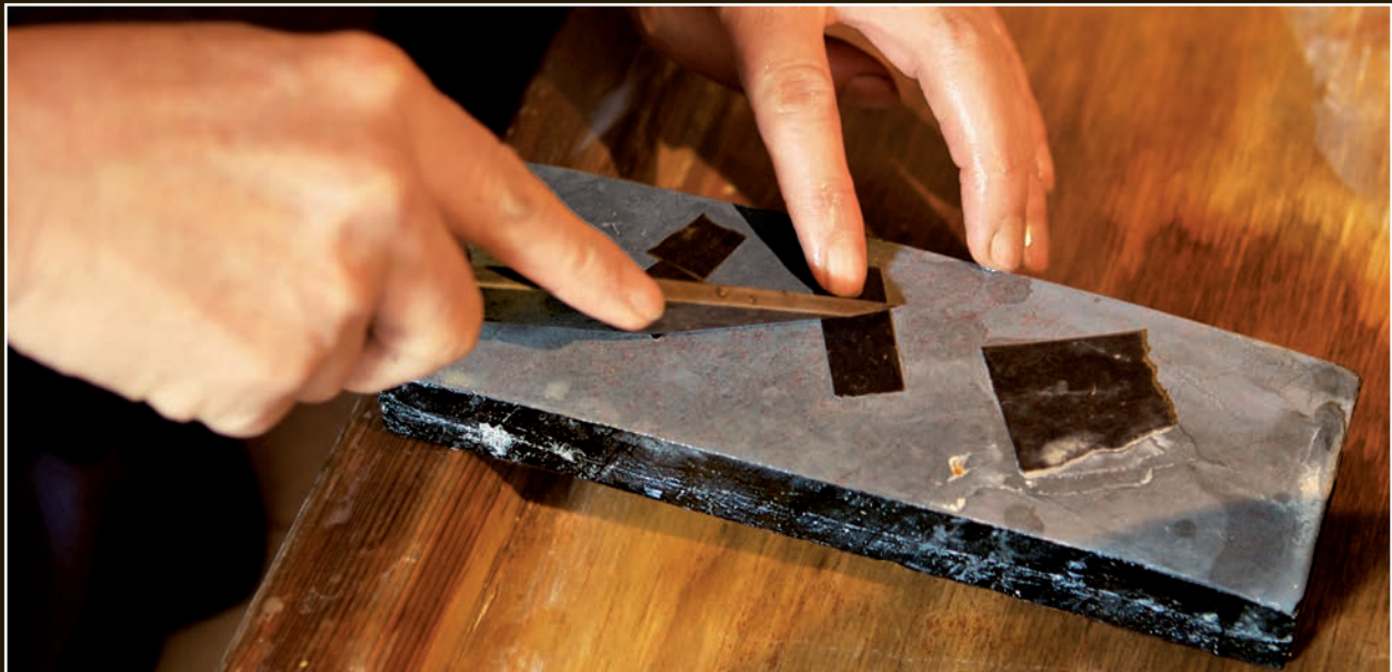
Takaiwa cuts hazuya into small pieces for hadori. He will use these to polish the hamon.
