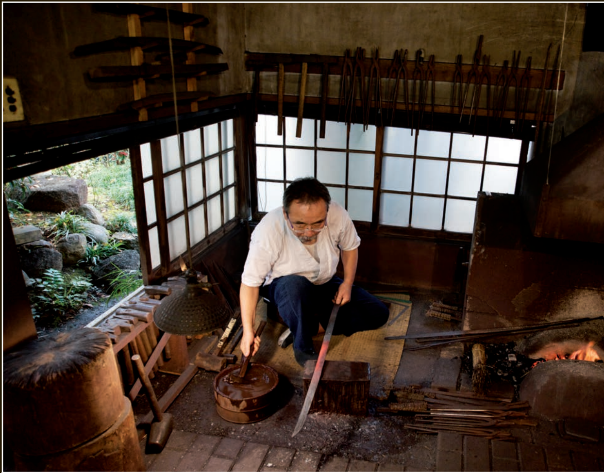
Yoshindo pauses to dip his hammer in water as he works his way back along the sword to the tang.
