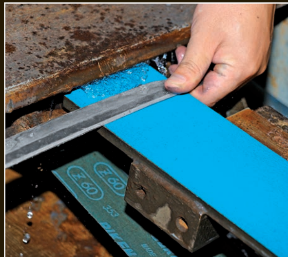
Working on the shinogi-ji surface from the machi to the point. This surface must have a continuous thickness in proportion to the blade's width.
