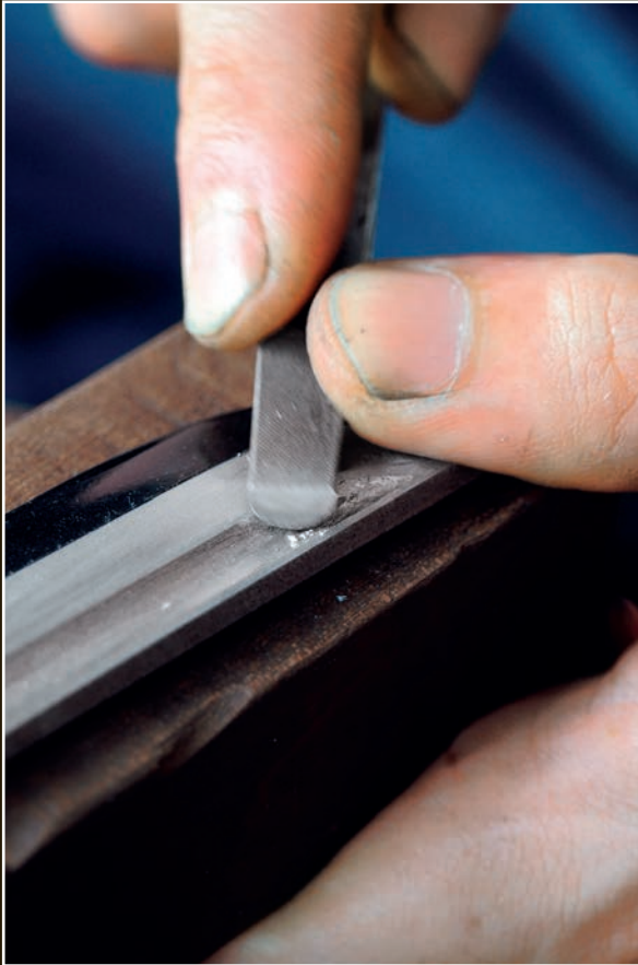
A handheld chisel is used to finish cutting the grooves right up to the original inked lines.
