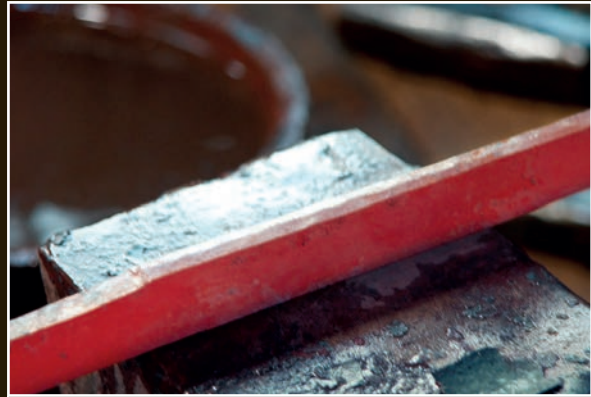
The mune (unsharpened back edge of the sword) has two surfaces topped by a ridge.
