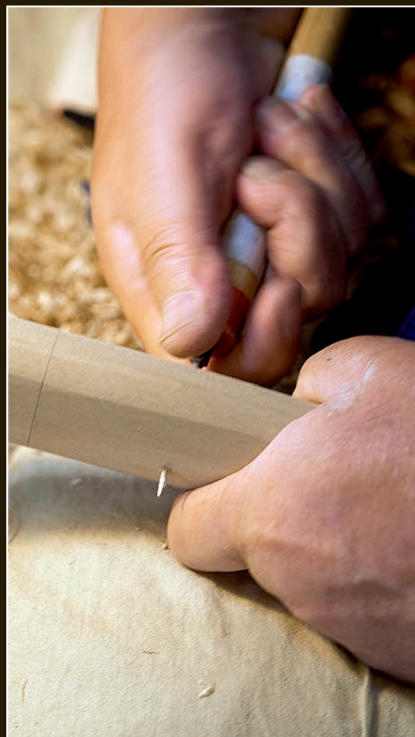
The mekugiana is drilled through the hilt while the blade is in the saya.
