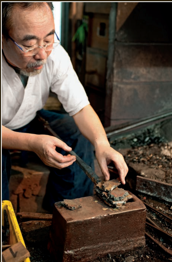
Stacking the tamahagane pieces on the plate.
