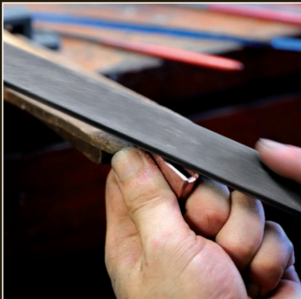
Filing the surface of the habaki that will be closest to the point.
