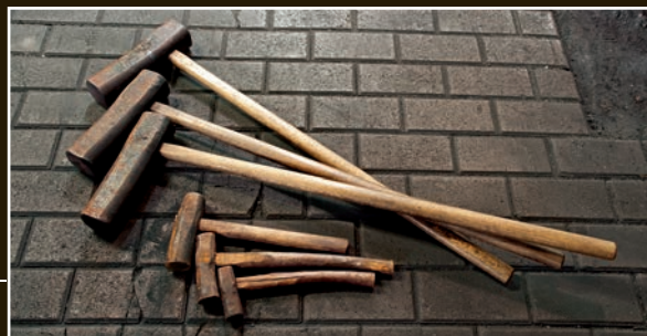
Hammers used in sword-making.
