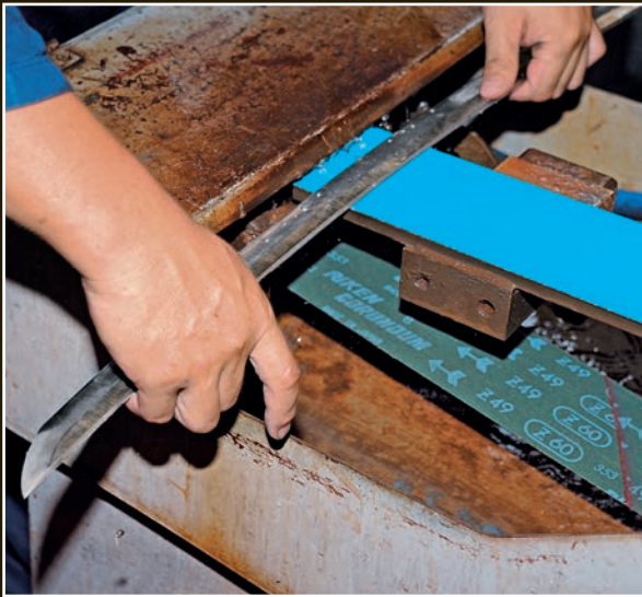
The two photos above show the shinogi-ji being formed on both sides of the sword. This defines the nikuoki (cross-section) of the blade.
