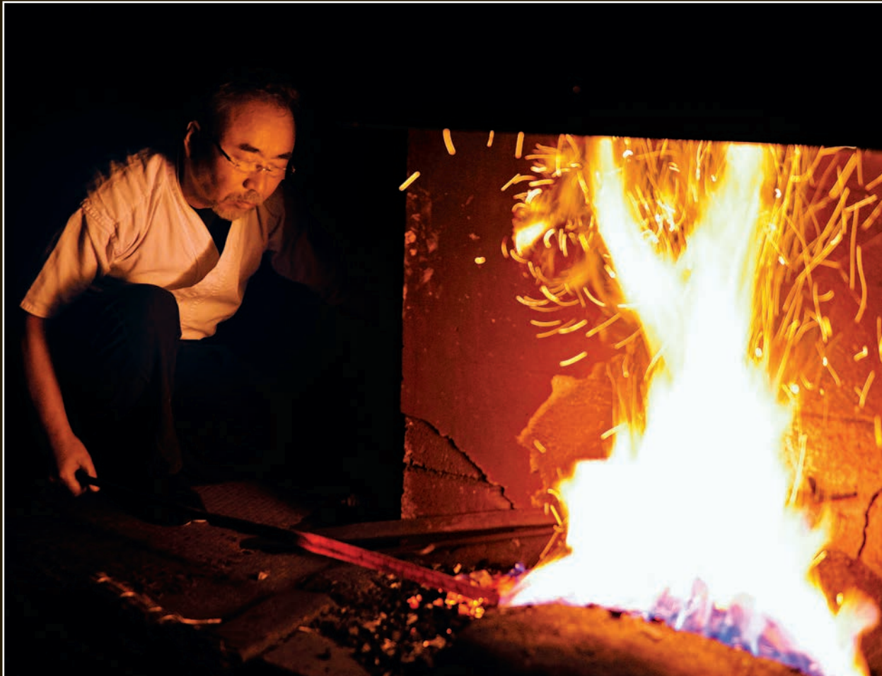
Yoshindo begins to heat the sword in the forge at the start of the yaki-ire process. Holding the blade edge-up, he slowly moves it into the forge and then pulls it out again, pumping the fuigo (bellows) all the while. The clay pattern on the blade can be seen clearly here.
