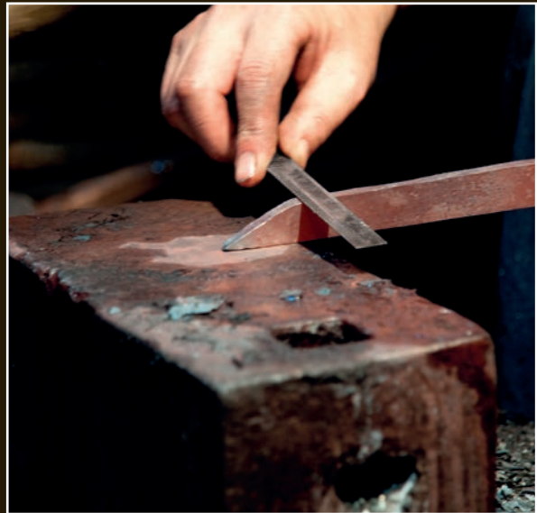
Yoshindo checks the dimensions of the point area.
