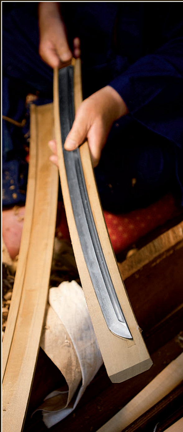
Checking the fit of the sword inside of the saya. Notice the square pocket carved below the point of the blade. This is to create a space inside of the saya where excess oil from the blade can accumulate.
