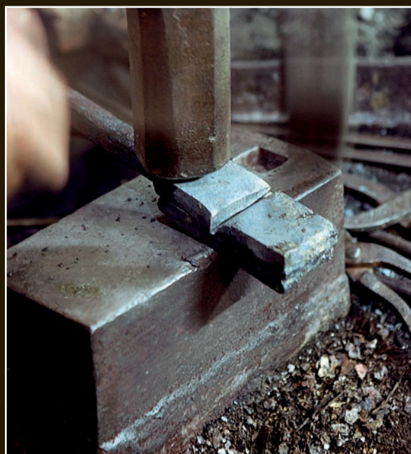
The cooled billet is broken into sections.
