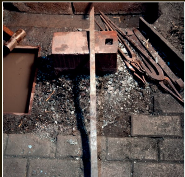
The composite steel bar has been forged into the sunobe, the blank from which the sword will be made.
