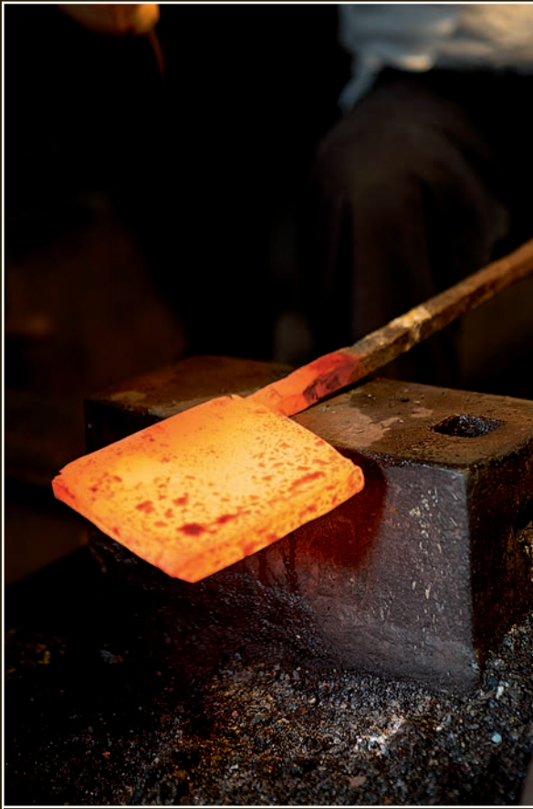
The kawagane bar has been forged into a nearly square plate.
