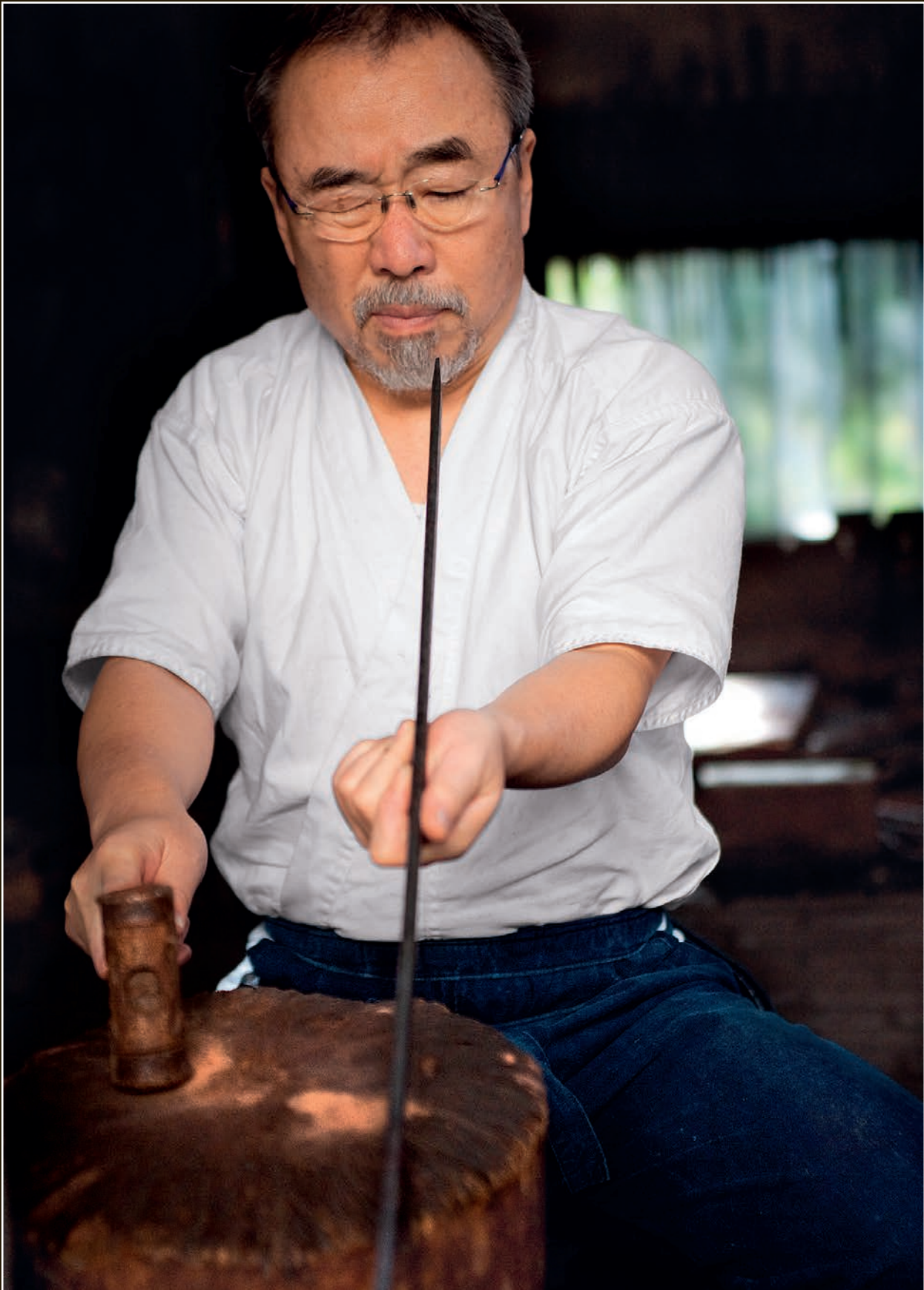
Yoshindo inspects the blade for straightness.
