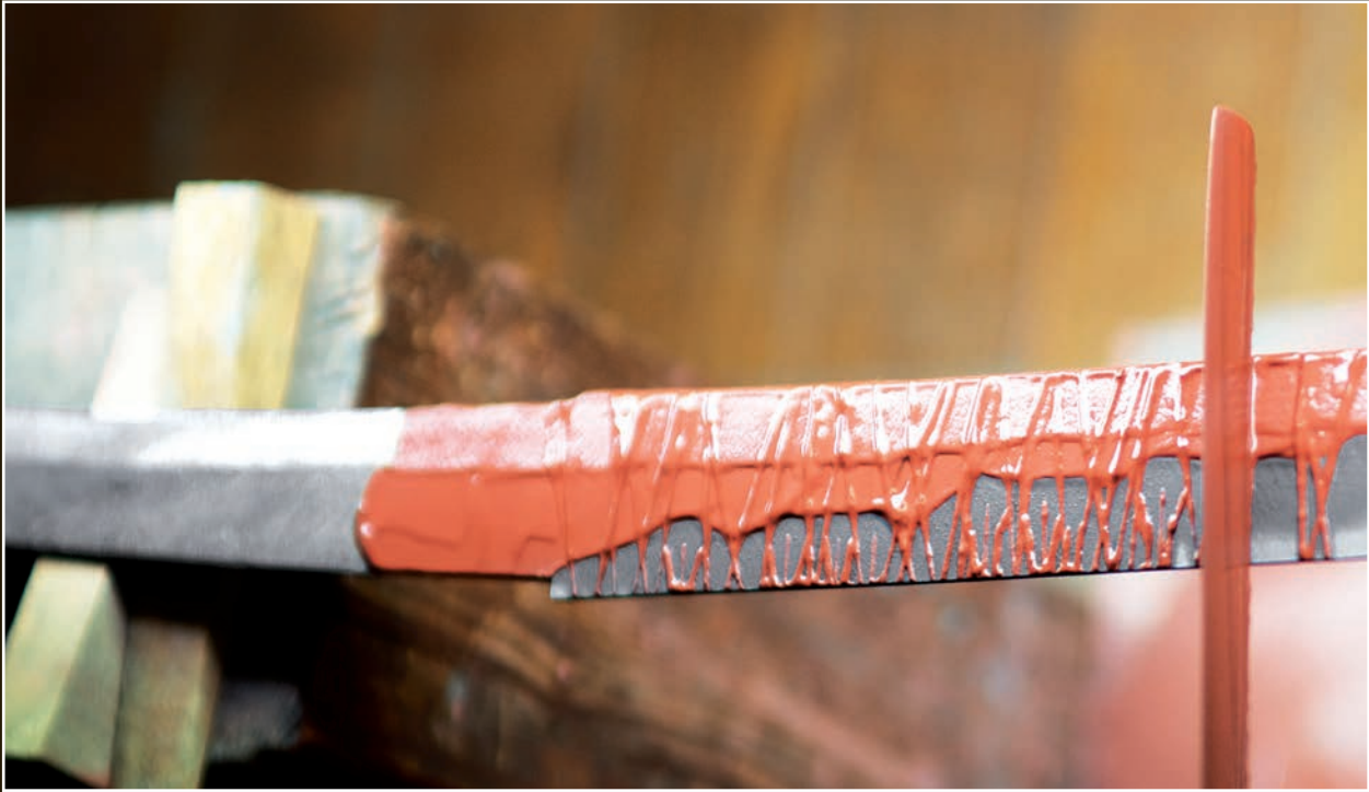
Applying the ashi. A spatula is dipped in red clay and rolled across the blade to leave a thin strip across the black clay coating. The area under the strips will not harden during yaki-ire, resulting in thin lines of soft steel across the hardened edge.
