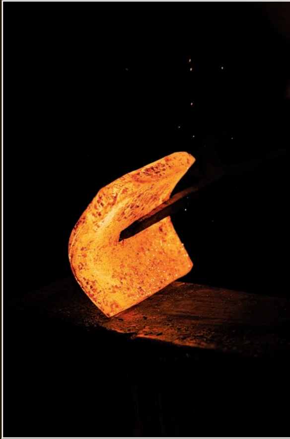
The kawagane plate has been bent slightly.
