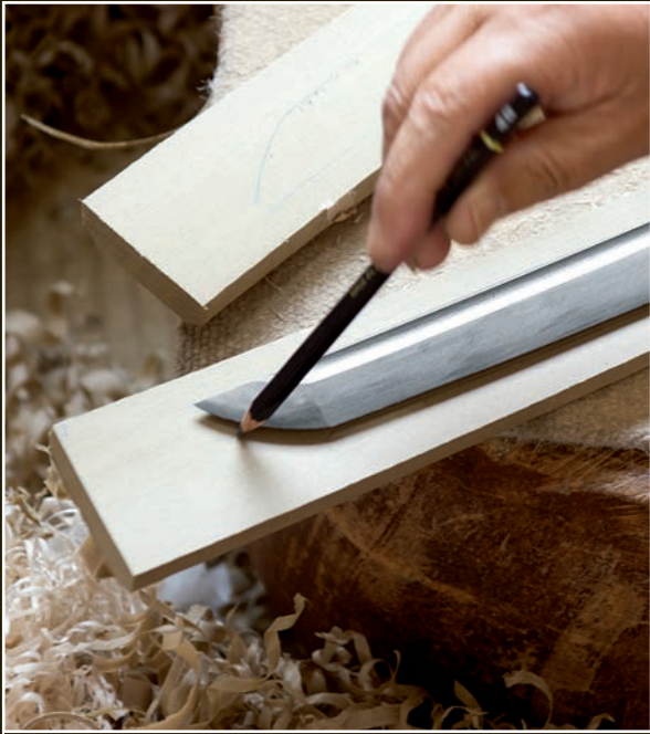
The wood has been cut into the rough shape of a saya and then split into two halves that will be glued back together again after the interior has been carved out. Okumura draws the outline of the sword on the saya blank.
