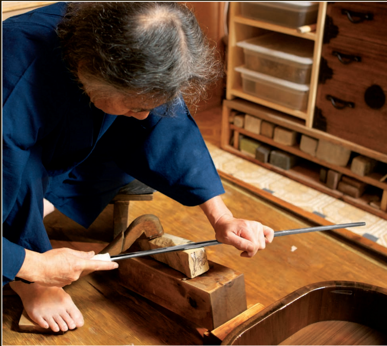
Takaiwa polishes a shinogi-zukuri sword. He uses the same hand position and way of handling the blade here as he did for the wakizashi shown previously.
