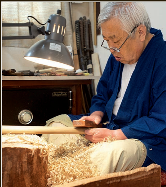
Okumura uses progressively finer planes to work on the surface of the saya.
