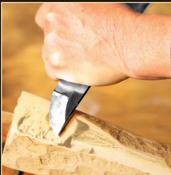
Here Takaiwa polishes the point area on a katana. The surface is whiter, contrasting strongly with the reflective body of the sword, because the point area is polished moving perpendicular to the sword's lengthwise axis.
