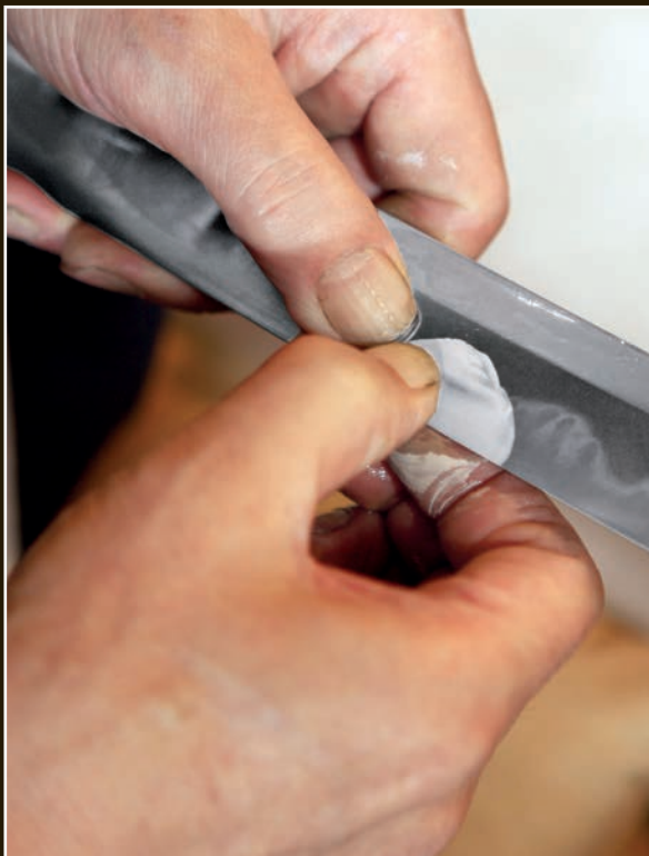
The hamon is polished very carefully from the edge side. The hadori is under Takaiwa's right thumb, surrounded by white tojiru paste. The part of the hamon to the right of Takaiwa's thumb, which has already been polished with the hadori, is much whiter than before.
