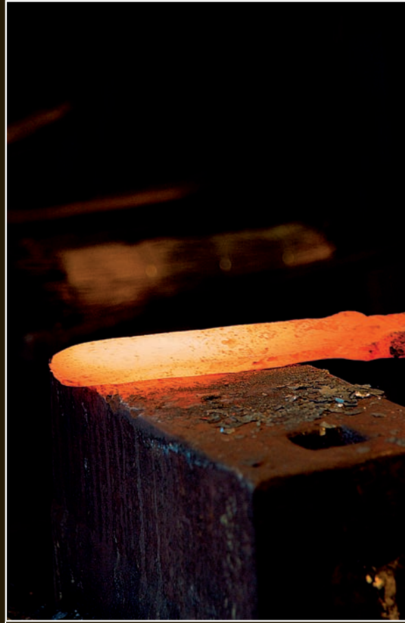
The shingane is forged so that it is tapered at one end.
