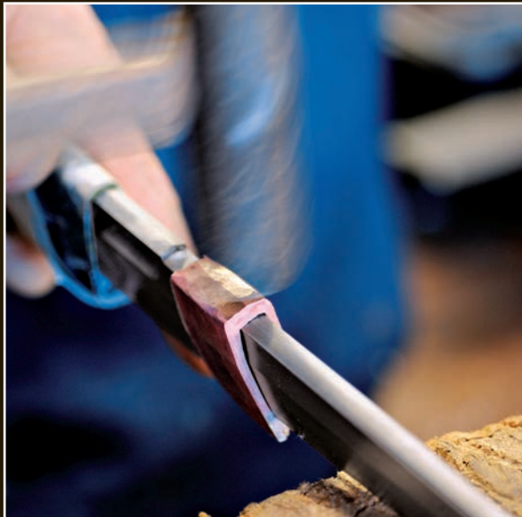
The habaki is being shaped over the tang and stretched into position with careful hammering.
