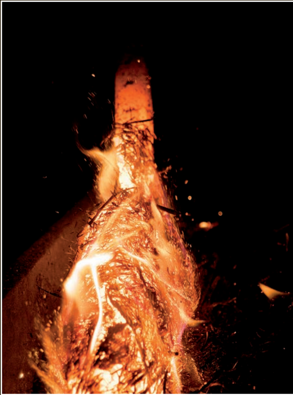
The steel is periodically rolled in straw ashes and returned to the forge.
