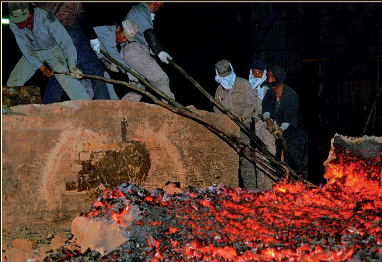
After the tatara operation is finished, the workers tear down the walls of the tatara and rake out the remaining charcoal to uncover the kera (steel mass).
