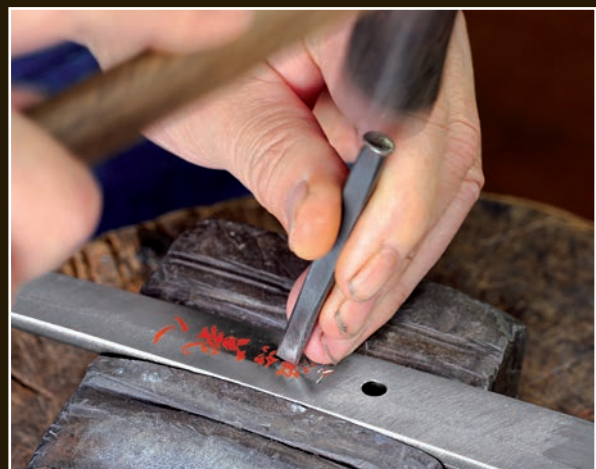
Inscribing the mei onto the tang. This is done using a hammer and chisel, following the inscription brushed in ink on the tang.
