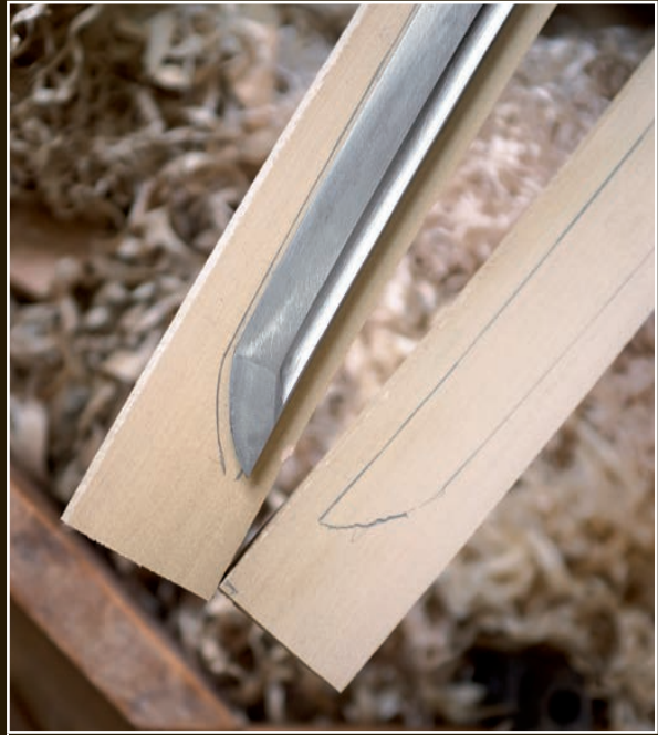
The outline of the sword is carefully marked on both halves of the saya blank.
