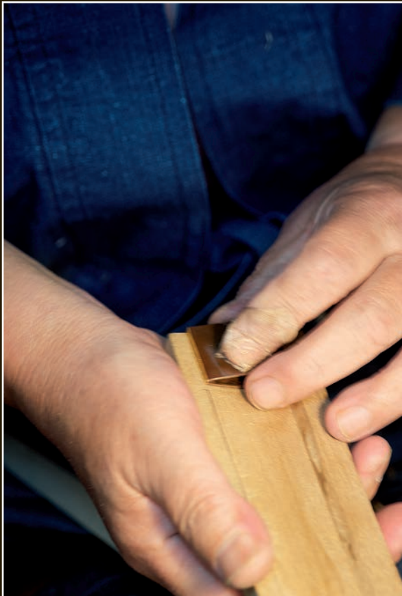
The mouth of the saya must be adjusted so that the habaki will fit snugly. The space must be carved out very carefully so that the upper third of the habaki grips the mouth of the saya.
