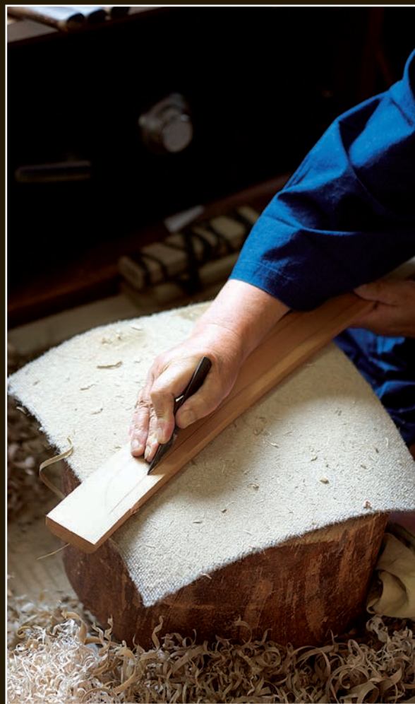
The kiridashi is used to cut all along the sword's outline.
