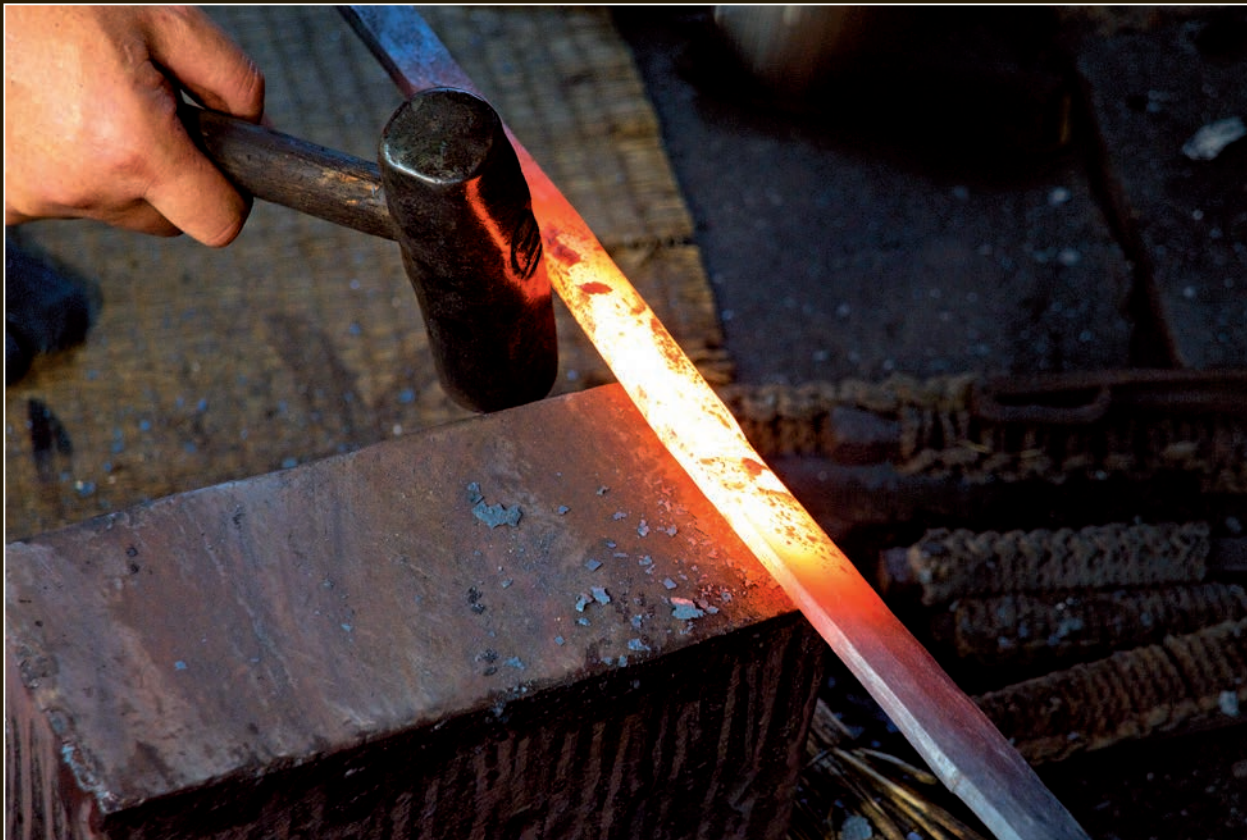
Yoshindo has shaped the first 4 to 6 inches (10-15 cm) of the sword, including the shinogi ridge line and the tang. The original sunobe shape is visible above the forged area.
