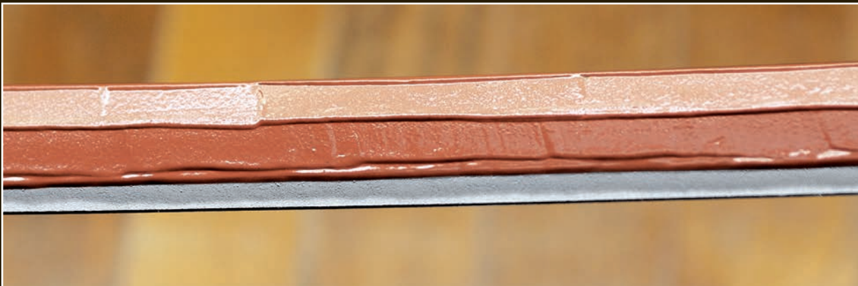
This clay coating will produce a suguha (straight) hamon without ashi.
