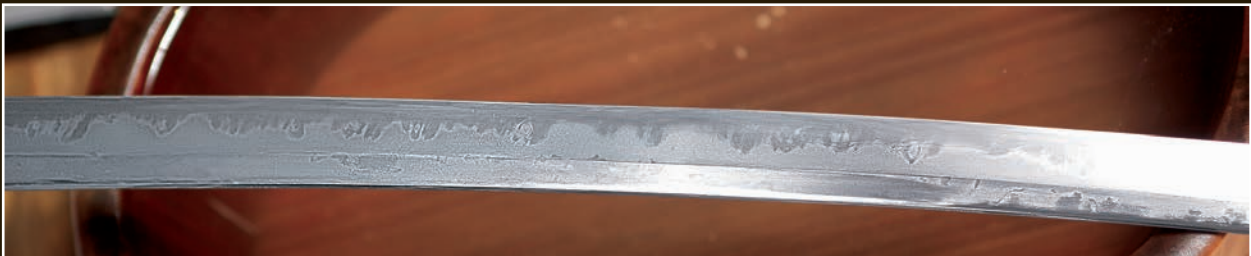
The surface has a uniform milky white appearance after being polished with the hazuya. The hamon and the nioi line are very clear.
