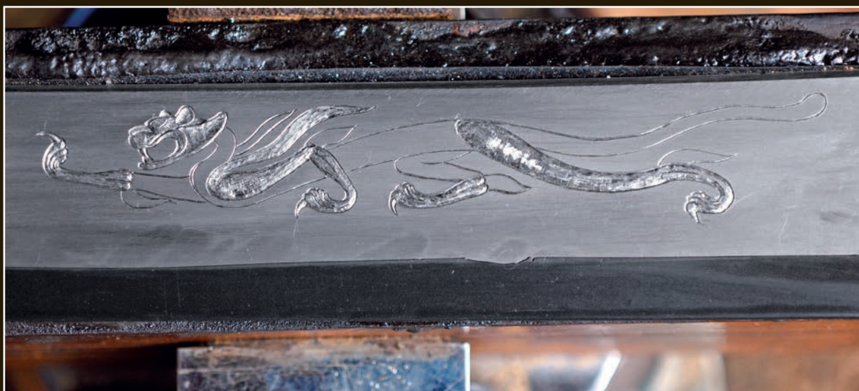
The horimono will not be flat, but is carved out from the surface of the sword. Here, the legs and head have been chiseled out.
