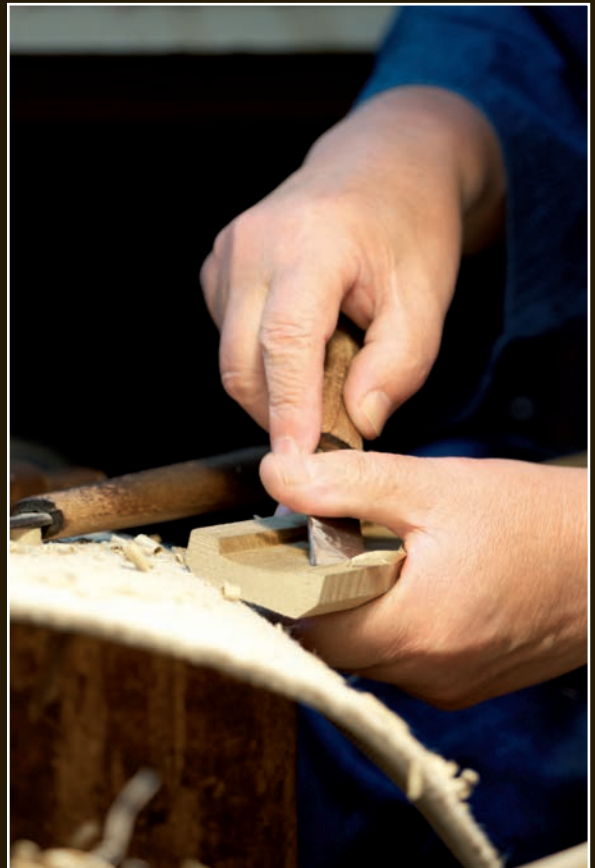
Carving out the mouth of the saya to fit the habaki properly.
