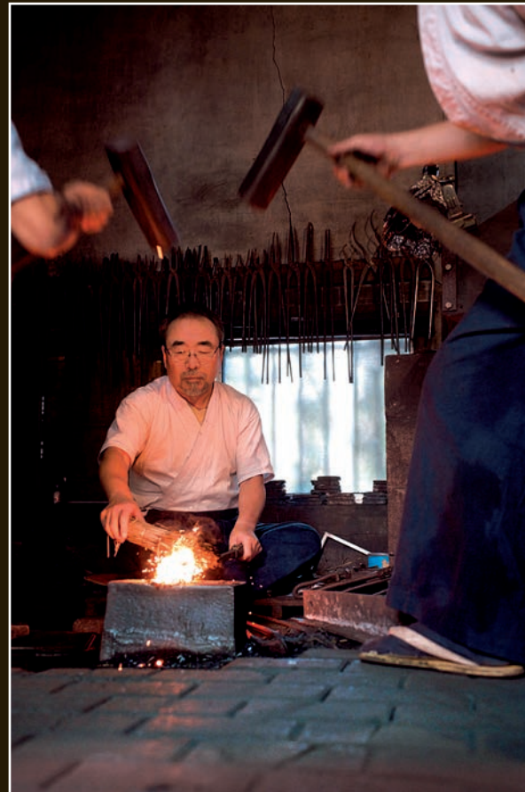
Hammering the tamahagane into a single mass.
