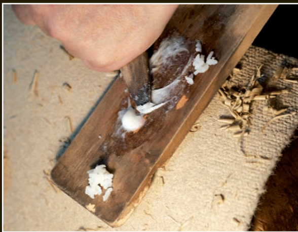
Compressing the rice into a paste to make sokui glue.
