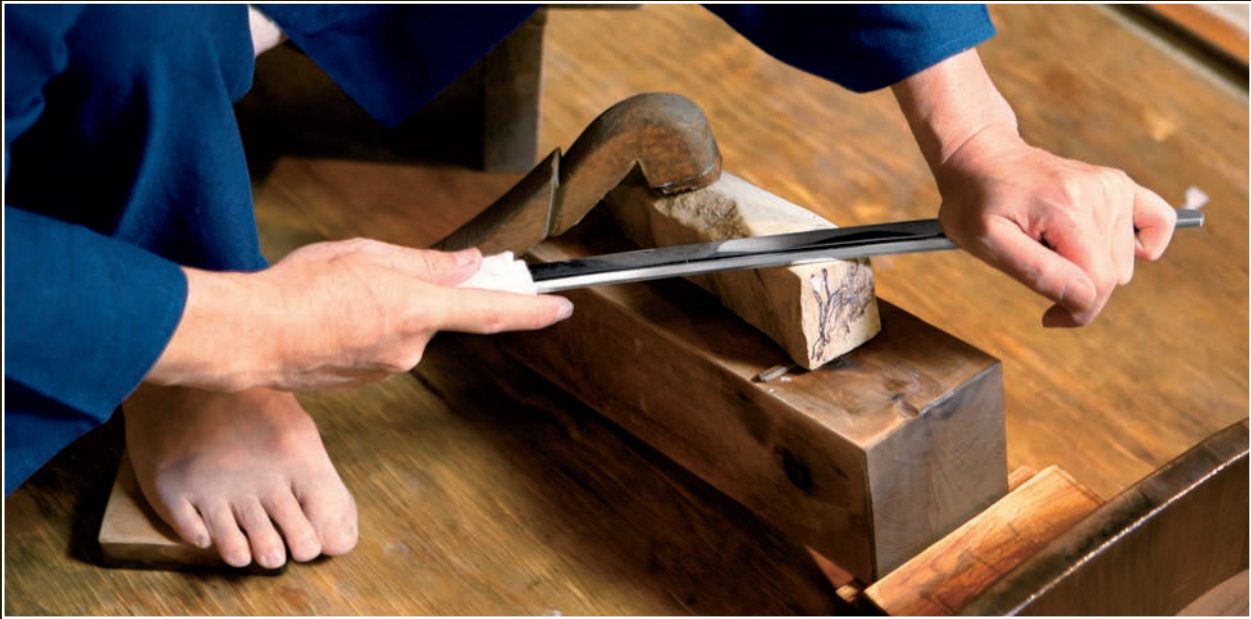
Takaiwa polishes a wakizashi. A rag protects his right hand and provides a grip while the left hand holds the bare blade. The very precise grip allows him to determine the exact part of the sword's surface that makes contact with the polishing stone.
