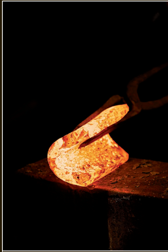
The kawagane plate is continually forged until it has a narrow U shape.
