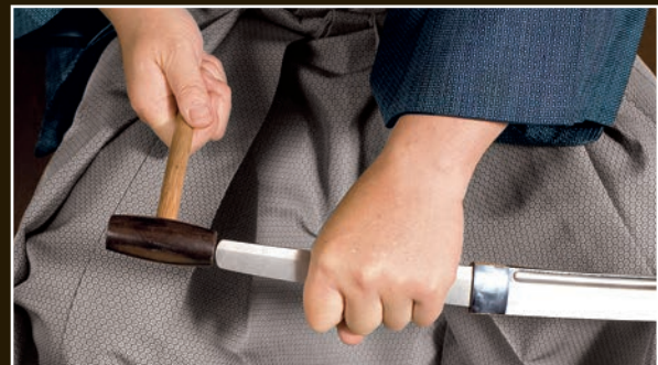
Sometimes a habaki is wedged very tightly on the tang of the sword and cannot be removed. In this situation, the bare tang is held in one hand while its base is tapped with a wooden hammer or mallet (using a steel hammer could bend or damage the tang). Several strikes with the mallet will usually loosen the habaki.
