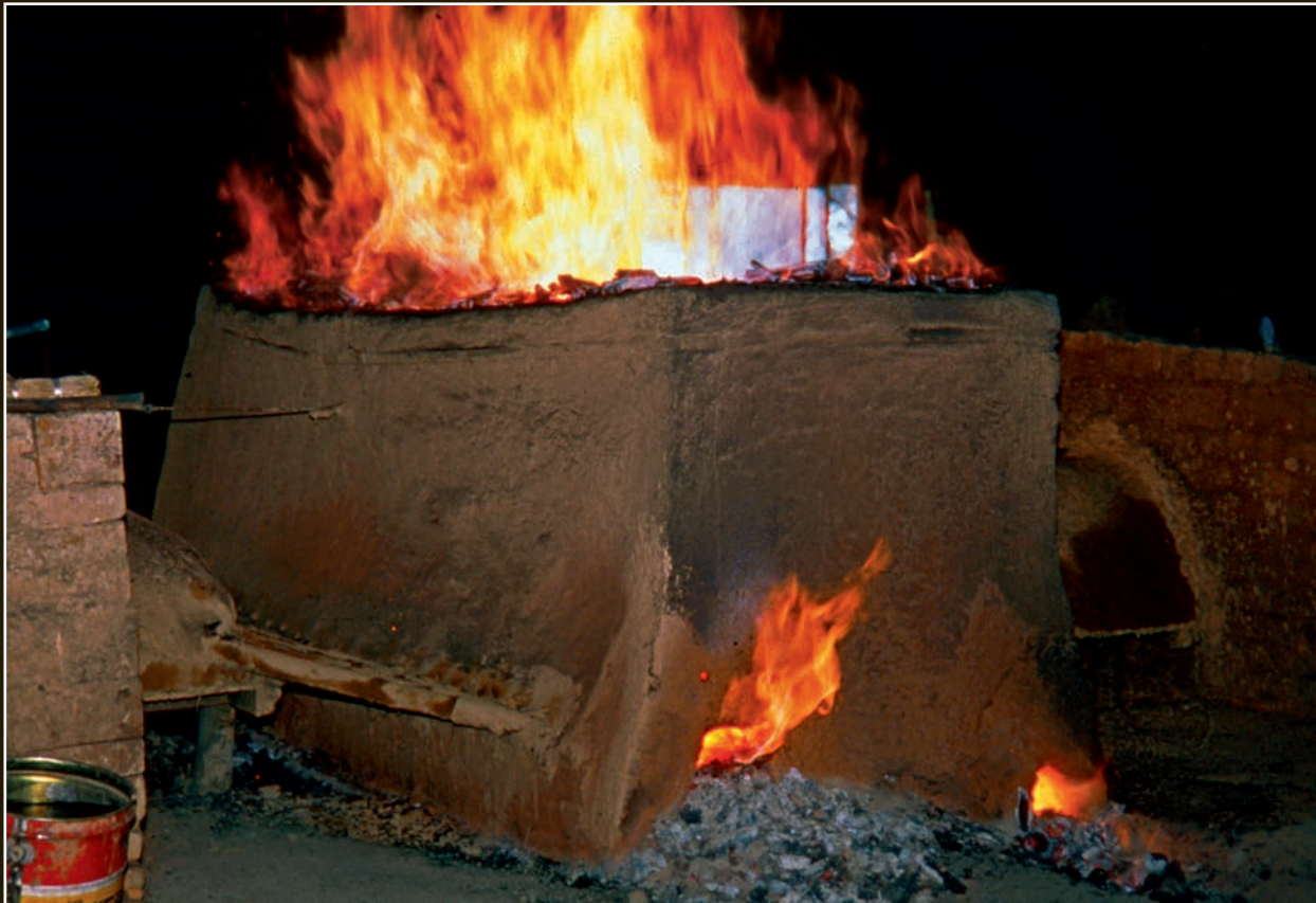
The tatara furnace in action. The furnace is filled alternately with charcoal and iron sand; the operation continues until a set amount of charcoal and iron sand is processed. The slag—impure material that melts at lower temperatures than iron and steel—will run out from the slag holes at the bottom of the tatara, where flames are emerging in this photo.
