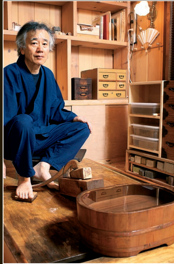
Takaiwa sits on a small stool on the togi-dai. The oke (water bucket), stone, and fumaegi (clamp) are all visible.
