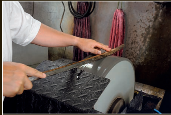
Using a water-cooled grinding wheel to clean and shape the blade after yaki-ire .
