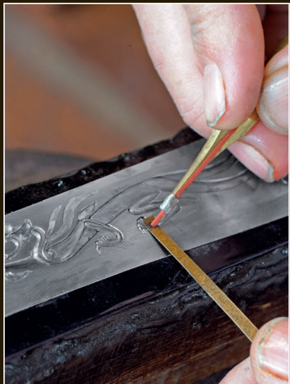
The inner surfaces of the horimono are sanded down with small strips of fine sandpaper. The sandpaper is held and guided with a small piece of a synthetic polishing stone.
