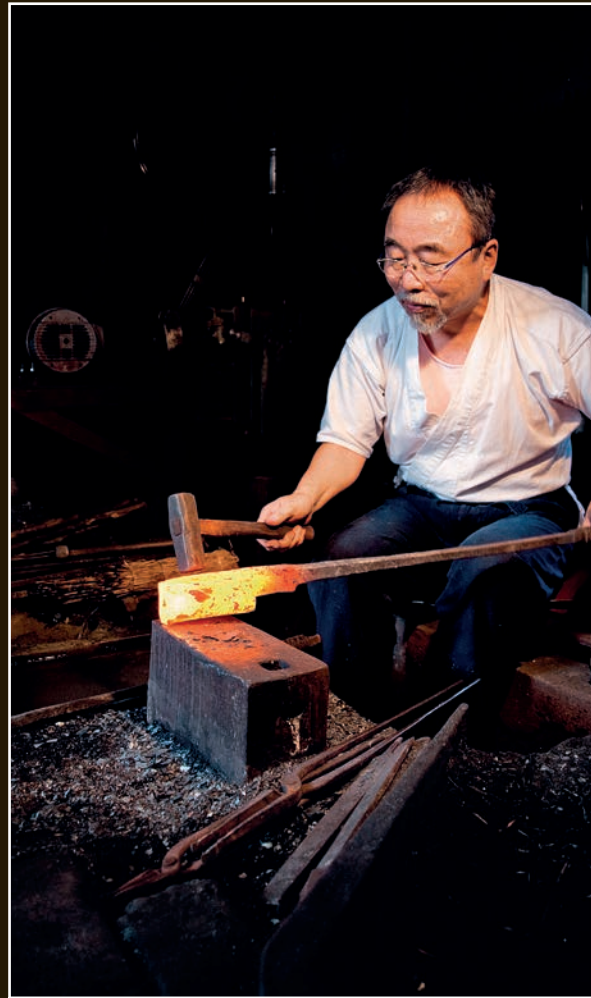
Yoshindo forges the kawagane and the shingane so that the two pieces of steel fit together seamlessly.
