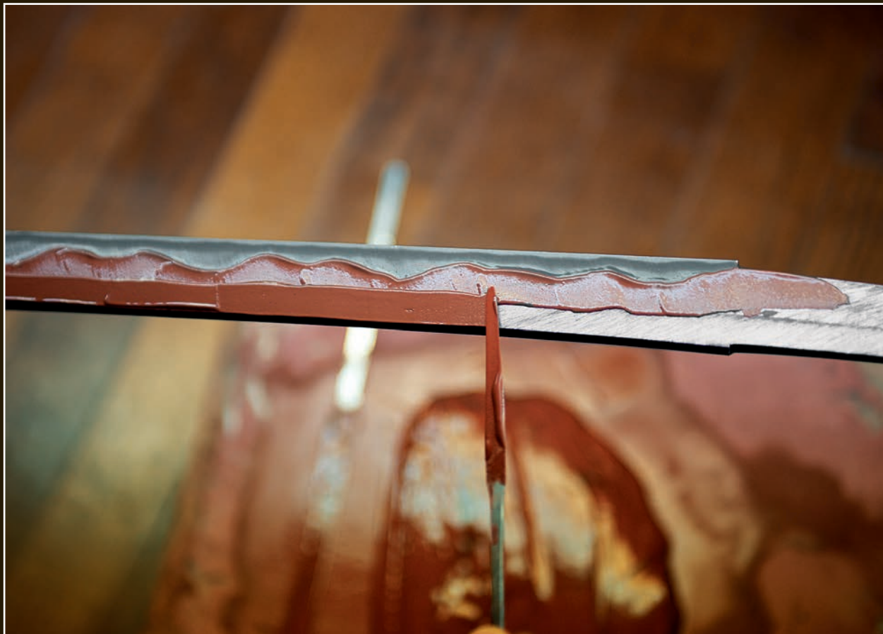
The red clay is spread down to the border of the black clay and on the remaining surface area of the sword. The entire blade must be covered with clay before yaki-ire.
