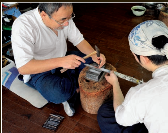
Yoshindo's student Mizuki holds the sword with the tang flat as Yoshindo inscribes the mei. The tang must be flat on the block at the proper angle for optimal results when inscribing the mei.
