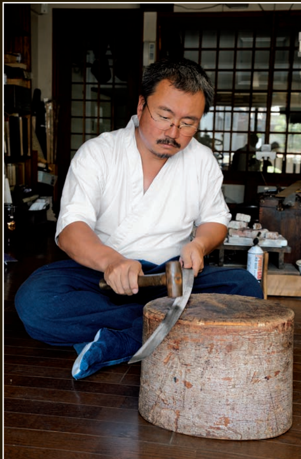
The curvature of the blade is adjusted by hammering.
