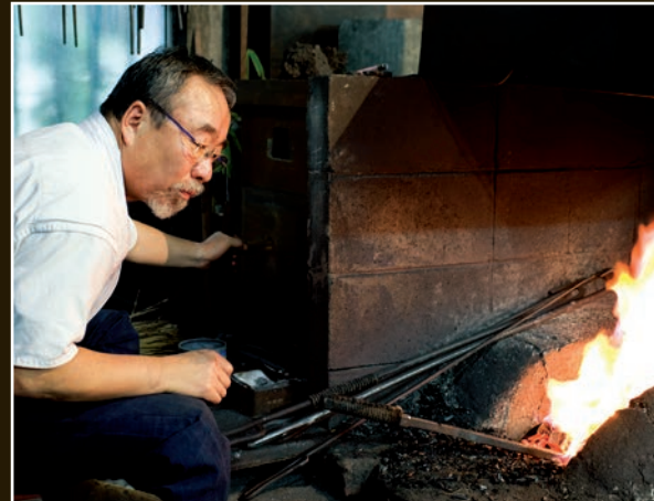
Yoshindo listens to the sound of the forge. This helps him determine when to end the smelting process.
