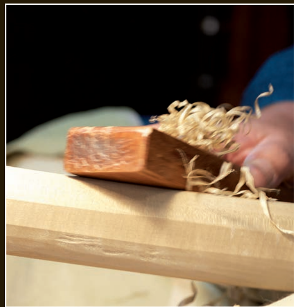
Okumura is using one of the smaller planes here. The shavings are becoming finer and the surface smoother.
