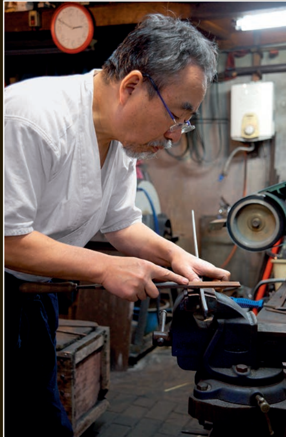
The mune and the cutting edge are finished with a file.
