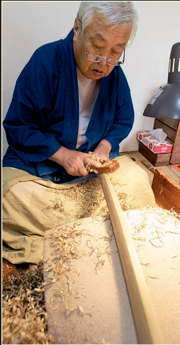
As he does the finishing, Okumura ensures that the lines and surfaces are straight and continuous along the entire length.
