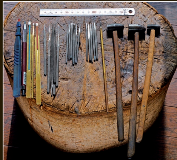
The various hammers, chisels, and other tools used to make horimono.
