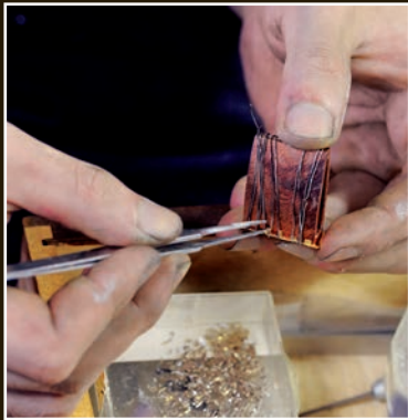
The gold foil is held securely in place with iron wire.
