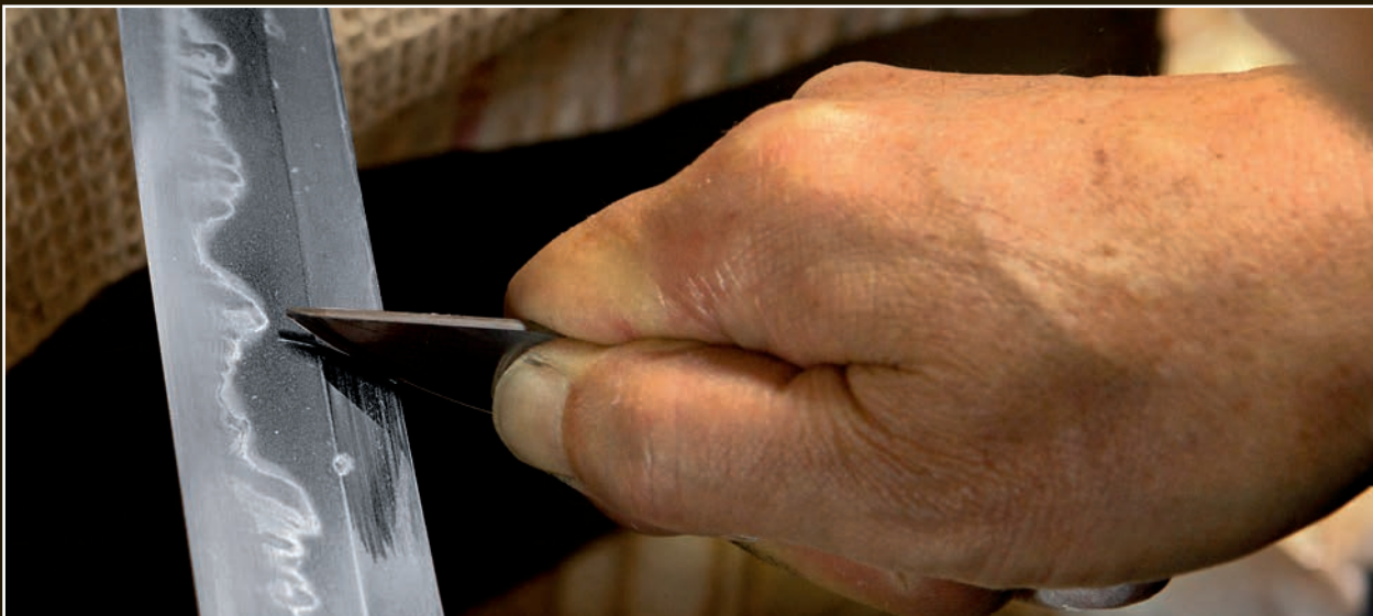
The first burnishing step is done with a migaki-bera, or burnishing spatula. The entire shinogi-ji and mune are burnished in 2-inch (5 cm) sections. The burnished section can be seen just below the burnishing spatula.
