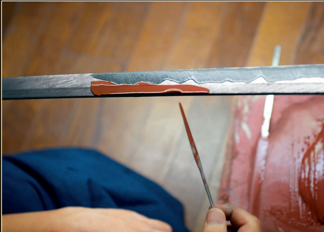
Yoshikazu applies the red clay to the upper part of the blade, which will not be hardened. The clay is applied with a small spatula and then spread down to the boundary of the black clay.
