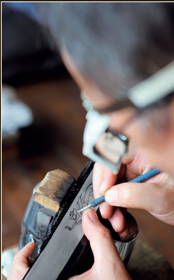
Yoshindo carefully draws the image to be engraved—a tiger—onto the blade.
