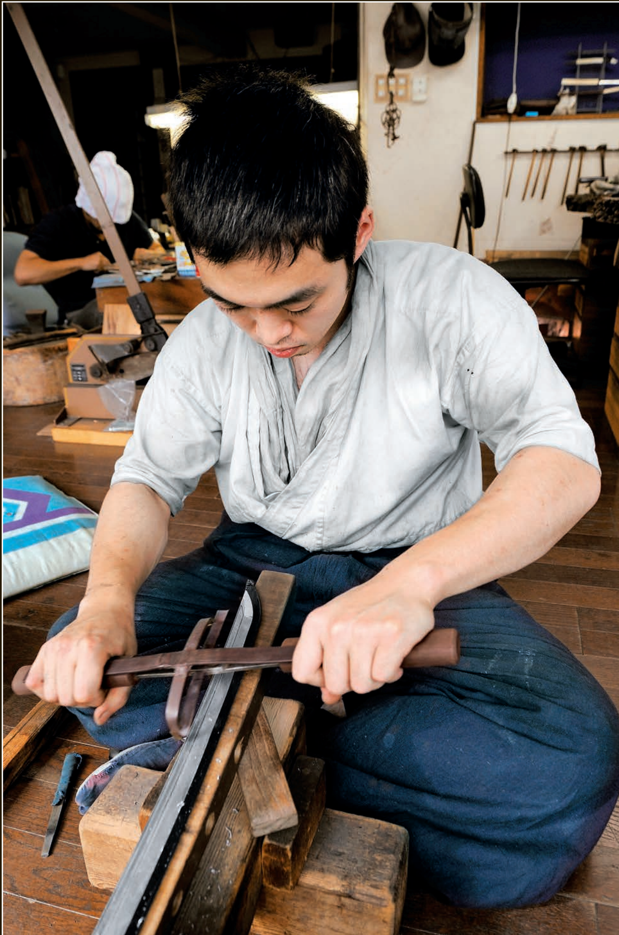
The blade is wedged securely between two pieces of wood to hold it in place while the groove is cut. The position of the new groove is marked in black ink.
