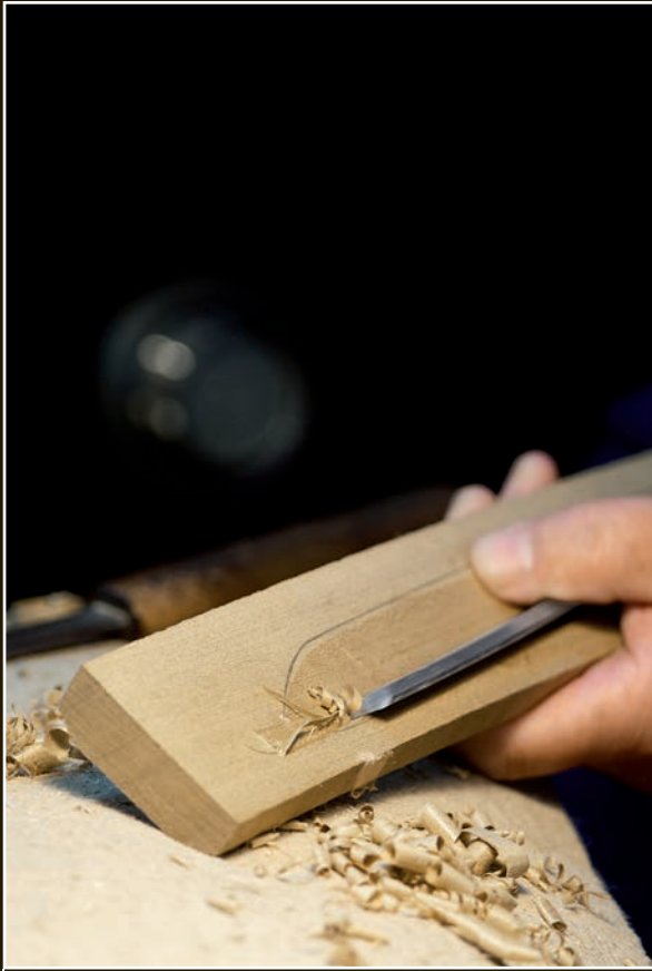
The space for the point is carved out carefully.
