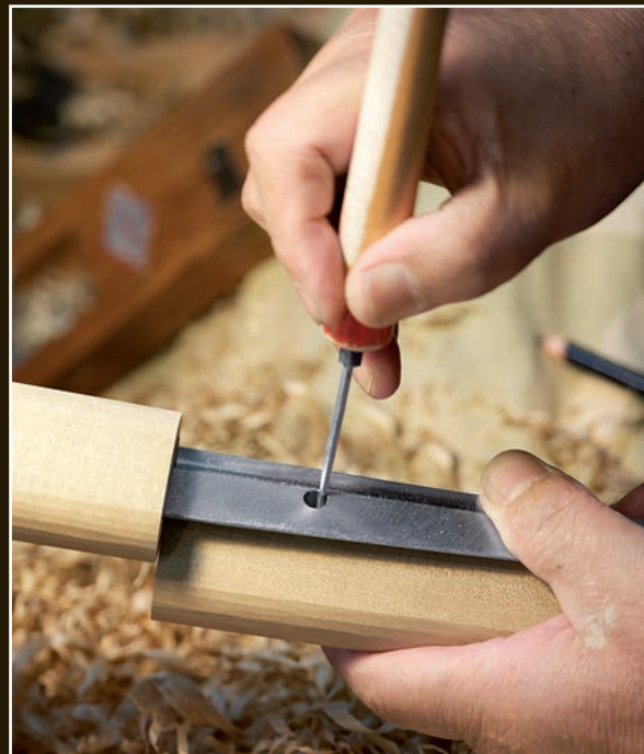
Starting to drill the mekugiana (rivet hole) in the hilt of the shirasaya.
