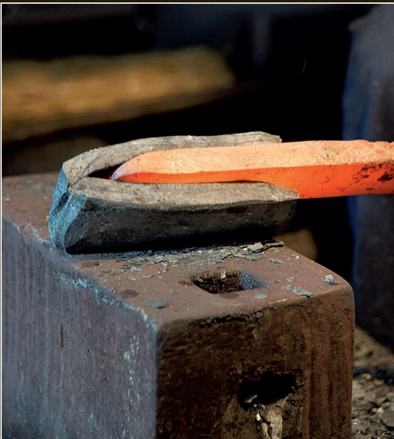
The shingane is fitted into the kawagane.
