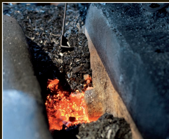
The center of the forge. The charcoal banks and the tuyeres are visible.
