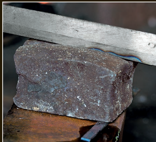
The sword is placed on the block at a third spot. A bit of curvature will appear wherever the sword has contacted the copper block. The three black areas show where the sword was placed on the block each time.
