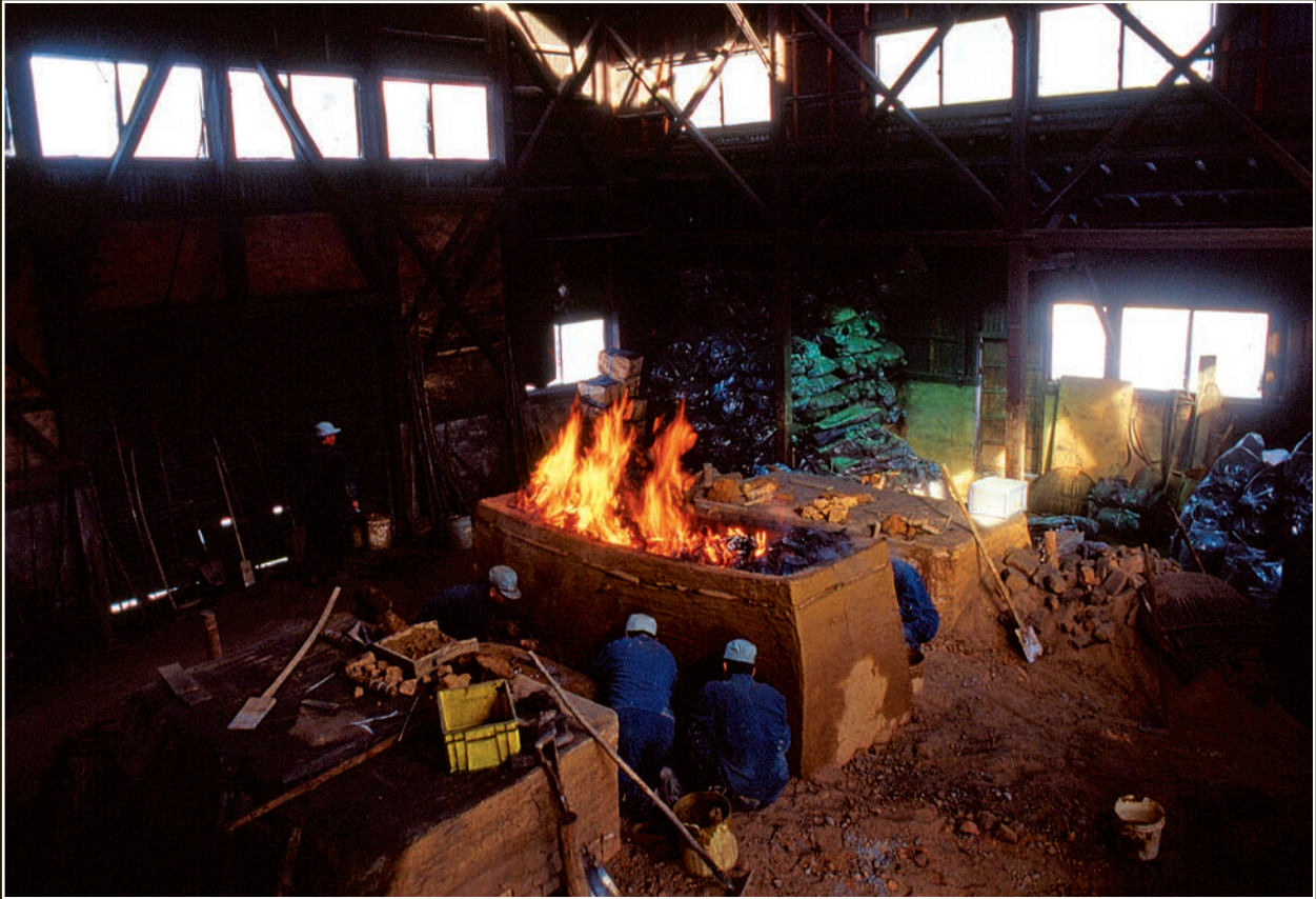
The operation of the tatar begins. The workers at the bottom of the tatar are checking the air ducts to insure that they are working properly and are unobstructed.
