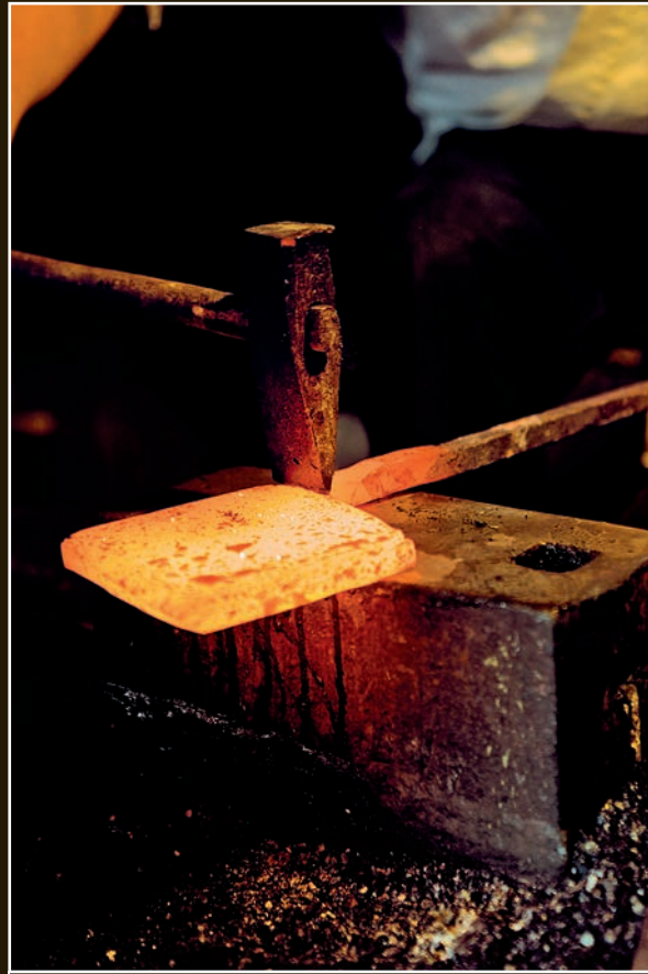
The handle is removed from the kawagane plate.
