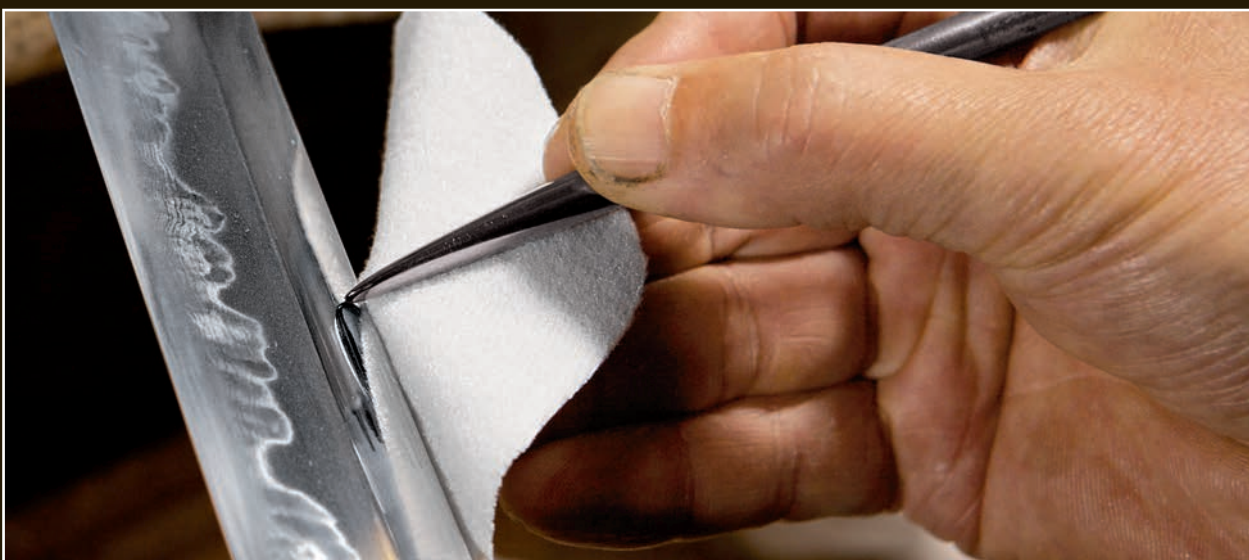
The second step of burnishing uses a migaki-bo (burnishing needle). Takaiwa keeps a piece of cotton cloth between his hand and the steel surface to protect the steel finish and allow the needle to move easily. The newly burnished section is visible around the burnishing needle; the needle and the cloth are clearly reflected in the burnished surface.
