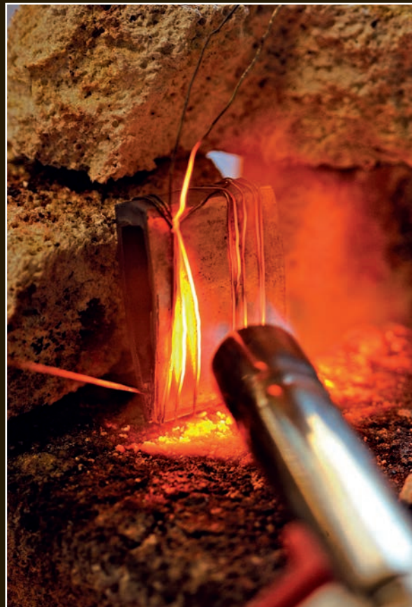
The insert, held in place with iron wire, is soldered into place in the habaki.
