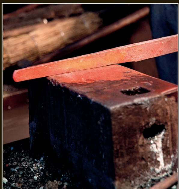
The end of the steel bar has been shaped to form the tang.
