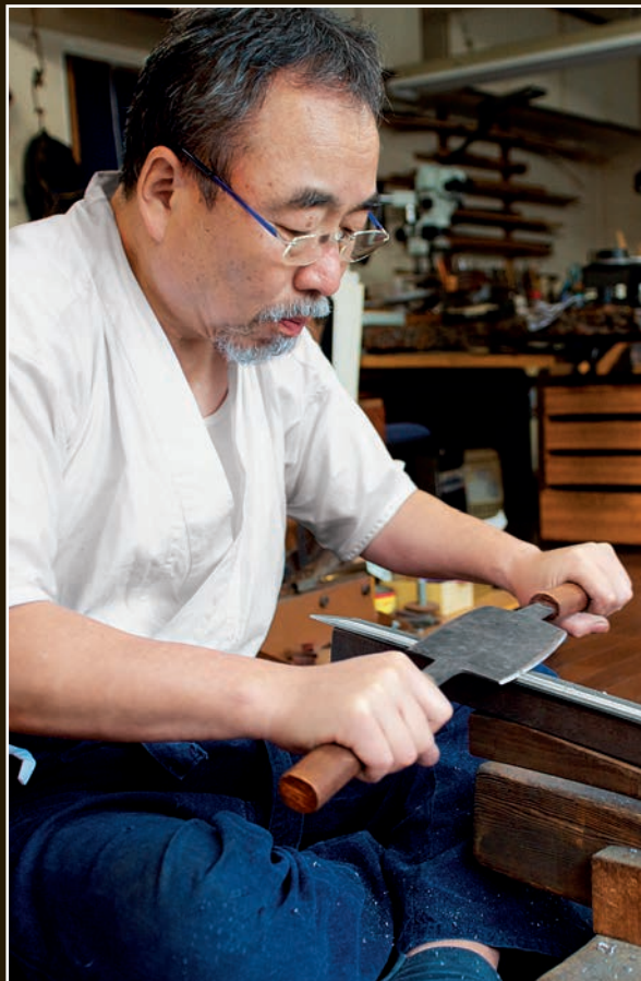
The sides of the blade are finished by shaving it with a sen, a drawknife made from hardened steel.
