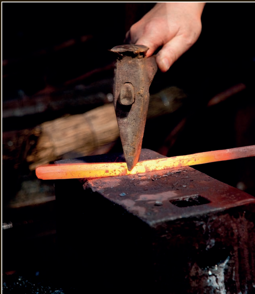
A chisel is used to cut partway through excess steel at the end of the bar.
