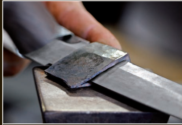
The narrow edge of the habaki is forged closed. Notice that the habaki is being fitted about 0.5 inches (1 cm) below the hamachi and munemachi at the base of the blade.
