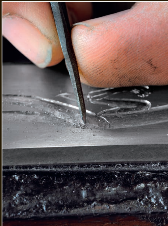
Yoshindo uses very fine small chisels to carve the surfaces of the horimono to a smooth finish. He shapes the points on all of these special chisels himself.
