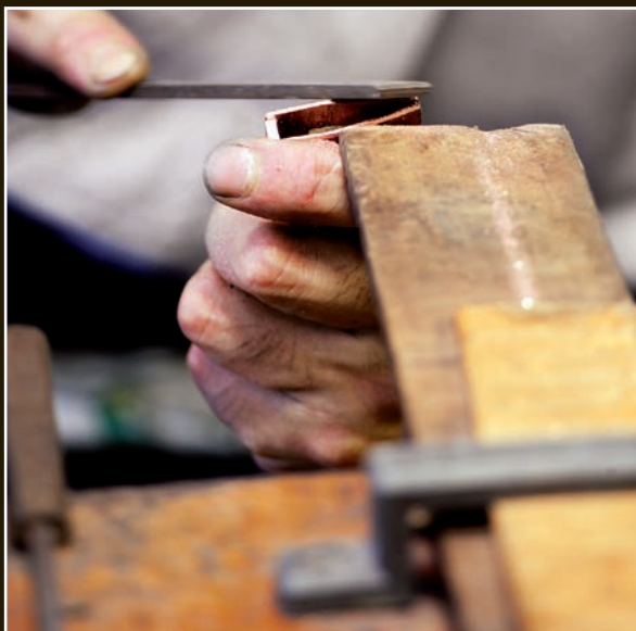
Filing the surface of the habaki that will be closest to the hilt.
