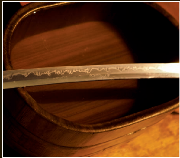
After nugui is applied, the ji has a darker tint, and the hamon outline is very clear.
