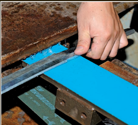
Using a water-cooled belt grinder to begin polishing the blade, starting from the mune-machi and working toward the point. Notice the water dripping down on the belt to keep the sword cool. If the blade becomes too hot, the hamon could be damaged.
