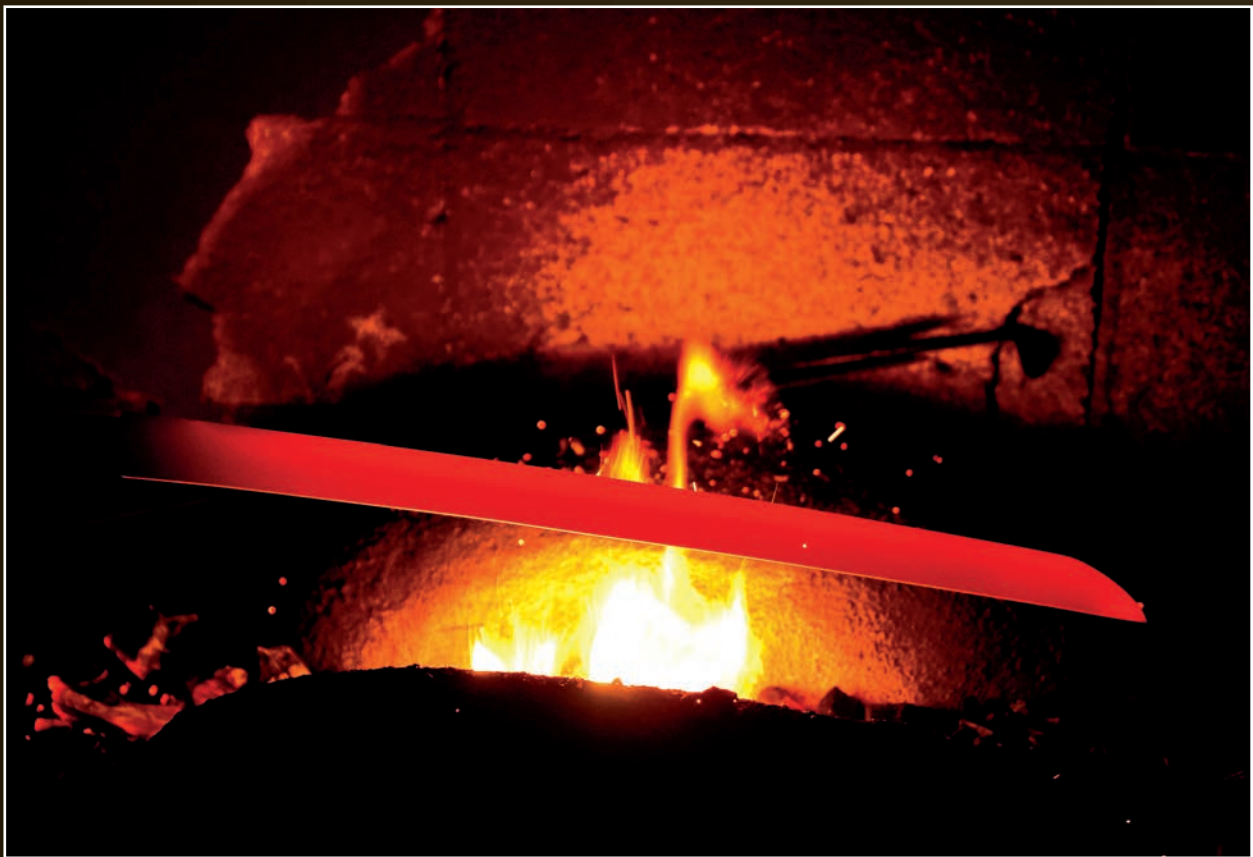
An uncoated blade, held edge-up, is heated in the forge for hadaka-yaki. Careful heating is essential for this process to work. The body of the blade is a dark red, while the edge is much brighter. Before quenching, the edge should be 1380 to 1470°F (750–800°C); the body must be 1130°F (720°C) or cooler.
