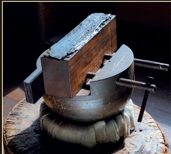
A vise is used to hold the sword in place as it is engraved. The surface is covered with a hard black paste made from pine sap and charcoal. The black surface is heated gently with a torch, and the sword is pressed right onto it. The sword can then be moved into any convenient position for engraving work.
