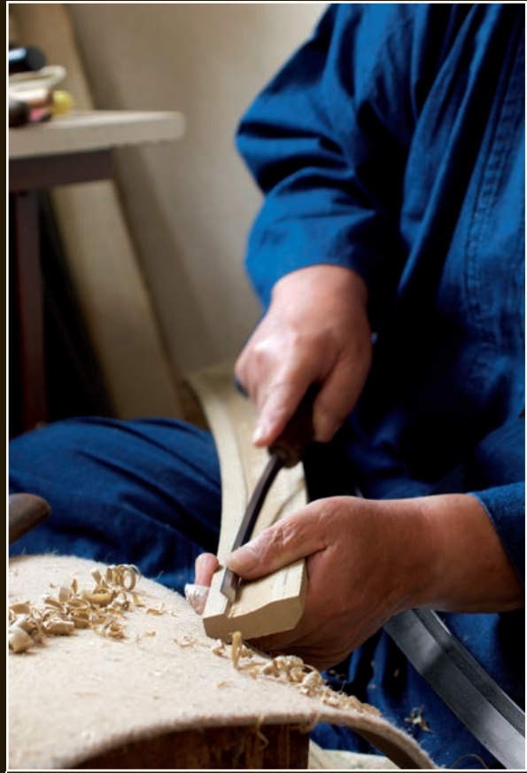
Shaping the mune side of the saya's interior.
