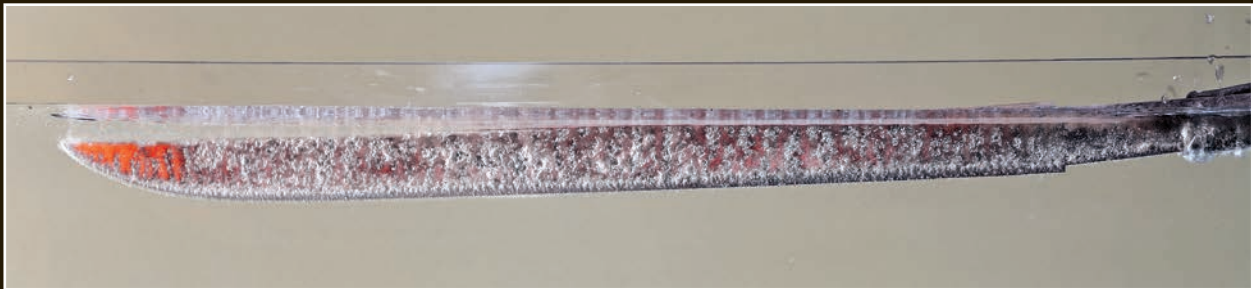
The blade 0.4 seconds after entering the water. A dense layer of bubbles forms along the edge. Numerous bubbles can also be seen along the sides of the blade up to the mune.
