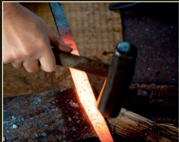
Yoshindo hammers on the edge of the anvil to begin forming the cutting edge.
