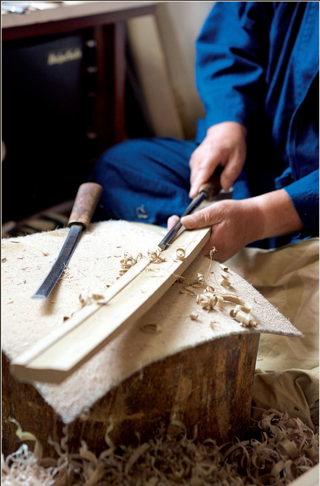
Working on the mune surface of the saya's interior.
