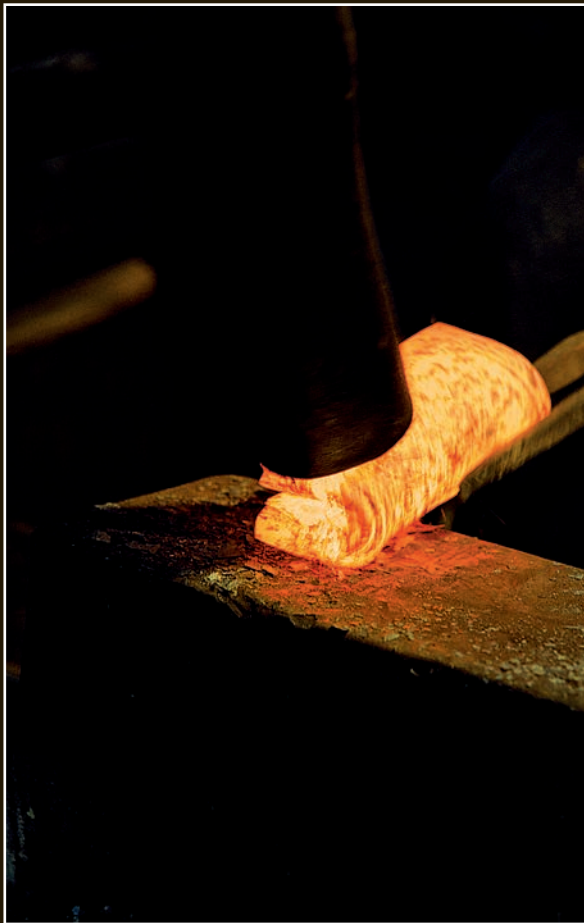
The U-shaped plate is hammered shut at one end.
