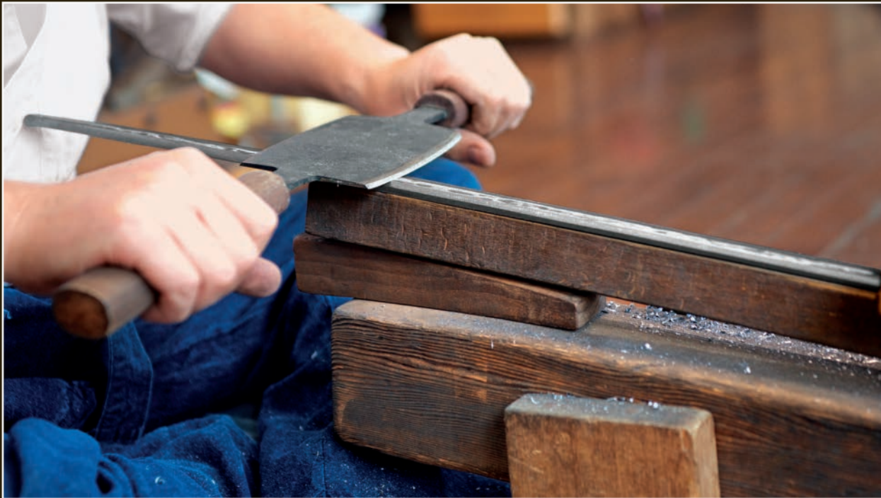
Using a sen to shape the new sword. The steel above the shinogi is white where it has been shaved with this tool.
