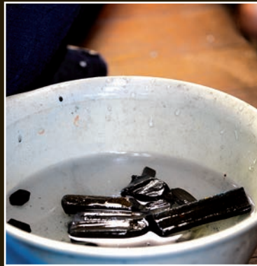
Charcoal made from ho wood is soaked in water before being used to clean up the habaki surfaces.
