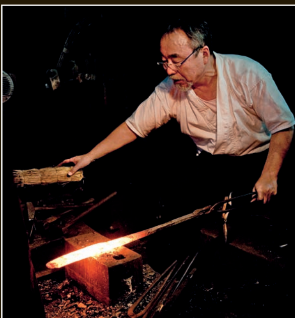
Drawing out the steel into a longer bar. The handle has already been cut off here.
