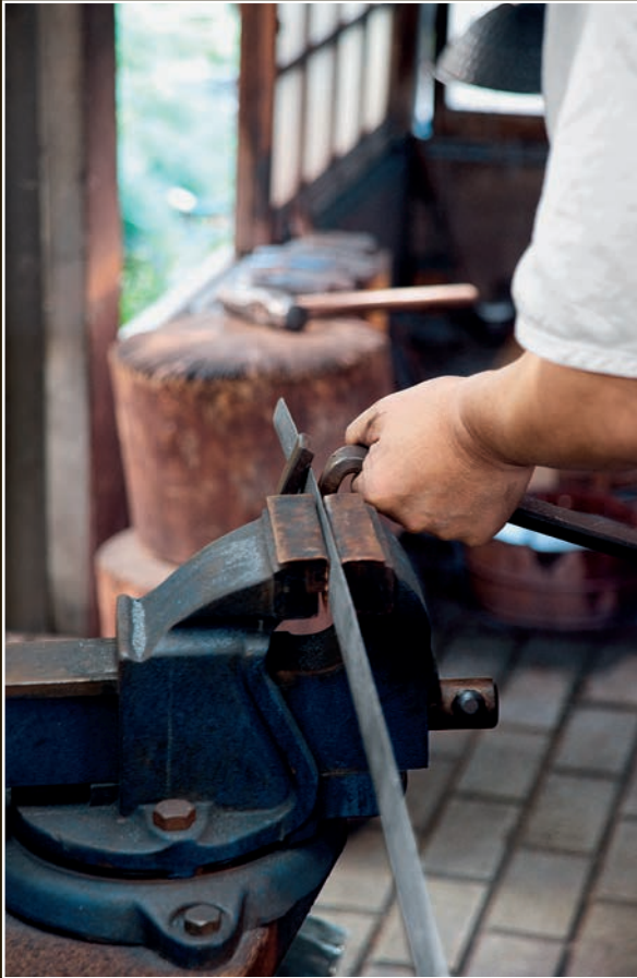
Using a U-shaped iron bar to correct a twisted area on the blade.
