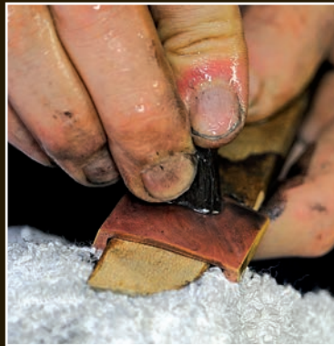
Soft charcoal is used to clean up all the shakudo and gold surfaces on the habaki. The habaki is held on a wooden blade during the final steps.
