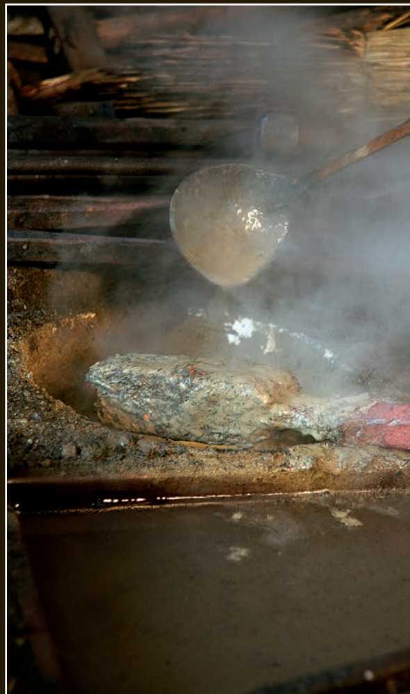
The steel is removed from the forge and covered with a clay slurry, and is then returned to the forge.
