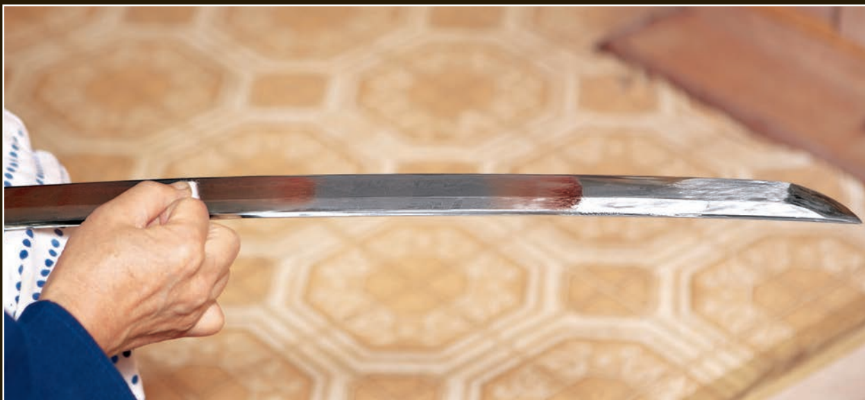
Takaiwa rubs the nugui over the blade's surface using a piece of cotton (visible under his thumb). His forefinger and middle finger are braced against the mune surface as he works.
