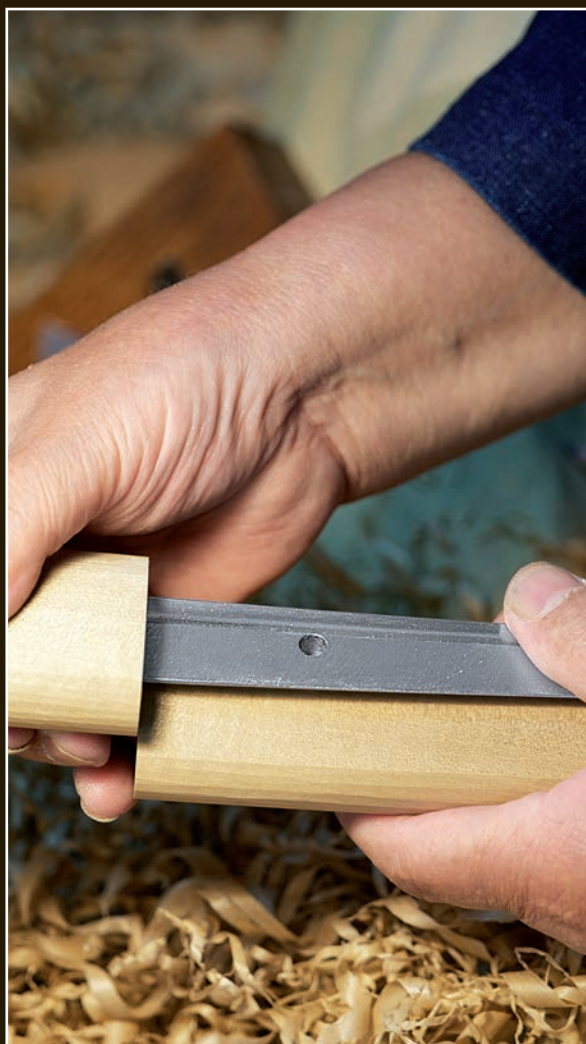
The hilt is held against the top of the saya so the correct spot to drill the mekugiana in the hilt can be determined. The mekugiana in the wood hilt must be in exactly the same place as the one in the tang of the sword.
