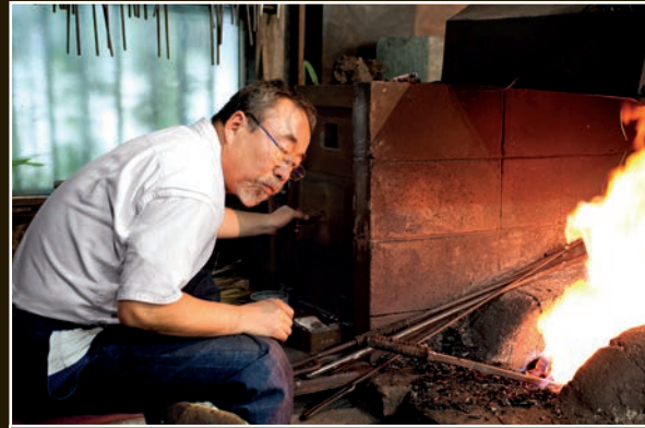
Yoshindo can judge when the tamahagane is hot enough to be welded into a single mass by listening to the sounds from the forge.
