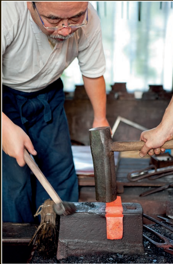
Yoshindo holds the billet as his apprentice folds it over with a sledgehammer.
