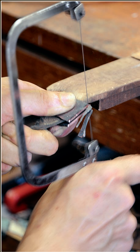
A jeweler's saw is used to cut excess metal from the open end of the habaki.
