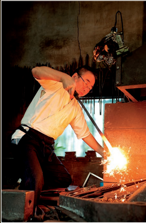
Removing the hot tamahagane from the forge.
