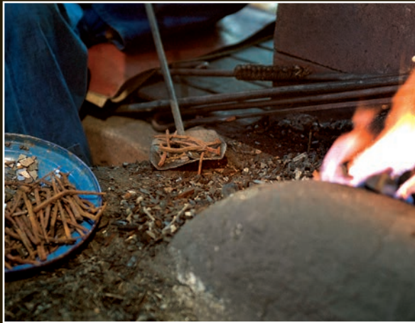
The salvaged iron pieces are ready to be placed in the forge.
