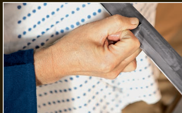
The hazuya (under Takaiwa's thumb in the photo) is used to polish a small section of the blade. The blade surface is acquiring a uniform whiteness, and the hamon is clearly visible.
