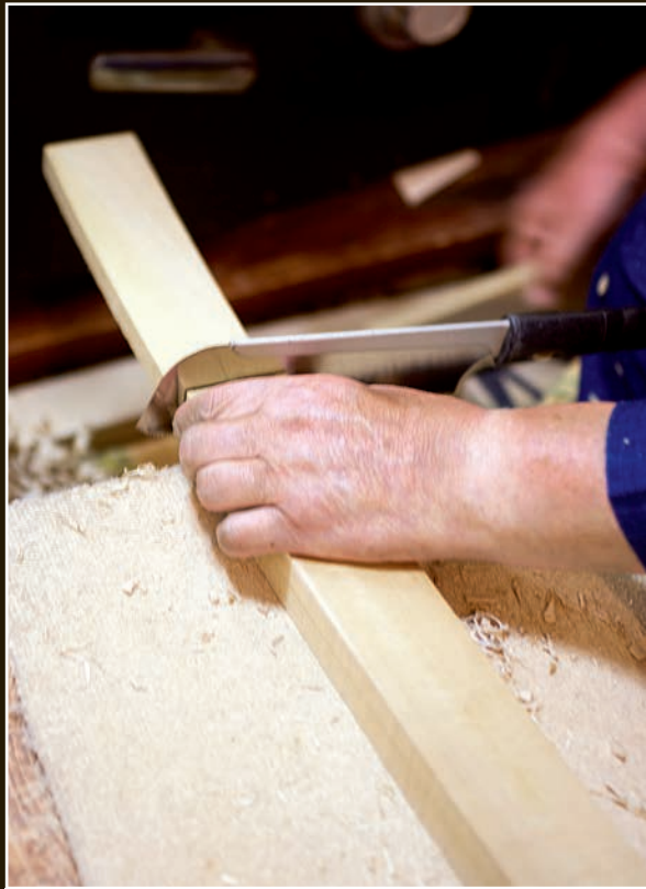
Cutting off the hilt from the saya blank.
