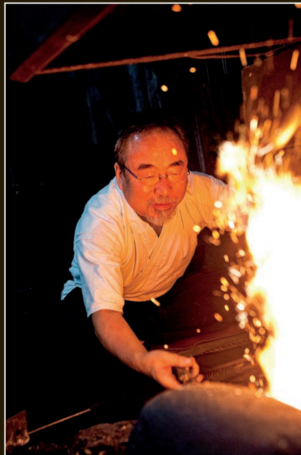
The billet of tamahagane is heated until it is ready to be forged.
