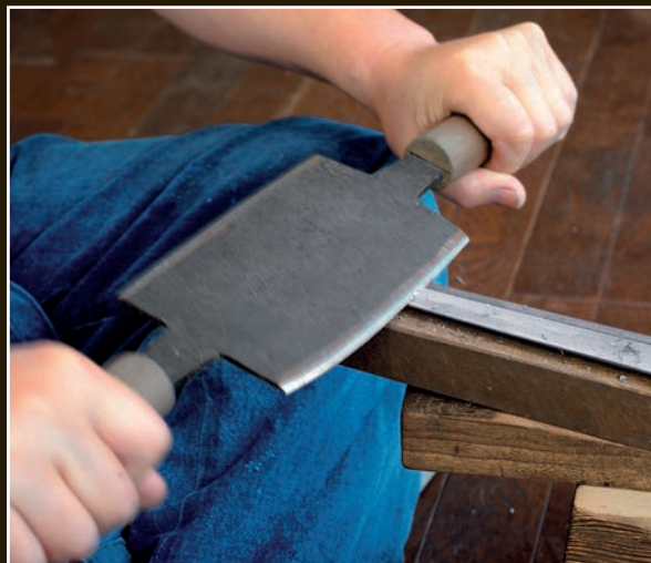
Using a sen to clean and shape the tang.
