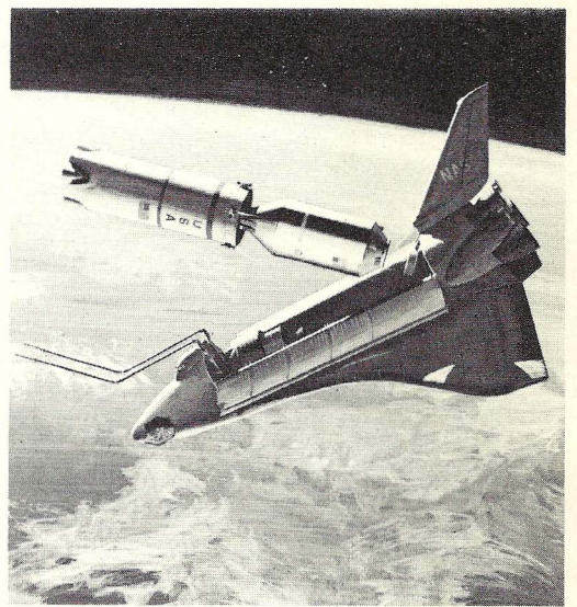
The space shuttle, shown with the cargo bay opened, will be able to deliver up to 65,000 pounds of varied payload into orbit in its 15 by 60 foot cargo bay. These drawings show the payload (a satellite) being pulled away from the cargo bay by a command-controlled space tug for precise orbital placement. The shuttle will be developed by the North American Rockwell Space Division under a six-year, estimated $2.6 billion contract.
