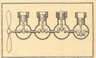
Showing how a four-cylinder engine drives the crankshaft which is directly connected to the propeller shaft which rotates the propeller. The arrows show the direction of motion of the pistons. pistons.
