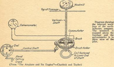
(The diagram below will illustrate the principle of the earth-inductor compass. It consists of three parts, a generator, a control and a galvanometer. The parts of the generator are shown as the commutator, brush and coil. The generator is operated by a windmill, the force of the wind against the vanes rotating the vertical shaft. The pilot sets the control dial
