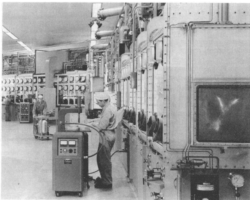
View from entrance of fabrication area. Operator in foreground is using dielectric sealing equipment for removal of items from the hood line.
