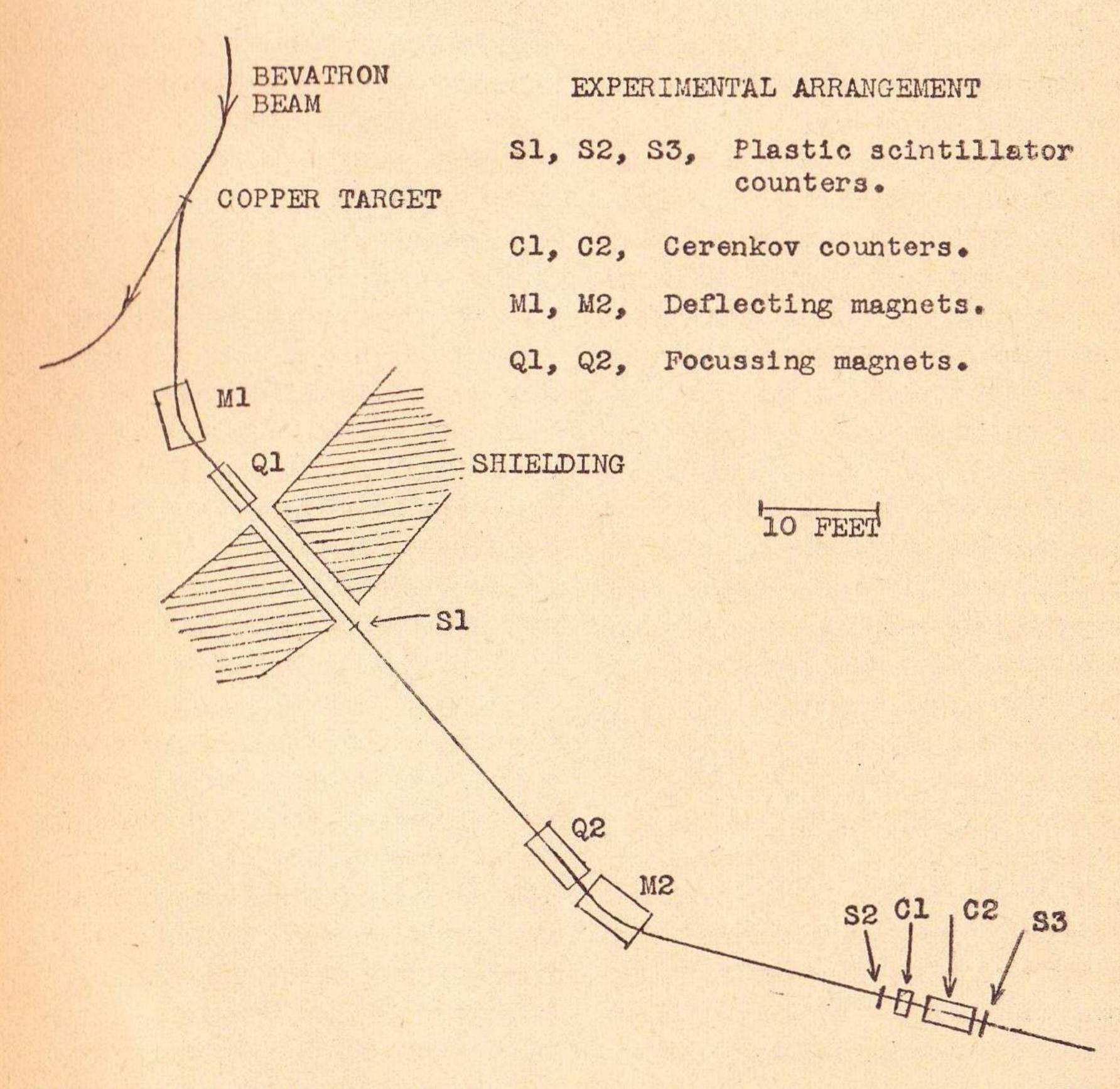
ed of plastic cylinders, 2.25 inches in diameter by 0.62 inches thick, mounted on very sensitive photo-electric tubes. The plastic is of a special type which fluoresces upon being struck by radiation. Whenever a high speed charged particle passes through one of these cylinders, a little scintillation of light is produced which is picked up by the phototube and converted into a little pulse of electricity. This can be amplified and counted.
