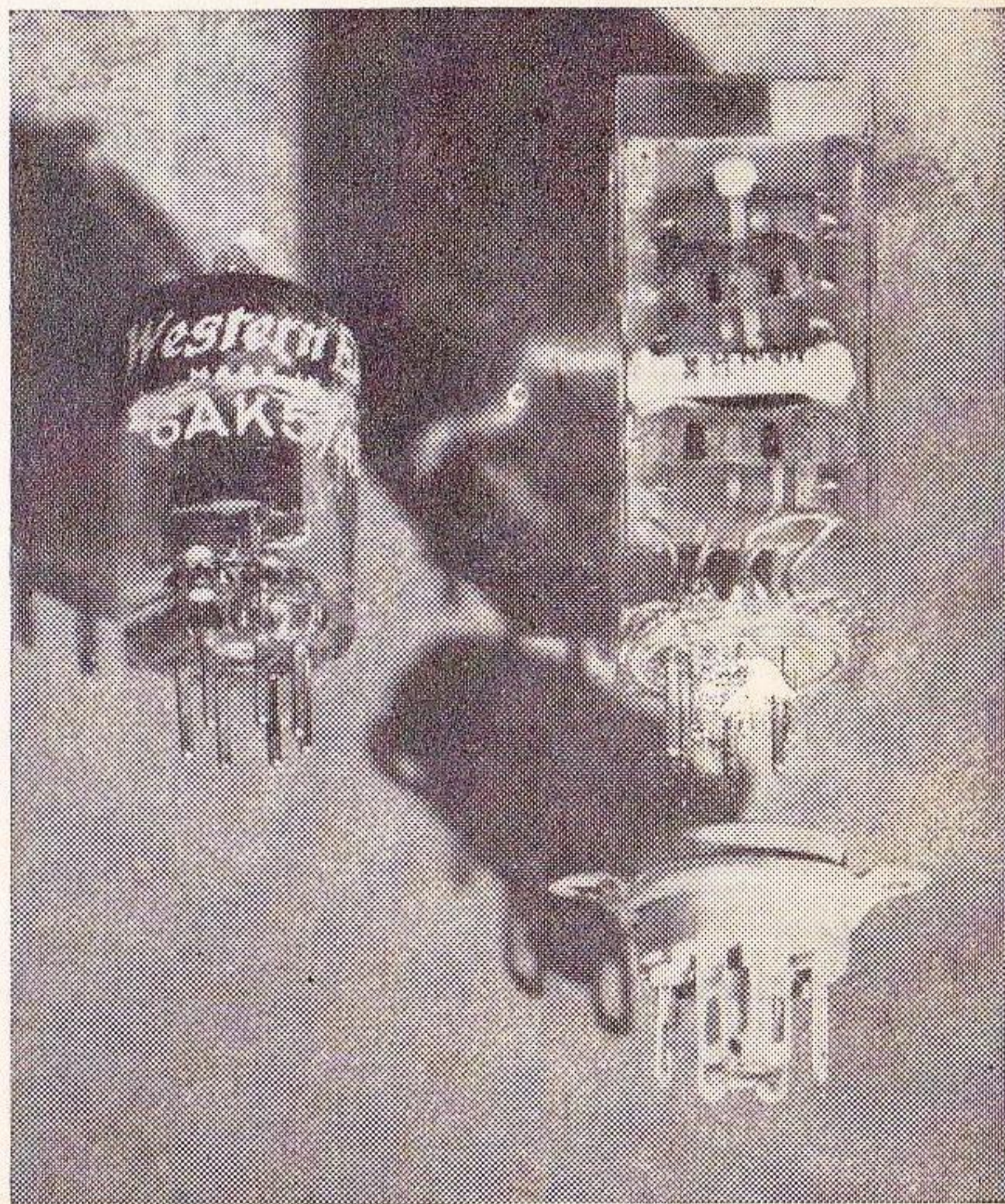
A packaged bit register, which stores one bit or unit of information, together with its socket and a 6AK5 miniature vacuum tube.
