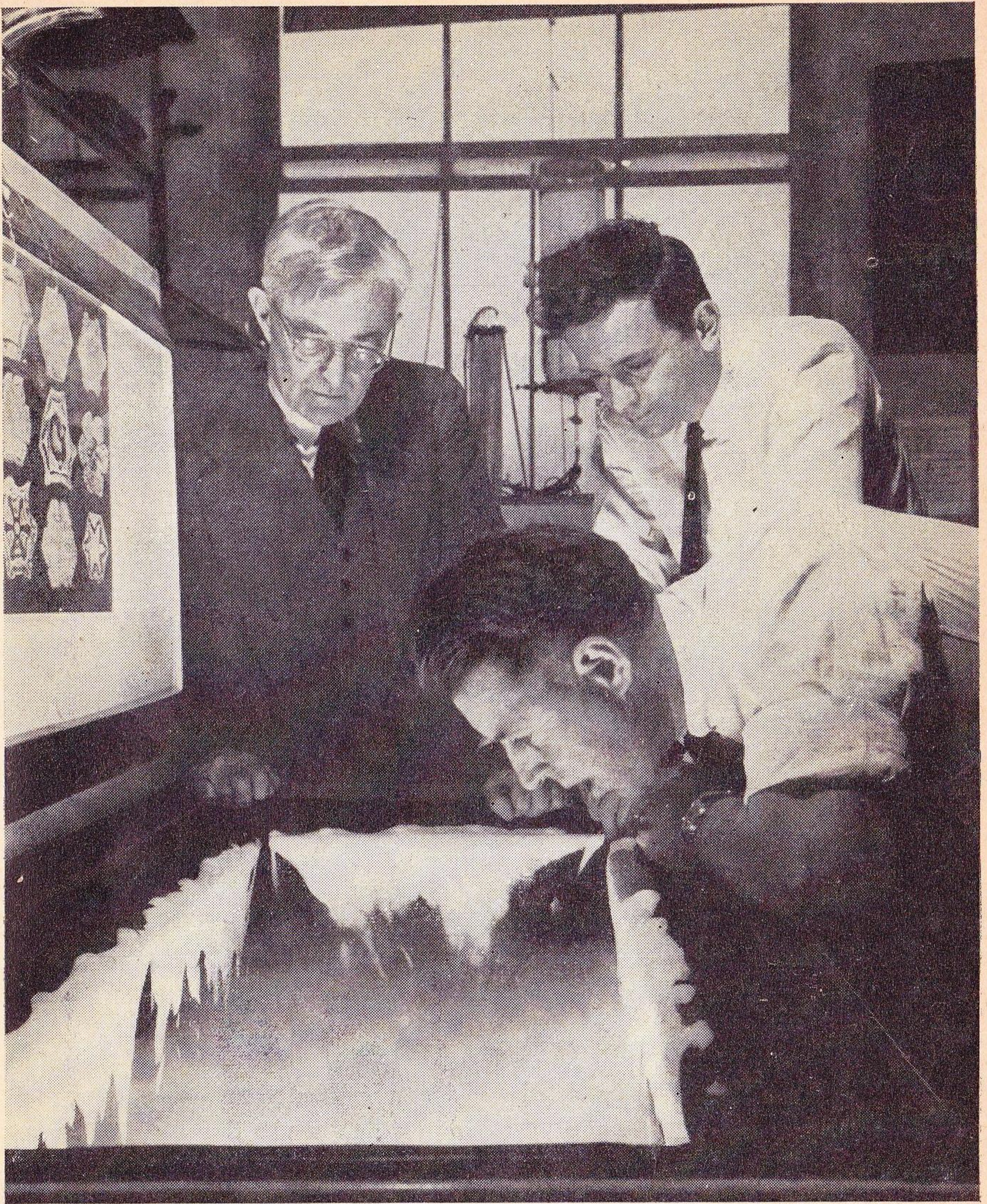
"BIG THREE" IN SNOWMAKING. Vincent J. Schaefer, weather scientist of the General Electric Company's Research Laboratory, prepares to make a miniature snowstorm in a Home Freezer in his laboratory, while Dr. Irving Langmuir, at left, and Dr. Bernard Vonnegut watch. Schaefer first produces a supercooled cloud in the freezer by blowing in his breath. A few small particles of dry ice, dropped into the freezer, then turn the supercooled cloud into snow.
