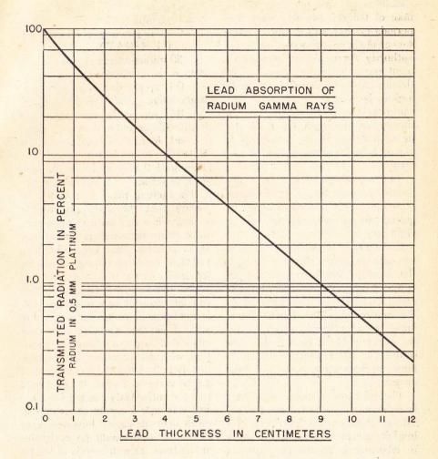
The protection afforded by a 11/2 inch lead storage container for a one milligram radium source is as follows: The radiation at 11/2" (3.81 cm) is 1270 mr/hour (see formula in text). A lead storage container 11/2" provides an eighty-nine percent radiation reduction. Neglecting the fact that the radium intensity of 8200 mr/hr is at one cm, the radiation outside the storage chamber would be approximately 140 mr/hr.
