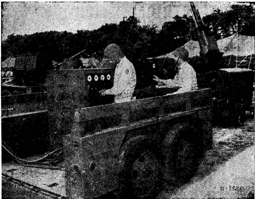
Fig. 1. The M-9 fire computer on station. The computer itself, with dials for setting in air pressure, wind, the other "given conditions" in the foreground. Background left, power supply truck. Background right, launching device for suicidal robots—VT fuzed shells!
