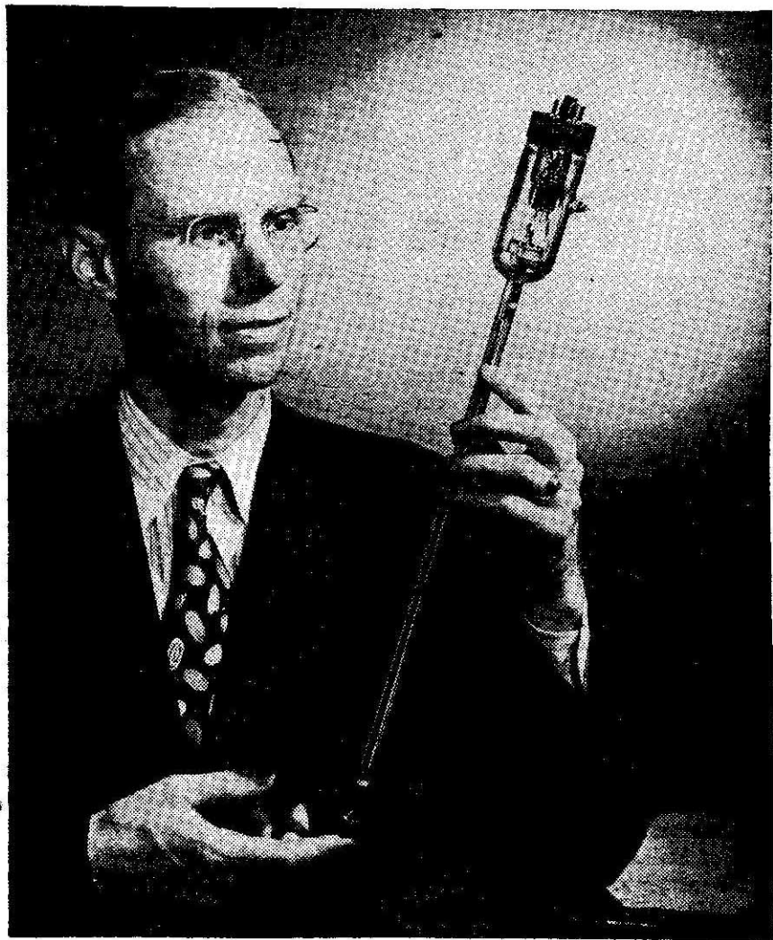
Figure 3: Bell Telephone Laboratories traveling wave tube extends the duration of interaction between electric wave and electron stream in both time and space so it can amplify a wider band.
