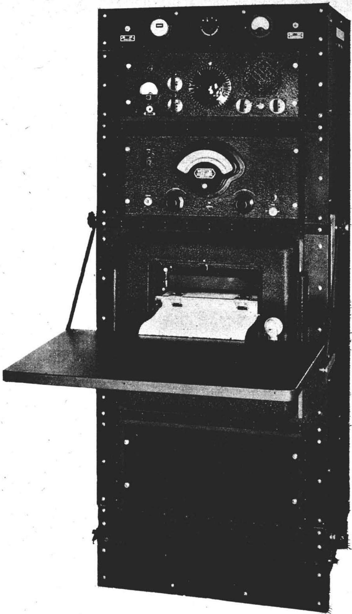
Ground instruments, designed to match the characteristics of the radio-sonde, record the radioed data.
