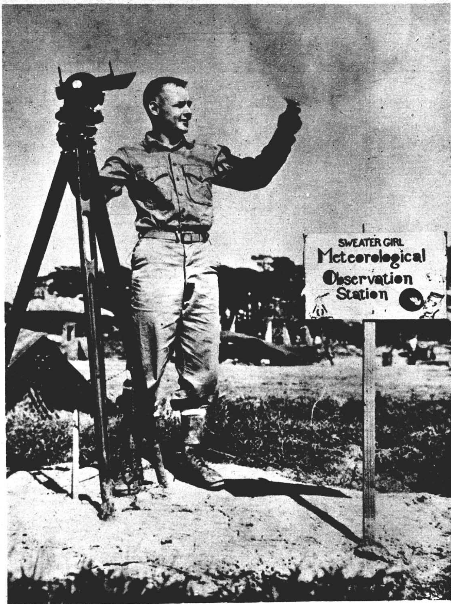
A Marine weather observer on Okinawa prepares to send up a sounding balloon. Following the rise and drift of the balloon by telescope is the older, and necessarily more common, method of testing weather conditions.
